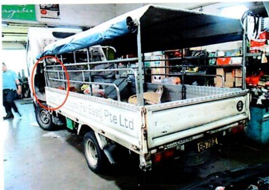
Photo 3 shows the left rear view of the Insured Vehicle at the time of our inspection. The exterior body of the Insured Vehicle was relatively unaffected by the incident except for the centre portion. The damage to the Insured Vehicle was confined to its centre portion. The damage was observed to be most severe at its left centre portion (circled).
