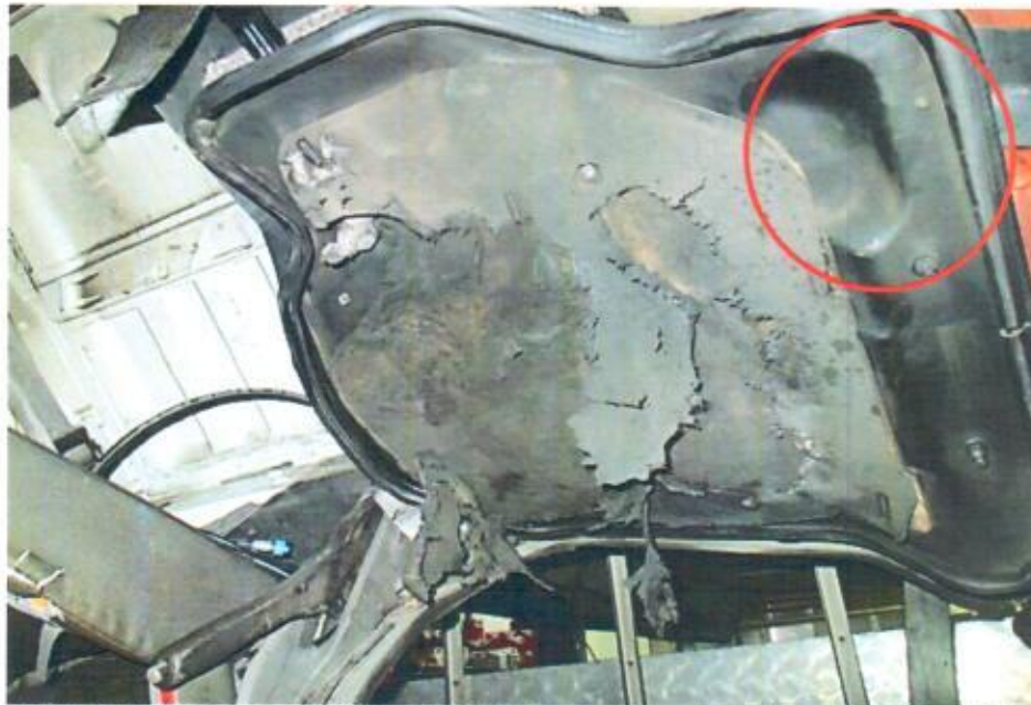
Photo 6 shows the whitish marks that were found on the underside of the passenger side engine access panel of the Insured Vehicle (circled). Such whitish marks are a result of exposure to prolonged heat intensity. Rust would also begin to develop on these areas soon after. The development of rust is an indication that the area was exposed to prolonged exposure to high heat intensity, which had caused the steel/metal material of the passenger side engine access panel to be exposed to natural environmental condition
