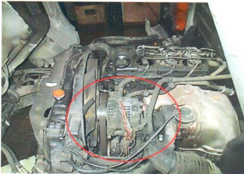
Photo 5 shows the engine compartment of the Insured Vehicle which is situated beneath the cab at the time of our inspection. The left portion of the engine compartment of the Insured Vehicle was significantly affected by the fire (circled).
