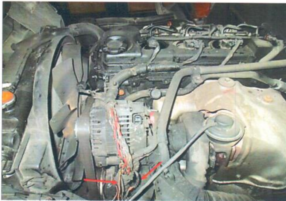
Photo 8 shows the wirings leading from the alternator of the Insured Vehicle. The wirings were original factory fitted wirings. We observed traces of greenish residue on these wirings (arrowed). The presence of such greenish residue indicates internal heating of copper wires, a sign of an electrical short circuit occurring. The greenish residue is normally left behind from oxidation as a result of chemical reaction involving the copper wires. This physical evidence would then appear to suggest that the cause of the smoke incident to the Insured Vehicle could have possibly been due to electrical in nature.
