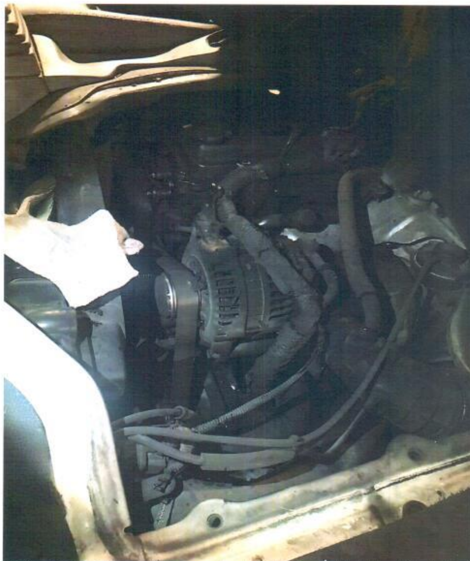
Photo 12 shows the engine compartment of the Insured Vehicle at the incident location post- incident. In general, the condition of the engine covered in soot had corresponded to the events that were related to us by Mr Lui, which is the smoke had emitted from the engine compartment.
