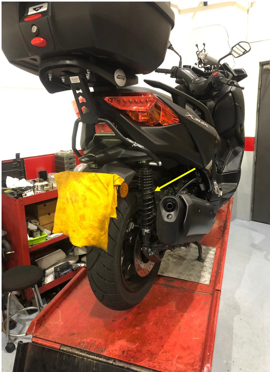
Photo 4 shows the rear right shock absorber (arrowed) of a similar make and model scooter as the Scooter for comparison purposes (photograph taken by Hong Leong Corporation Holdings Pte Ltd during their checks of the Scooter). The rear shock absorbers fitted on the Scooter were non-original. Refer to photograph 2 above
