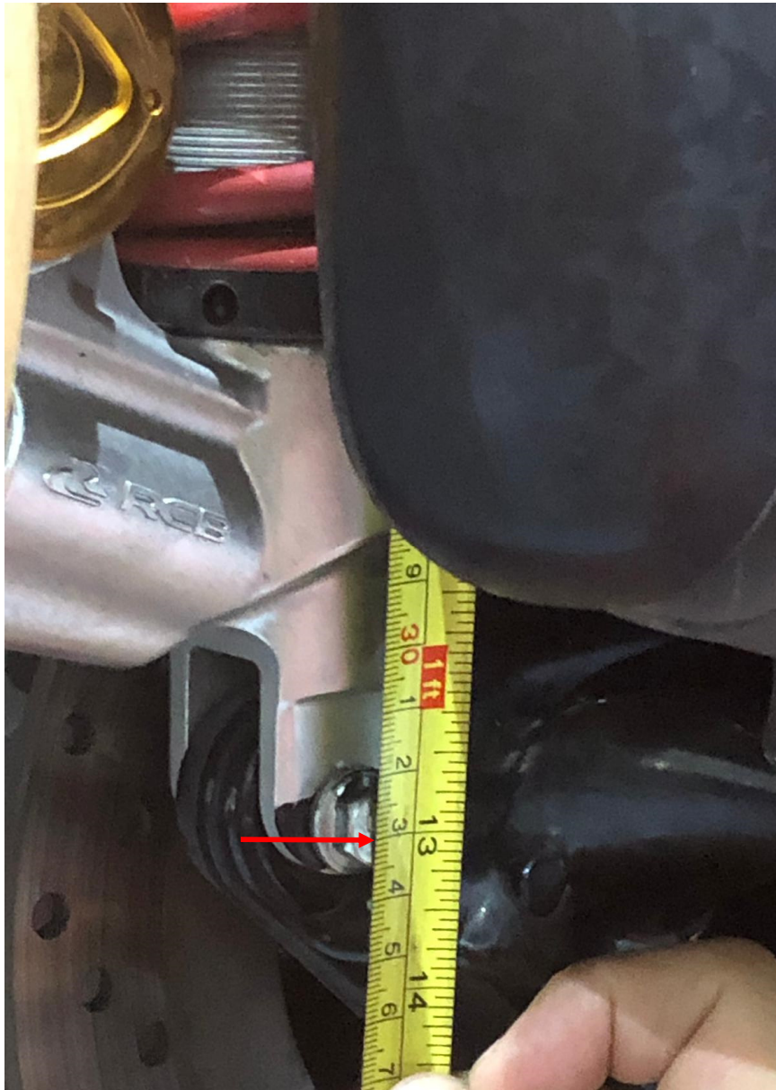
Photo 3 shows measurement of the rear right shock absorber of the Scooter. The height of the non-original rear shock absorbers was measured to be 33cm (arrowed). This was 2cm shorter as compared to the height of an original rear shock absorbers. Refer to photograph 5 below.
