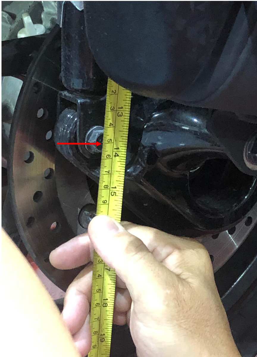
Photo 5 shows measurement of the rear right shock absorber of the similar make and model scooter as the Scooter. The height of an original rear shock absorbers was measured to be 35cm (arrowed). The non-original rear shock absorbers fitted on the Scooter was 2cm shorter as compared to the height of an original rear shock absorbers. Refer to photograph 3 above.
