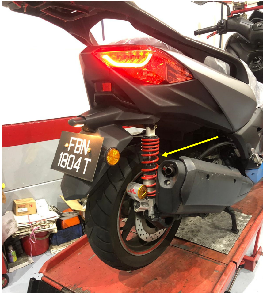
Photo 2 shows the rear right shock absorber (arrowed) of the Scooter (photograph taken by Hong Leong Corporation Holdings Pte Ltd during their checks of the Scooter). The rear shock absorbers fitted on the Scooter were non-original. Refer to photo 4 below for comparison.
