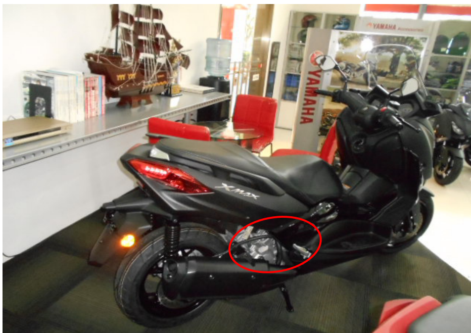
Photo 6 shows a similar make and model scooter as the Scooter. The engine area is highlighted by the red circle. From my observations, the engine of the Scooter was a horizontal incline engine. The mechanical components inside a horizontal incline engine are all horizontally aligned. When the centre stand is applied/engaged, I had observed that the engine front block is tilted slightly upwards.
