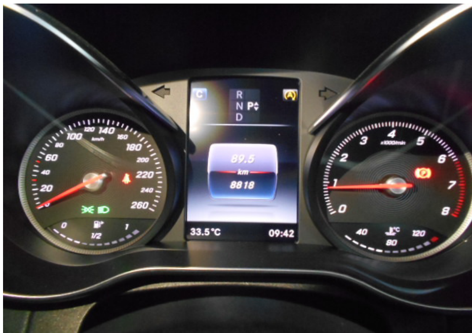
Photo 7 shows the respective warning lights no longer illuminated, indicating that there is no fault detected to the ABS, SRS, PSA, TPM and TCS of the Motor Car during the self-test. These electronic systems were hence in working condition at the time of my inspection.
