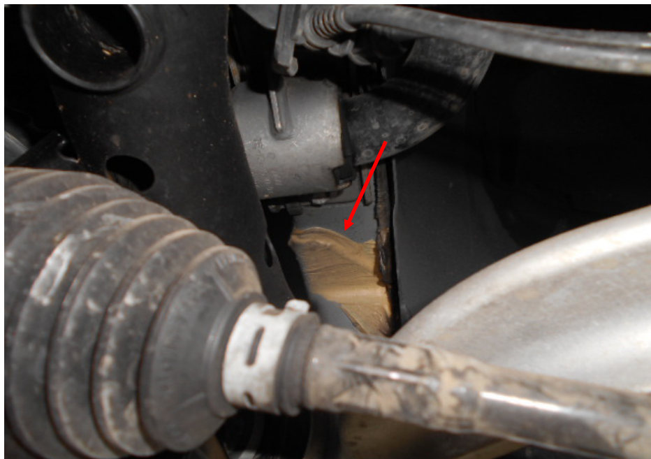
Photo 14 shows the structure/chassis body at the front right underside of the Motor Car. The original factory sealant (arrowed) at the joints along the structure/chassis body was untouched, indicating that the structure/chassis body of the Motor Car was originally fitted.
