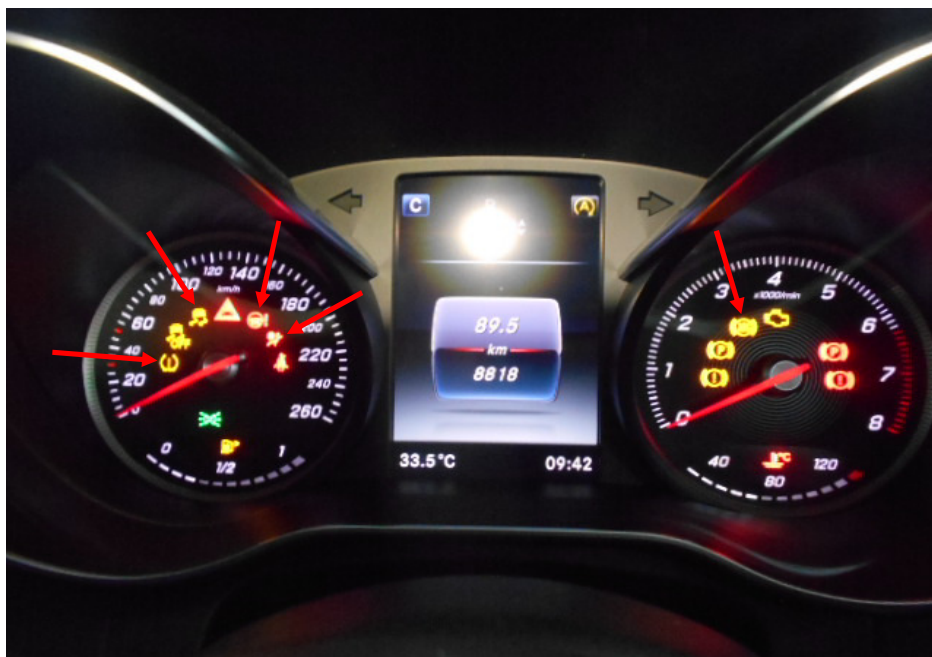
Photo 6 shows the warning lights for the various electronic safety features appearing on the instrument panel of the Motor Car during its self-test when the engine is cranked, in particular the ABS, SRS, PSA, TPM and TCS lights (arrowed).
