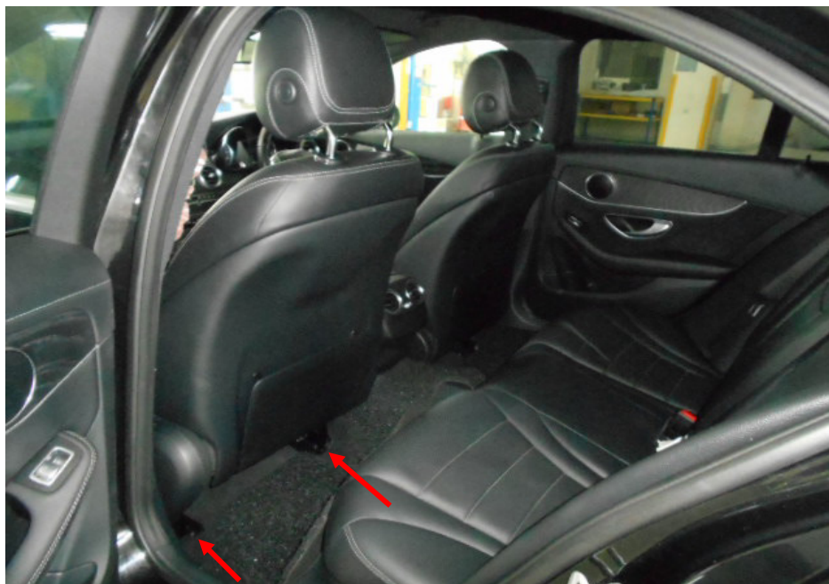
Photo 5 shows the rear seats of the Motor Car. All the seats were secured via seat rails (arrowed) to the floor board. The seats were also individually fitted with a retractable seat belt reel and pre-tensioner. The seat belts were tested and able to be fastened to the pretensioners that were fitted on the side of each individual seat.
