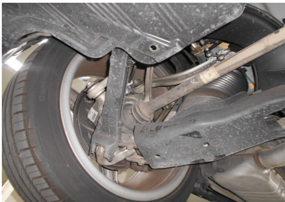
Photo 10 shows a general view of the control arms and linkages at the rear right wheel of the Motor Car. I did not observe any fluid leak and/or fluid stain on the underside of the Motor Car. All of the Motor Car's undercarriage components were observed to be intact and secured in an appropriate manner.
