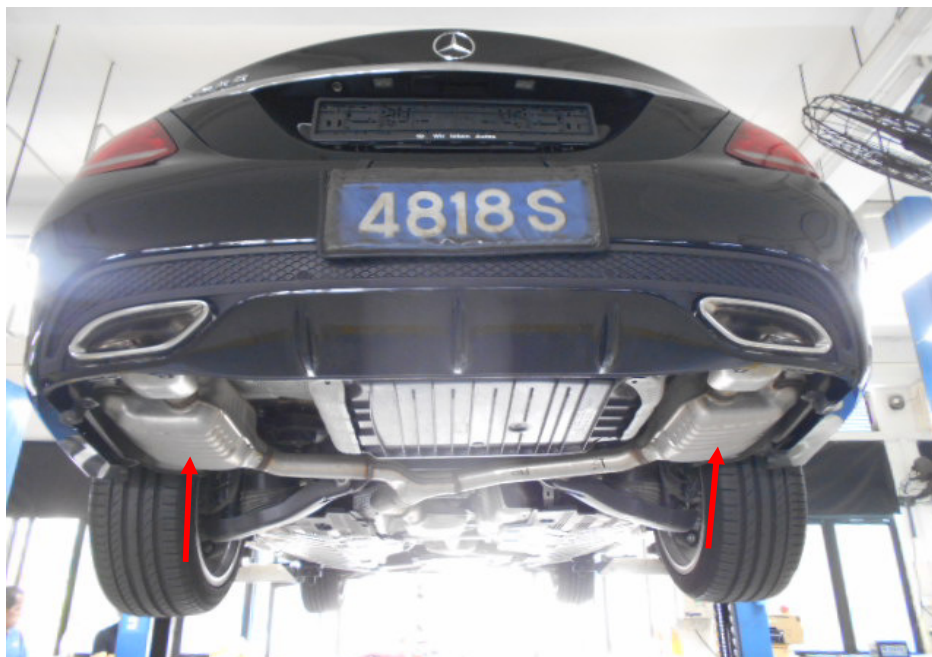
Photo 9 shows the Motor Car's rear exhaust mufflers (arrowed). My examination of the Motor Car's exhaust system revealed no sign(s) or indication(s) of any cut or weld marks along its exhaust pipes and on its rear mufflers.
