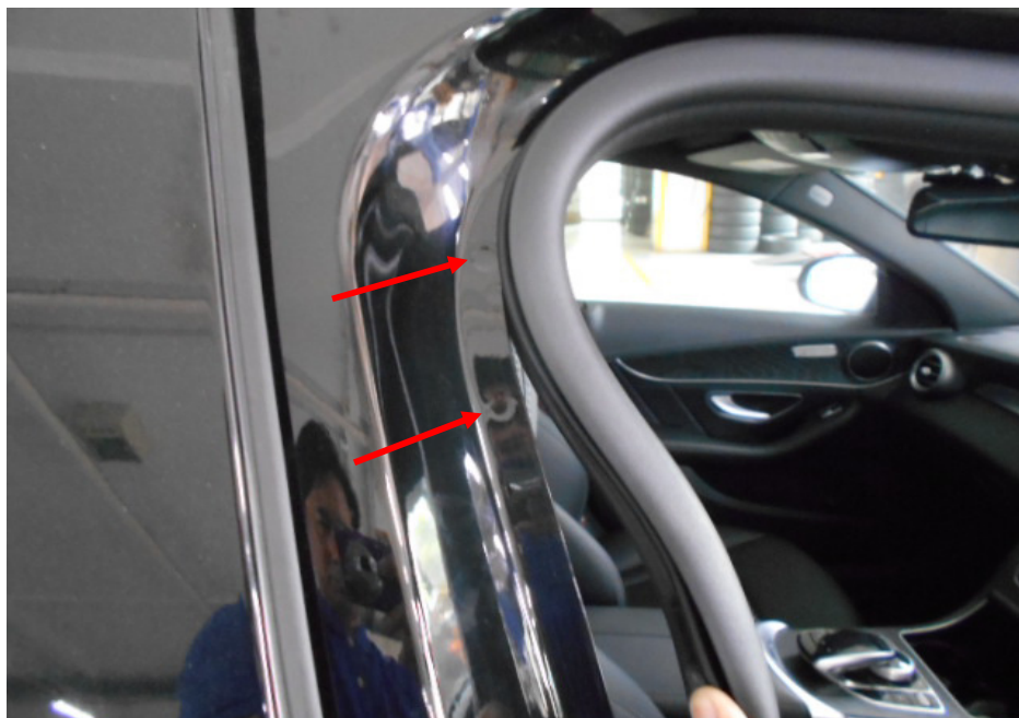
Photo 17 shows the right “B” pillar of the Motor Car. I did not find any weld marks other than original spot weld marks (arrowed) on the body panels of the Motor Car, indicating that there was no re-welding works carried out; and that the non-detachable body panels of the Motor Car were originally fitted.
