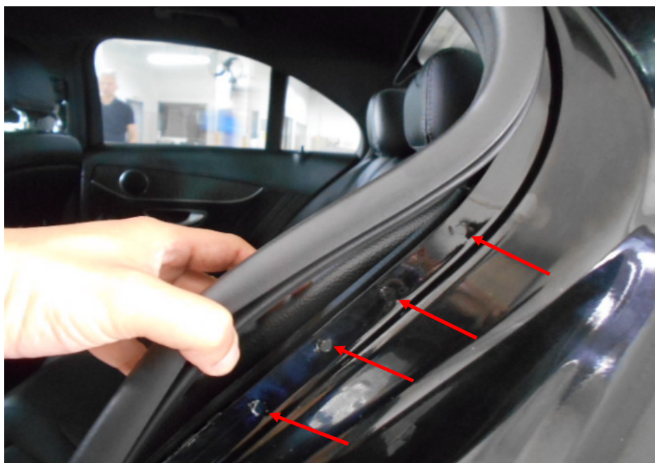
Photo 16 shows the rear left "C" pillar of the Motor Car. I did not find any weld marks other than original spot weld marks (arrowed) on the body panels of the Motor Car, indicating that there was no re-welding works carried out; and that the non-detachable body panels of the Motor Car were originally fitted.
