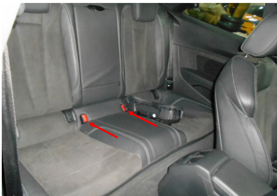
Photo 5 shows the rear seats of the Motor Car. All the seats of the Motor Car were found to be secured to the floor board of the Motor Car via seat rails bolted onto the floor board. The seats were also fitted with a retractable seat belt reel and pre-tensioner (arrowed). The seat belts were tested and were able to be fastened into the respective pretensions that were fitted on the side of each individual seat.
