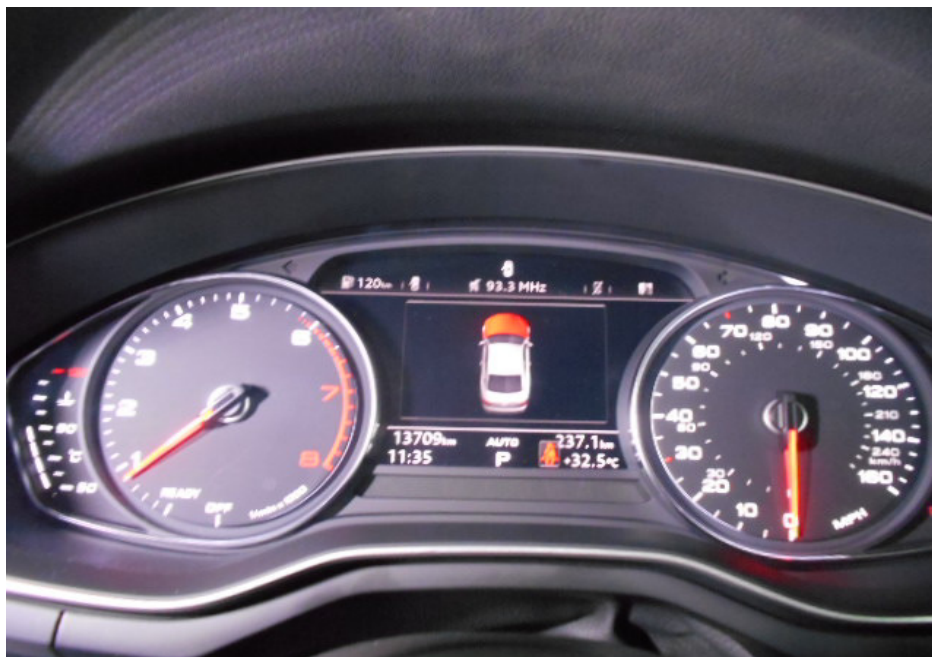
Photo 7 shows the respective warning lights no longer illuminated, indicating that there is no fault detected to the ABS, SRS, TPM, ESC and ESS systems of the Motor Car during the self-test. These electronic systems were hence in working condition at the time of my inspection.
