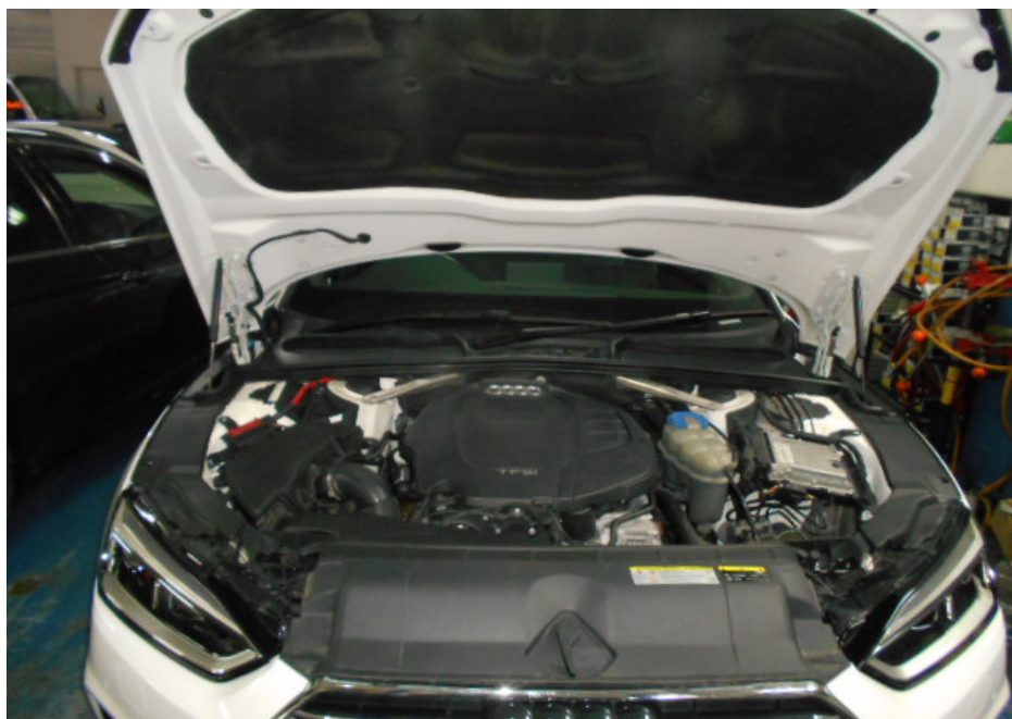
Photo 4 shows a general view of the engine compartment of the Motor Car at the time of my inspection. The various parts and components inside the engine compartment were all observed to be intact and properly fitted. There was also no sign(s) or indication(s) of fluid leak and/or fluid stain found inside the engine compartment. The brake fluid and engine coolant were all found to be of sufficient level for operating purposes. Visually, there was also no contamination found to these fluids.
