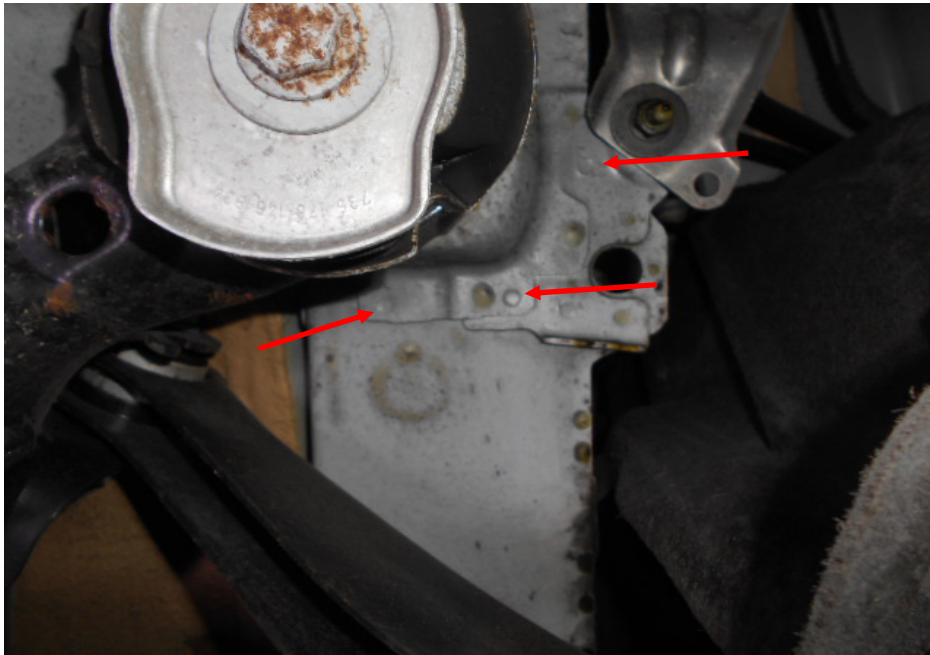
Photo 13 shows the structure/chassis body at the rear right underside of the Motor Car. Visually, I did not find any weld marks other than original spot weld marks (arrowed) along the structure/chassis. This would indicate that no work was done on the structure/chassis body of the Motor Car and that the structure/chassis body was originally fitted.
