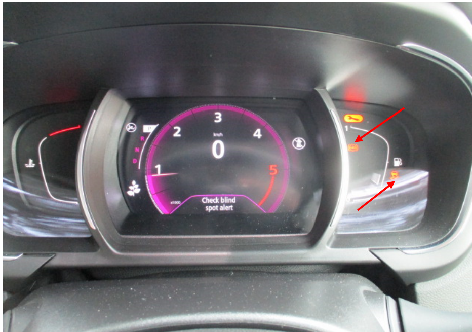
Photo 21 shows no warning lights illuminated on the instrument panel of the Motor Car after the engine was cranked. This would suggest that there was no abnormality to the various electronic operating systems of the Motor Car. The ABS light and ESC light had however remained illuminated after the self-test (arrowed) due to a fault in the system as a result of the accident.
