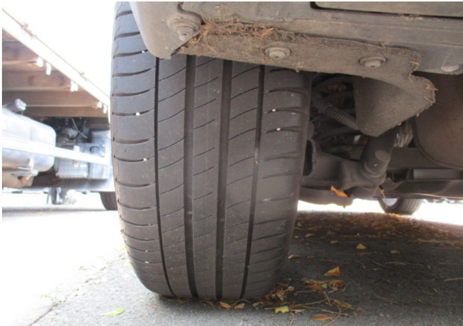
Photo 8 shows the condition of the rear left tyre of the Motor Car, which was observed to be in serviceable condition with remaining tread depth of approximately 5mm. The tyre, which was wrapped around alloy wheel rim, was also observed to be sufficiently inflated for vehicular operation.
