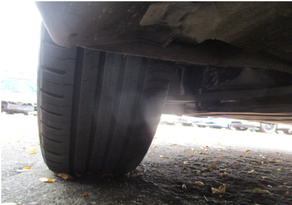
Photo 5 shows the condition of the front left tyre of the Motor Car, which was observed to be in serviceable condition with remaining tread depth of approximately 6mm. The tyre, which was wrapped around alloy wheel rim, was also observed to be sufficiently inflated for vehicular operation. There was no tear, cut or burst mark(s) on the outer and the inner sidewalls as well as across the tread of the 4 tyres.
