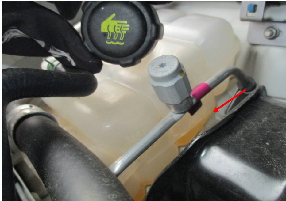
Photo 12 shows checks being carried out to the engine coolant of the Motor Car at the time of our inspection. The engine coolant was observed to be of sufficient level (arrowed) and without any visible contamination.
