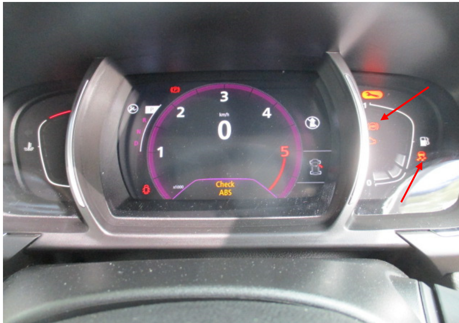
Photo 20 shows the warning lights for the various electronic operating systems of the Motor Car appearing on its instrument panel during the self-test when the engine is cranked, in particular the ESC light & ABS light (arrowed).
