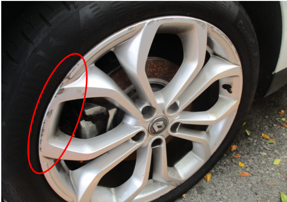
Photo 6 shows the left front wheel rim and tyre of the Motorcar at the time of our inspection. The front tyre was observed to be in serviceable condition and sufficiently inflated for vehicular operation. Some relatively minor marks of grazing nature were observed on the edges of the front wheel rim (circled), at the left side of the Motorcar.
