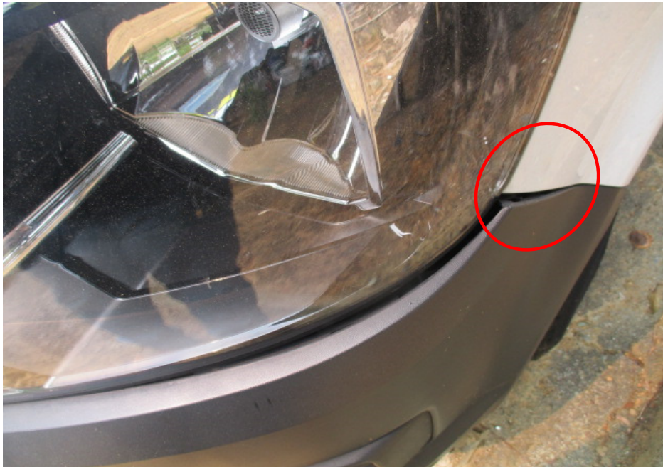
Photo 4 shows a close up view of the slightly dislodged front bumper (circled) of the Motor Van at the time of our inspection.
