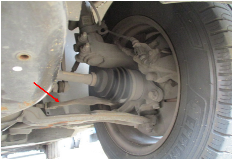
Photo 19 shows the various undercarriage components at the front left wheel of the Motor Van, in particular the steering tie rod (arrowed). The various undercarriage components of the Motor Van were all found to be intact without any visible damage. There was also no sign of fluid stain(s) observed on the various undercarriage components.
