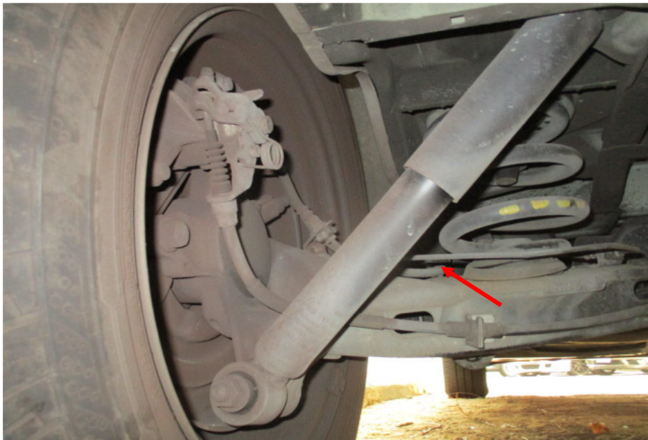
Photo 15 shows the brake pipe (arrowed) at the rear left wheel of the Motor Van. We did not observe any leakage of brake fluid at the time of our inspection of the Motor Van. Our static tests of the Motor Van's braking system had indicated that there was no internal leakage of pressure/vacuum. Hence the braking system was likely to be in serviceable condition at the material time of accident.
