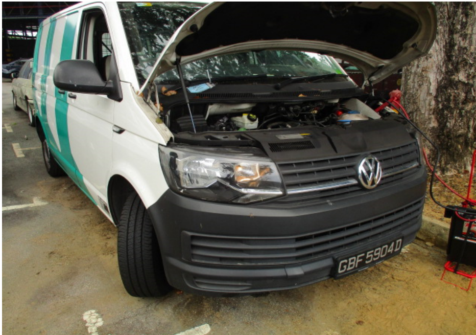
Photo 16 shows the front right wheel of the Motor Van turned to its full right. During our steering system test, we did not experience any abnormal free play and/or resistance when we had turned the steering wheel towards the left and right. This would suggest that the steering system of the Motor Van was likely to be in serviceable condition at the material time of accident.
