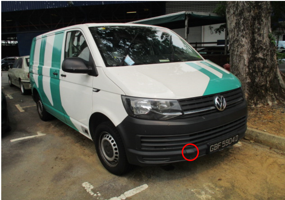
Photo 2 shows a general view of the front right body of the Motor Van at the time of our inspection. The Motor Van was observed to have sustained minimal impact damage that was confined to its frontal portion. Its front right tow hook cover (circled) as well as its front bumper was observed to be slightly dislodged as a result of the accident.
