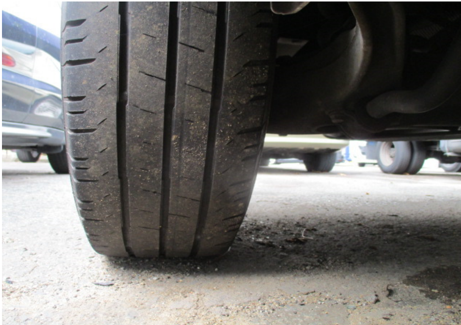
Photo 8 shows the condition of the rear right tyre of the Motor Van, which was observed to be in serviceable condition with remaining tread depth of approximately 4mm. There was also no tear, cut or burst mark(s) on the outer and the inner sidewalls as well as across the tread of the 4 tyres.
