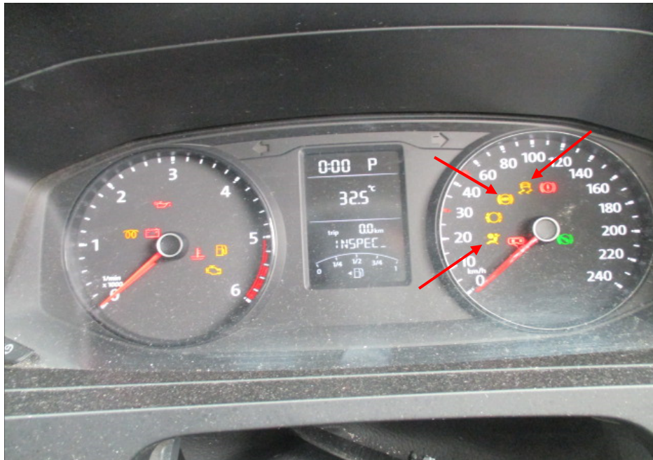
Photo 20 shows the warning lights for the various electronic operating systems of the Motor Van appearing on its instrument panel during the self-test when the engine is cranked, in particular the ESC, ABS and SRS light (arrowed).
