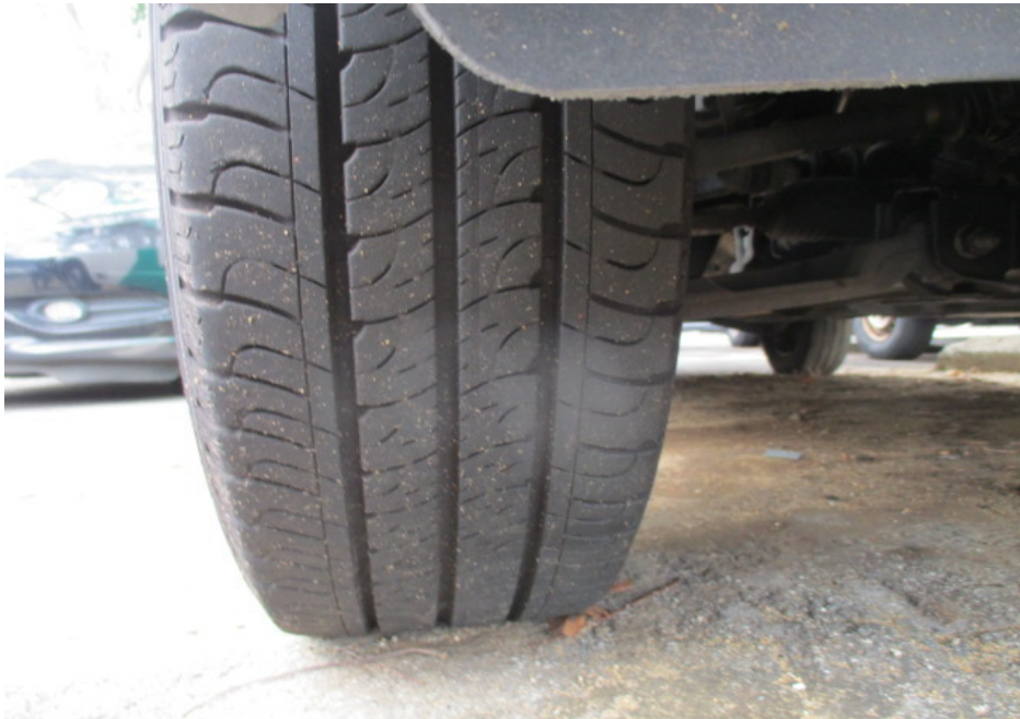
Photo 6 shows the condition of the front right tyre of the Motor Van, which was observed to be in serviceable condition with remaining tread depth of approximately 7mm. The tyre, which was wrapped around standard steel wheel rim, was also observed to be sufficiently inflated for vehicular operation.
