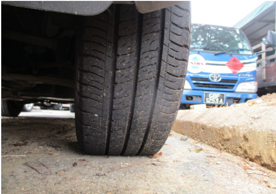
Photo 5 shows the condition of the front left tyre of the Motor Van, which was observed to be in serviceable condition with remaining tread depth of approximately 8mm. The tyre, which was wrapped around standard steel wheel rim, was also observed to be sufficiently inflated for vehicular operation. There was no tear, cut or burst mark(s) on the outer and the inner sidewalls as well as across the tread of the 4 tyres.
