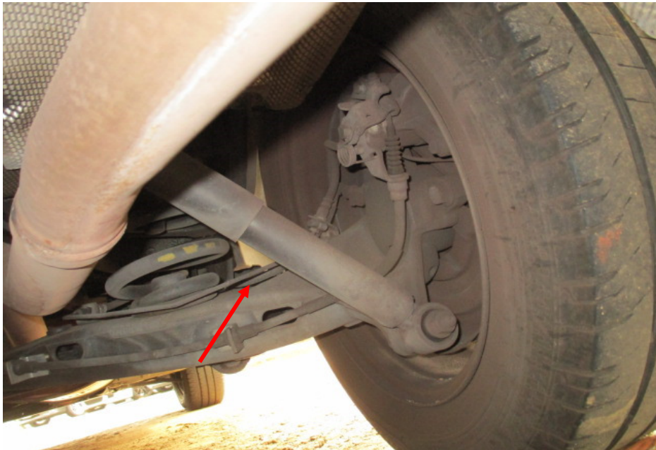
Photo 14 shows the brake pipe (arrowed) at the rear right wheel of the Motor Van. We did not observe any leakage of brake fluid at the time of our inspection of the Motor Van. Our static tests of the Motor Van's braking system had indicated that there was no internal leakage of pressure/vacuum. Hence the braking system was likely to be in serviceable condition at the material time of accident.
