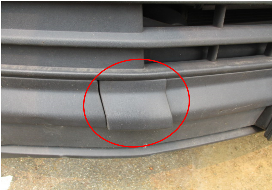
Photo 3 shows a close up view of the slightly dislodged front right tow hook cover (circled) of the Motor Van at the time of our inspection.
