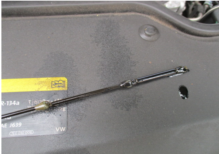
Photo 13 shows the engine dip stick of the Motor Van at the time of our inspection. The engine oil was observed to be of sufficient level and without any visible contamination.
