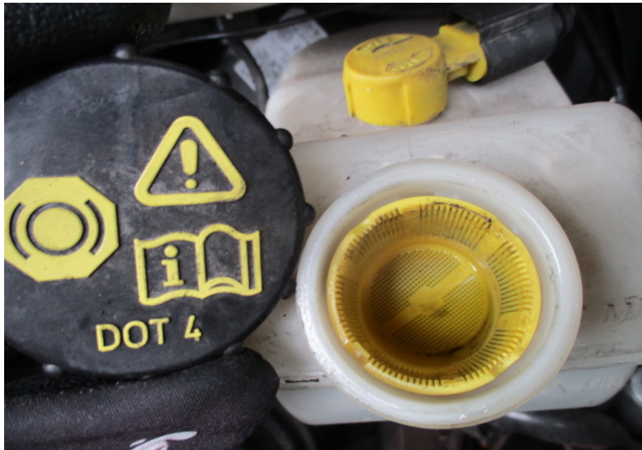
Photo 10 shows the brake fluid reservoir of the Motor Van at the time of our inspection. The brake fluid was observed to be of sufficient level and without any visible contamination.
