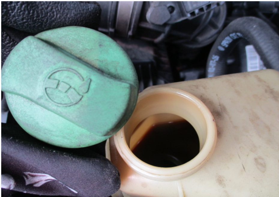
Photo 12 shows the power steering fluid reservoir of the Motor Van at the time of our inspection. The power steering fluid was observed to be of sufficient level and without any visible contamination.
