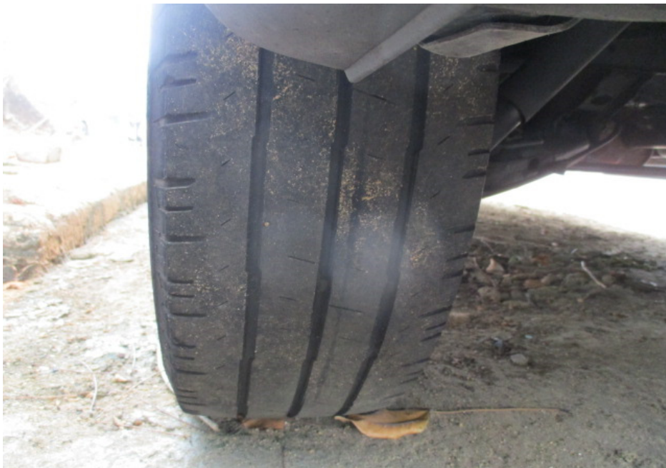
Photo 7 shows the condition of the rear left tyre of the Motor Van, which was observed to be in serviceable condition with remaining tread depth of approximately 4mm. The tyre, which was wrapped around standard steel wheel rim, was also observed to be sufficiently inflated for vehicular operation. There was also no damage found on the 4 wheel rims of the Motor Van.
