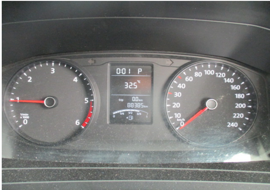
Photo 21 shows no warning lights illuminated on the instrument panel of the Motor Van after the engine was cranked. This would suggest that there was no abnormality to the various electronic operating systems of the Motor Van, like the ESC, ABS and SRS.
