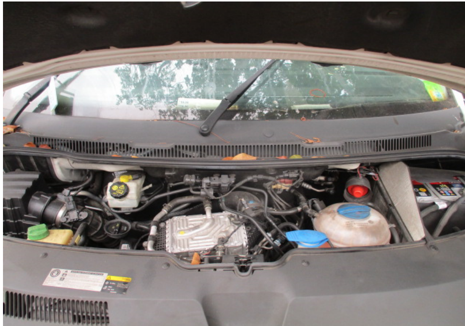
Photo 9 shows a general view of the Motor Van's engine compartment. The various parts and components inside the engine compartment were unaffected by the accident. There was also no sign(s) or indication(s) of fluid leakage and/or fluid stain within the engine compartment. The wirings and cables were all observed to be intact and adequately secured to their respective connectors and/or connecting ports.
