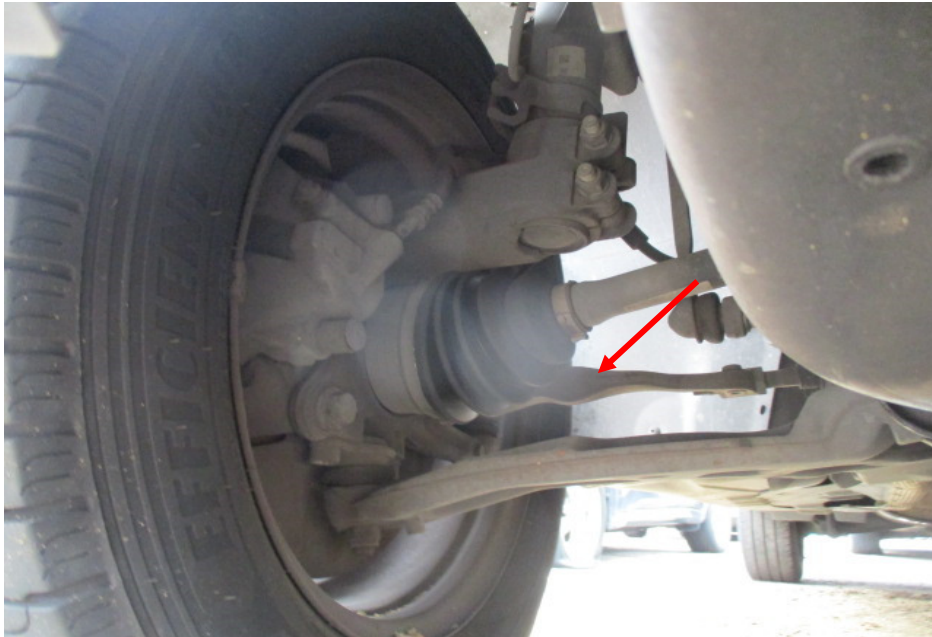
Photo 18 shows the various undercarriage components at the front right wheel of the Motor Van, in particular the steering tie rod (arrowed). The various steering components were all found to be intact, suggesting that the steering system of the Motor Van was likely to be in serviceable condition at the material time of accident. There was also no sign of fluid stain(s) observed on the various undercarriage components.
