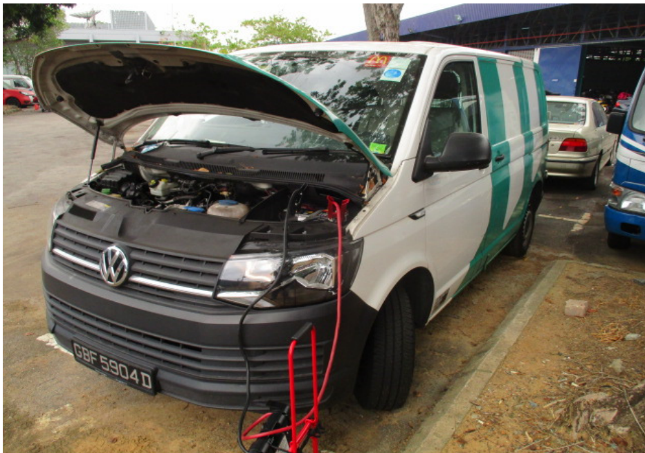
Photo 17 shows the front left wheel of the Motor Van turned to its full left. During our steering system test, we did not experience any abnormal free play and/or resistance when we had turned the steering wheel towards the left and right. This would suggest that the steering system of the Motor Van was likely to be in serviceable condition at the material time of accident.
