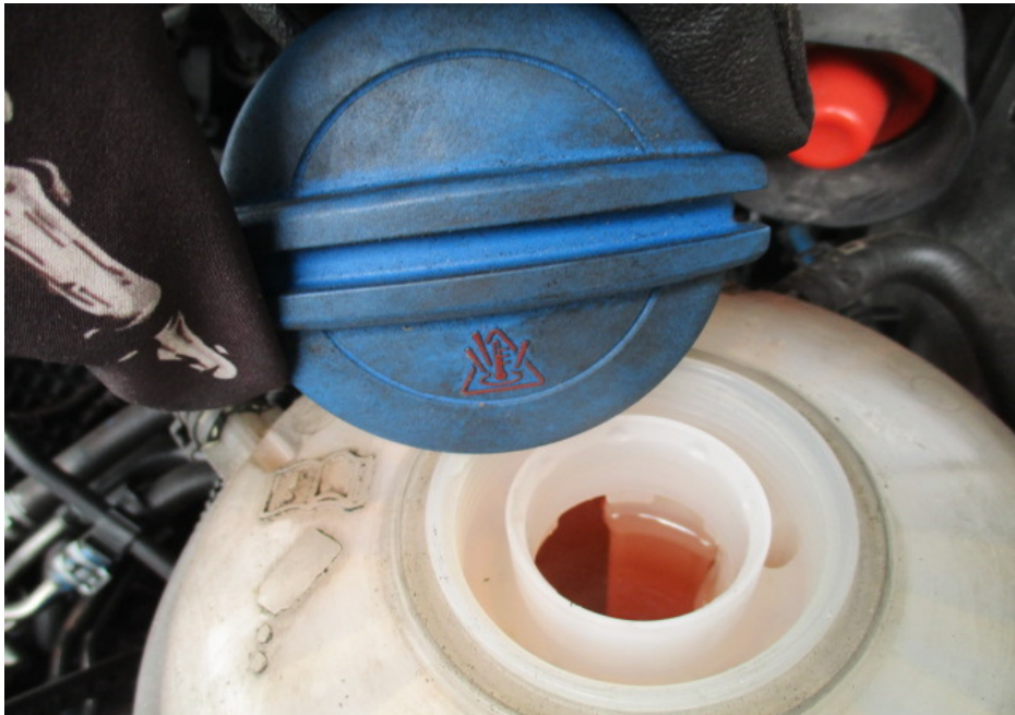
Photo 11 shows the engine coolant reservoir of the Motor Van at the time of our inspection. The engine coolant was observed to be of sufficient level and without any visible contamination.
