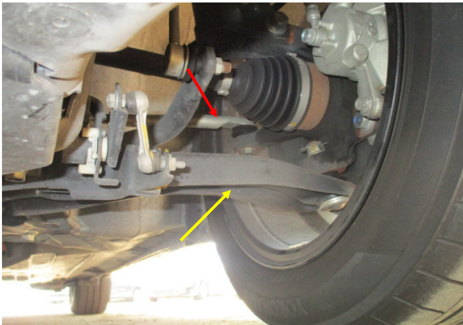
Photo 17 shows the various undercarriage components at the front left wheel of the Motor Car, which had included the steering tie rod (red arrow) and left drive shaft (yellow arrow). The various undercarriage components of the Motor Car were all found to be intact without any visible damage.
