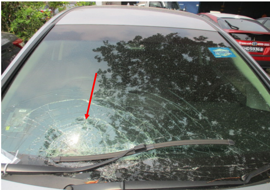
Photo 5 shows a closer view of the shattered front windscreen (arrowed) of the Motor Car at the time of our inspection.
