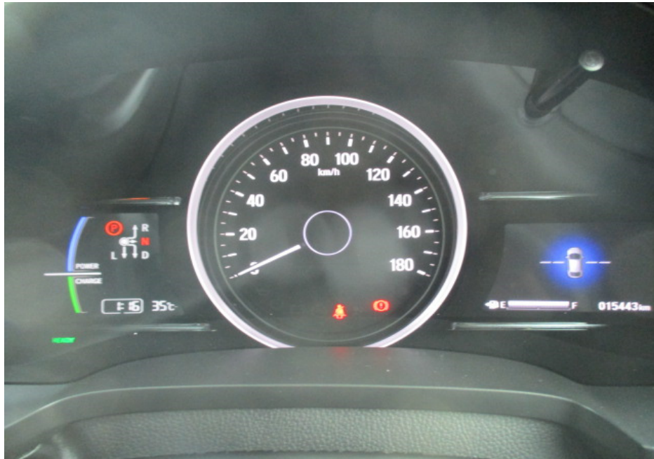
Photo 21 shows no warning lights illuminated on the instrument panel of the Motor Car after the engine was cranked. This would suggest that there was no abnormality to the various electronic operating systems of the Motor Car, like the EPS, ABS, ESC and SRS etc.
