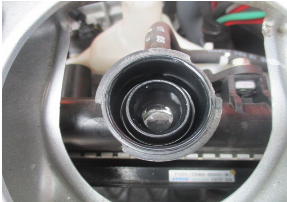
Photo 12 shows checks being carried out to the engine coolant of the Motor Car at the time of our inspection. The engine coolant was observed to be of sufficient level and without any visible contamination.
