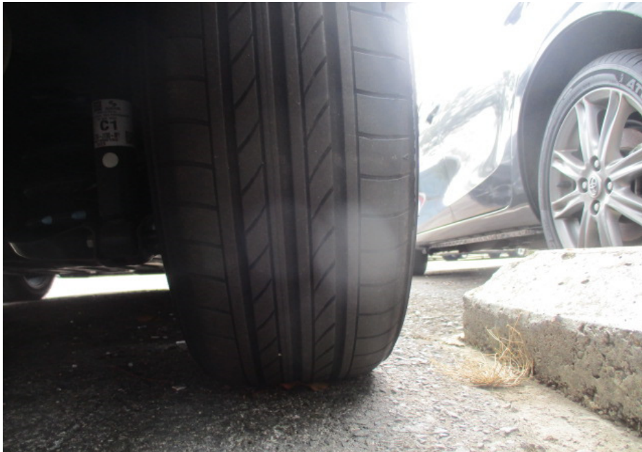
Photo 9 shows the condition of the rear right tyre of the Motor Car, which was observed to be in serviceable condition with remaining tread depth of approximately 5mm. There was also no tear, cut or burst mark(s) on the outer and the inner sidewalls as well as across the tread of the 4 tyres.
