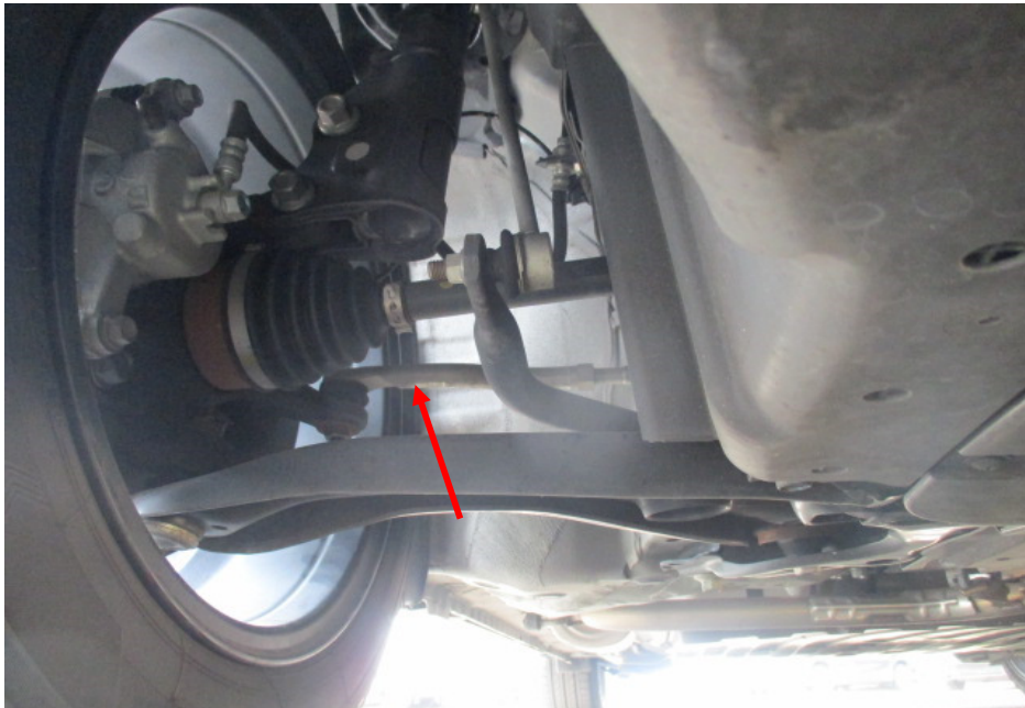
Photo 16 shows the various undercarriage components at the front right wheel of the Motor Car, in particular the steering tie rod (arrowed). The various steering components were all found to be intact, suggesting that the steering system of the Motor Car was likely to be in serviceable condition at the material time of accident. There was also no sign of fluid stain observed on the various undercarriage components at the front right wheel of the Motor Car.
