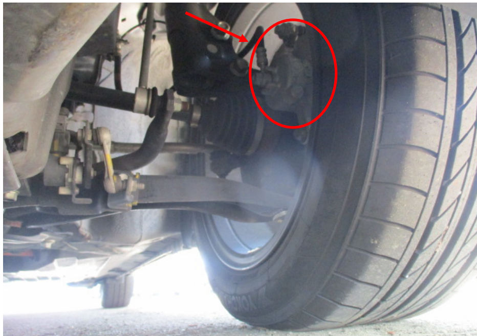
Photo 15 shows the brake hose/pipe (arrowed) at the front left wheel of the Motor Car. No leakage of brake fluid was observed. Visual examination of the various components of the braking system like the brake caliper (circled), brake pedal etc. had revealed all to be intact and without visible damage.
