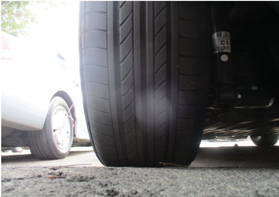
Photo 8 shows the condition of the rear left tyre of the Motor Car, which was observed to be in serviceable condition with remaining tread depth of approximately 5mm. The tyre, which was wrapped around alloy wheel rim, was also observed to be sufficiently inflated for vehicular operation. There was also no damage found on the 4 wheel rims of the Motor Car.
