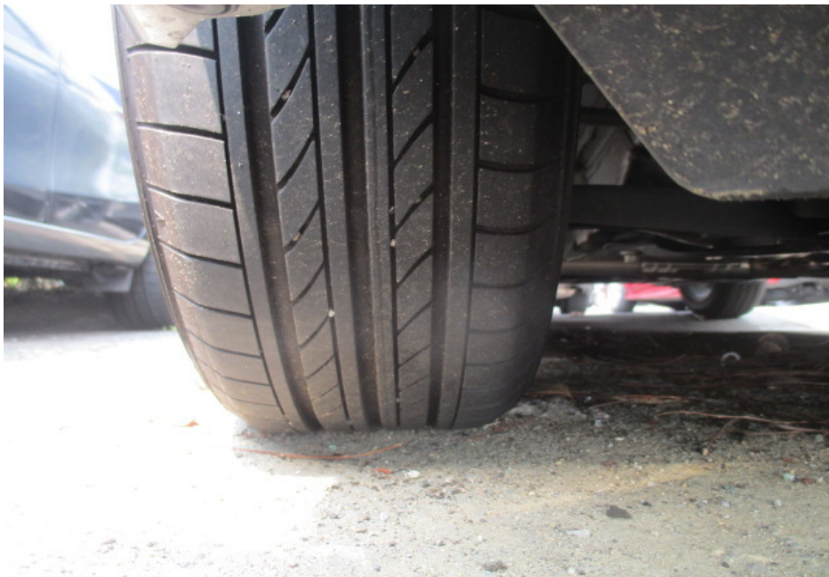
Photo 7 shows the condition of the front right tyre of the Motor Car, which was observed to be in serviceable condition with remaining tread depth of approximately 6mm. The tyre, which was wrapped around alloy wheel rim, was also observed to be sufficiently inflated for vehicular operation.
