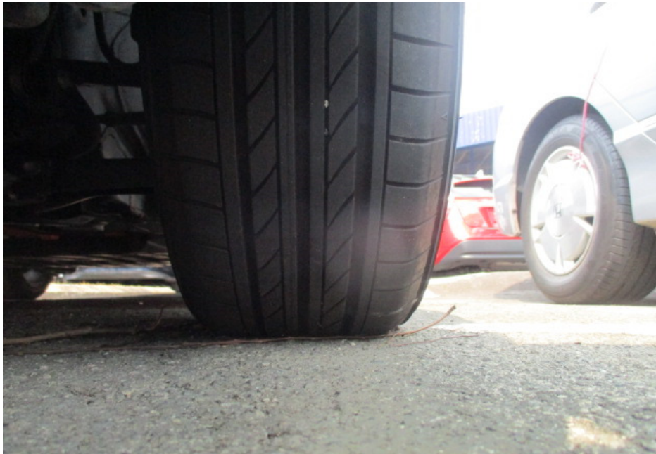
Photo 6 shows the condition of the front left tyre of the Motor Car, which was observed to be in serviceable condition with remaining tread depth of approximately 6mm. The tyre, which was wrapped around alloy wheel rim, was also observed to be sufficiently inflated for vehicular operation. There was no tear, cut or burst mark(s) on the outer and the inner sidewalls as well as across the tread of the 4 tyres.
