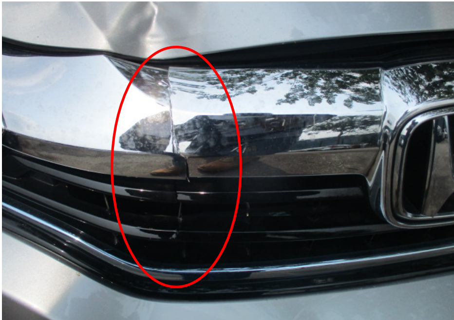
Photo 4 shows a closer view of the cracked radiator grille of the Motor Car at the time of our inspection (circled).
