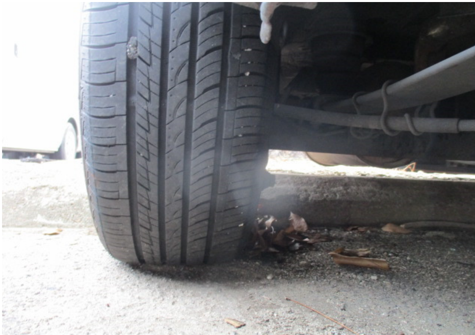
Photo 9 shows the condition of the rear right tyre of the Motor Van, which was observed to be in serviceable condition with remaining tread depth of approximately 6mm. There was also no tear, cut or burst mark(s) on the outer and the inner sidewalls as well as across the tread of the 4 tyres.
