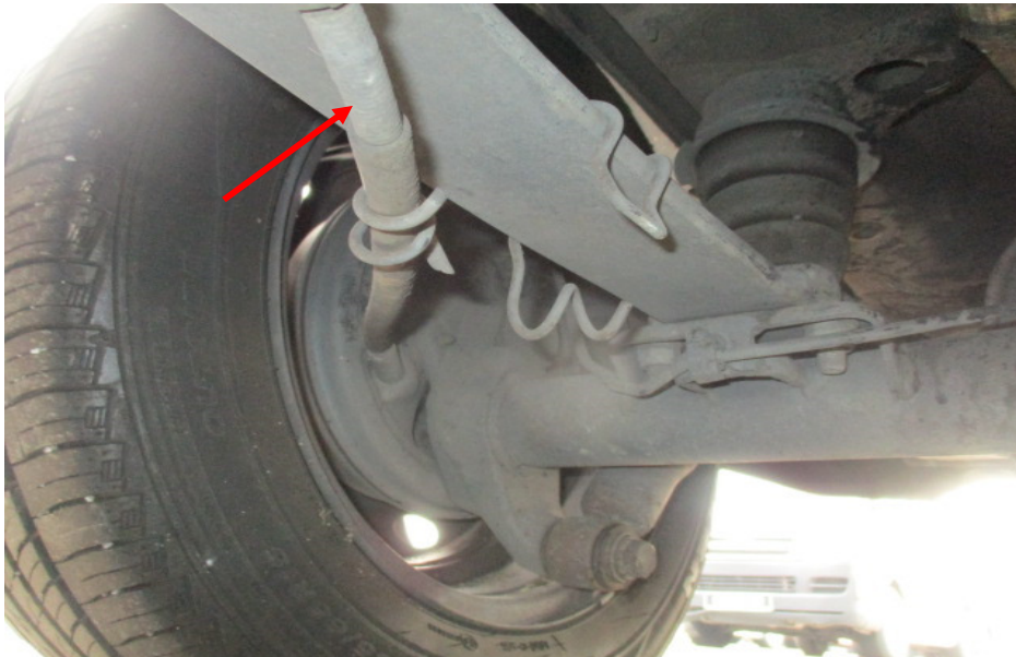
Photo 15 shows the brake pipe (arrowed) at the rear right wheel of the Motor Van. We did not observe any leakage of brake fluid at the time of our inspection of the Motor Van. Our static tests of the Motor Van's braking system had indicated that there was no internal leakage of pressure/vacuum. Hence the braking system was likely to be in serviceable condition at the material time of accident.
