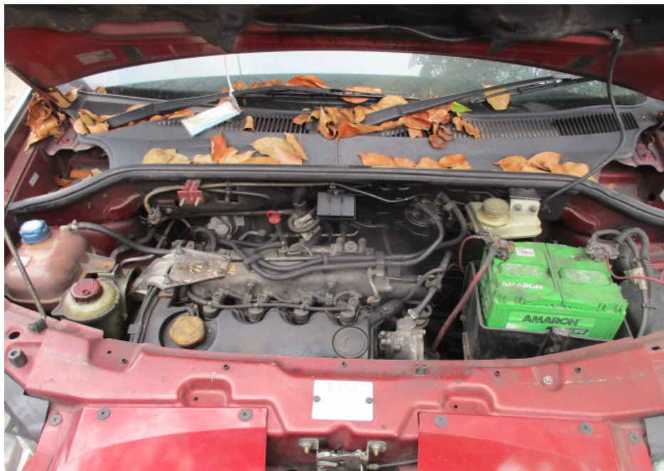
Photo 10 shows a general view of the Motor Van's engine compartment. The various parts and components inside the engine compartment were unaffected by the accident. There was also no sign(s) or indication(s) of fluid leakage and/or fluid stain within the engine compartment. The wirings and cables were all observed to be intact and adequately secured to their respective connectors and/or connecting ports.
