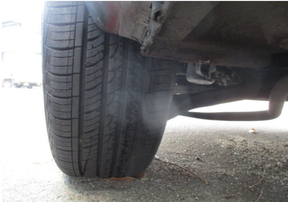
Photo 6 shows the condition of the front left tyre of the Motor Van, which was observed to be in serviceable condition with remaining tread depth of approximately 7mm. The tyre, which was wrapped around standard steel wheel rim, was also observed to be sufficiently inflated for vehicular operation. There was no tear, cut or burst mark(s) on the outer and the inner sidewalls as well as across the tread of the 4 tyres.
