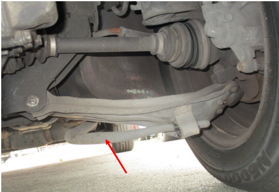
Photo 19 shows the various undercarriage components at the front left wheel of the Motor Van, in particular the steering tie rod (arrowed). The various undercarriage components of the Motor Van were all found to be intact without any visible damage. There was also no sign of fluid stain(s) observed on the various undercarriage components.
