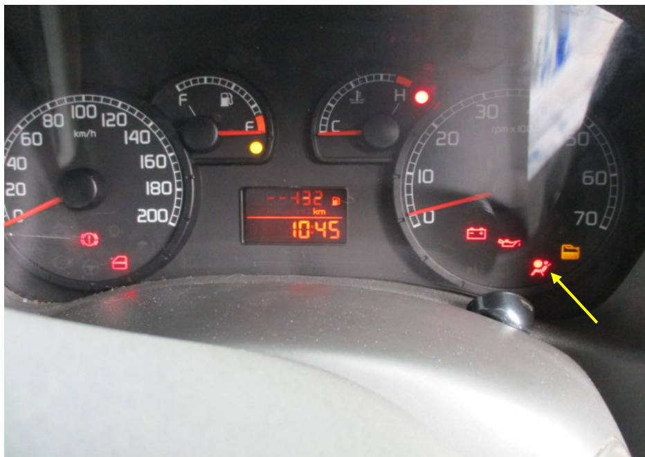
Photo 20 shows the warning lights for the various electronic operating systems of the Motor Van appearing on its instrument panel during the self-test when the engine is cranked, in particular the SRS light (arrowed).
