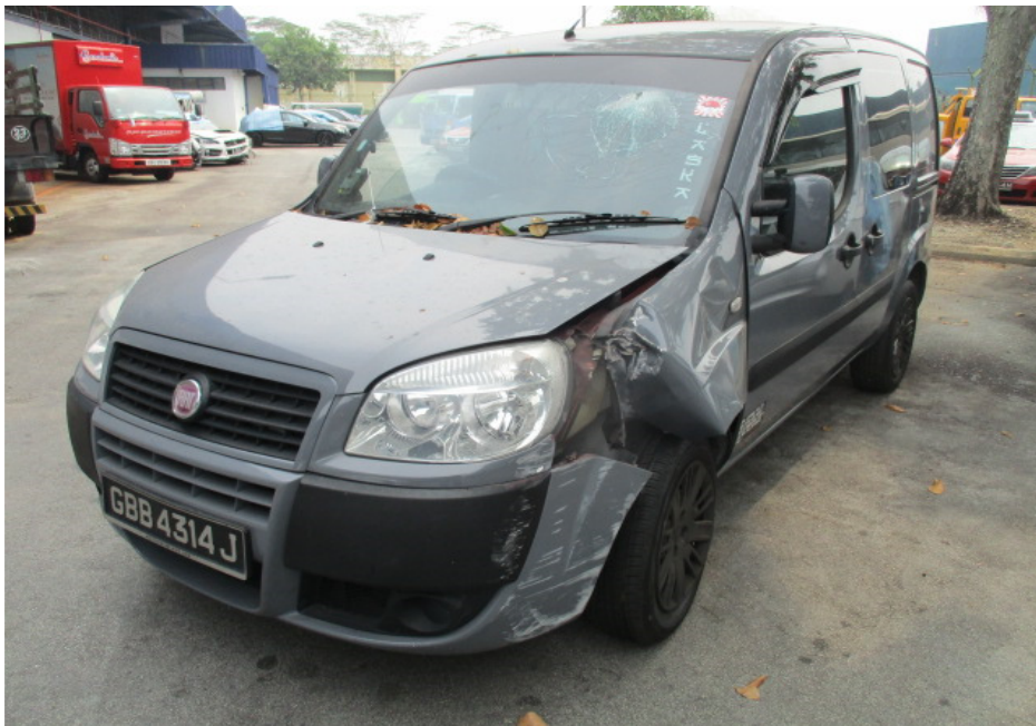
Photo 17 shows the front left wheel of the Motor Van turned slightly to the left. We were unable to turn the steering wheel left to full lock position due to the dented left front fender.
