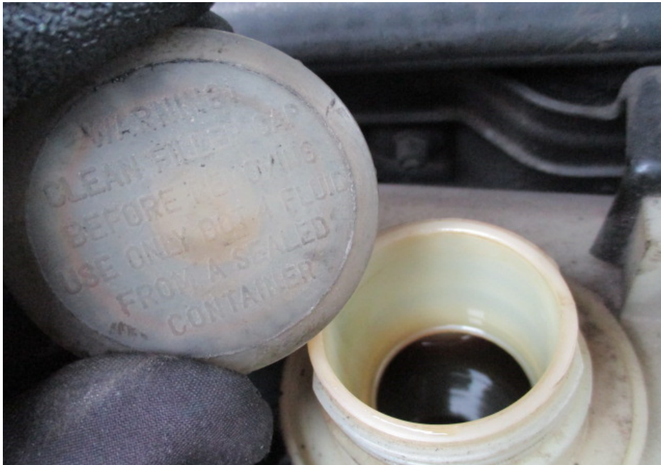
Photo 11 shows the brake fluid reservoir of the Motor Van at the time of our inspection. The brake fluid was observed to be of sufficient level and without any visible contamination.
