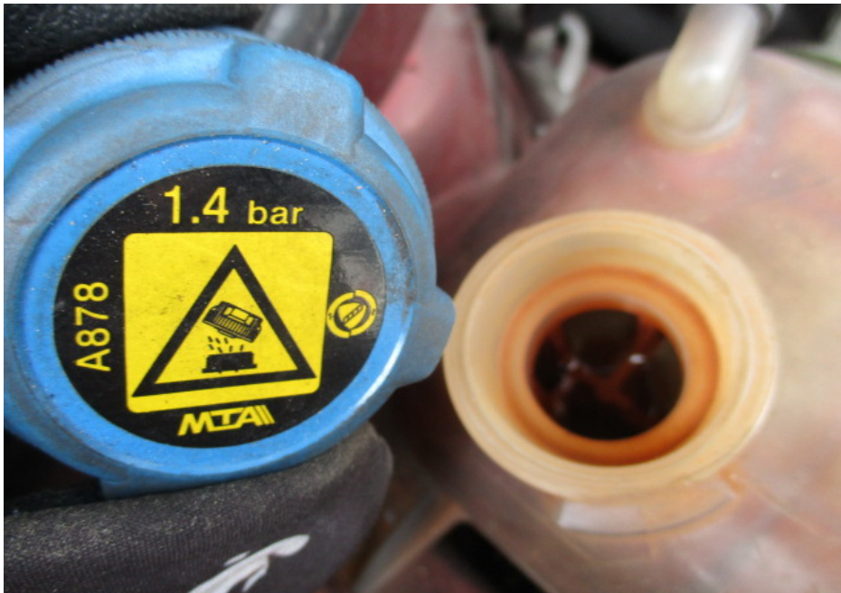
Photo 12 shows the engine coolant reservoir of the Motor Van at the time of our inspection. The engine coolant was observed to be of sufficient level and without any visible contamination.
