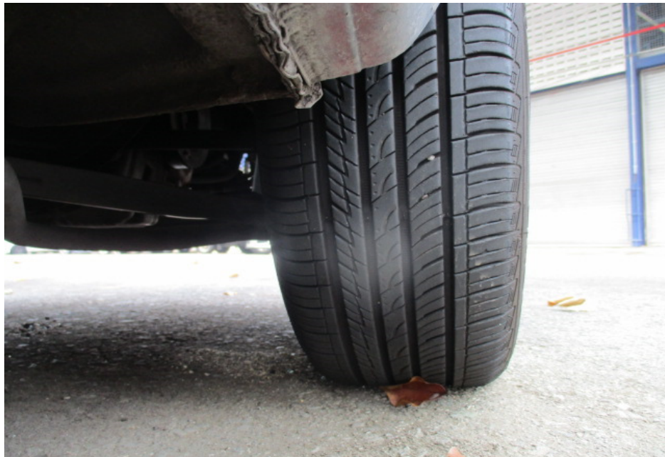
Photo 7 shows the condition of the front right tyre of the Motor Van, which was observed to be in serviceable condition with remaining tread depth of approximately 6mm. The tyre, which was wrapped around standard steel wheel rim, was also observed to be sufficiently inflated for vehicular operation.
