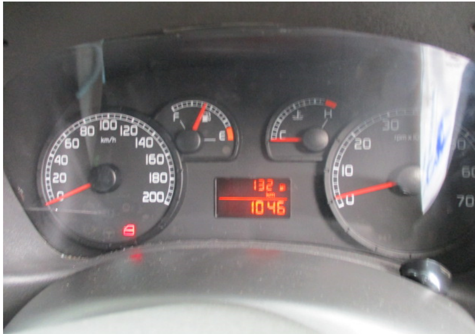
Photo 21 shows no warning lights illuminated on the instrument panel of the Motor Van after the engine was cranked. This would suggest that there was no abnormality to the various electronic operating systems of the Motor Van, like the SRS.
