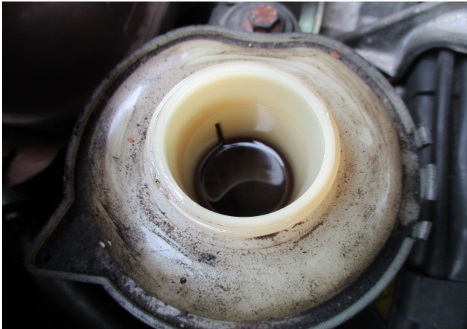
Photo 13 shows the power steering fluid reservoir of the Motor Van at the time of our inspection. The power steering fluid was observed to be of sufficient level and without any visible contamination.
