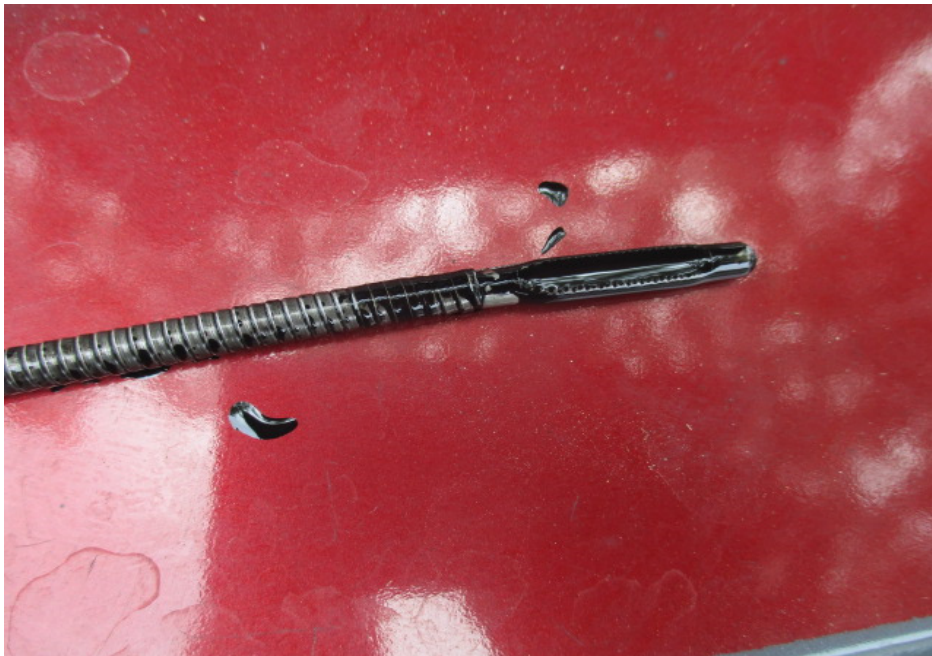
Photo 14 shows the engine dip stick of the Motor Van at the time of our inspection. The engine oil was observed to be of sufficient level and without any visible contamination.
