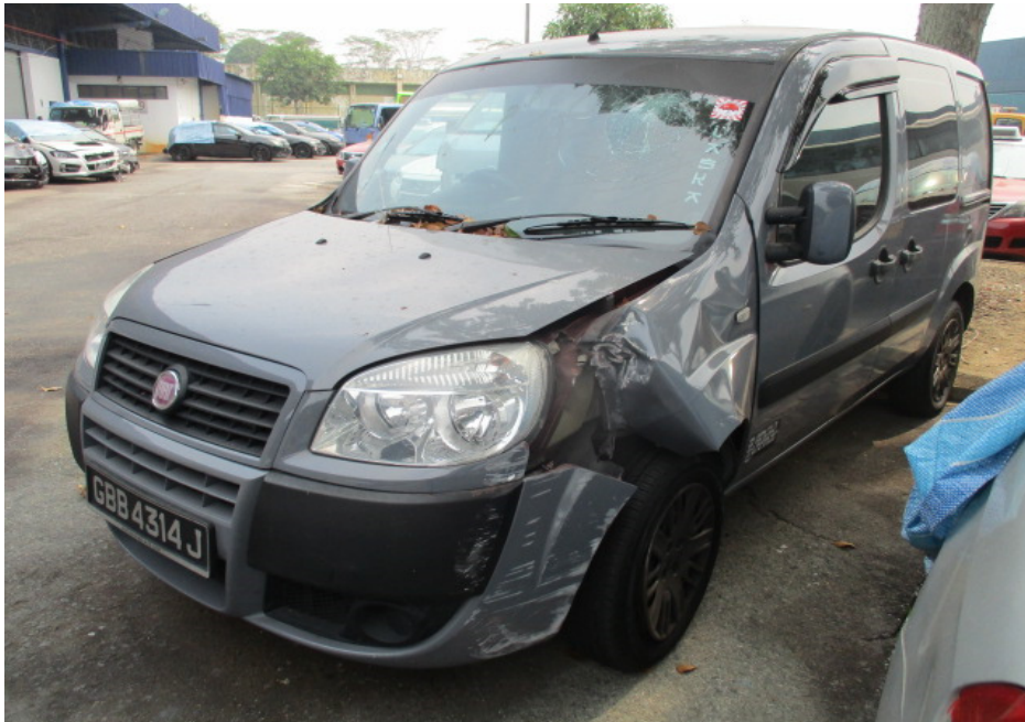
Photo 2 shows a general view of the front left body of the Motor Van at the time of our inspection. The Motor Van was observed to have sustained minimal impact damage that was confined to its left front portion. Its left front fender was observed to have been dented; its front bumper was observed to have been dislodged; its front windscreen was observed to be shattered.
