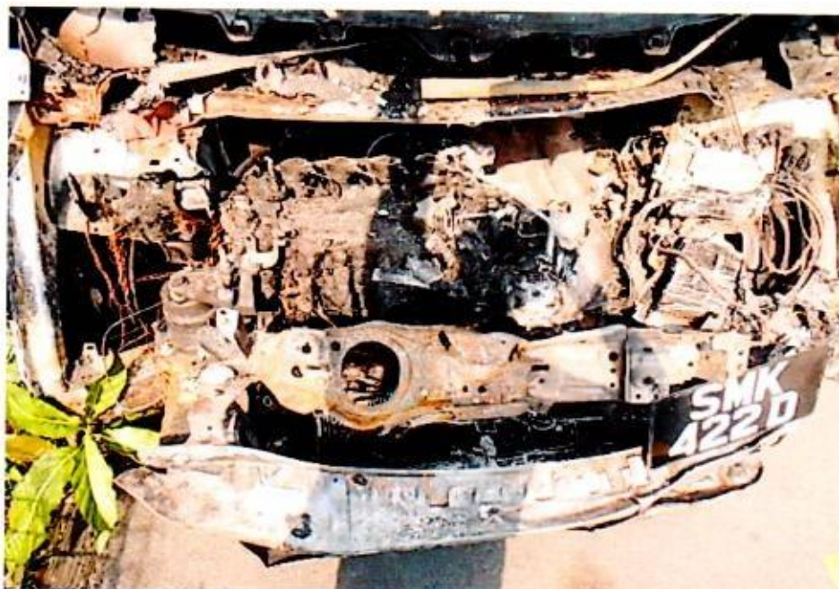
Photo 2 shows the engine compartment of the Insured Vehicle at the time of inspection. The entire engine compartment of the Insured Vehicle was observed to be severely burnt. Almost all the parts inside the engine compartment were burnt to char.
