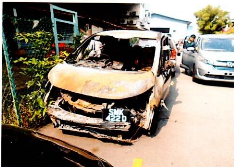
Photo 1 shows a general view of the front left body of the Insured Vehicle at the time of inspection. The Insured Vehicle was noted to have sustained severe fire damage at its frontal portion. Its front bumper, front bonnet, front grille, front headlamps, front windscreen and front fenders were amongst the body parts that were found to have been affected as a result of the fire.
