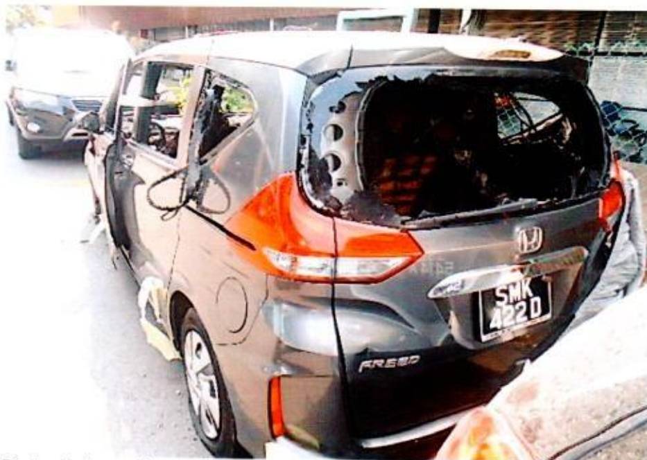
Photo 4 shows the rear left body of the Insured Vehicle. Exterially, the body panels at the rear of the Insured Vehicle were unaffected, apart from a shattered rear windscreen.
