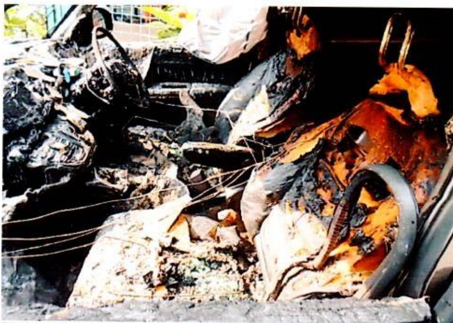
Photo 3 shows the interior compartment of the Insured Vehicle, which had also sustained severe damage of fire nature. The front dashboard, roof upholstery, carpet and seats amongst others, inside the interior compartment were burnt and/or melted.
