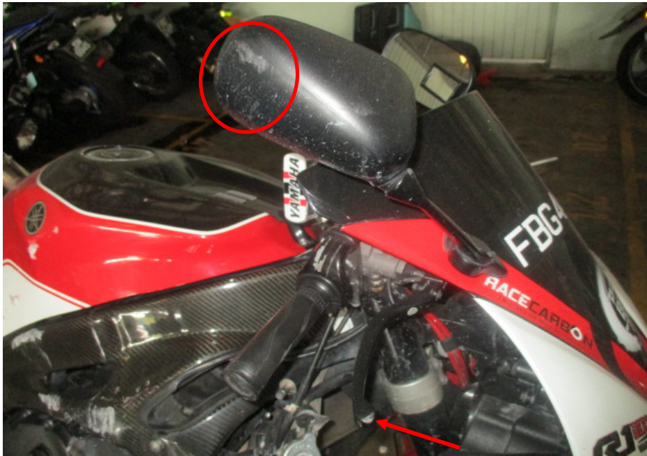
Photo 7 shows a closer view of the front brake lever (arrowed) and right side mirror (circled) which were amongst the body parts at the front body of the Motorcycle that had sustained damage as a result of the accident.
