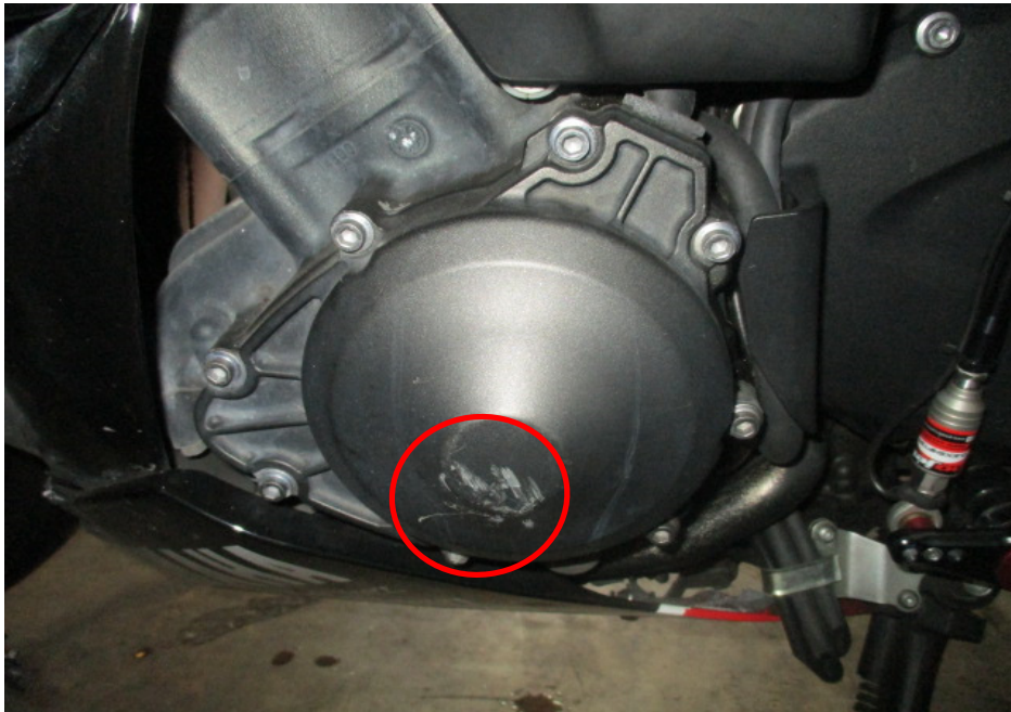
Photo 20 shows the left side of the engine of the Motorcycle at the time of our inspection. The various left engine components had sustained damage of grazing nature as a result of the accident (circled) however the engine components were still intact. There was also no fluid leak and/or fluid stain found around the left engine area of the Motorcycle.
