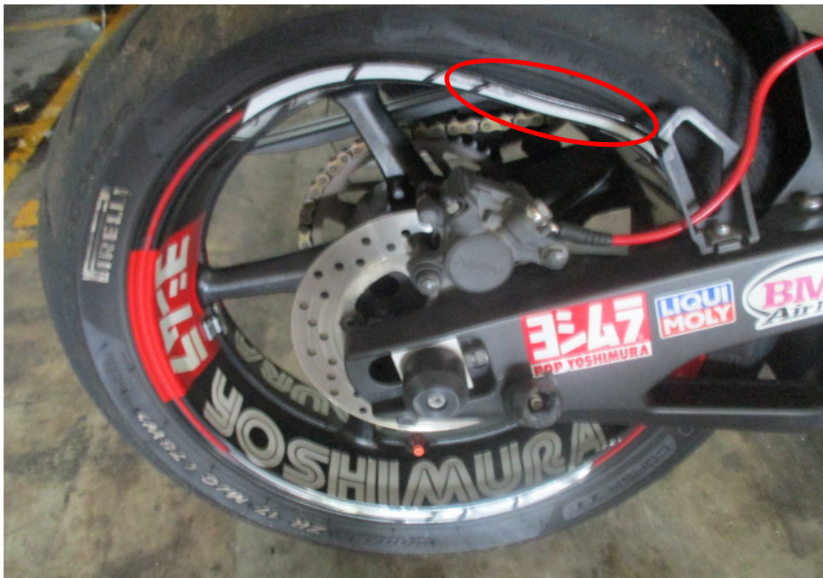
Photo 18 shows the bent rear wheel rim of the Motorcycle at the time of our inspection (circled).
