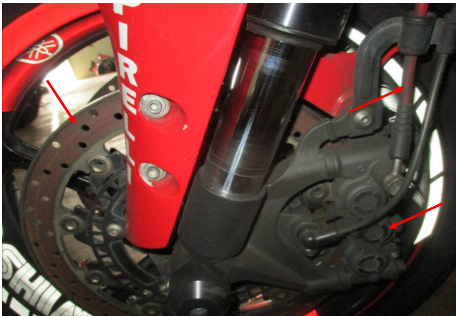
Photo 30 shows a close up view of the front brake caliper, front brake disc and front brake hose (arrowed) at the left side of the Motorcycle's front wheel, which are all part of the components in the hydraulic front brake system of the Motorcycle. Our visual checks of these various components had revealed all to be intact with no visible damage. No leakage of brake fluid was also observed.
