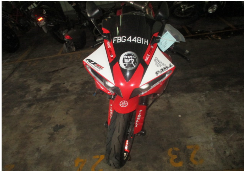
Photo 27 shows the front wheel of the Motorcycle turned slightly towards the right. We were unable to fully turn the handle bar towards the right due to the resistance from the broken components of the head cowl which were found to be pushed inwards as a result of the accident.
