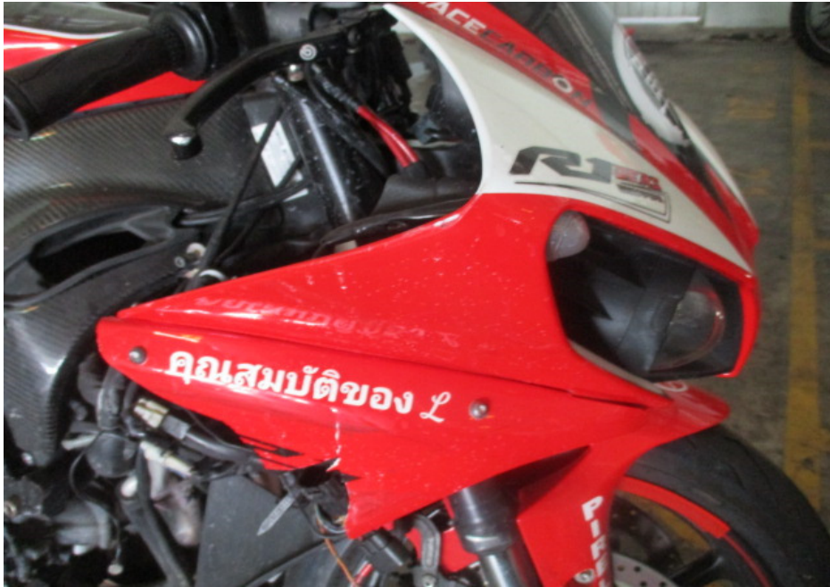
Photo 5 shows a closer view of the head cowl which was amongst the body parts at the front body of the Motorcycle that had sustained damage as a result of the accident.
