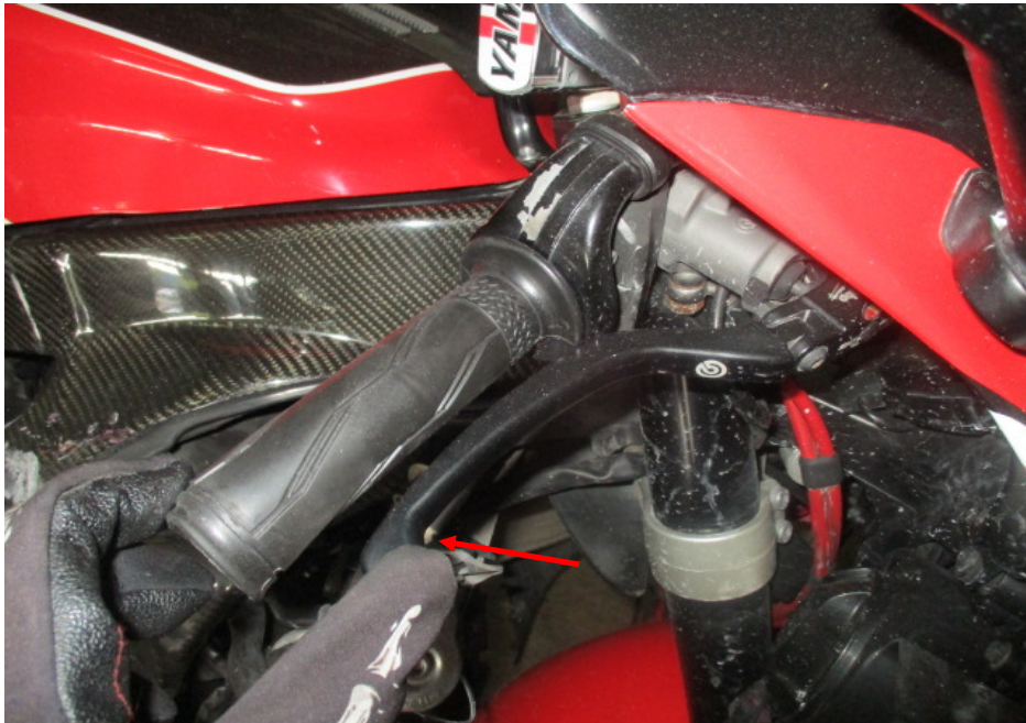
Photo 31 shows the front brake lever being depressed. There was no resistance felt (spongy like feel) upon pressing the front brake lever (arrowed). This would indicate that there is a leakage of pressure/vacuum in the brake system.
