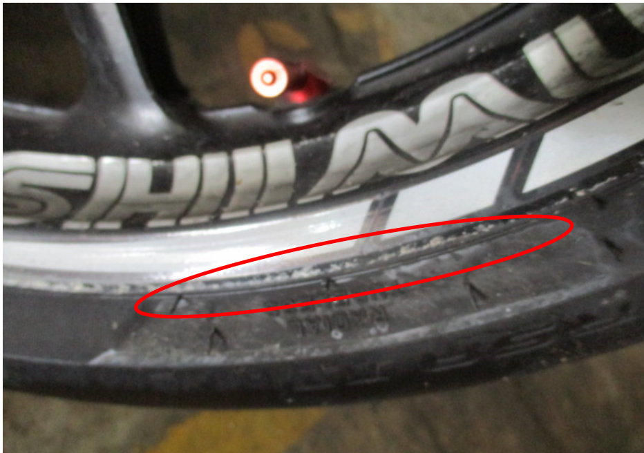
Photo 16 shows the front wheel rim of the Motorcycle at the time of our inspection. Some relatively minor marks of grazing nature were observed on the edges of the front wheel rim (circled), at the right side of the Motorcycle.
