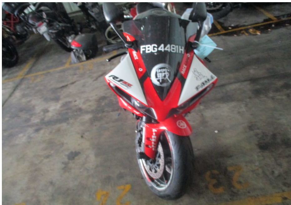
Photo 28 shows the front wheel of the Motorcycle turned towards its full left. Turning the Motorcycle's handle bar towards the left did not produce any abnormal free play and/or resistance. This would indicate that the steering system of the Motorcycle was in serviceable condition at the time of our inspection.
