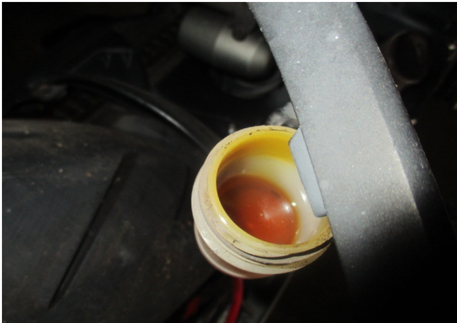
Photo 34 shows the brake fluid reservoir for the rear brake of the Motorcycle. The brake fluid was observed to be of sufficient level and without contamination for operational purposes.
