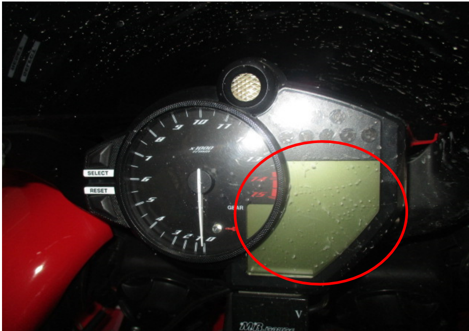
Photo 1 shows a closer view of the speedometer gauge of the Motorcycle. The mileage of the Motorcycle was not recorded at the time of our inspection due to the damage sustained to the odometer display screen as a result of the accident (circled).
