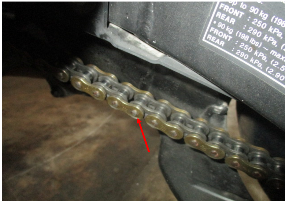
Photo 24 shows the closer view of the gear chain (arrowed) of the Motorcycle, which was observed to be intact with no misalignment. It was also adequately lubricated for operating purposes.
