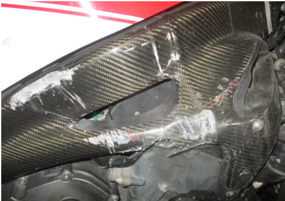
Photo 6 shows a closer view of the cracked right frame cover of the Motorcycle which was amongst the body parts of the Motorcycle damaged as a result of the accident.
