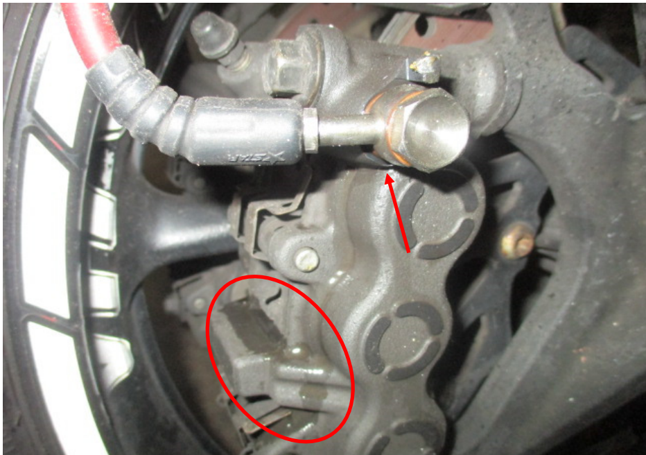
Photo 32 shows the right front brake caliper for the front brake of the Motorcycle. A leakage of brake fluid (circled) was observed from the right front brake banjo bolt (arrowed) when the front brake lever was depressed.
