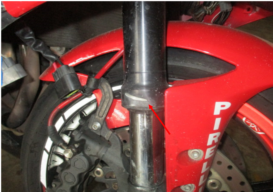
Photo 26 shows the front forks (arrowed) of the Motorcycle. The fork bracket of the Motorcycle was observed to be intact and undamaged. However the right outer fork tube was slightly dented as a result of the accident (arrowed).
