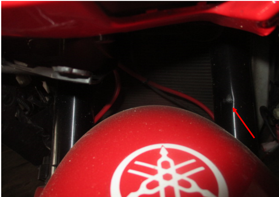
Photo 25 shows the front forks (arrowed) of the Motorcycle. The fork bracket of the Motorcycle was observed to be intact and undamaged. However the left outer fork tube was slightly dented as a result of the accident (arrowed).
