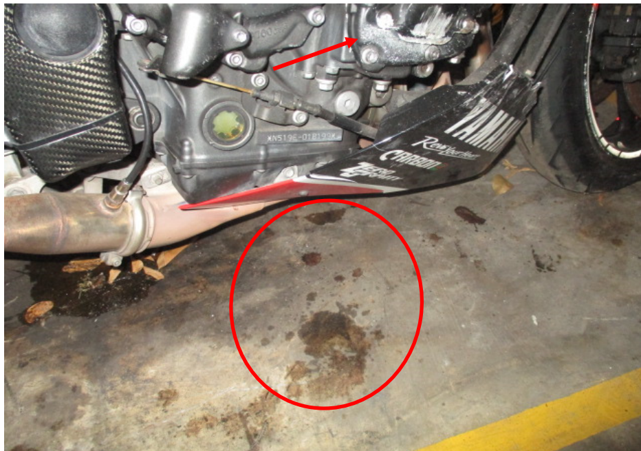
Photo 22 shows wet fluid stains observed on the ground (circled) directly below the damaged right engine cover of the Motorcycle (arrowed), indicating that a fluid leak had occurred as a result of the accident.
