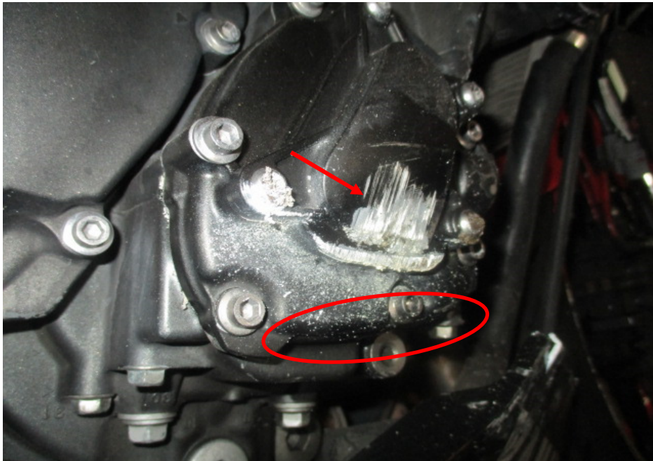
Photo 21 shows the right side of the engine of the Motorcycle at the time of our inspection. The various left engine components had sustained damage of grazing nature as a result of the accident (arrowed). Wet fluid stains were observed on the underside of the damaged right engine cover of the Motorcycle (circled).
