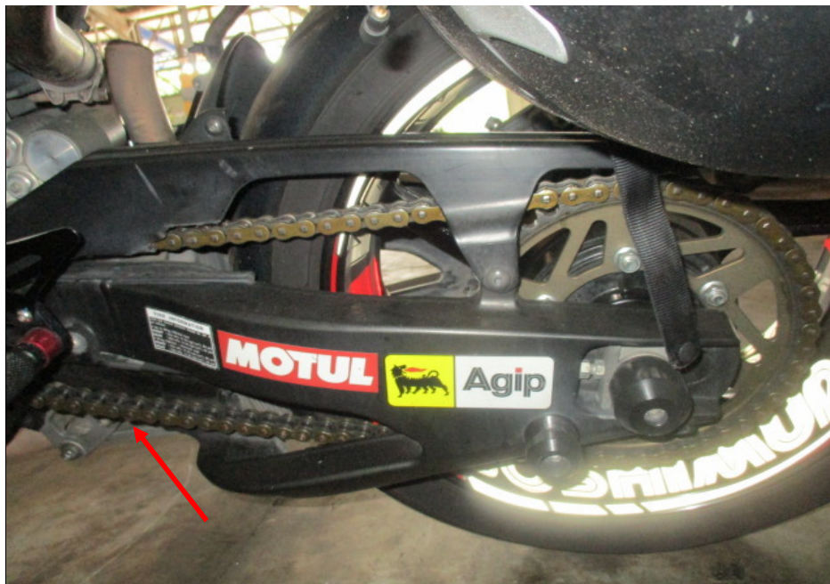
Photo 23 shows the gear chain (arrowed) of the Motorcycle, which was observed to be intact with no misalignment. It was also adequately lubricated for operating purposes. The gear chain rotates the rear wheel of the Motorcycle.
