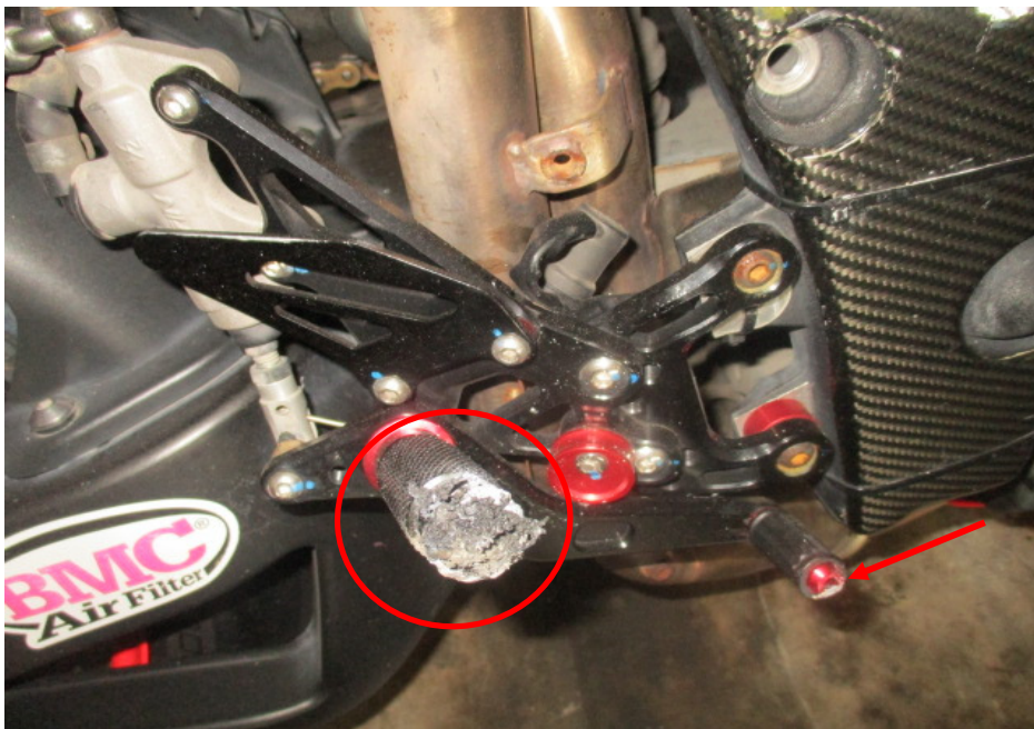
Photo 12 shows a closer view of the right front footrest (circled) and rear brake pedal (arrowed) which were amongst the body parts of the Motorcycle that had sustained damage as a result of the accident.
