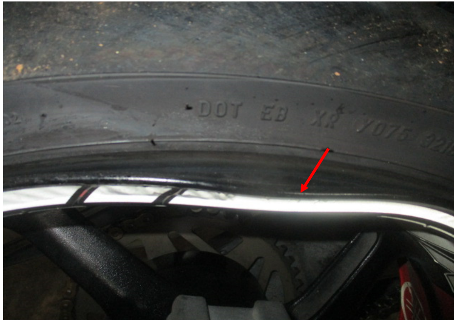
Photo 19 shows a close up view of the bent rear wheel rim of the Motorcycle at the time of our inspection (arrowed).
