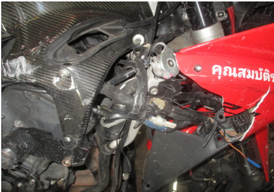
Photo 10 shows a closer view of the broken right cowling of the Motorcycle as a result of the accident.
