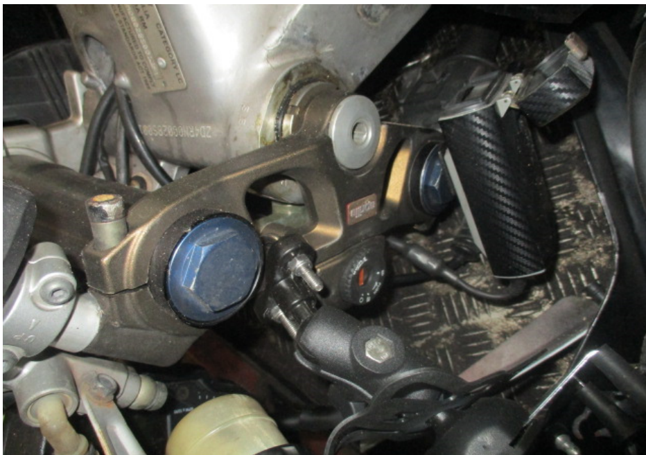
Photo 6 shows a closer view of the top clamp, side mirrors and handlebars of the Motorcycle. These parts were amongst the body parts of the Motorcycle which were damaged as a result of the accident.
