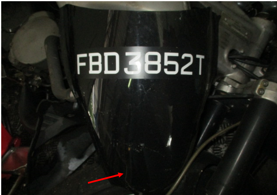
Photo 4 shows a closer view of the cracked windshield the Motorcycle as a result of the accident (arrowed).
