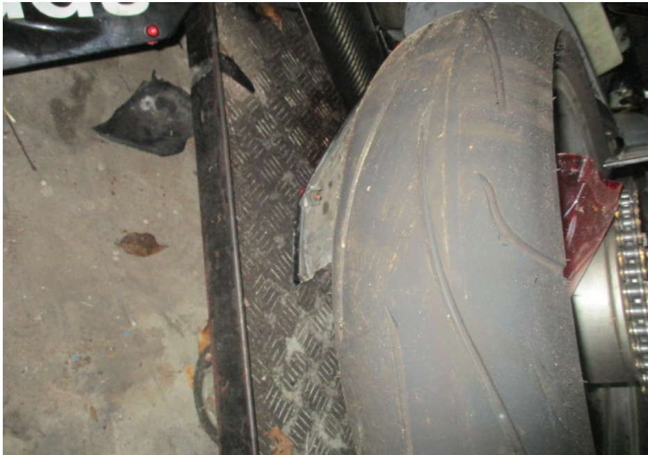
Photo 11 shows the condition of the Motorcycle's rear tyre. The rear tyre was observed to be in serviceable condition with remaining tread depth of approximately 6mm. The tyre was also observed to be sufficiently inflated for vehicular operation. We did not observe any tear, burst mark(s) and/or punctured hole(s) on the sidewalls as well as across the tread of the rear tyre.
