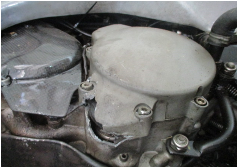
Photo 12 shows the right side of the engine of the Motorcycle at the time of our inspection. We had observed a crack at the bottom of the right engine cover which was a result of the accident. However there was no sign(s) or indication(s) of fluid leak observed around the right engine area of the Motorcycle.
