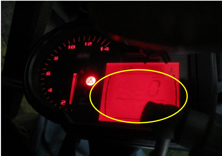
Photo 5 shows a closer view of the speedometer gauge of the Motorcycle. The mileage of the Motorcycle at the time of our inspection was not recorded due to the damage sustained to the speedometer display screen as a result of the accident (circled).
