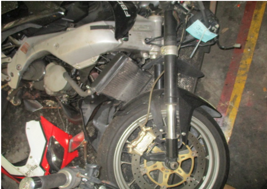
Photo 15 shows the front forks of the Motorcycle. The accident had rendered the Motorcycle immobile. We were hence not able to conduct any tests on the steering system of the Motorcycle.
