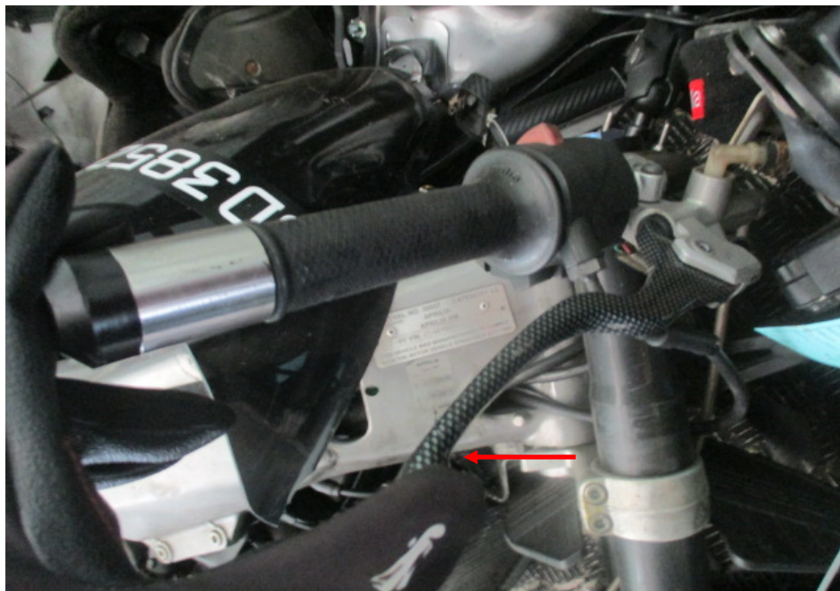
Photo 17 shows the front brake lever being depressed. There was some resistance felt (spongy like feel) upon pressing the front brake lever (arrowed). This would indicate that there is no leakage of pressure/vacuum in the brake system.
