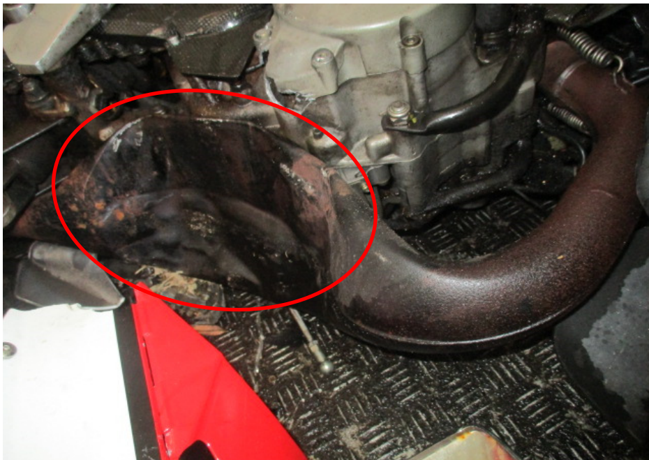
Photo 8 shows a closer view of the dented exhaust pipe of the Motorcycle as a result of the accident (circled).
