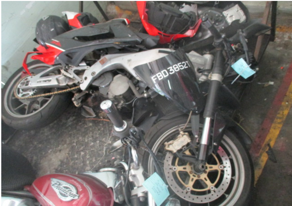
Photo 1 shows a general view of the right body of the Motorcycle at the time of our inspection. The Motorcycle had sustained damages all around. Body parts that were found to have been damaged include its windshield, head cowl, speedometer gauge, side mirrors, top clamp, handlebars, right cowling, fuel tank, rear brake pedal bracket and exhaust pipe, amongst others.
