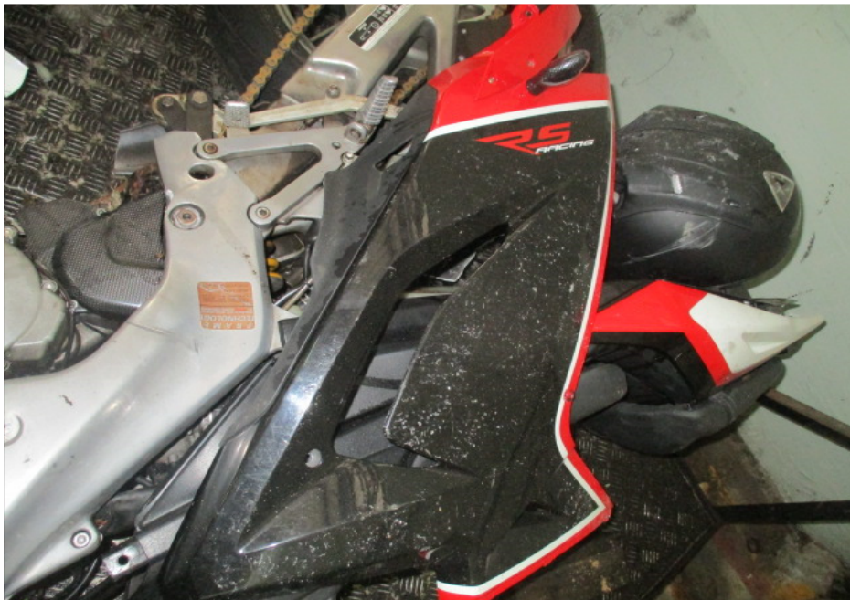
Photo 2 shows a closer view of the right cowling which was amongst the body parts of the Motorcycle that had sustained damage as a result of the accident.
