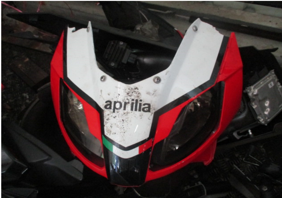
Photo 3 shows a closer view of the head cowling which was amongst the body parts at the front body of the Motorcycle that had sustained damage as a result of the accident.
