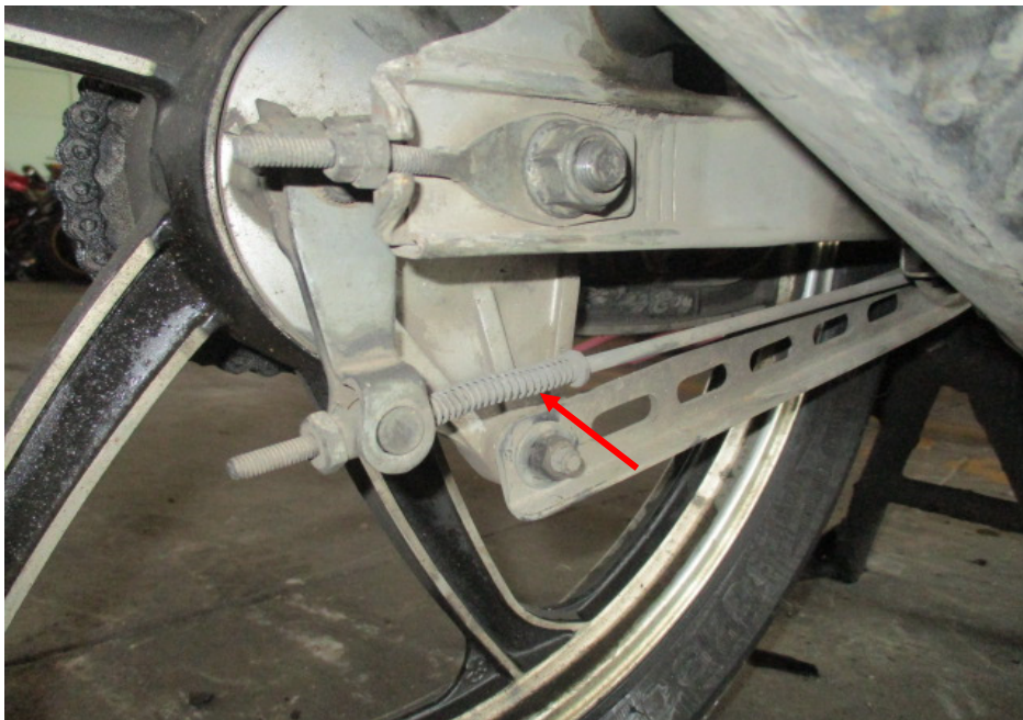
Photo 26 shows the rear wheel of the Motorcycle. The type of brake system for the rear wheel was of a mechanical type, controlled by the brake foot pedal of the Motorcycle. Our checks of the cable (arrowed), spring and drum which are all part of the components in the rear brake system of the Motorcycle reveal all to be intact and without damage.
