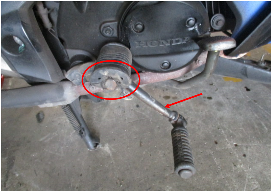
Photo 9 shows a closer view of the right front footrest (circled) and the kickstart pedal (arrowed) which were amongst the body parts of the Motorcycle that had sustained damage as a result of the accident.
