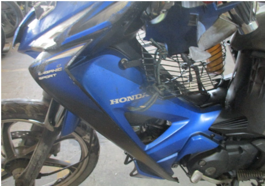
Photo 7 shows a closer view of the left cowling of the Motorcycle that had sustained damages as a result of the accident.
