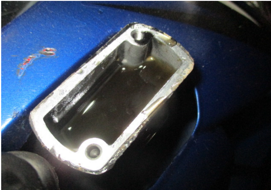
Photo 24 shows the brake fluid reservoir for the front brake of the Motorcycle. The brake fluid was observed to be without contamination and of sufficient level for operational purposes.
