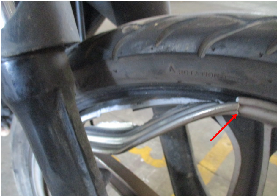
Photo 16 shows a closer view of the broken front wheel rim of the Motorcycle as a result of the accident (arrowed).
