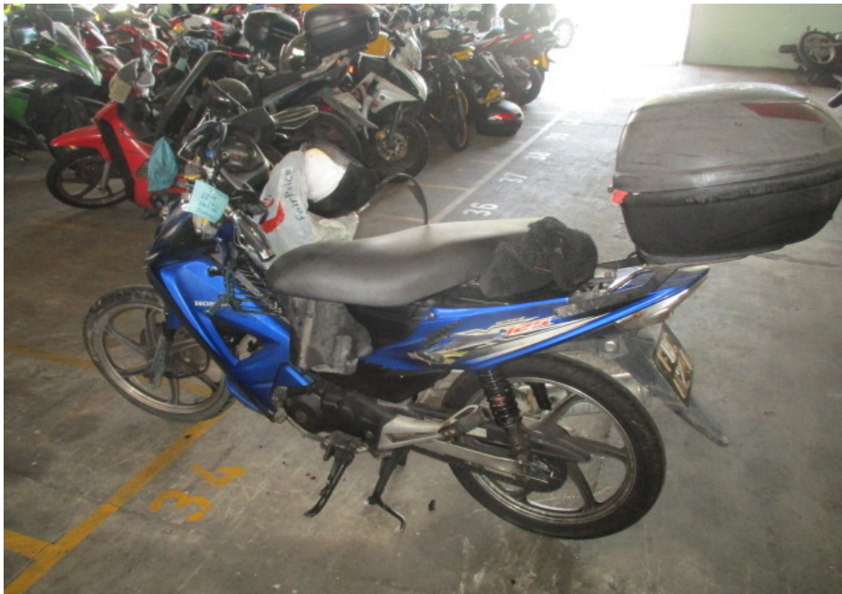
Photo 3 shows a general view of the left body of the Motorcycle at the time of our inspection. The Motorcycle was observed to have sustained damages all around. Amongst the body parts that were found to have been damaged include its headlamp assembly, front cowling, side cowlings, left handlebar grip, left side mirror, left front footrest, gear shift pedal, rear side covers and exhaust muffler, amongst others.
