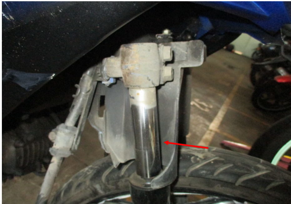
Photo 22 shows the front right fork of the Motorcycle. The front right fork was observed to be bent (arrowed) as a result of the accident. We were hence not able to conduct any tests on the steering system of the Motorcycle.
