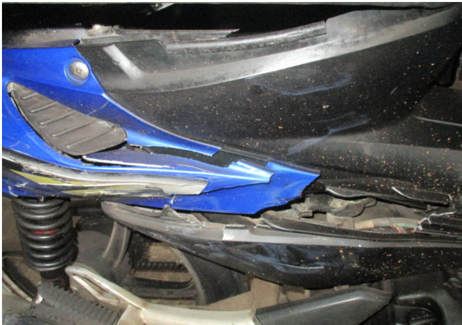
Photo 13 shows a closer view of the right rear side cover of the Motorcycle that had cracked as a result of the accident.
