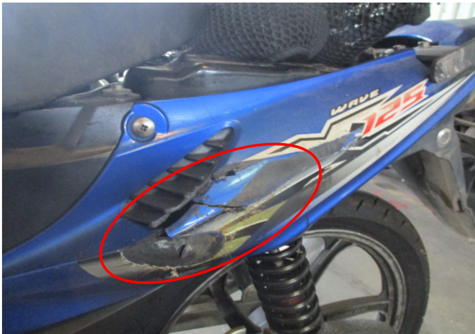
Photo 11 shows the left rear side cover of the Motorcycle which was observed to be cracked as a result of the accident (circled).
