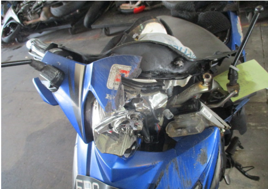
Photo 4 shows a closer view of the cracked headlamp assembly which was amongst the body parts at the front body of the Motorcycle that had sustained damage as a result of the accident.
