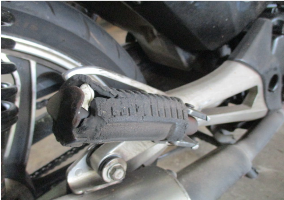
Photo 14 shows a closer view of the right pillion foot peg which was amongst the body parts of the Motorcycle that had sustained damage as a result of the accident.
