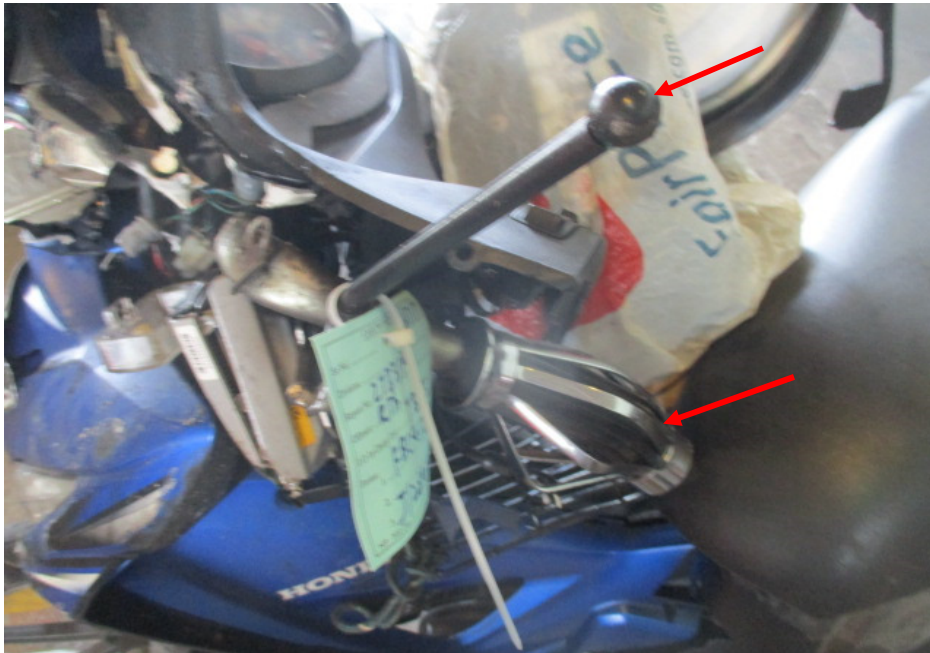
Photo 8 shows a closer view of the left handlebar grip and left side mirror (arrowed) which were amongst the body parts of the Motorcycle that had sustained damage as a result of the accident.
