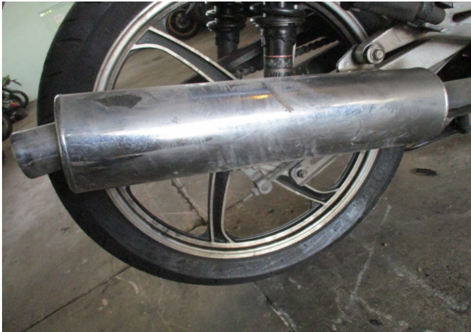
Photo 12 shows the exhaust muffler which was amongst the body parts of the Motorcycle that had sustained damages of grazing nature as a result of the accident.
