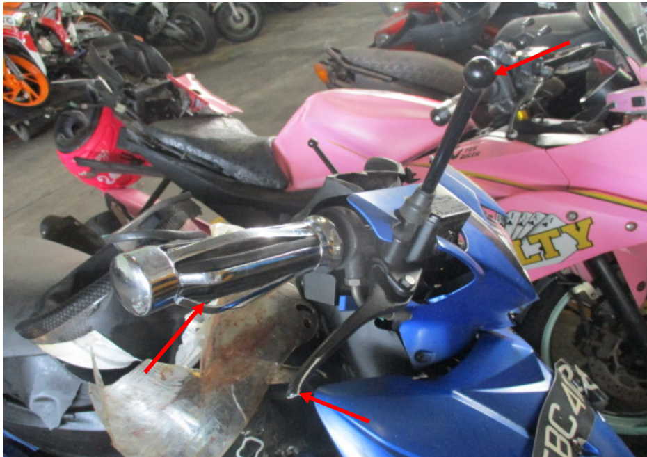
Photo 6 shows a closer view of the front brake lever, left side mirror and right handlebar grip (arrowed) which were amongst the body parts at the front body of the Motorcycle that had sustained damage as a result of the accident.
