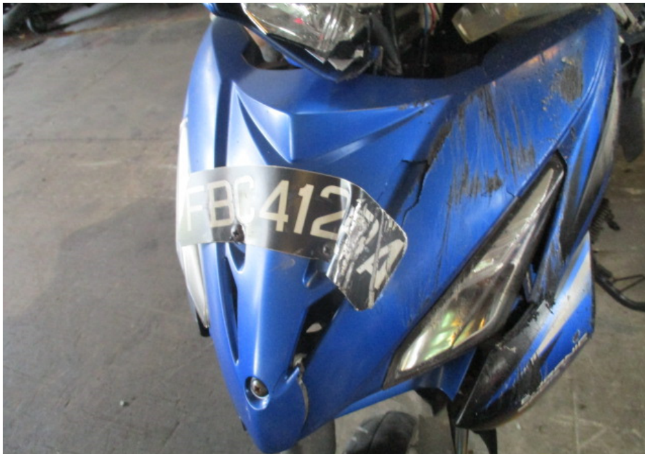
Photo 5 shows a close up view of the cracked front cowling which was amongst the body parts of the Motorcycle that had sustained damage as a result of the accident.
