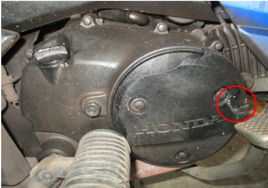
Photo 19 shows the right side of the engine of the Motorcycle at the time of our inspection. The outer engine cover at the right side of the Motorcycle had cracked as a result of the accident (circled) however the engine components were still intact. There was also no fluid leak and/or fluid stain found around the right engine area of the Motorcycle.
