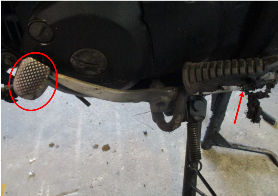
Photo 10 shows a closer view of the left front footrest (arrowed) and gear shift pedal (circled) which were amongst the body parts of the Motorcycle that had sustained damage as a result of the accident.
