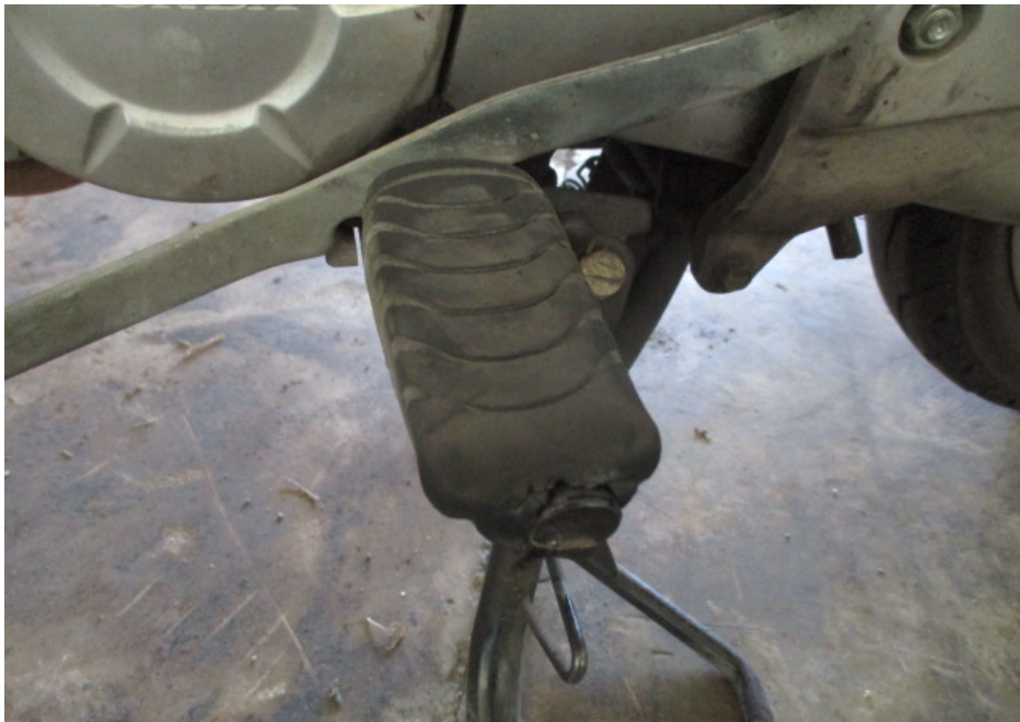
Photo 11 shows a closer view of the left front footrest which was amongst the body parts of the Motorcycle that had sustained damage as a result of the accident.
