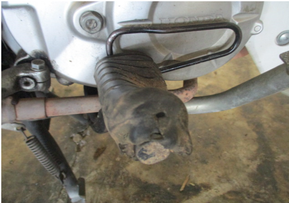
Photo 14 shows a closer view of the right front foot rest which was amongst the body parts of the Motorcycle that had sustained damage as a result of the accident.
