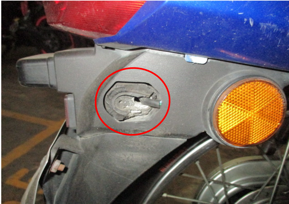
Photo 10 shows a closer view of the broken right rear signal lamp of the Motorcycle as a result of the accident (circled).
