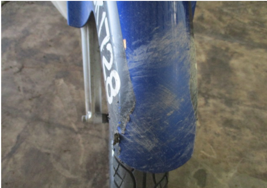
Photo 6 shows a close up view of the front mudguard which was amongst the body parts of the Motorcycle that had sustained damage as a result of the accident.
