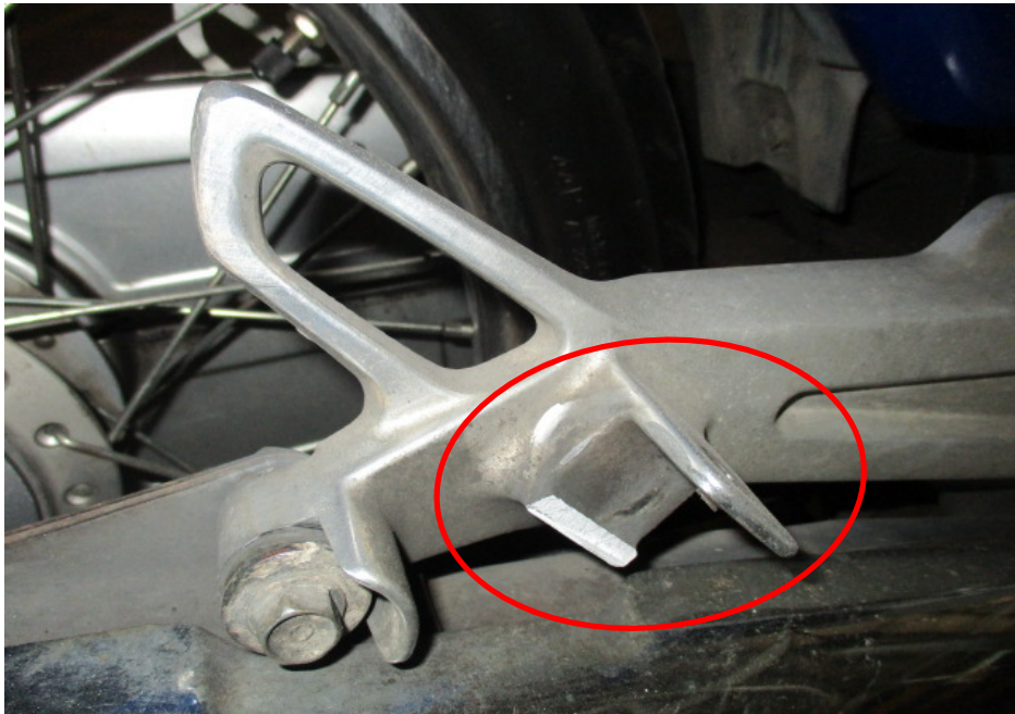
Photo 10 shows a closer view of the broken right pillion foot peg of the Motorcycle as a result of the accident (circled).
