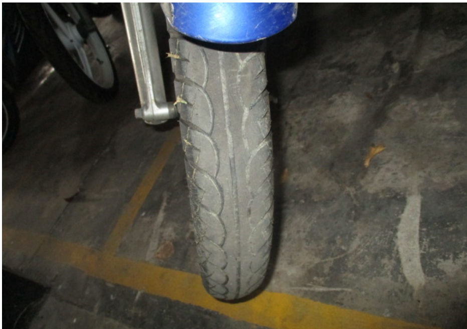
Photo 16 shows the condition of the Motorcycle's front tyre. The front tyre was observed to be in serviceable condition with remaining tread depth of approximately 3mm. There was no tear, burst mark(s) and/or punctured hole(s) on the sidewalls as well as across the tread of the front tyre.
