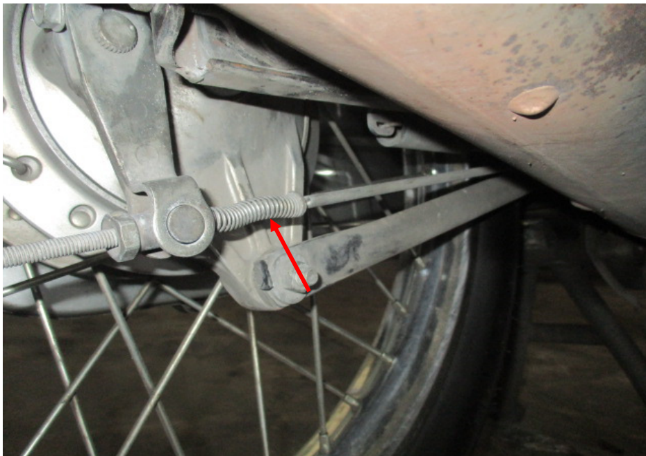
Photo 25 shows the rear wheel of the Motorcycle. The type of brake system for the rear wheel was of a mechanical type, controlled by the brake foot pedal of the Motorcycle. Our checks of the cable (arrowed), spring and drum which are all part of the components in the rear brake system of the Motorcycle reveal all to be intact and without damage.
