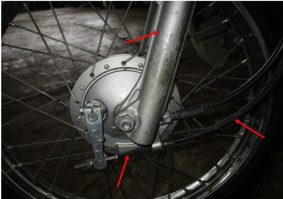
Photo 24 shows a close up view of the front fork, front brake cables and spring of the Motorcycle (arrowed), which are all part of the components in the mechanical front brake system of the Motorcycle. Our visual checks of these various components had revealed all to be intact with no visible damage.
