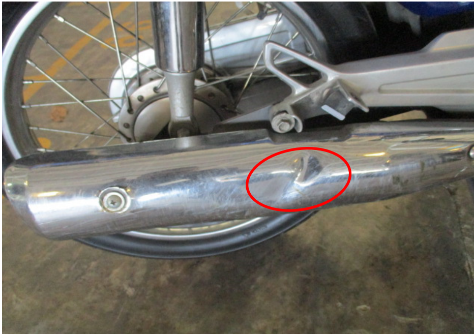
Photo 15 shows a closer view of the dented exhaust muffler heat shield of the Motorcycle as a result of the accident (circled).
