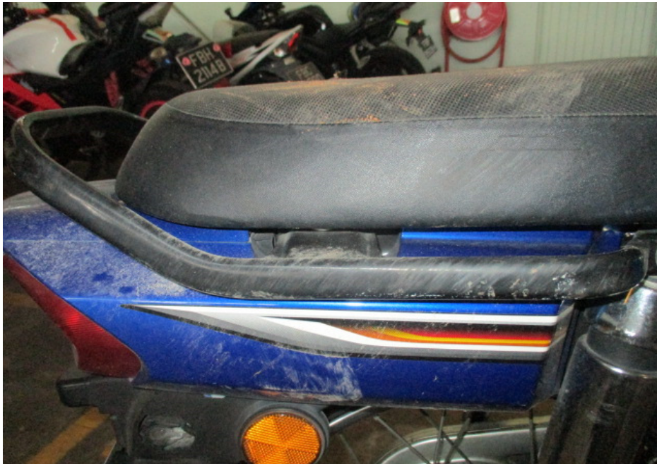
Photo 8 shows a closer view of the pillion grab rail of the Motorcycle that had sustained damages of grazing nature as a result of the accident.
