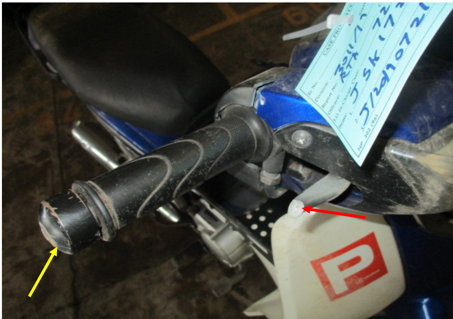
Photo 9 shows a closer view of the right handlebar end (yellow arrow) and broken front brake lever (red arrow) which were amongst the body parts of the Motorcycle that had sustained damage as a result of the accident.
