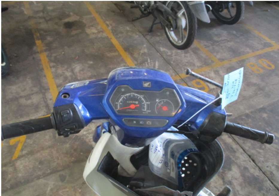
Photo 7 shows a closer view of the missing side mirrors of the Motorcycle as a result of the accident.
