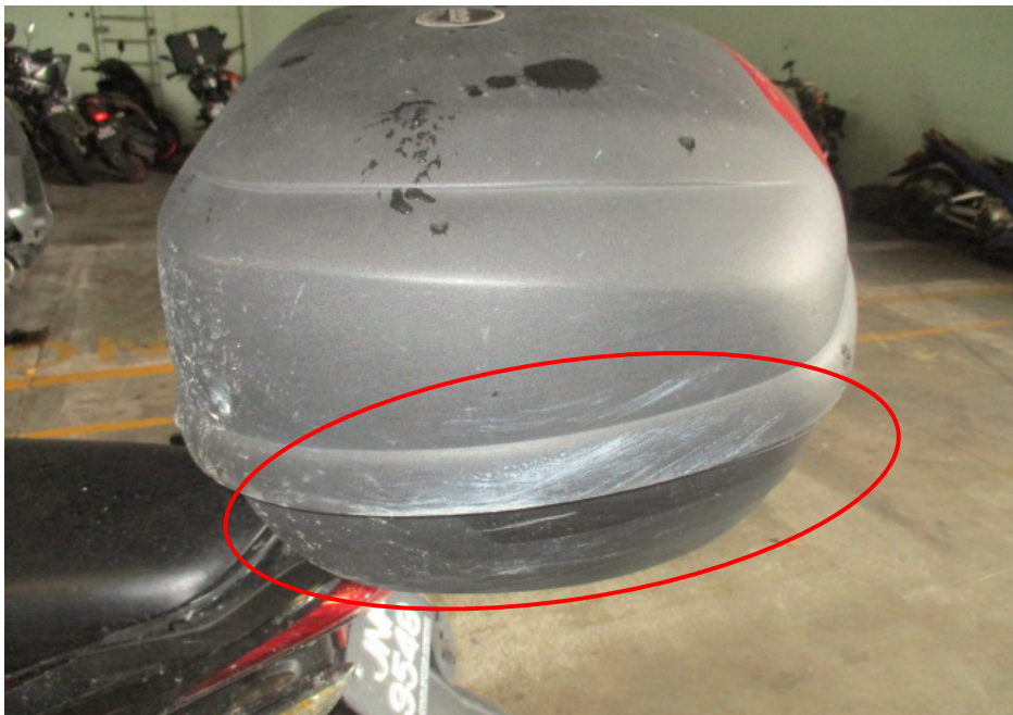
Photo 12 shows a closer view of the top box of the Motorcycle which had sustained damage due to the accident (circled).
