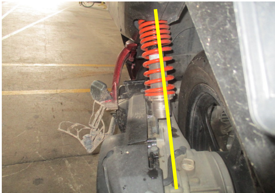
Photo 17 shows the left shock absorber of the Motorcycle which was found to be intact without any misalignment.
