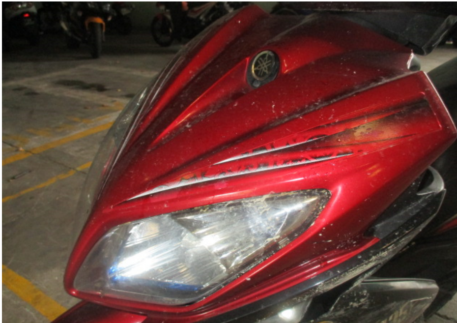
Photo 4 shows a closer view of the front cowling of the Motorcycle at the time of our inspection. The Motorcycle was also observed to have sustained cracked headlights due to the accident.
