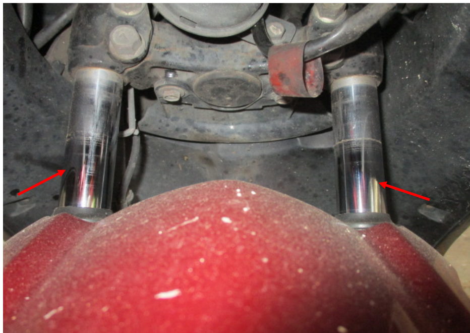
Photo 19 shows the front forks (arrowed) of the Motorcycle. The front forks and fork brackets of the Motorcycle were both found to be intact and undamaged. Turning the Motorcycle's handle bar towards the left and right did not produce any abnormal free play and/or resistance. The steering system of the Motorcycle was in serviceable condition at the time of our inspection.
