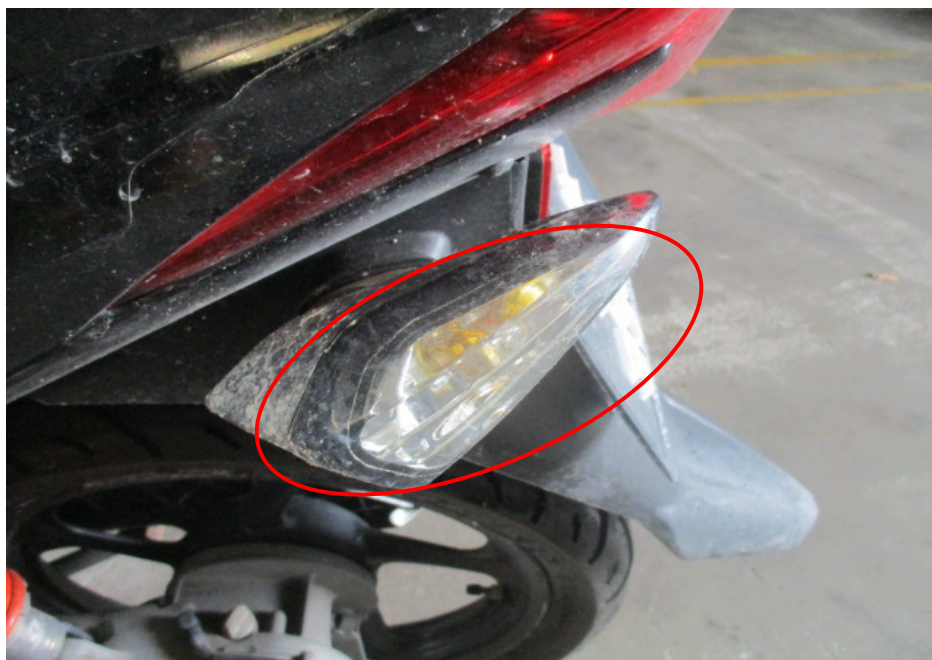
Photo 10 shows a closer view of the grazed left rear signal lamp of the Motorcycle at the time of our inspection (circled).
