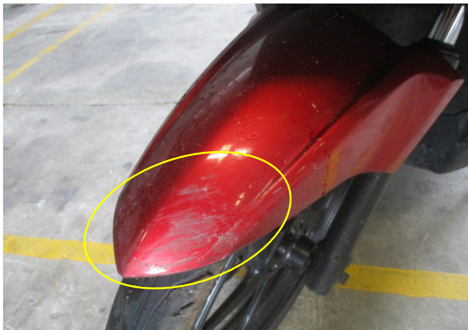
Photo 5 shows a closer view of the front mudguard which was amongst the body parts at the front body of the Motorcycle that had sustained damage as a result of the accident (circled.)
