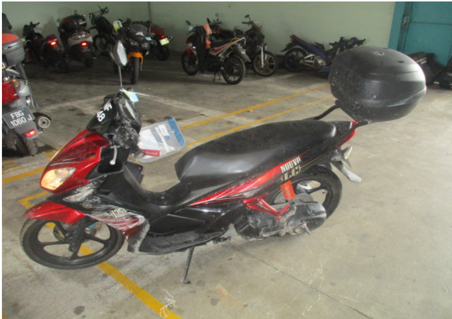
Photo 3 shows a general view of the left body of the Motorcycle at the time of our inspection. The body parts that were found to have been damaged include its front cowling, headlamps, front mudguard, rear brake lever, left side mirror, left side cowling, left rear side cover, left pillion foot rest, left rear signal lamp and top box, amongst others as a result of the accident.
