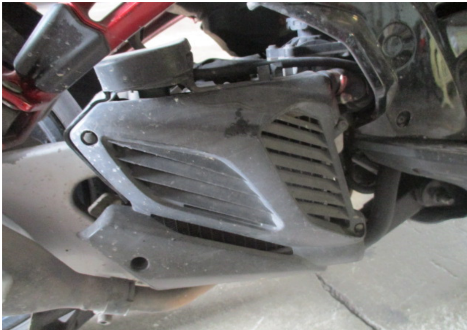
Photo 15 shows the radiator of the Motorcycle at the time of our inspection. The radiator was found to be intact with no visible damage. There was also no sign(s) or indication(s) of fluid leak observed around the radiator of the Motorcycle.
