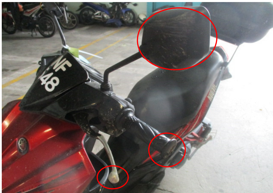
Photo 6 shows a closer view of the left side mirror, left handlebar end and rear brake lever of the Motorcycle which were observed to be damaged due to the accident (circled).
