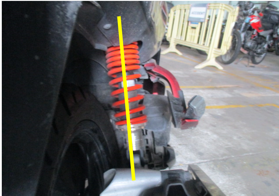
Photo 18 shows the right shock absorber of the Motorcycle which was found to be intact without any misalignment.
