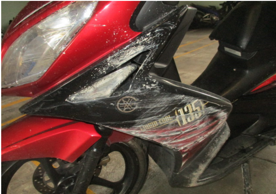
Photo 7 shows the damaged left side cowling of the Motorcycle. The damage sustained was mainly of grazing nature.
