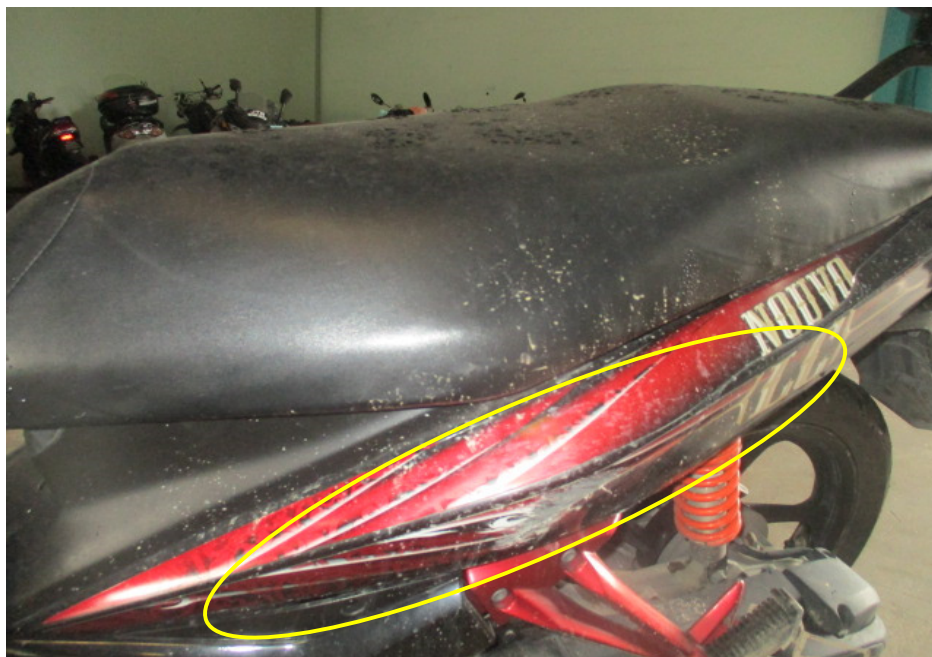
Photo 9 shows a closer view of the damaged left rear side cover of the Motorcycle which was observed to have sustained scratches due to the accident (circled).
