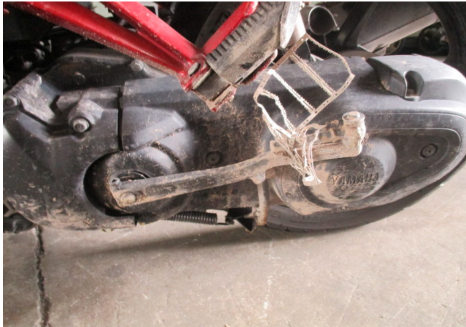
Photo 16 shows the drive train of the Motorcycle which was found to be intact without any misalignment.
