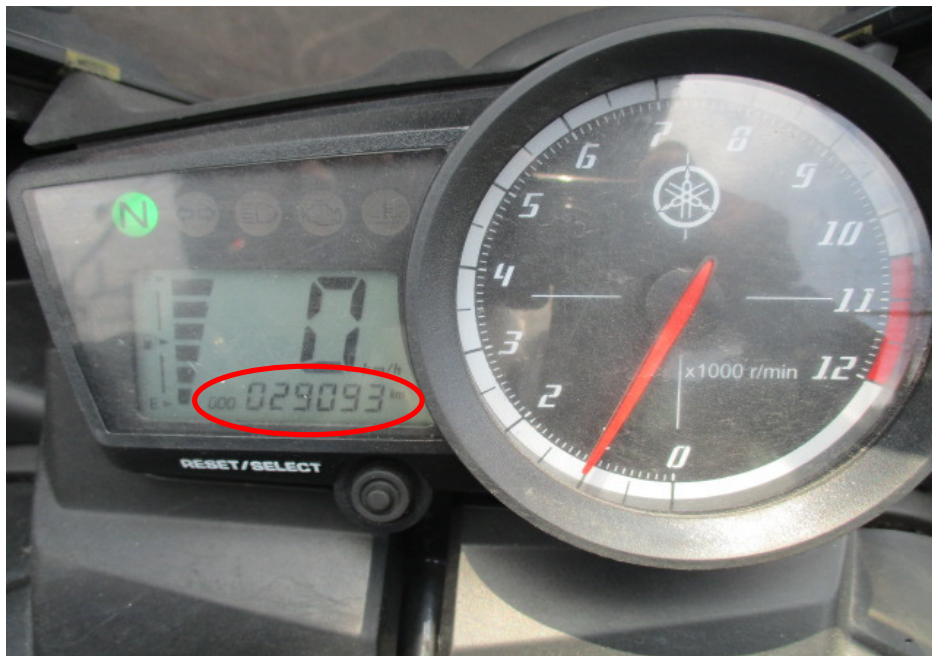
Photo 1 shows the speedometer gauge of the Motorcycle where the mileage recorded at the time of our inspection was 29, 093km (circled).
