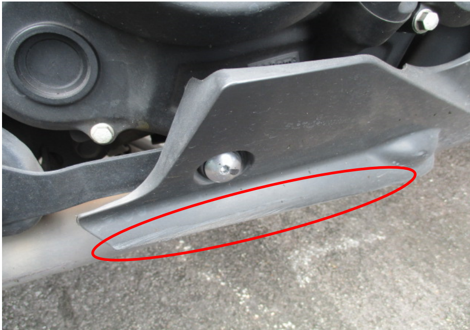
Photo 12 shows a closer view of the right bottom cowling which was amongst the body parts of the Motorcycle that had sustained damages of grazing nature as a result of the accident (circled).
