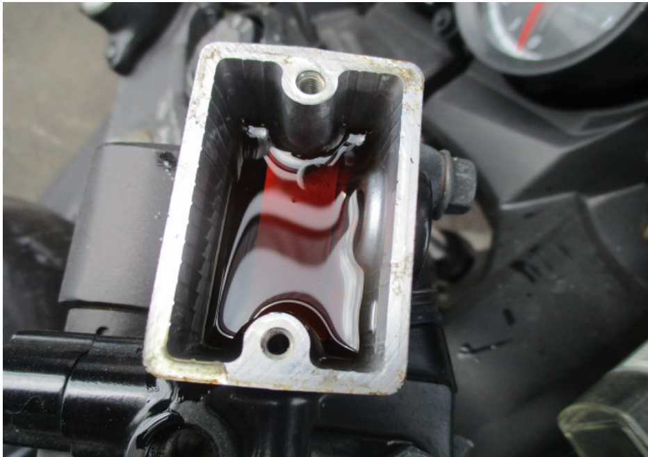
Photo 24 shows the brake fluid reservoir for the front brake of the Motorcycle. The brake fluid was observed to be of sufficient level and without contamination for operational purposes.
