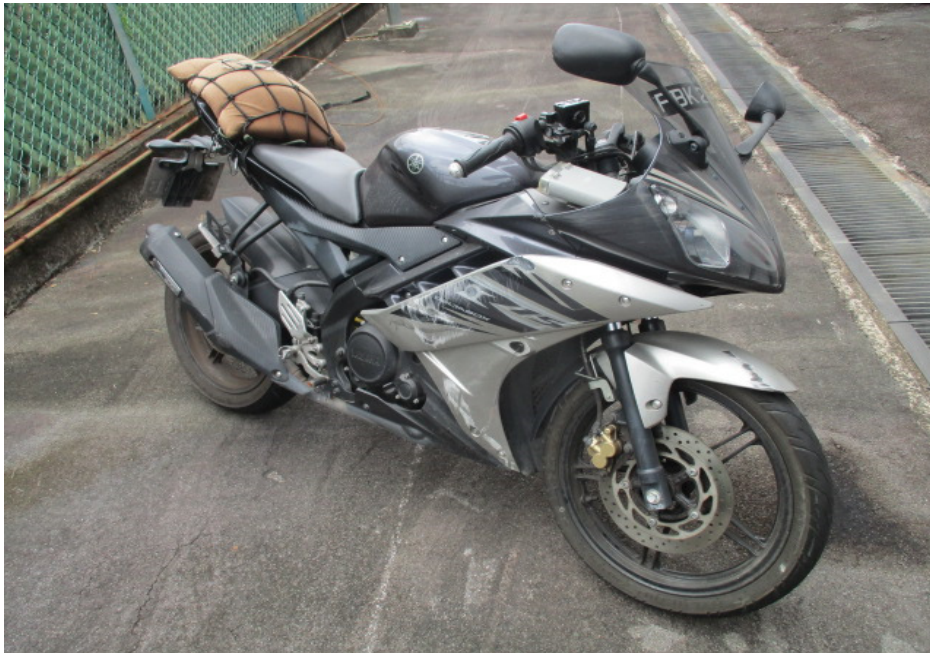
Photo 4 shows a general view of the right body of the Motorcycle at the time of our inspection. The Motorcycle was observed to have sustained damages at its frontal portion and right body. Amongst the body parts that were found to have been damaged include its head cowling, right side cowling, right handlebar end, right side mirror, front brake lever, rear brake pedal, right front footrest, right rear side cover and exhaust muffler, amongst others.
