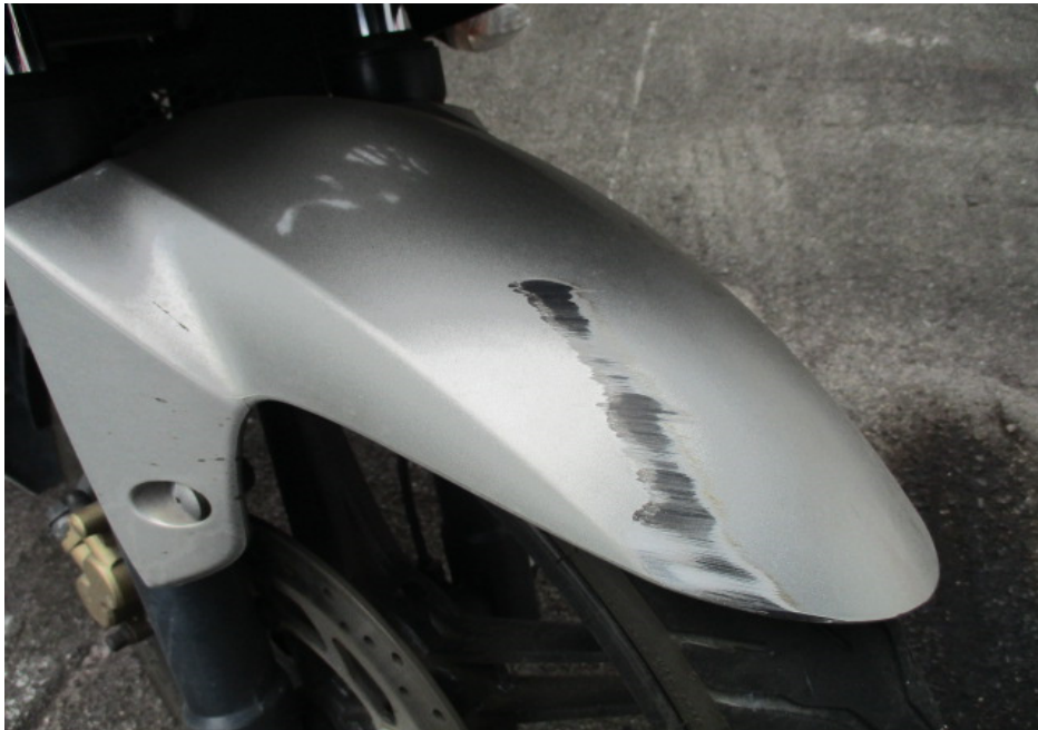
Photo 7 shows a closer view of the front mudguard which was amongst the body parts at the front body of the Motorcycle that had sustained damage as a result of the accident.
