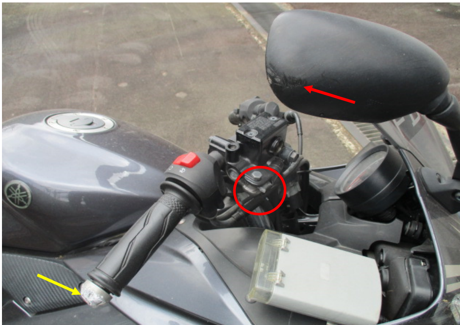
Photo 9 shows a closer view of the right handlebar end (yellow arrow), right side mirror (red arrow) and broken front brake lever (circled) which were amongst the body parts of the Motorcycle that had sustained damage as a result of the accident.
