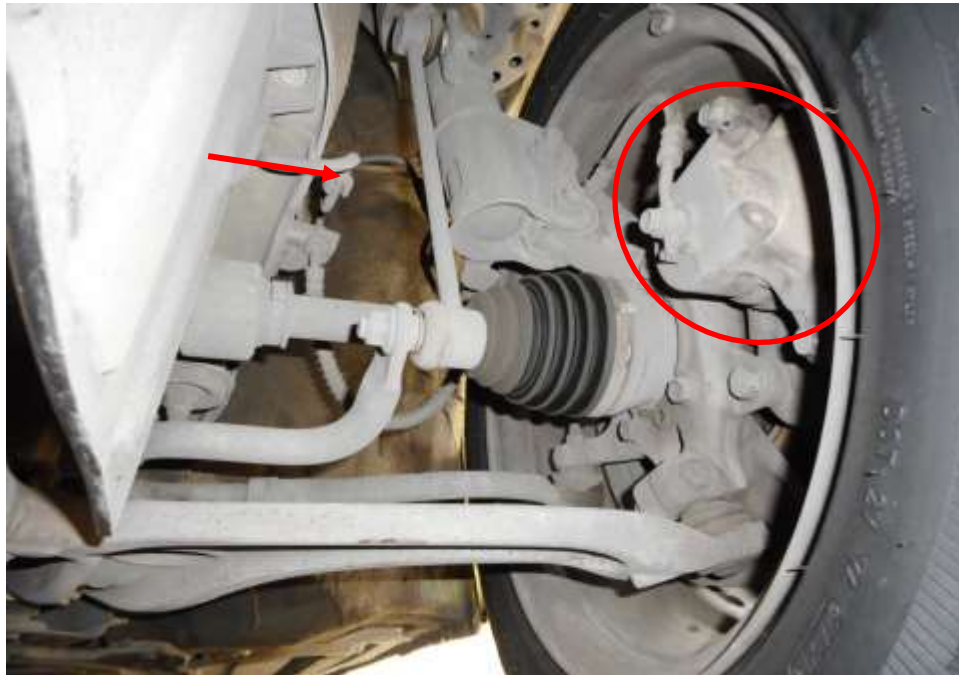
Photo 20 shows the brake hose/pipe (arrowed) at the front left wheel of the Motor Taxi. No leakage of brake fluid was observed. Visual examination of the various components of the braking system like the brake caliper (circled), brake booster, brake pedal etc had revealed all to be intact and without visible damage.
