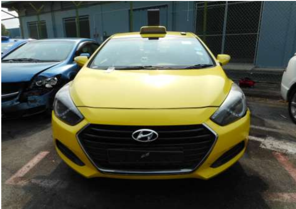
Photo 2 shows a general view of the Motor Taxi's front body at the time of my inspection. The Motor Taxi was observed to have sustained damage at its frontal portion. Its front bumper and front number plate were amongst the body parts that were damaged as a result of the accident.
