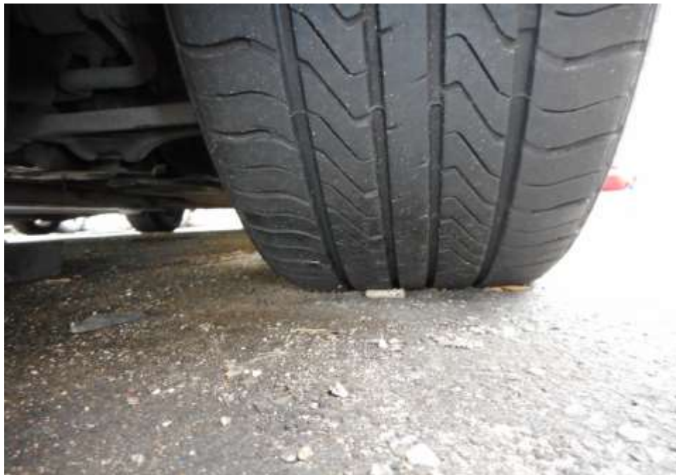
Photo 11 shows the condition of the front left tyre of the Motor Taxi, which was observed to be in serviceable condition with remaining tread depth of approximately 4.1mm. There was also no tear, cut or burst mark(s) on the outer and the inner sidewalls as well as across the tread of the Motor Taxi's 4 tyres.
