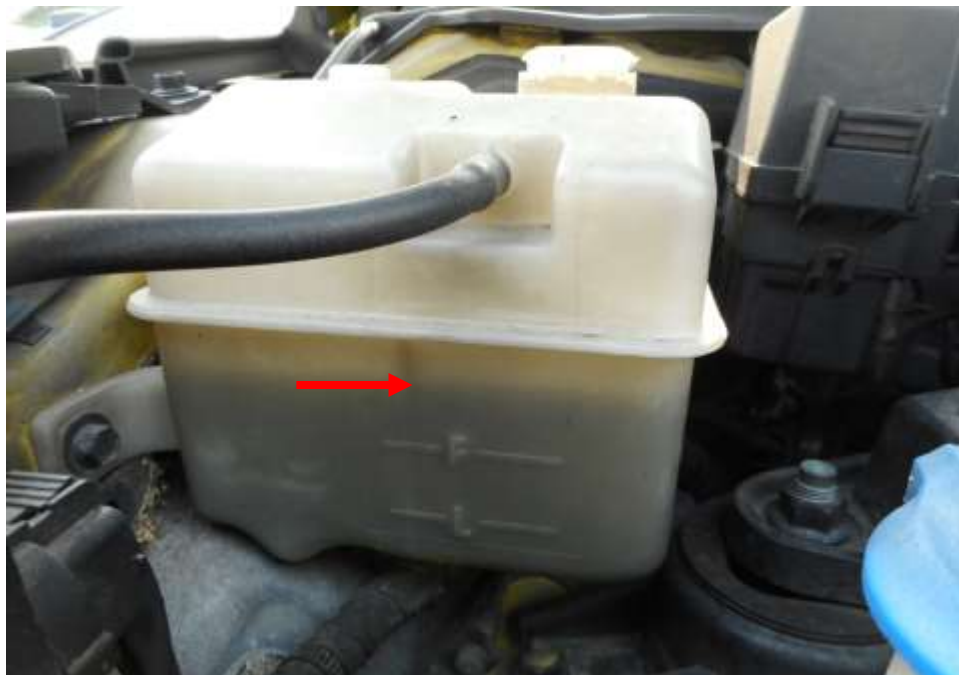
Photo 14 shows checks being carried out to the engine coolant of the Motor Taxi at the time of my inspection. The engine coolant was observed to be of sufficient level (arrowed) and without any visible contamination.
