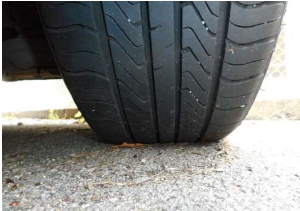
Photo 10 shows the condition of the rear left tyre of the Motor Taxi, which was observed to be in serviceable condition with remaining tread depth of approximately 5.6mm. The tyre, which was wrapped around steel wheel rim, was also observed to be sufficiently inflated for vehicular operation. The 4 tyres of the Motor Taxi were wrapped around standard steel wheel rims.
