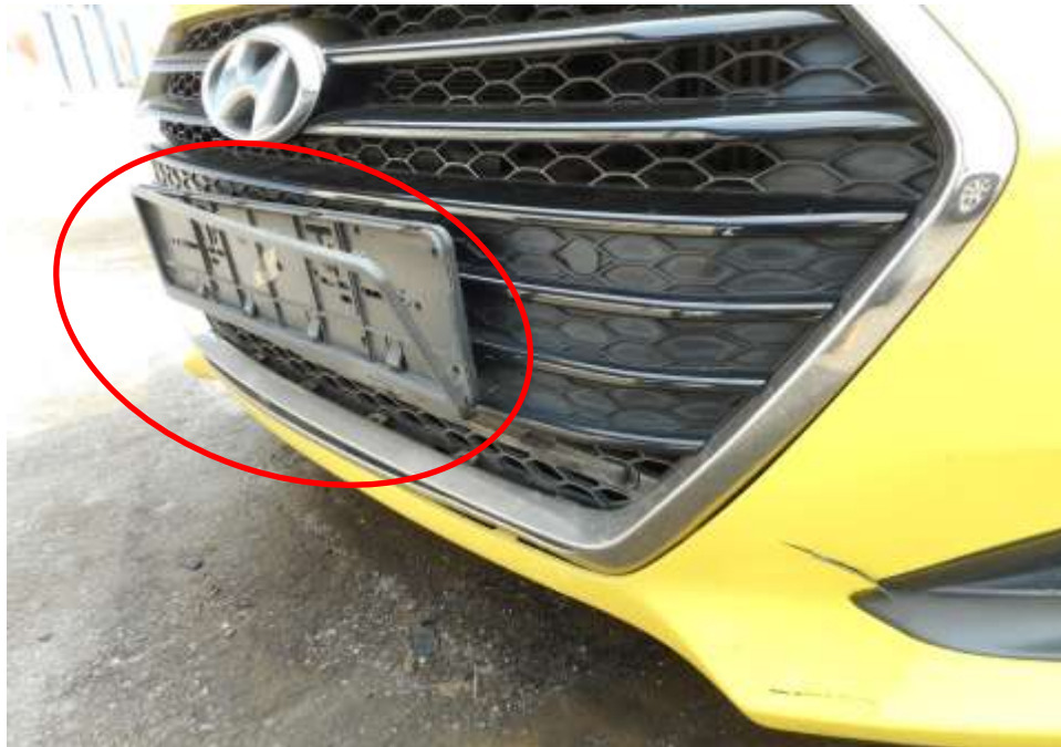
Photo 4 shows the close up view of the Motor Taxi's front body at the time of my inspection. The Motor Taxi was observed to have sustained damage at its front number plate (circled) as a result of the accident.
