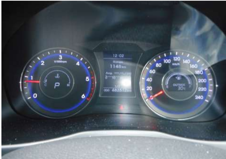
Photo 25 shows no warning lights illuminated on the instrument panel of the Motor Taxi after the engine was cranked. This would suggest that there was no abnormality to the various electronic operating systems of the Motor Taxi, like the ABS, EPS, TC and SRS etc.
