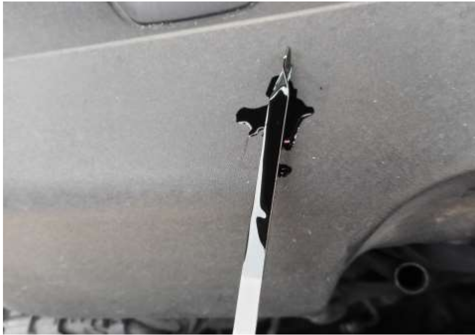
Photo 15 shows the engine oil dip stick of the Motor Taxi at the time of my inspection. The engine oil was observed to be of sufficient level and without any visible contamination.
