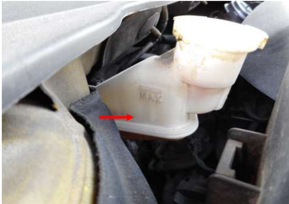
Photo 13 shows the brake fluid reservoir of the Motor Taxi at the time of my inspection. The brake fluid was observed to be of sufficient level (arrowed) and without any visible contamination.
