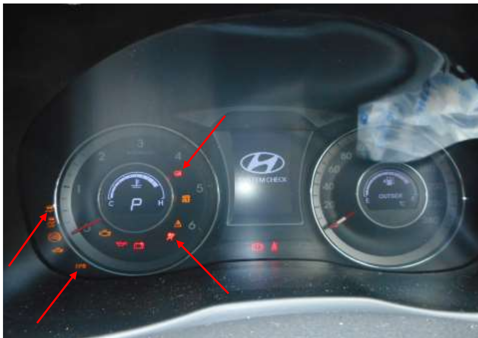
Photo 24 shows the warning light for Anti-Lock Brake System (ABS), Electric Power Steering System (EPS) Traction control (TC) and Supplemental Restraint System (SRS) appearing on the instrument panel of the Motor Taxi during the self-test of its various electronic operating systems when its engine was cranked.
