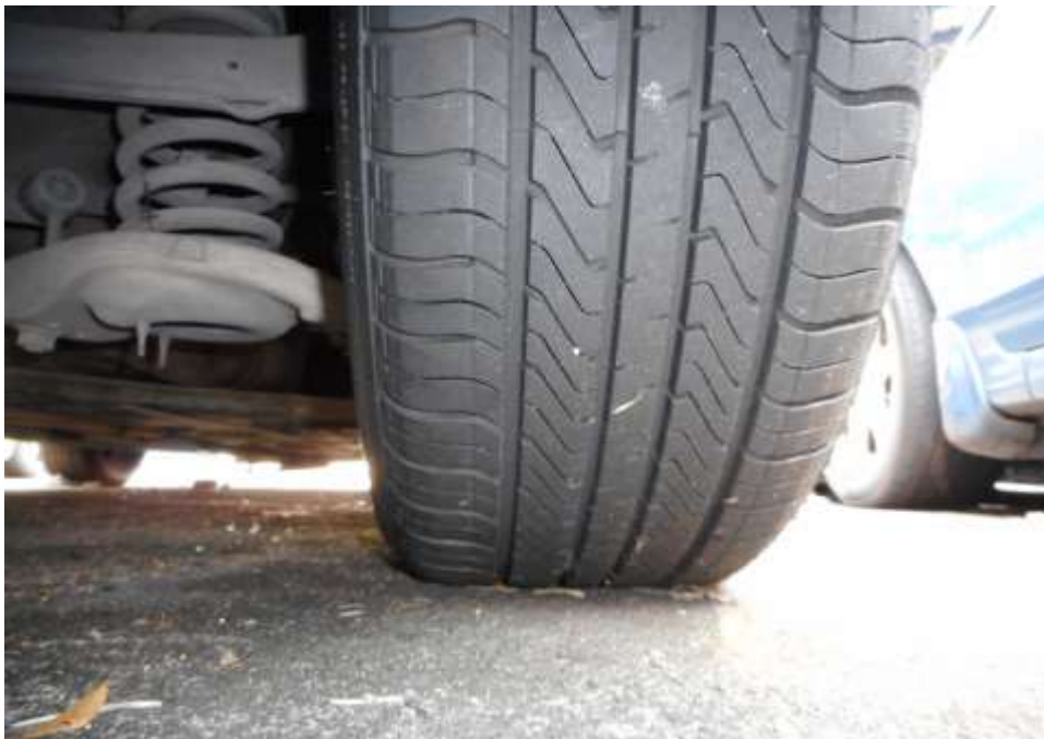
Photo 9 shows the condition of the rear right tyre of the Motor Taxi, which was observed to be in serviceable condition with remaining tread depth of approximately 6.4mm. The tyre was also observed to be sufficiently inflated for vehicular operation with no tear, cut or burst mark(s).
