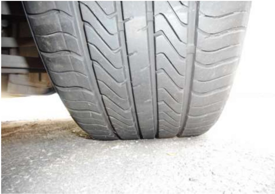
Photo 8 shows the condition of the front right tyre of the Motor Taxi, which was observed to be in serviceable condition with remaining tread depth of approximately 5.9mm. The tyre was sufficiently inflated for vehicular operation with no tear, cut or burst mark(s) on the outer and the inner sidewalls as well as across the tread. The 4 tyres of the Motor Taxi were wrapped around standard steel wheel rims without any damage.
