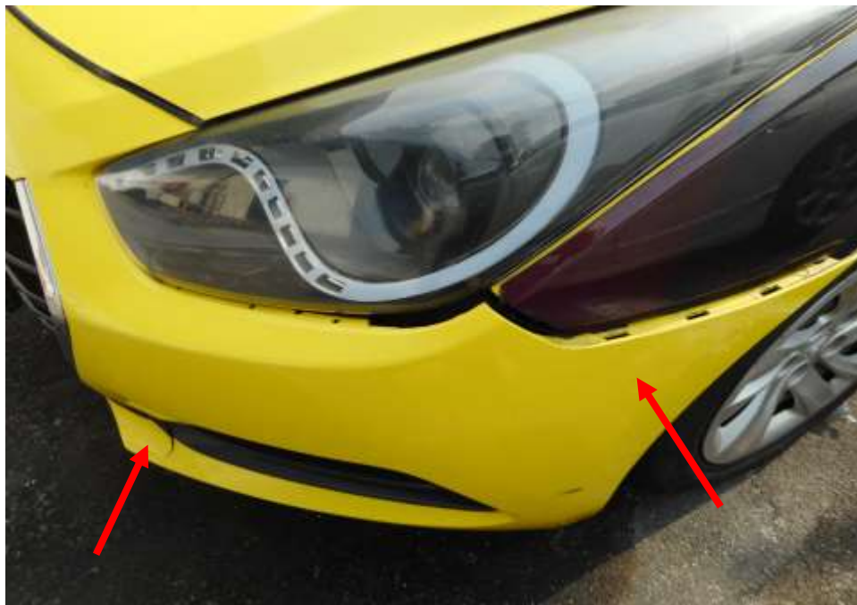
Photo 5 shows the close up view of the Motor Taxi's front body at the time of my inspection. The Motor Taxi was observed to have sustained damage at its front bumper (arrowed) as a result of the accident.
