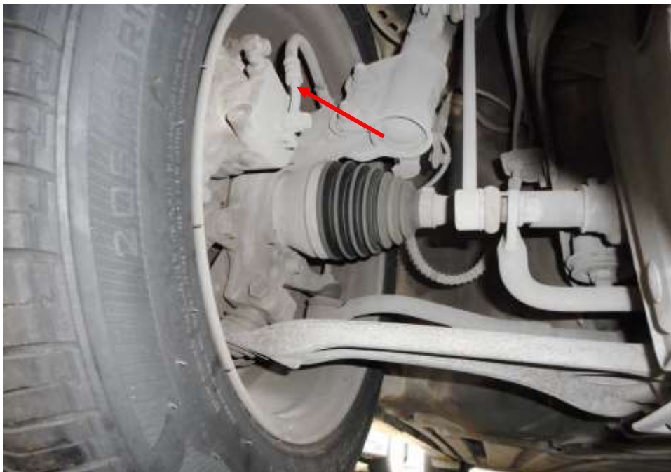
Photo 19 shows the brake hose/pipe (arrowed) at the front right wheel of the Motor Taxi. I did not observe any leakage of brake fluid at the time of my inspection of the Motor Taxi. Static tests of the Motor Taxi's braking system had indicated that there was no internal leakage of pressure/vacuum. The undercarriage components of the Motor Taxi were also all found to be intact and without any visible damage.
