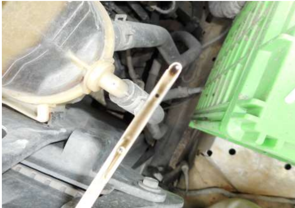
Photo 17 shows the engine oil dip stick of the Police Hilux at the time of my inspection. The engine oil was observed to be of sufficient level and without any visible contamination.
