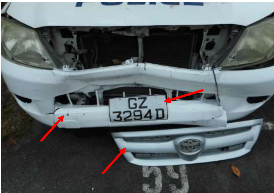
Photo 3 shows a close up view of the Police Hilux's front body at the time of my inspection. The front portion of the Police Hilux was observed to have sustained damage, its front grille, front bumper and number plate (arrowed) as a result of the accident.
