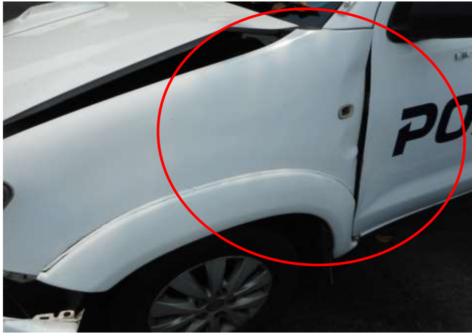
Photo 8 shows a close up view of the Police Hilux's left body at the time of my inspection. The left portion of the Police Hilux was observed to have sustained damage; its left fender (circled) was damaged as a result of the accident.
