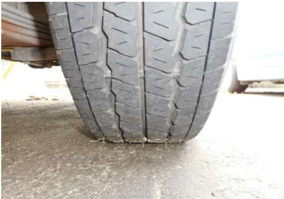
Photo 11 shows the condition of the rear left tyre of the Police Hilux, which was observed to be in serviceable condition with remaining tread depth of approximately 6.4mm. The tyre, which was wrapped around alloy wheel rim, was also observed to be sufficiently inflated for vehicular operation. The 4 tyres of the Police Hilux were wrapped around standard alloy wheel rims.
