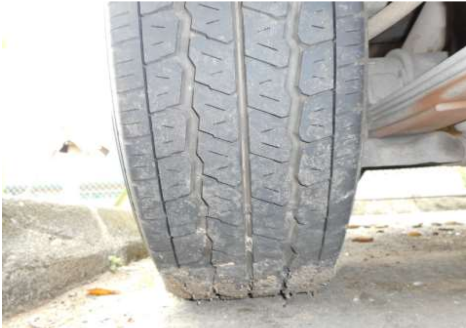
Photo 10 shows the condition of the rear right tyre of the Police Hilux, which was observed to be in serviceable condition with remaining tread depth of approximately 6.5mm. The tyre was also observed to be sufficiently inflated for vehicular operation with no tear, cut or burst mark(s).
