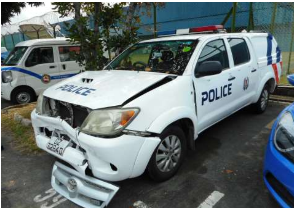
Photo 7 shows a general view of the Police Hilux's left body at the time of my inspection. The left portion of the Police Hilux was observed to have sustained damage; its left fender was damaged as a result of the accident.
