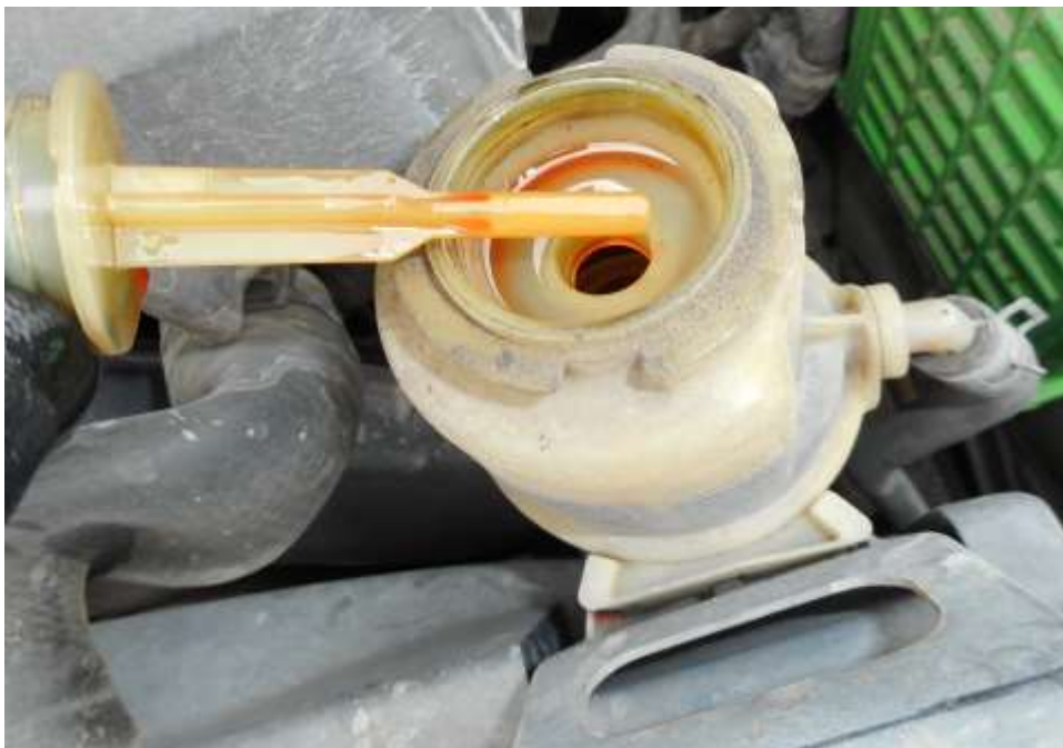
Photo 16 shows checks being carried out to the Power steering fluid of the Police Hilux at the time of my inspection. The steering fluid was observed to be of sufficient level and without any visible contamination.
