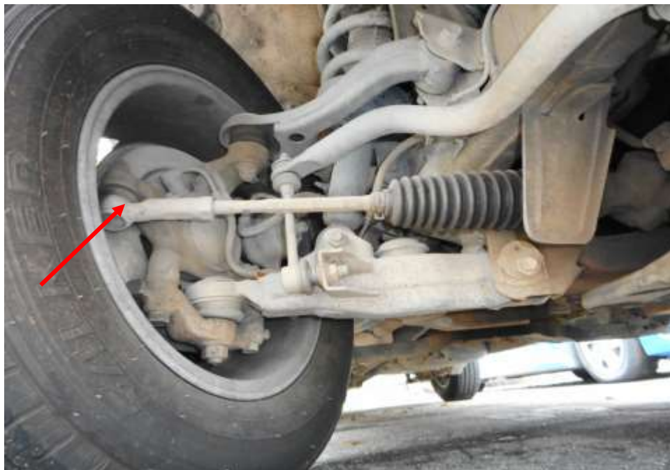
Photo 23 shows the various undercarriage components at the front right wheel of the Police Hilux, in particular the steering tie rod (red arrow). The various steering components were all found to be intact, suggesting that the steering system of the Police Hilux was likely to be in serviceable condition at the material time of accident. There was also no sign of fluid stain observed on the various undercarriage components at the front right wheel of the Police Hilux.
