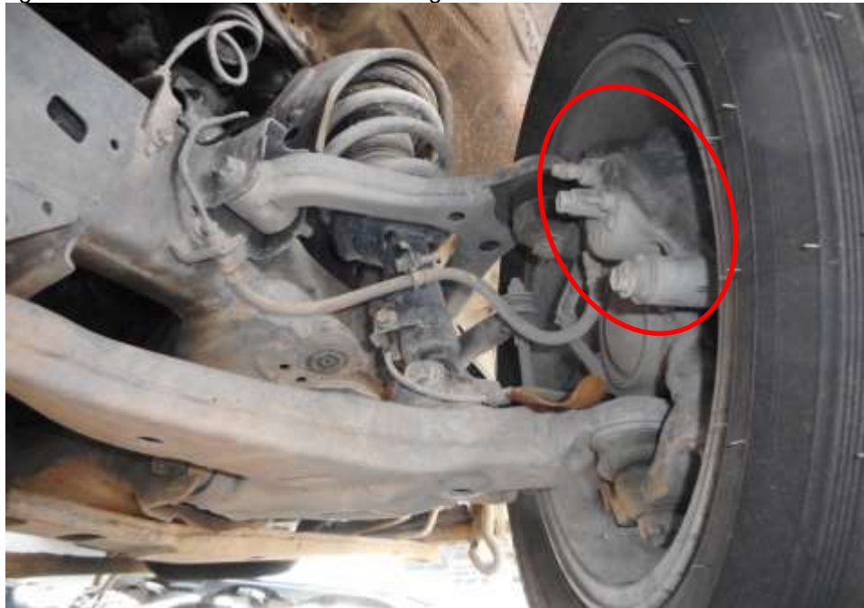
Photo 21 shows the old stain of brake fluids leakage on the front right brake caplier surface (circled) at the time of my inspection of the Police Hilux. Static tests of the Police Hilux's braking system had indicated that there was internal leakage of pressure/vacuum.
