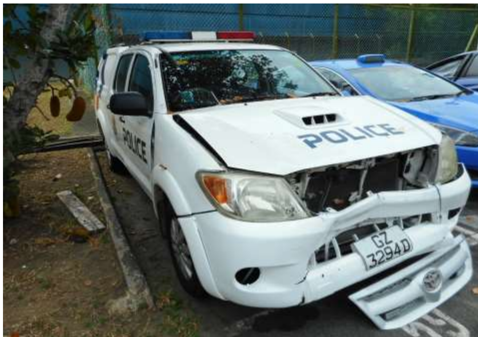
Photo 5 shows a general view of the Police Hilux's right body at the time of my inspection. The right portion of the Police Hilux was observed to have sustained damage; its right fender was damaged as a result of the accident.
