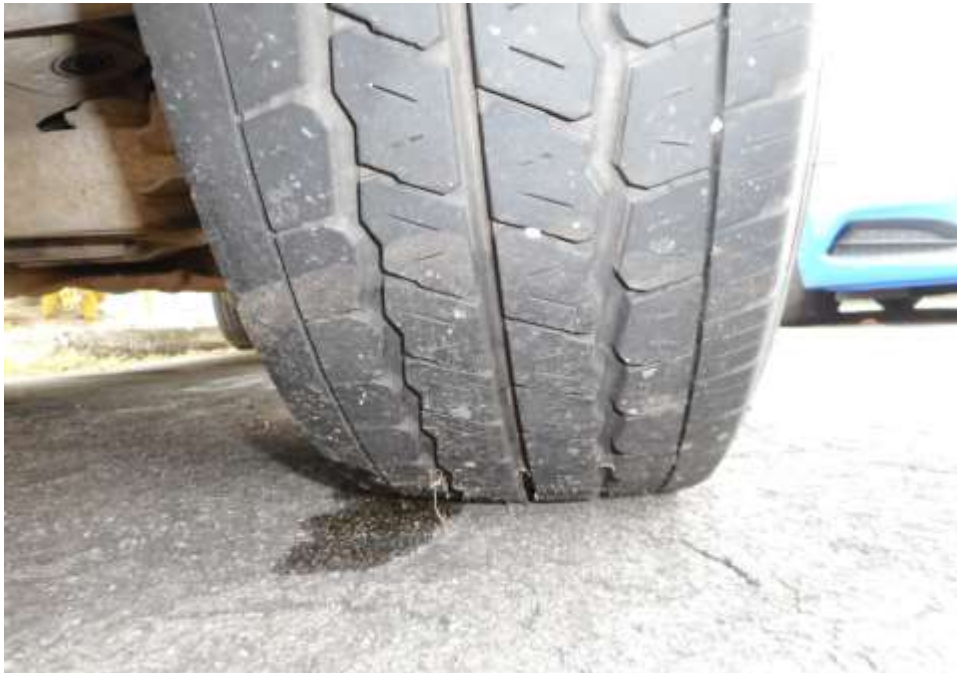
Photo 12 shows the condition of the front left tyre of the Police Hilux, which was observed to be in serviceable condition with remaining tread depth of approximately 6.6mm. There was also no tear, cut or burst mark(s) on the outer and the inner sidewalls as well as across the tread of the Police Hilux's 4 tyres.
