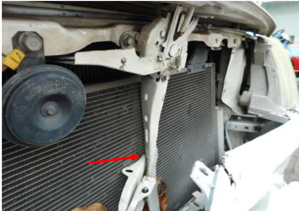
Photo 4 shows a close up view of the Police Hilux's front body at the time of my inspection. The front portion of the Police Hilux was observed to have sustained damage, its front radiator (arrowed) as a result of the accident.
