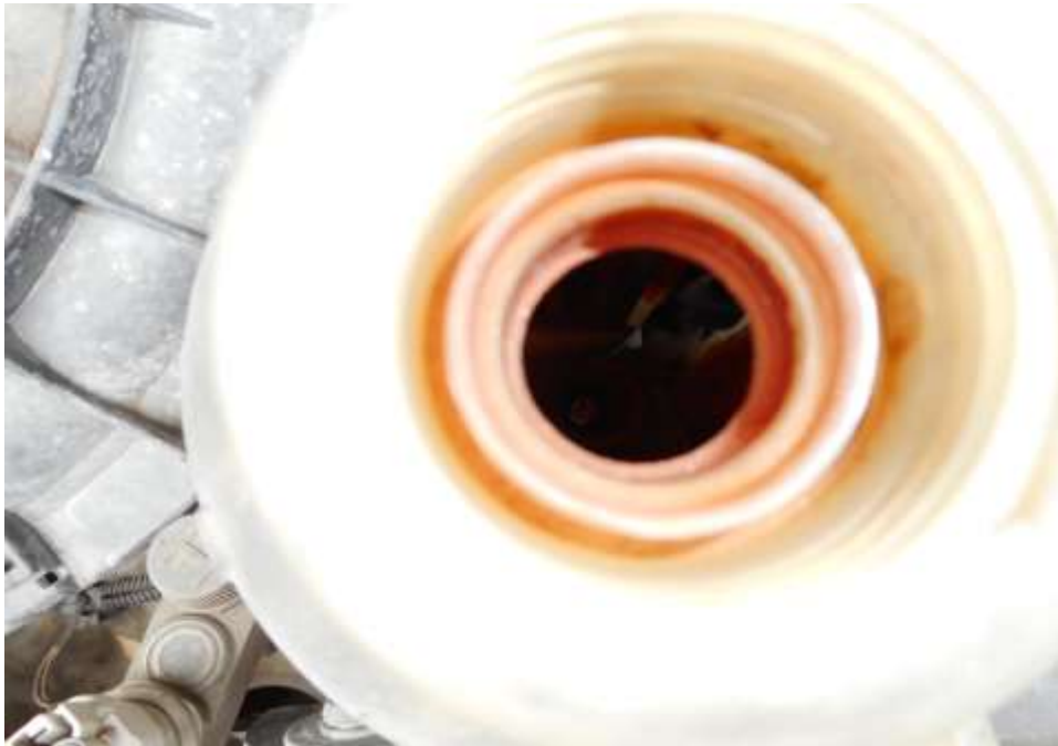
Photo 15 shows checks being carried out to the engine coolant of the Police Hilux at the time of my inspection. The engine coolant was observed to be of insufficient level due to the damage to the front radiator which causes a leakage of coolant fluids.
