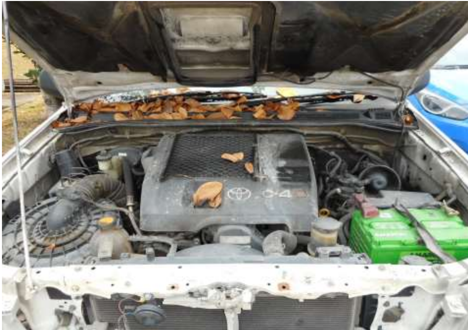
Photo 13 shows a general view of the Police Hilux's engine compartment. The various parts and components inside the engine compartment were unaffected by the accident. There was also no sign(s) or indication(s) of fluid leakage and/or fluid stain within the engine compartment.
