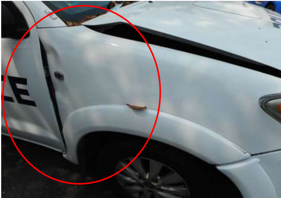
Photo 6 shows a close up view of the Police Hilux's right body at the time of my inspection. The right portion of the Police Hilux was observed to have sustained damage; its right fender (circled) was damaged as a result of the accident.
