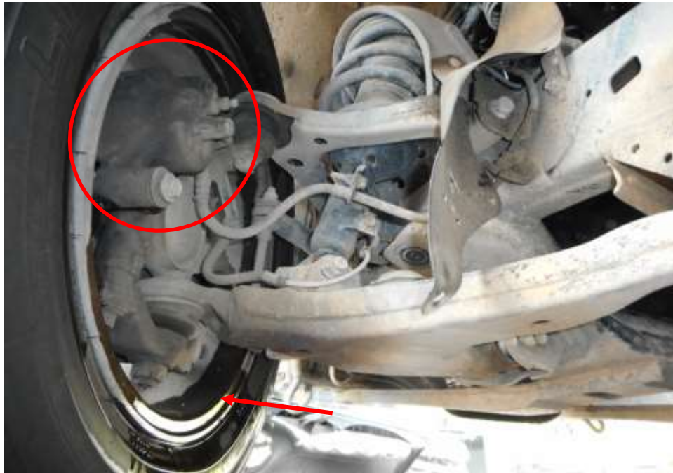
Photo 22 shows the old stain and fresh brake fluids leakage on the front left brake caplier (circled) and rims surface (arrowed) at the time of my inspection of the Police Hilux. Static tests of the Police Hilux's braking system had indicated that there was internal leakage of pressure/vacuum.
