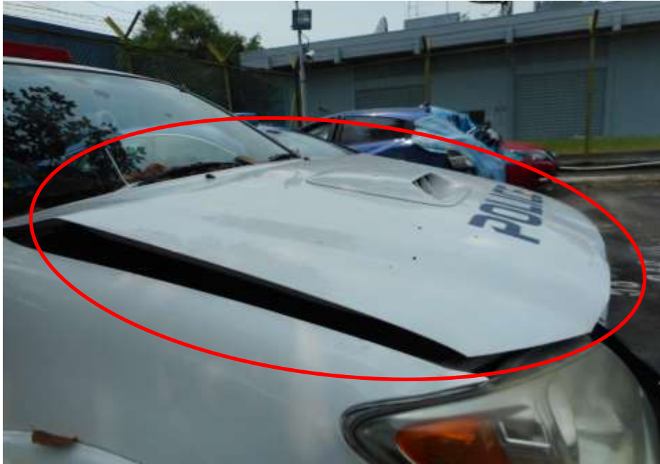
Photo 2 shows the close up view of the Police Hilux's front body at the time of my inspection. The Police Hilux was observed to have sustained damage at its front bonnet (circled) as a result of the accident.
