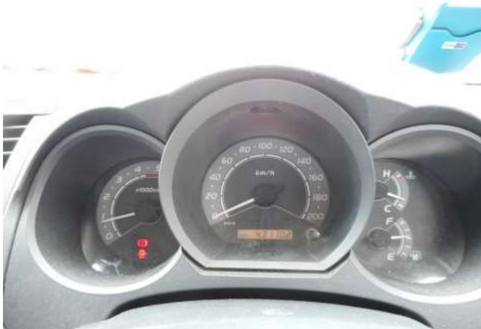
Photo 26 shows no warning lights illuminated on the instrument panel of the Police Hilux after the engine was cranked. This would suggest that there was no abnormality to the various electronic operating systems of the Police Hilux, like the ABS.
