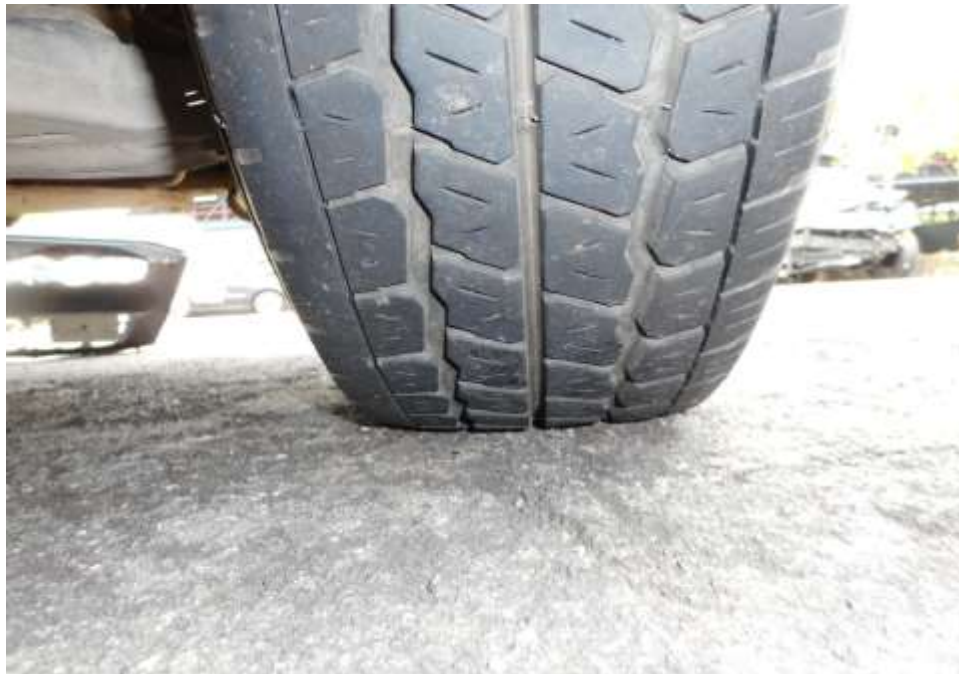
Photo 9 shows the condition of the front right tyre of the Police Hilux, which was observed to be in serviceable condition with remaining tread depth of approximately 7.2mm. The tyre was sufficiently inflated for vehicular operation with no tear, cut or burst mark(s) on the outer and the inner sidewalls as well as across the tread. The 4 tyres of the Police Hilux were wrapped around standard alloy wheel rims without any damage.
