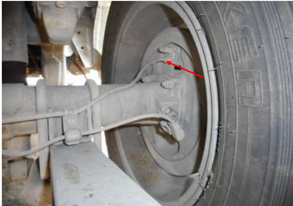
Photo 20 shows the brake hose/pipe (arrowed) of the drum brake at the rear right wheel of the Police Hilux. No leakage of brake fluid was observed.
