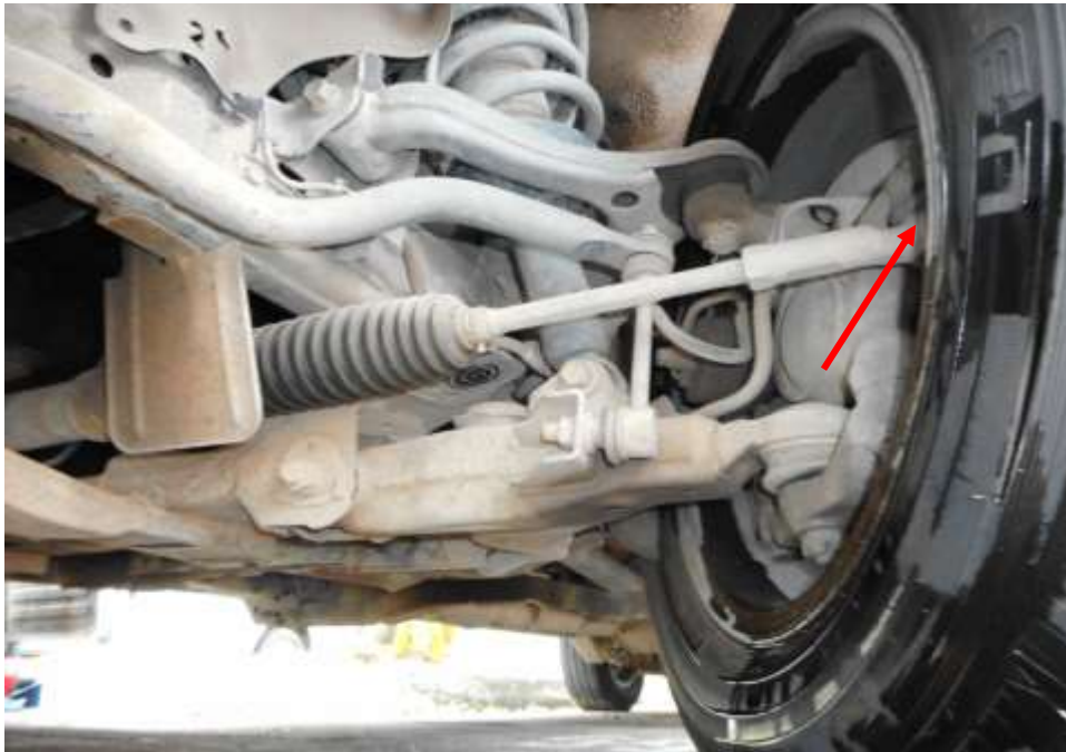
Photo 24 shows the various undercarriage components at the front left wheel of the Police Hilux, which had included the steering tie rod (red arrow). The various undercarriage components of the Police Hilux were all found to be intact without any visible damage.
