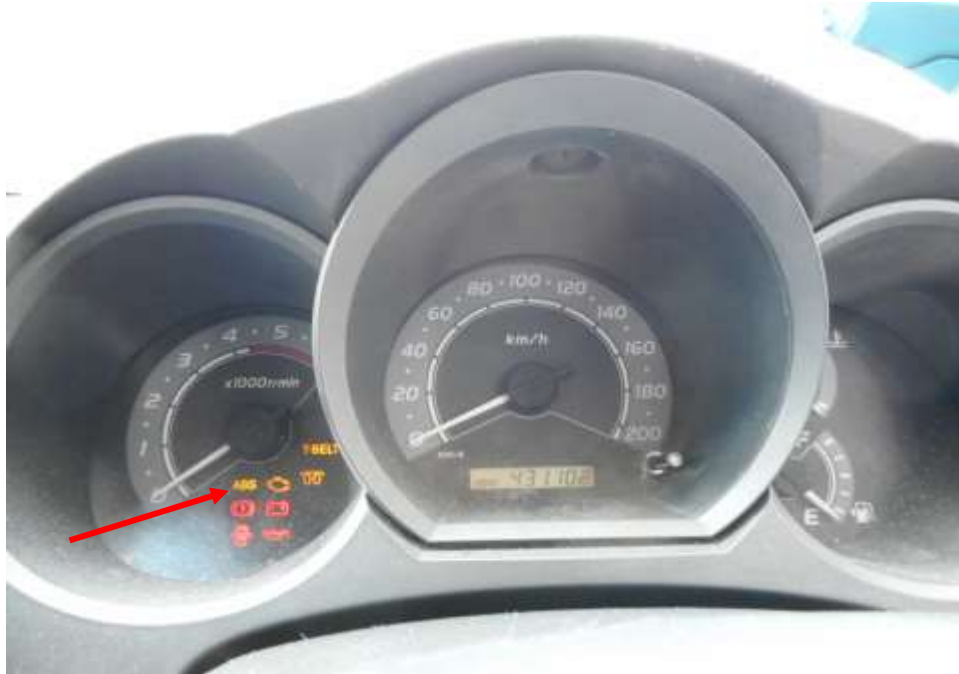
Photo 25 shows the warning light for Anti-Lock Brake System (ABS) appearing on the instrument panel of the Police Hilux during the self-test of its various electronic operating systems when its engine was cranked.
