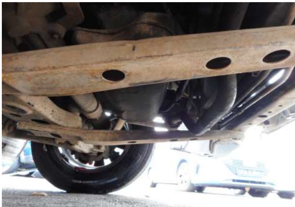
Photo 18 shows the undercarriage of the Police Hilux, at the area where the engine housing and transmission housing are located. I did not find any sign(s) or indication(s) of fluid leak and/or fluid stain(s) on the underside of the Police Hilux.
