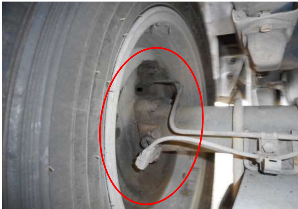
Photo 19 shows the old stain of brake fluids leakage on the rear left drum brake surface (circled) at the time of my inspection of the Police Hilux. Static tests of the Police Hilux's braking system had indicated that there was internal leakage of pressure/vacuum.
