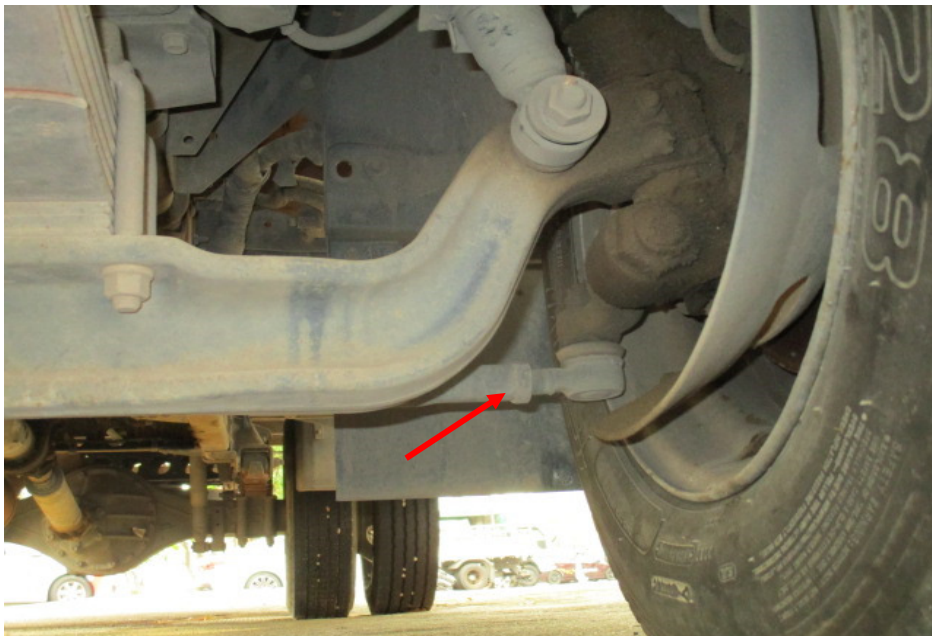
Photo 17 shows the various undercarriage components at the front left wheel of the Motor Lorry, in particular the steering tie rod end (arrowed). The various undercarriage components of the Motor Lorry were all found to be intact without any visible damage. There was also no sign of fluid stain(s) observed on the various undercarriage components.
