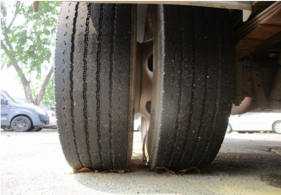
Photo 7 shows the condition of the rear right tyres of the Motor Lorry, which were observed to be in serviceable condition with remaining tread depth of approximately 5mm. There was also no tear, cut or burst mark(s) on the outer and the inner sidewalls as well as across the tread of the 6 tyres that were fitted on the Motor Lorry.
