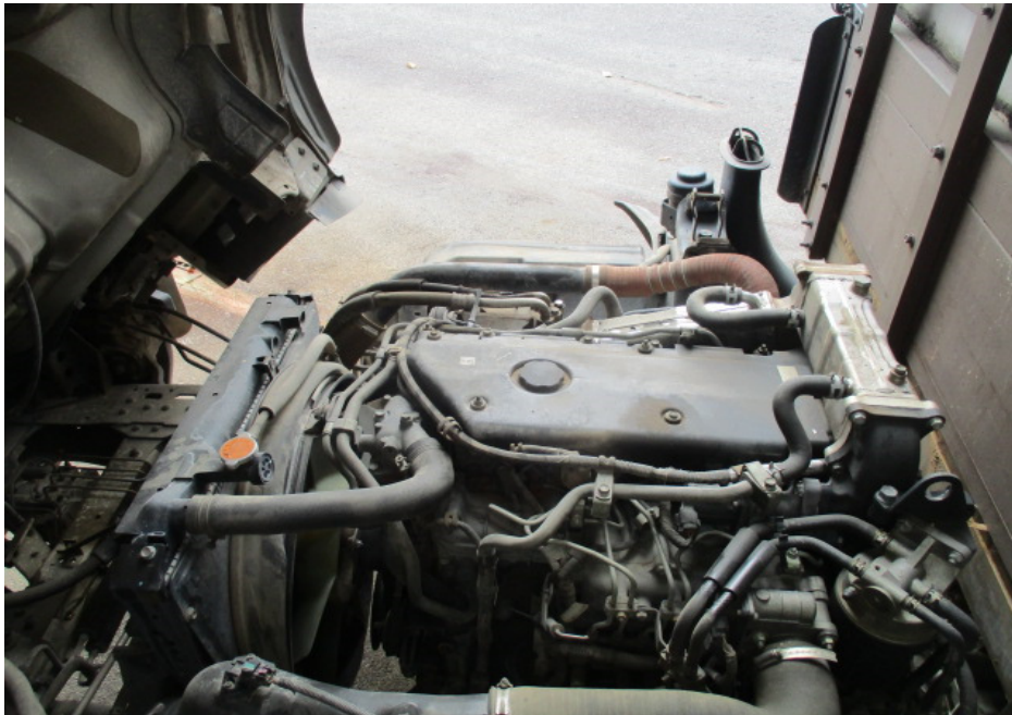
Photo 8 shows a general view of the Motor Lorry's engine compartment, which was accessed by lifting the front cabin of the Motor Lorry. The various parts and components inside the engine compartment were unaffected by the accident. There was also no sign(s) or indication(s) of fresh fluid leakage and/or fluid stain within the engine compartment (photograph shows the engine compartment as viewed from the left front side of the Motor Lorry).
