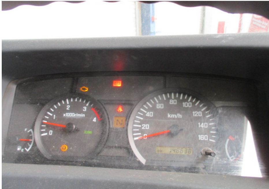
Photo 19 shows the ABS warning light was not illuminated on the instrument panel of the Motor Lorry after the engine was cranked. This would suggest that there was no abnormality to the various electronic operating systems of the Motor Lorry, like the ABS.
