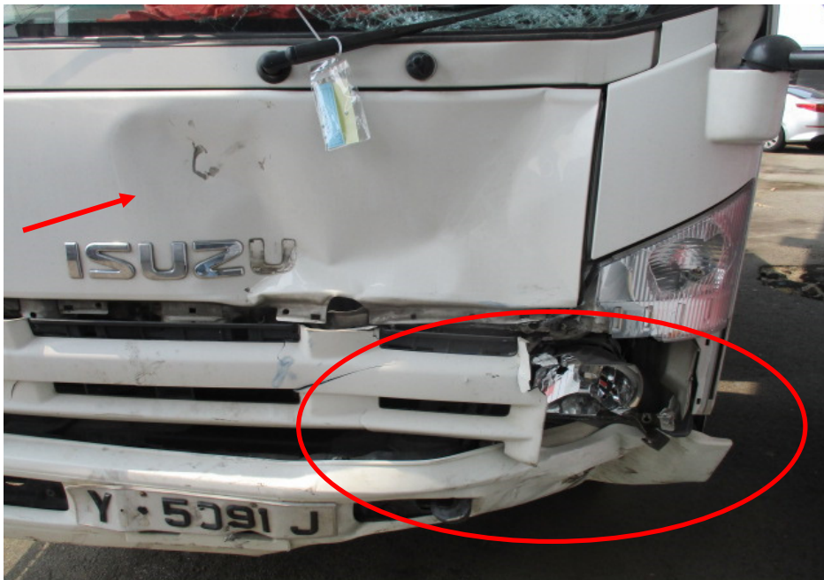
Photo 3 shows a closer view of the deformed front bumper and cracked left headlight (circled) as well as the dented front panel (arrowed) of the Motor Lorry at the time of our inspection.
