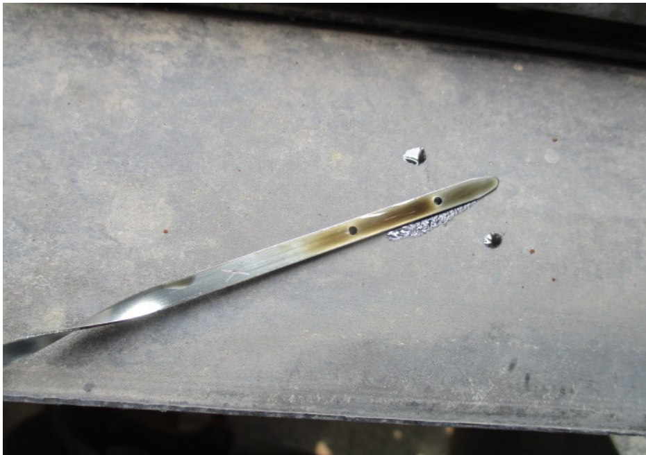
Photo 12 shows the engine dip stick of the Motor Lorry at the time of our inspection. The engine oil was observed to be of sufficient level and without any visible contamination.
