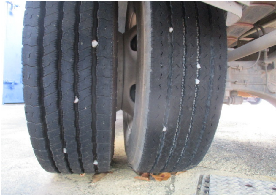
Photo 6 shows the condition of the rear left tyres of the Motor Lorry, which was observed to be in serviceable condition with remaining tread depth of approximately 11mm. The tyres, which were wrapped around standard alloy wheel rim, were also observed to be sufficiently inflated for vehicular operation. There was also no damage found on all 6 alloy wheel rims of the Motor Lorry.
