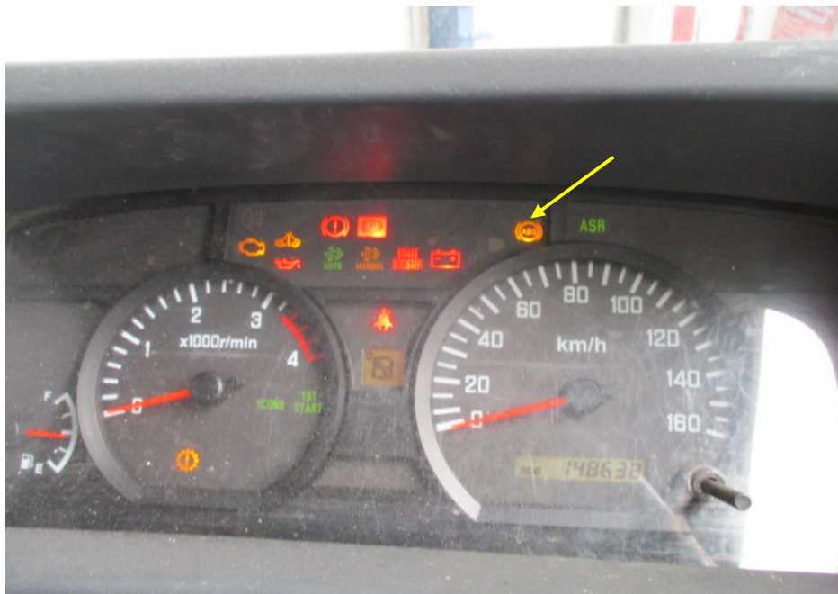
Photo 18 shows the warning lights for the various electronic operating systems of the Motor Lorry appearing on its instrument panel during the self-test when the engine is cranked, in particular the ABS light (arrowed).
