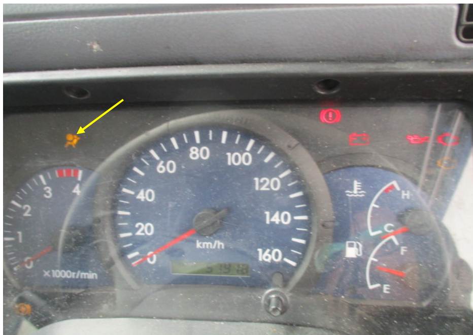
Photo 18 shows the warning lights for the various electronic operating systems of the Motor Lorry appearing on its instrument panel during the self-test when the engine is cranked, in particular the SRS light (arrowed).
