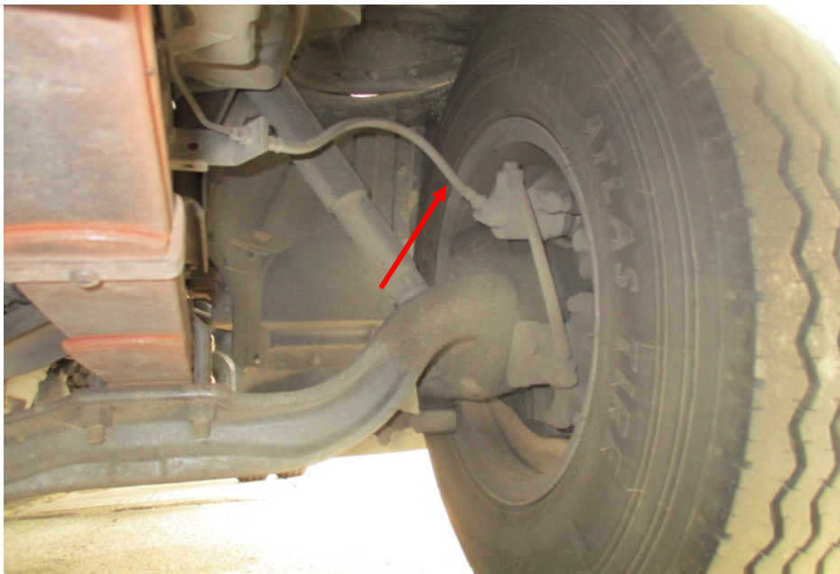
Photo 13 shows the brake pipe (arrowed) at the rear right wheel of the Motor Lorry. We did not observe any leakage of brake fluid at the time of our inspection of the Motor Lorry. Our static tests of the Motor Lorry's braking system, along with our visual examination of the various mechanical components in the braking system, had indicated that there was no internal leakage of pressure/vacuum. Hence the braking system of the Motor Lorry was likely to be in serviceable condition at the material time of accident.
