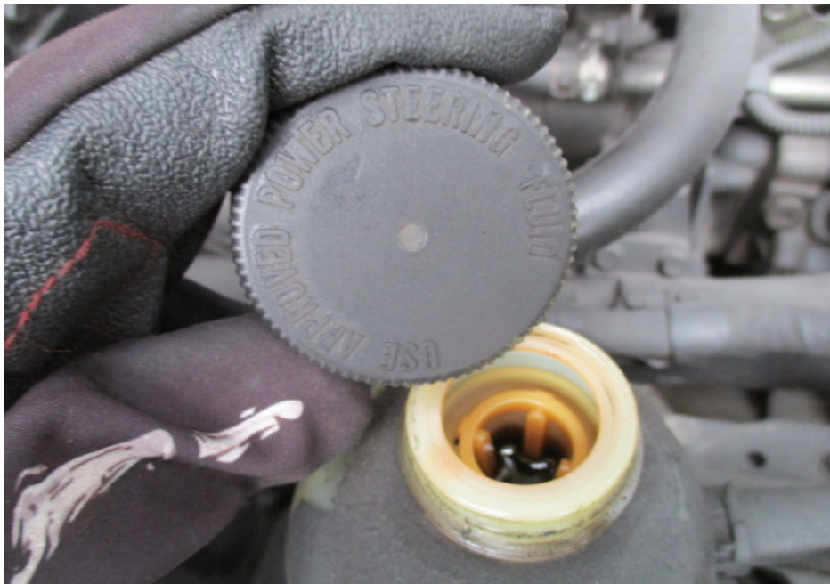
Photo 10 shows the power steering fluid reservoir of the Motor Lorry at the time of our inspection. The power steering fluid was observed to be of sufficient level and without any visible contamination.
