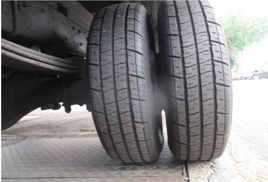
Photo 6 shows the condition of the rear left tyres of the Motor Lorry, which was observed to be in serviceable condition with remaining tread depth of approximately 5mm and 6mm. The tyres, which were wrapped around standard alloy wheel rim, were also observed to be sufficiently inflated for vehicular operation. There was also no damage found on all 6 alloy wheel rims of the Motor Lorry.
