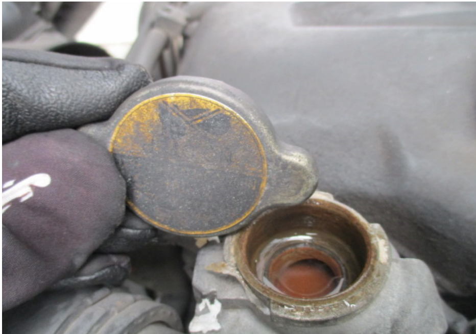
Photo 9 shows the engine coolant of the Motor Lorry at the time of our inspection. The engine coolant was observed to be of sufficient level and without any visible contamination.
