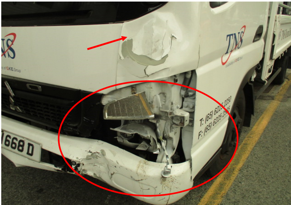
Photo 3 shows a closer view of the deformed front bumper and cracked left headlight (circled) as well as the dented front left panel (arrowed) of the Motor Lorry at the time of our inspection.
