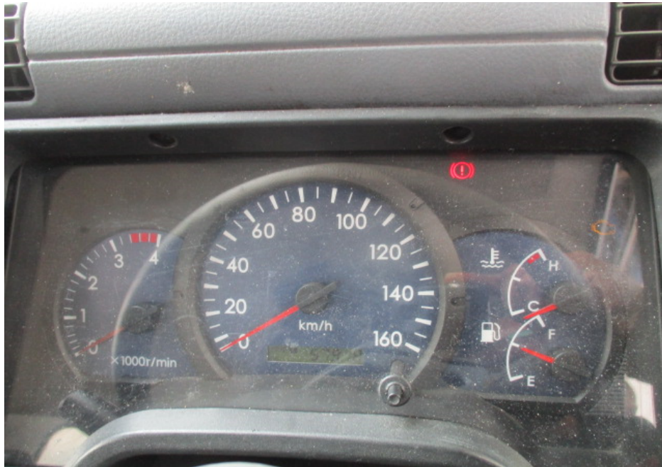
Photo 19 shows the SRS warning light was not illuminated on the instrument panel of the Motor Lorry after the engine was cranked. This would suggest that there was no abnormality to the various electronic operating systems of the Motor Lorry, like the SRS.
