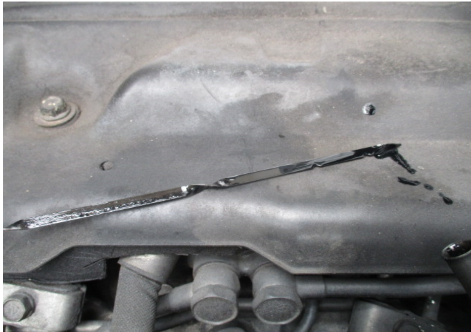
Photo 11 shows the engine dip stick of the Motor Lorry at the time of our inspection. The engine oil was observed to be of sufficient level and without any visible contamination.
