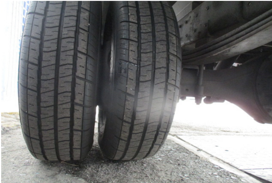
Photo 7 shows the condition of the rear right tyres of the Motor Lorry, which were observed to be in serviceable condition with remaining tread depth of approximately 5mm and 6mm. There was also no tear, cut or burst mark(s) on the outer and the inner sidewalls as well as across the tread of the 6 tyres that were fitted on the Motor Lorry.
