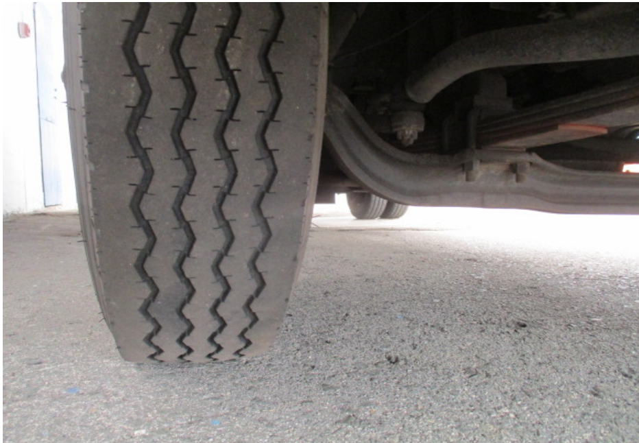
Photo 5 shows the condition of the front right tyre of the Motor Lorry, which was observed to be in serviceable condition with remaining tread depth of approximately 5mm. The tyre, which was wrapped around standard alloy wheel rim, was also observed to be sufficiently inflated for vehicular operation.
