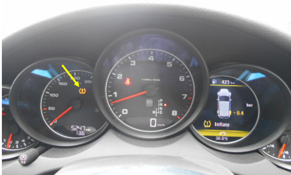
Photo 7 shows the respective warning lights no longer illuminated except for the Tyre Pressure Monitor (TPM) warning light (arrowed), which remained lighted to alert the vehicle operator that air pressure of the rear right tyre was below the pre-set limit. The self-test had indicated that there is no fault detected to the ABS, SRS, TPM and TCS systems of the Motor Car. These electronic systems were hence found to be in working condition at the time of my inspection.
