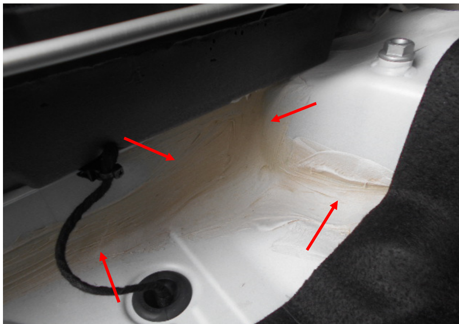
Photo 17 shows the rear floor board of the Motor Car. The original factory sealant (arrowed) at the joints along the chassis/structural body was untouched. In general, I had found no work done on the structure/chassis body of the Motor Car and that the structure/chassis body was originally fitted.
