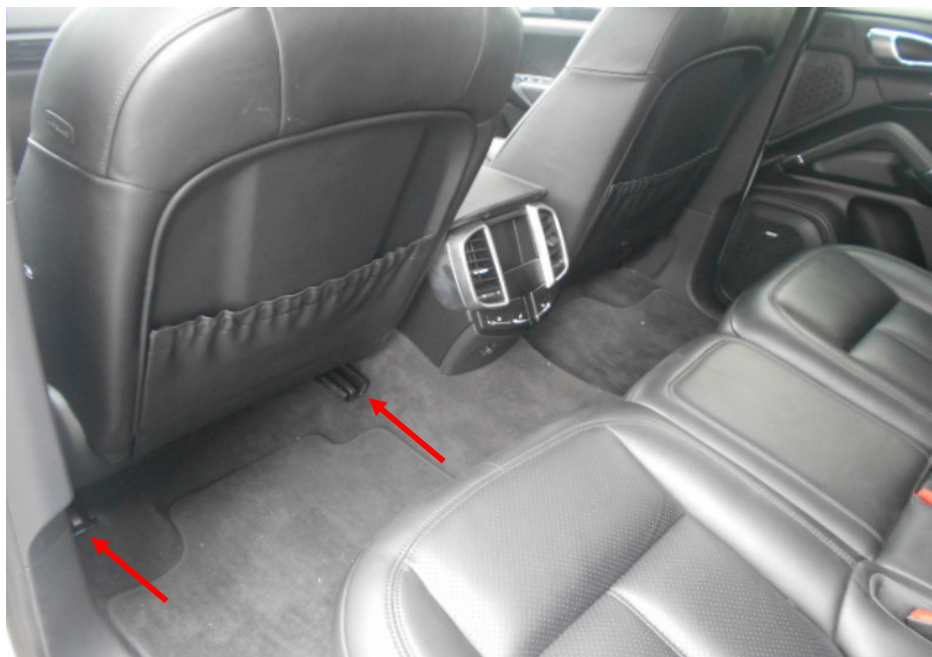
Photo 5 shows the seats of the Motor Car, which were secured via seat rails (arrowed) to the floor board. All the seats of the Motor Car were fitted with a retractable seat belt reel and pre-tensioner. The seat belts were also able to be fastened to the pretension that were fitted on the side of each individual seat.
