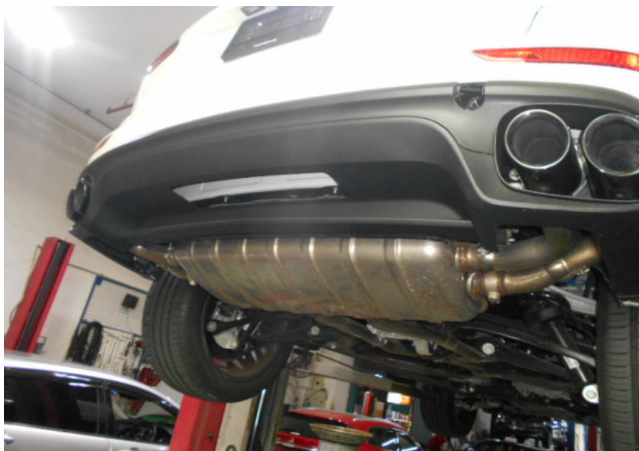
Photo 12 shows the Motor Car's rear exhaust muffler. My examination of the Motor Car's exhaust system revealed no sign(s) or indication(s) of any cut or weld marks along its exhaust pipes and on its rear mufflers.
