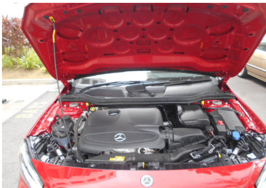
Photo 4 shows a general view of the engine compartment of the Motor Car at the time of my inspection. The various parts and components inside the engine compartment were all observed to be intact and properly fitted. There was also no sign(s) or indication(s) of fluid leak and/or fluid stain found within the engine compartment.
