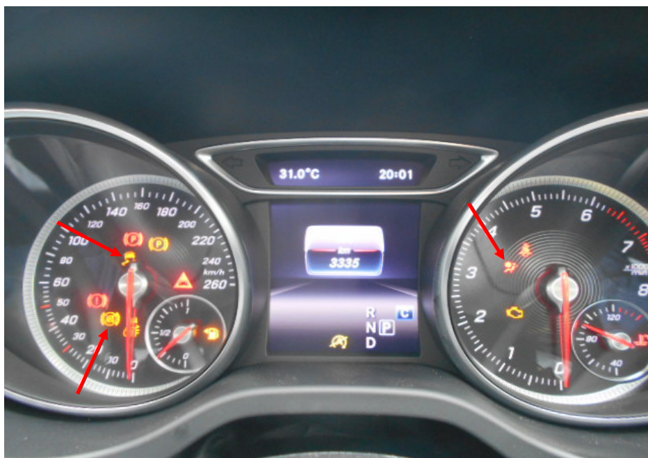
Photo 6 shows the warning lights for the various electronic safety features appearing on the instrument panel of the Motor Car during its self-test when the engine is cranked, in particular the ABS, SRS and TCS lights (arrowed).
