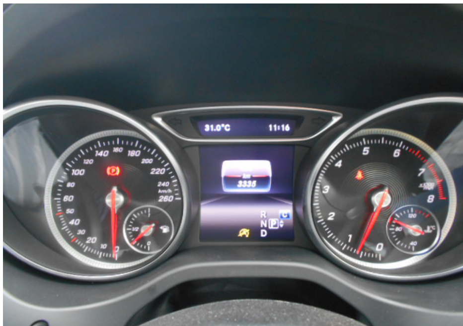
Photo 7 shows the respective warning lights no longer illuminated, indicating that there is no fault detected to the ABS, SRS and TCS systems of the Motor Car during the self-test. These electronic systems were hence in working condition at the time of my inspection.
