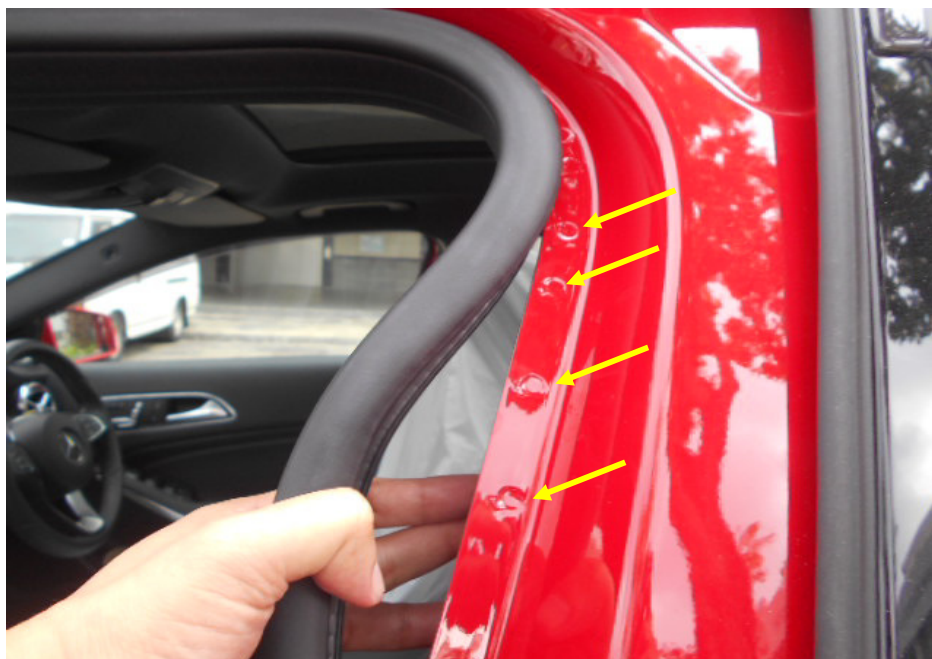
Photo 17 shows the left side "B" pillar of the Motor Car. I did not find any weld marks other than original spot weld marks (arrowed) on the body panels of the Motor Car, indicating that there was no re-welding works carried out; and that the body panels of the Motor Car were originally fitted.
