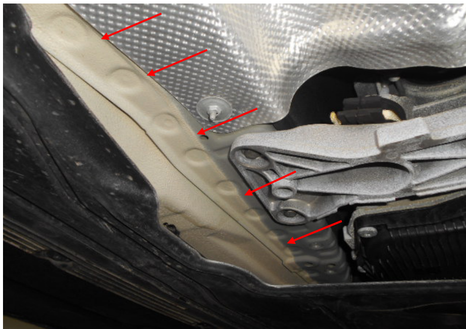
Photo 15 shows the chassis/structural body at the left centre underside of the Motor Car. The original factory sealant (arrowed) at the joints along the chassis/structural body was untouched, indicating no work was done on the chassis/structural body of the Motor Car and that the chassis/structural body was originally fitted.
