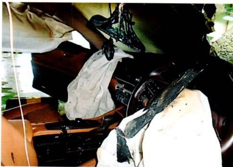
Photo 4 shows the interior compartment of the Insured Vehicle, which was observed to be partially burnt at the front area. The front dashboard and roof upholstery were amongst the parts that were found to have been burnt and/or melted as a result of the fire. The driver's airbag, front left passenger airbag and curtain airbag were also observed to have been activated.
