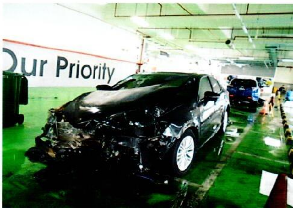
Photo 2 shows a general view of the front left portion of the Insured Vehicle at the time of my inspection. The fire damage to the Insured Vehicle was confined to its frontal portion. Its front bonnet and front left headlamp were amongst the body parts that were found to have been affected as a result of the fire. Apart for the fire damage, the Insured Vehicle was also observed to have sustained impact damage at its frontal portion.
