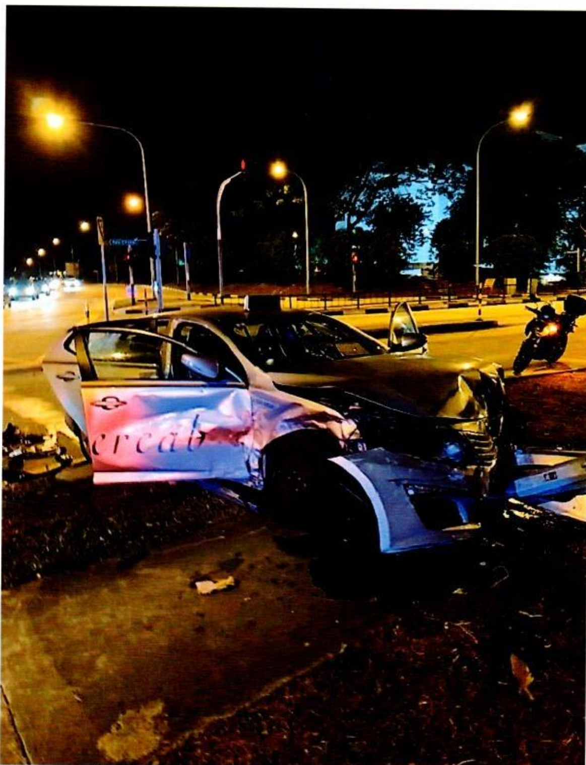
Photo 7 shows the Premier motor taxi SHB 8588M at its stopped position. Its frontal portion had collided into a lamppost after the accident with the Insured Vehicle. Leaked fluid from the motor taxi could also be seen on the ground beneath the frontal portion of the motor taxi. Overall, the extent of damage to the Premier motor taxi SHB 8588M was relatively severe with damages at its frontal portion and its right side.
