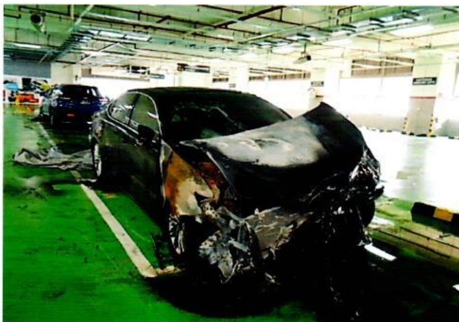
Photo 1 shows a general view of the front right portion of the Insured Vehicle at the time of my inspection. The fire damage to the Insured Vehicle was confined to its frontal portion. Its front bonnet, front bumper, front right fender, front right headlamp and front windscreen were amongst the body parts that were found to have been affected as a result of the fire. Apart for the fire damage, the Insured Vehicle was also observed to have sustained impact damage at its frontal portion. The impact damage pattern suggests that the direction of impact was from the front left to front right of the Insured Vehicle.
