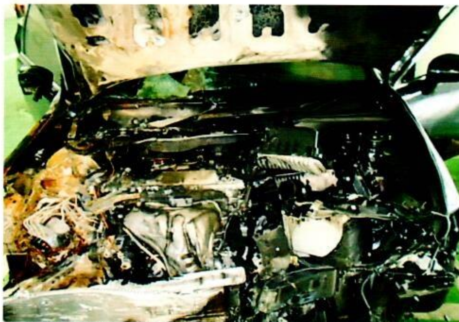
Photo 3 shows the engine compartment of the Insured Vehicle at the time of my inspection. The engine compartment of the Insured Vehicle was observed to be burnt. The parts at the right side of the engine compartment had sustained more severe fire damage as compared to the parts at the left side.
