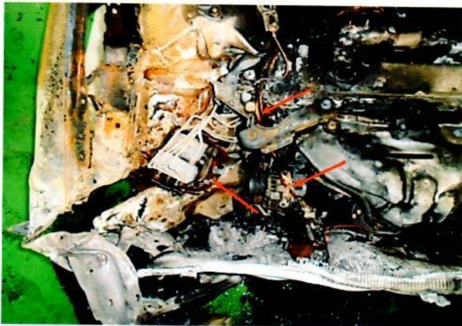
Photo 9 shows the wirings around the front right area of the engine compartment, which was where the fire to the Insured Vehicle had originated. Several stretches of wirings (arrowed) were observed to be completely burned to its bare copper state. The bright reddish colour of the copper wires suggest that the wirings were exposed to high heat. Such condition normally indicates internal heating of copper wires, which is a sign of an electrical short circuit occurring.
