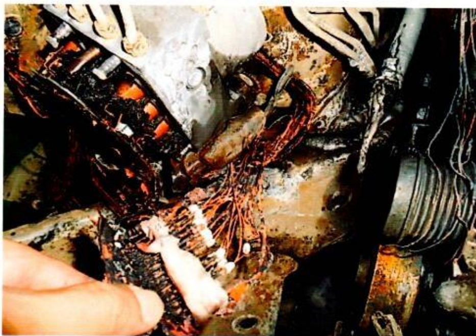
Photo 11 shows the wiring harness for the ABS control module of the Insured Vehicle. The wirings were observed to be burnt to its bare copper state, indicating internal heating of copper wires, which is a sign of an electrical short circuit occurring. In general, the condition of the wirings seen at the area where the fire had originated suggest that the cause of fire to the Insured Vehicle was due to electrical in nature.
