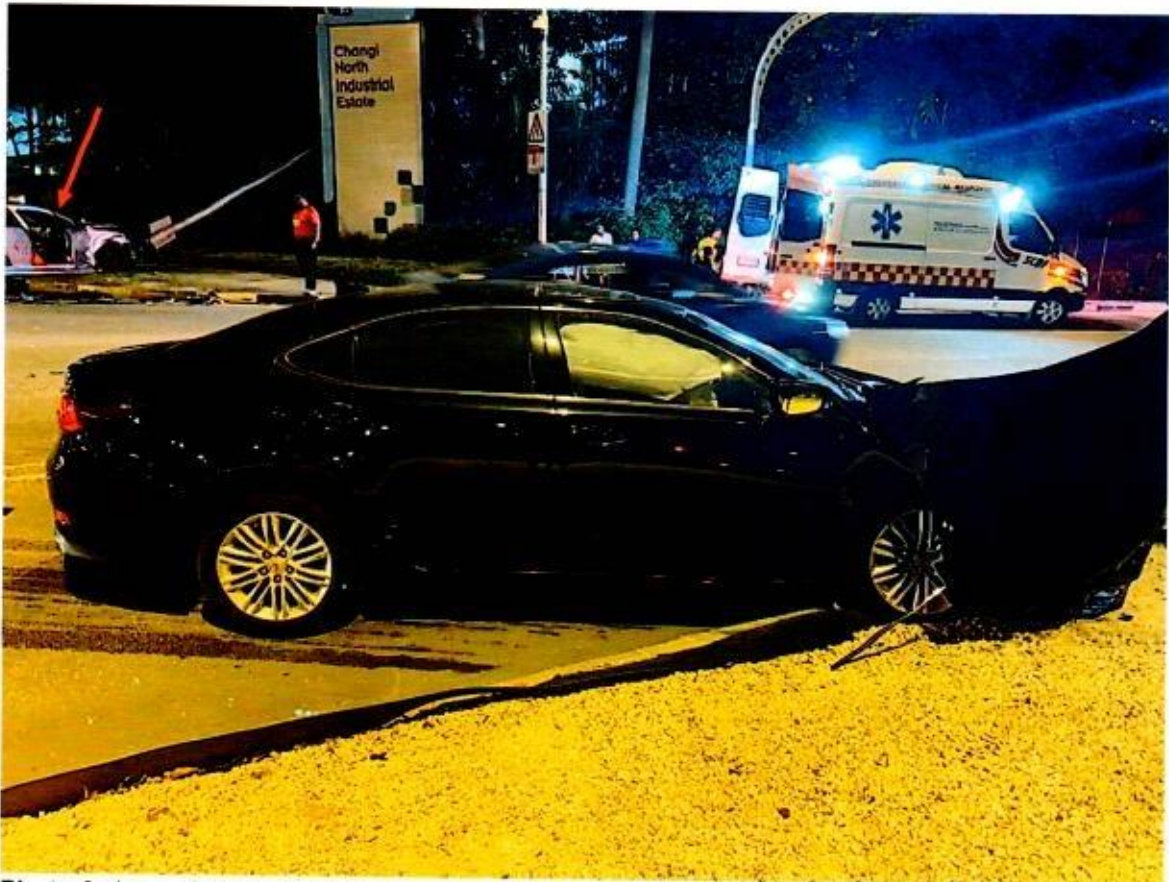
Photo 6 shows the Insured Vehicle stopped on the extreme right lane of Upper Changi Road East in the direction of Singapore Expo. The front bonnet was observed to be partially dislodged and its front right wheel mounted the divider road kerb. There was no damage of fire nature seen on the Insured Vehicle at the accident scene. The Premier motor taxi SHB 8588M (arrowed), on the other hand, had stopped almost fully mounting the grass verge and pedestrian walkway at the slip road of Upper Changi Road North onto Upper Changi Road East. Its frontal portion had also collided into a lamppost at the grass verge.
