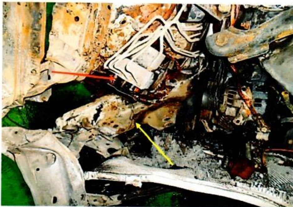
Photo 12 shows the front right chassis (yellow arrow) of the Insured Vehicle badly bent. This was a result of the collision with the Premier motor taxi SHB 8588M. The ABS control module (red arrow) was also shifted towards the right as a result of the collision. This could have caused slight instability to the current/voltage along the wiring harness of the ABS control module, ultimately leading to the fire a few hours after the accident.
