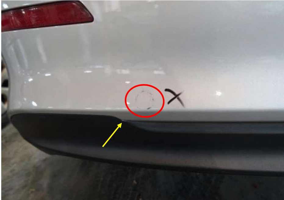
Photo 3 shows a close up view of the paint graze marks (arrowed) as well as circular blackish marks (circled) on the left bottom portion of the Taxi's rear bumper.
