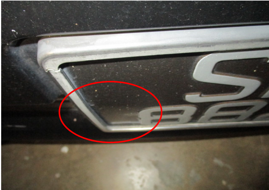
Photo 12 shows a close up view of the right lower portion of the Nissan's front number plate which was observed to be bent inwards (circled)
