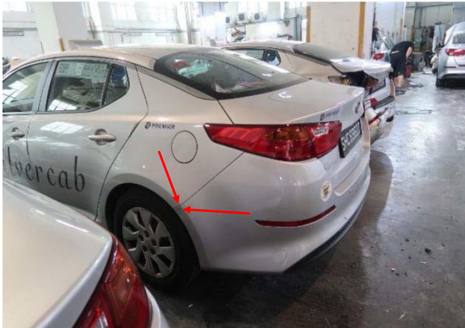
Photo 7 shows a close up view of the left corner edge of the rear bumper of the Taxi. We observed that there was no misalignment at the corner edges (red arrows).
