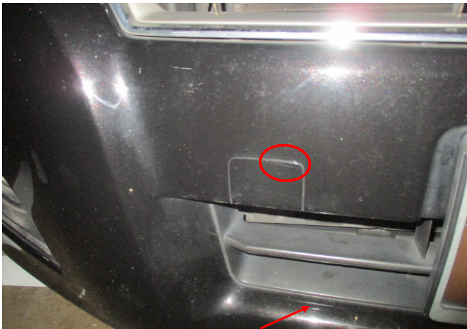
Photo 9 shows the white graze marks on the right front tow cover (circled) and below the front bumper grille (arrowed) of the Nissan.
