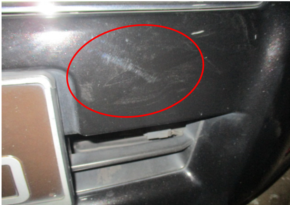
Photo 10 shows a close up view of the scuff marks on the left portion of the Nissan's front bumper (circled).
