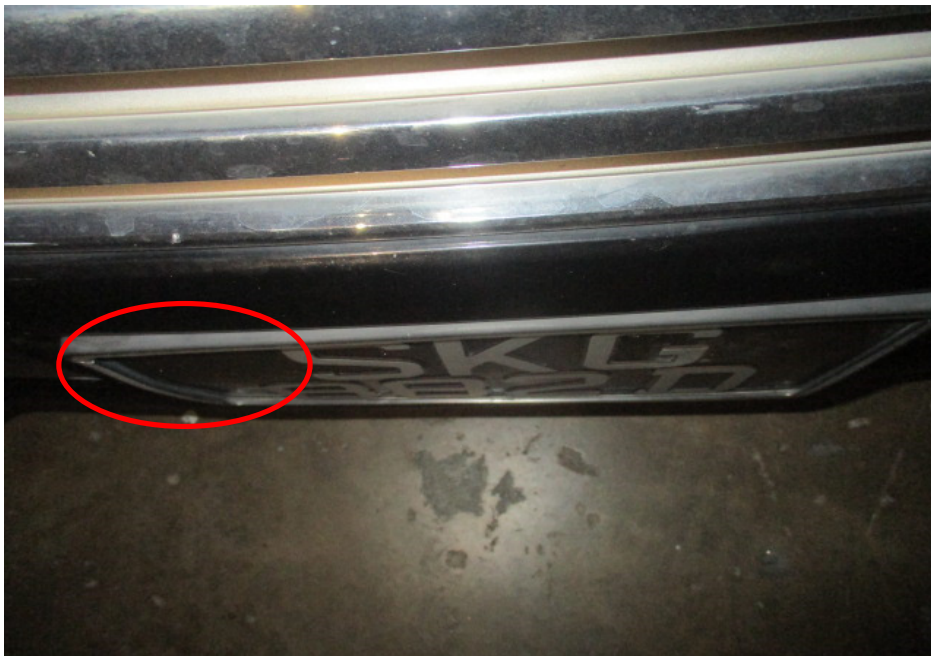
Photo 11 shows upon closer examination of the front number plate of the Nissan, we observed that the right lower portion was bent inwards (circled).
