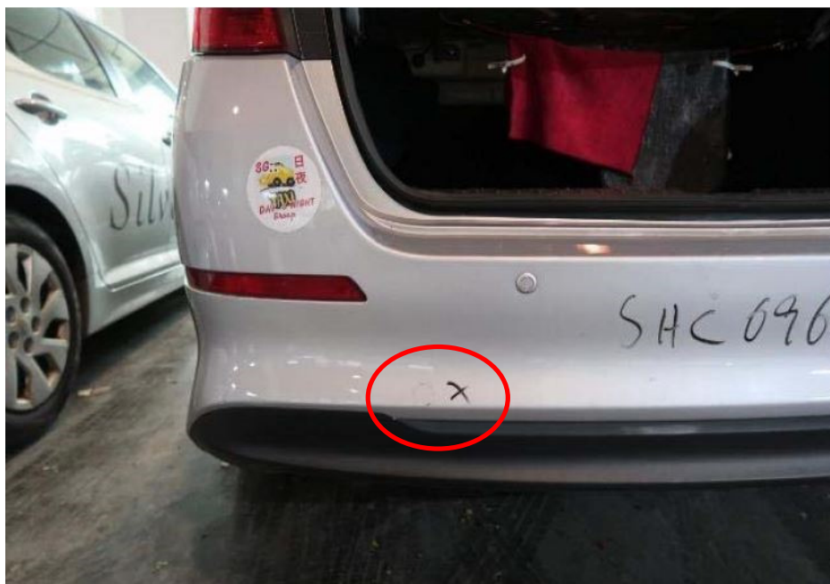
Photo 2 shows a closer view of the left bottom portion of the Taxi's rear bumper. We observed paint graze marks as well as circular blackish marks on the left bottom portion of the Taxi's rear bumper (circled).
