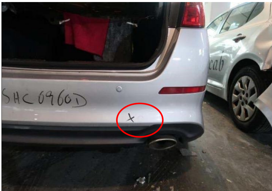
Photo 4 shows a closer view of the right bottom portion of the Taxi's rear bumper. We observed paint graze marks as well as circular blackish marks on the right bottom portion of the Taxi's rear bumper (circled).
