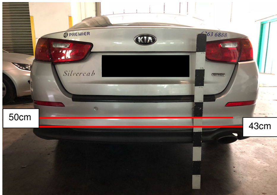
Photo 15 shows the height measurement being conducted on the rear portion of the Taxi (using a similar make and model). The height range of the circular blackish marks on the bottom portion of the rear bumper was measured to be approximately between 43cm and 50cm above ground level.
