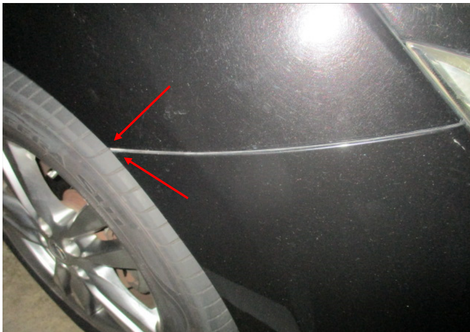
Photo 13 shows a close up view of the right corner edge of the front bumper of the Nissan. We observed that there was no misalignment at the corner edges (red arrows).
