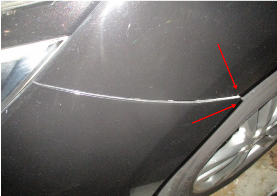
Photo 14 shows a close up view of the left corner edge of the front bumper of the Nissan. We observed that there was no misalignment at the corner edges (red arrows).
