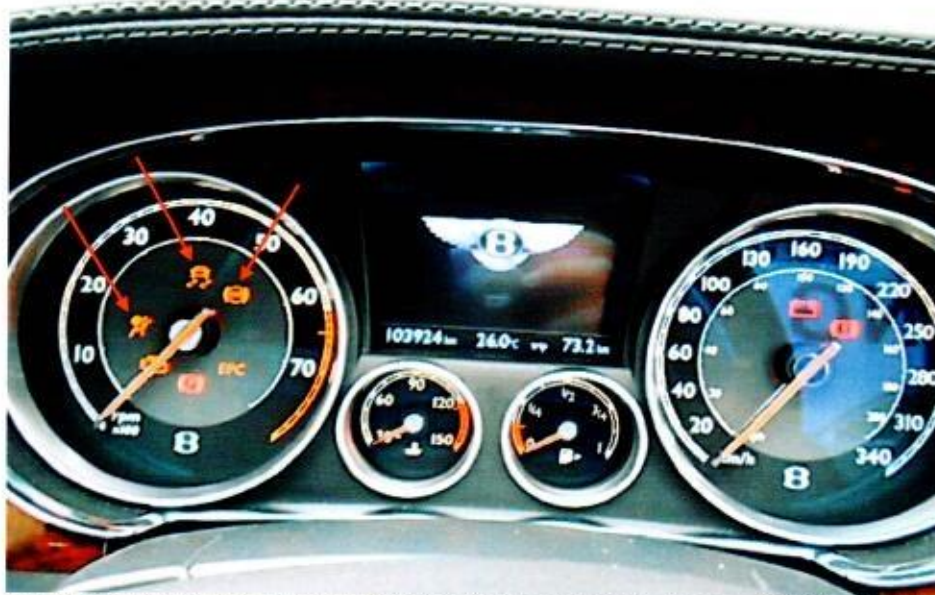
Photo 10 shows the warning light for Anti-Lock Brake System (ABS), Traction Control (TC) and Supplemental Restraint System (SRS) appearing on the instrument panel of the Insured Vehicle during the self-test of its various electronic operating systems when its engine was cranked.
