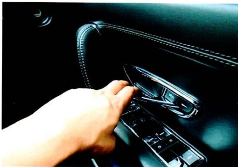
Photo 14 shows the inner handle of the Insured Vehicle's front right door. Whilst seated inside the Insured Vehicle, the front right door could only be opened by manually pulling the inner handle and pushing the front right door outwards. Exerting some force by leaning onto the front right door without pulling the inner handle will not open the front right door. I had found no issue/fault with the condition of the Insured Vehicle's front right door that could have suggested malfunction of the front right door.
