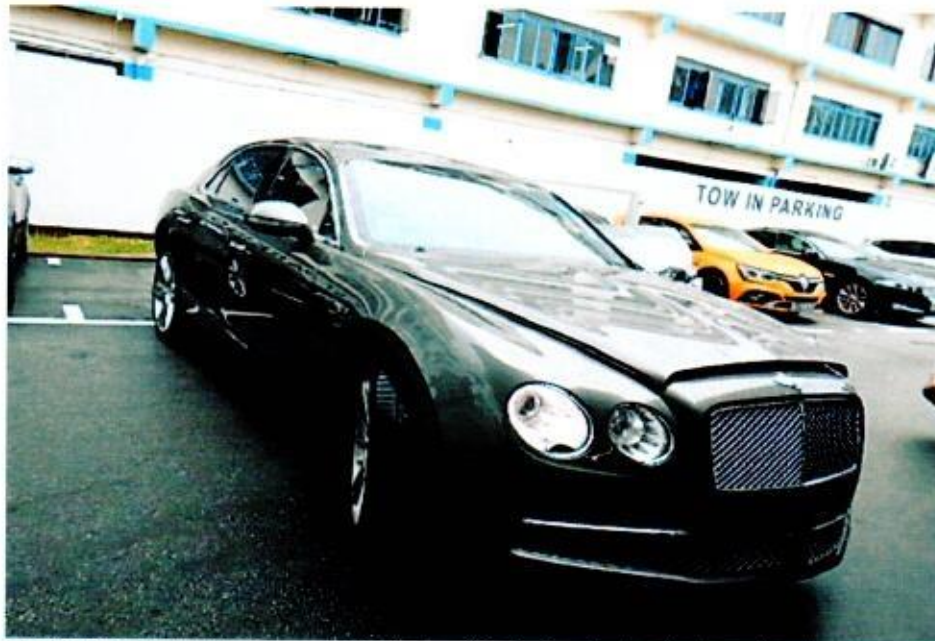
Photo 12 shows the Insured Vehicle, with its front wheels turned to its full right, after it was driven forward from its original position. As part of my tests on the braking system and steering system of the Insured Vehicle, I had driven the Insured Vehicle forward and stopped, thereafter reverse and stopped. In general, I had found the braking system and steering system to be operating normally. The Insured Vehicle was able to stop effectively, and the steering wheel was able to turn without any abnormal free play and/or other resistance. The front wheels were able to turn in the direction that the steering wheel was turned.
