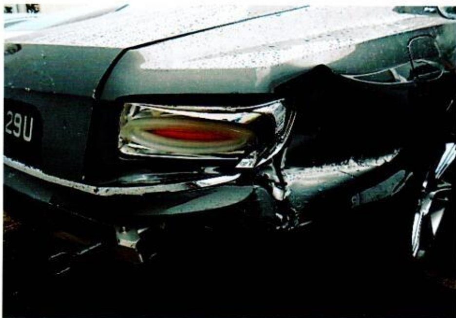
Photo 5 shows the damage at the right rear body of the Insured Vehicle. Its rear bumper, rear bumper reinforcement, rear bootlid, rear right taillamp and rear right fender were amongst the body parts that were damaged as a result of the accident.
