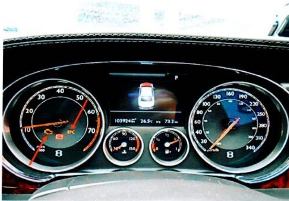
Photo 11 shows the engine check light and EPC light still illuminated after the self-test. This indicates a fault to either one or more electric operating system of the Insured Vehicle. The illumination of the engine check light accompanies the illumination of the EPC light. The ABS, TC and SRS lights were however no longer illuminated indicating that these electronic operating systems were in working condition and without abnormality.
