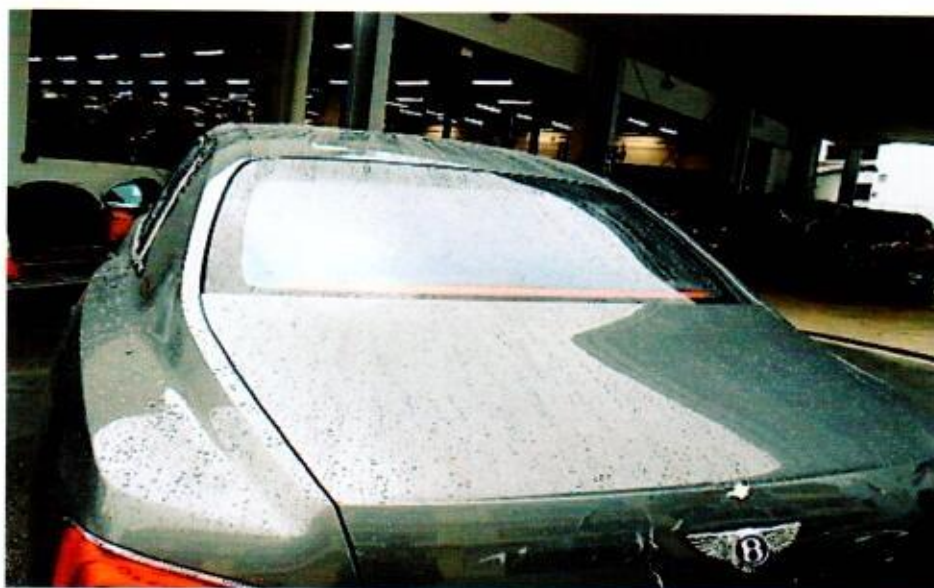
Photo 17 shows a closer view of the Insured Vehicle's third brake light, which lights up when the brake pedal was depressed. The third brake light covers almost the entire width at the bottom part of the rear windscreen.
