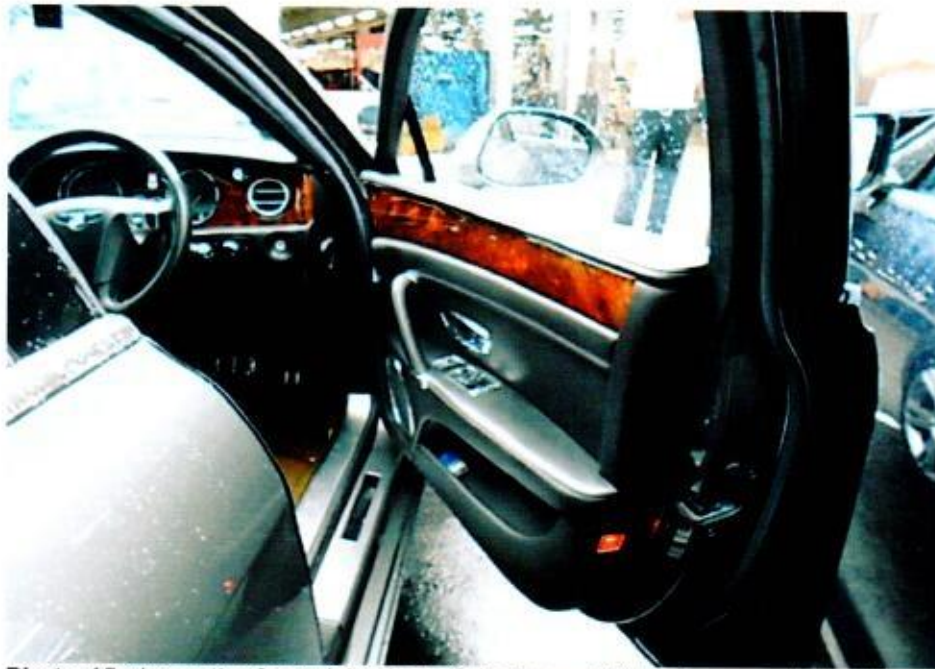
Photo 15 shows the front right door of the Insured Vehicle opened. The hinges were able to securely hold the front right door open. Generally, I did not find any loose swinging of the front right door during my checks and tests.
