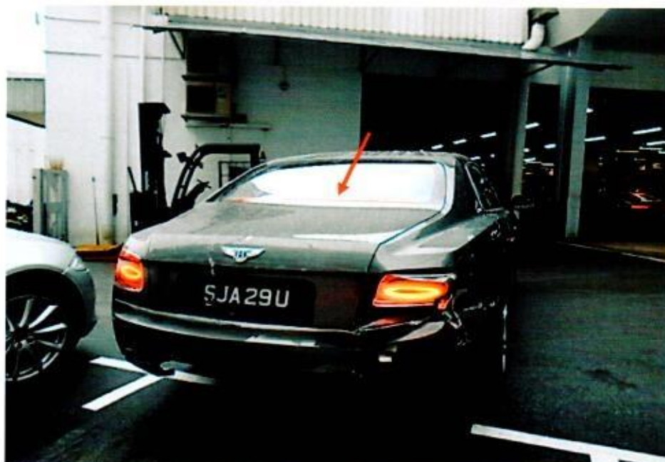
Photo 16 shows the brake light at the rear left taillamp and the rear right taillamp of the Insured Vehicle lighted up together with the third brake light (arrowed) when the brake pedal was depressed. From my observations, it can be ascertained that the brake lights of the Insured Vehicle were in working condition.
