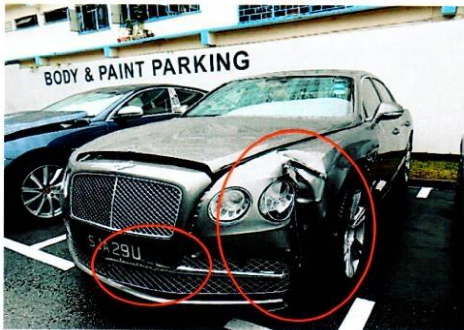
Photo 2 shows a general view of the damage (circled) at the left front body of the Insured Vehicle. The front bumper, front left headlamp, front bumper lower grille and front left fender were amongst the body parts that were found to be damaged as a result of the accident.
