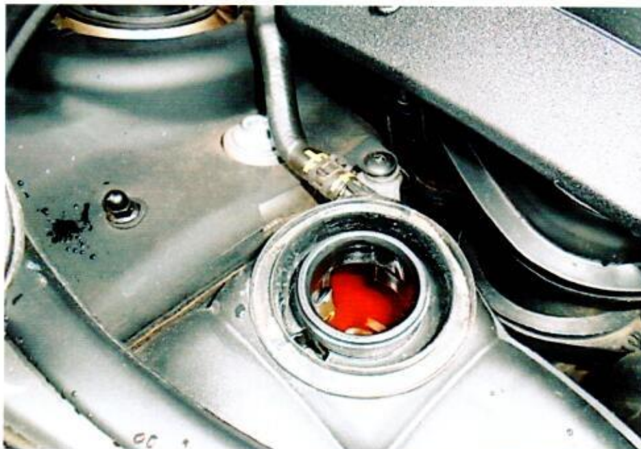
Photo 8 shows the engine coolant reservoir of the Insured Vehicle at the time of my inspection. I had found the engine coolant to be of sufficient level and without any visible contamination.
