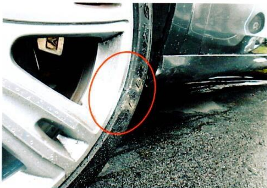
Photo 3 shows a general view of the damage (circled) to the front left wheel rim of the Insured Vehicle. The 4 tyres fitted on the Insured Vehicle were all found to be in serviceable condition with remaining tread depth of approximately 5mm each with no tear, cut or burst mark(s) on the outer and the inner sidewalls as well as across the tread of the 4 tyres.
