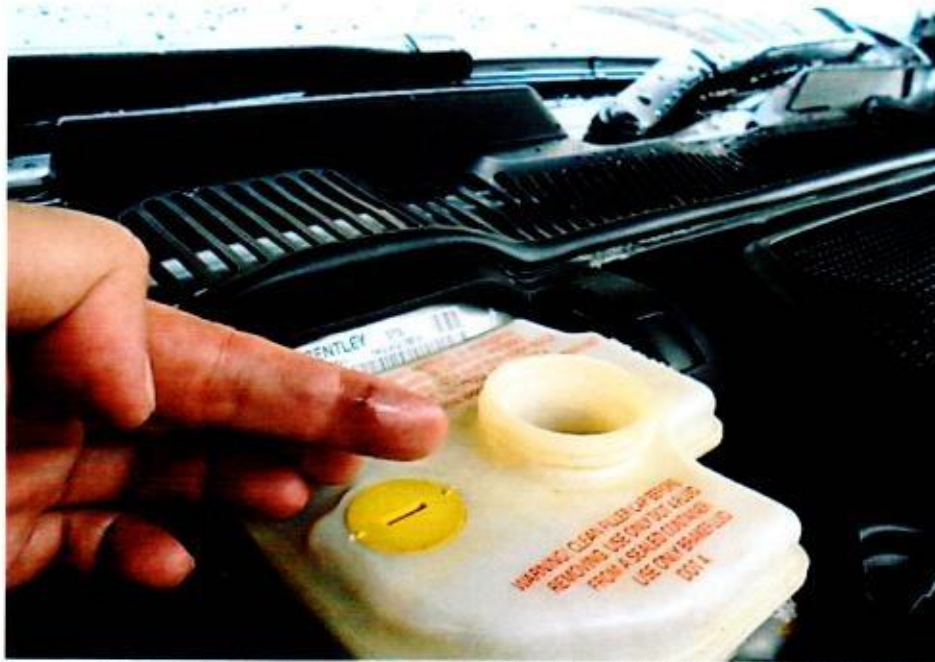
Photo 7 shows the brake fluid reservoir of the Insured Vehicle at the time of my inspection. I had found the brake fluid to be of sufficient level and without any visible contamination for operating purposes.
