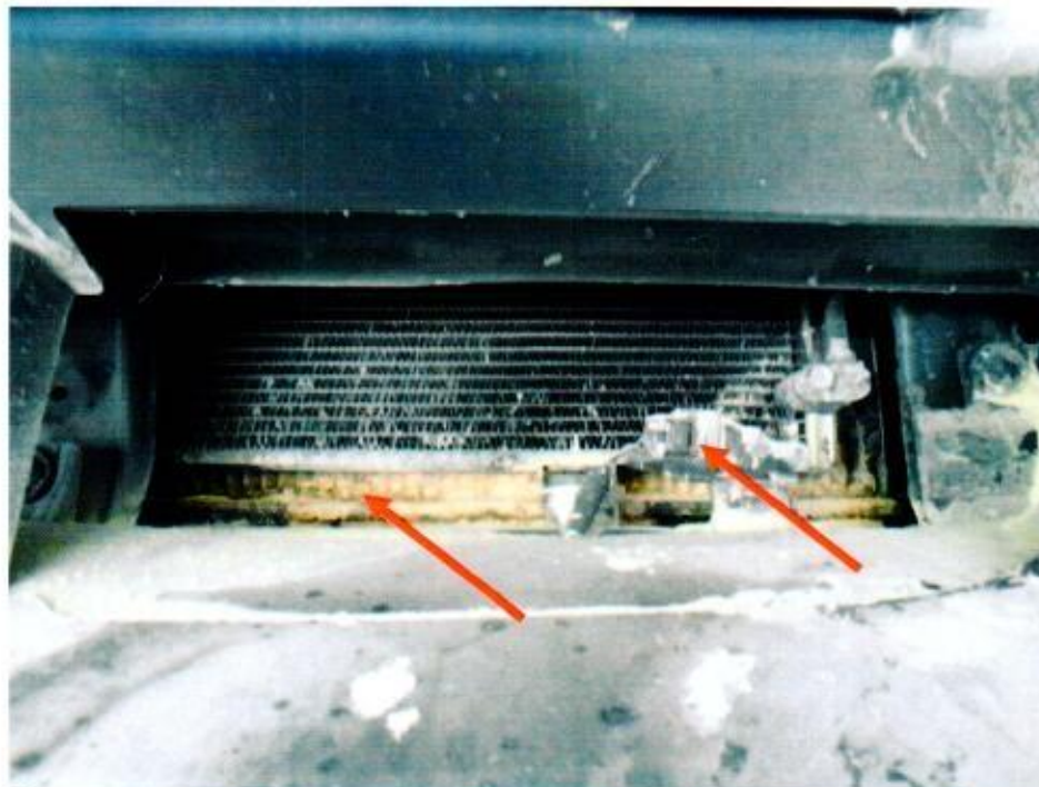
Photo 5 shows the damage of heat nature to the condenser and original wiring harness in the engine compartment portion of the Insured Vehicle at the time of our inspection. This was amongst the body parts that were found to have been affected as a result of the fire
