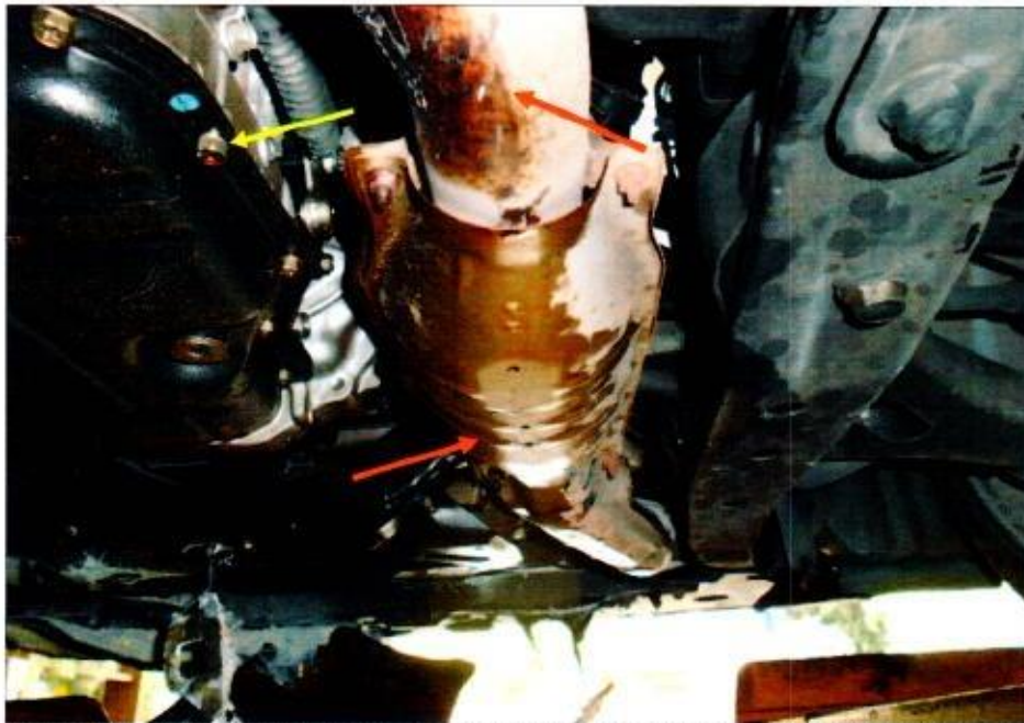
Photo 8 shows the fluid burn marks on the exhaust pipe at the undercarriage portion of the Insured Vehicle. This is the immediate vicinity where the fire to the Insured Vehicle had likely started. The transmission fluid residue can be seen on the screws of the transmission fluid sump (yellow arrow), the presence of fluid burn marks on the exhaust pipe was a sign of transmission fluid leakage onto the heated exhaust (red arrows) and this physical evidence would then appear to suggest that the cause of fire to the Insured Vehicle could have possibly been due to leakage of transmission fluids from the gasket of the fluid pan onto heated exhaust pipe surface.
