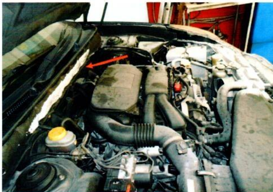
Photo 3 shows the general view of the front engine compartment portion of the Insured Vehicle at the time of our inspection. The fire damage to the Insured Vehicle was confined to its front undercarriage portion and. Its engine compartment firewall insulator (arrowed) was amongst the body parts that were found to have been affected as a result of the fire.
