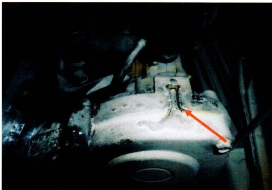
Photo 4 shows the damage of heat nature to the timing case cover (arrowed) in the engine compartment portion of the Insured Vehicle at the time of our inspection. This was amongst the body parts that were found to have been affected as a result of the fire.
