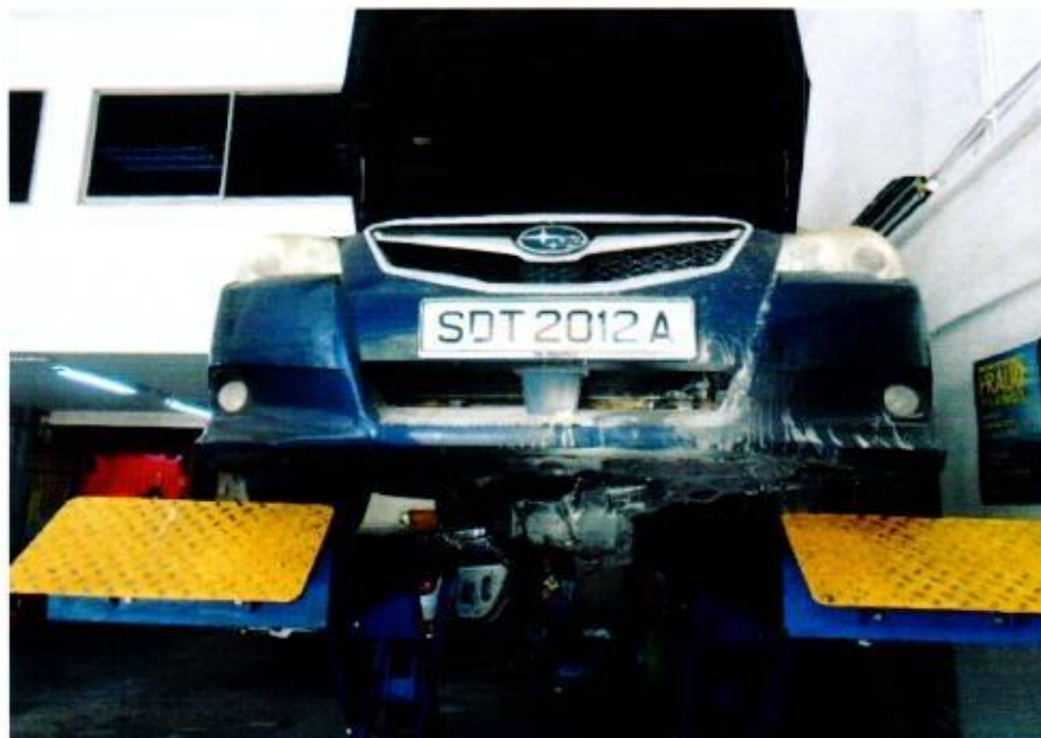
Photo 1 shows the general view of the front portion of the Insured Vehicle at the time of our inspection. The fire damage to the Insured Vehicle was confined to its front undercarriage portion. Its undercarriage splash shield, engine compartment firewall insulator, timing cover and condenser and original harness are amongst the body parts that were found to have been affected as a result of the fire.
