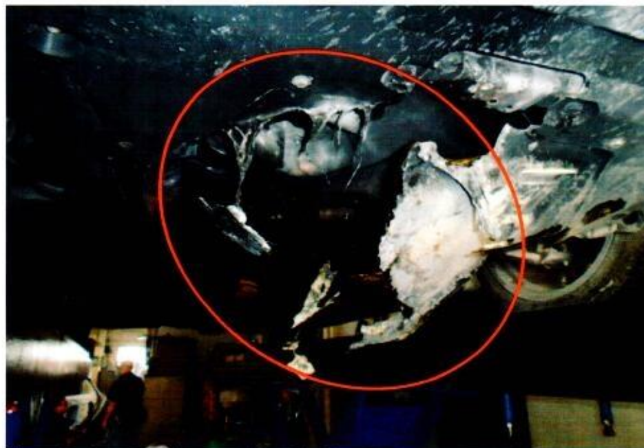
Photo 2 shows the close up view of the front undercarriage portion of the Insured Vehicle at the time of our inspection. The fire damage to the Insured Vehicle was confined to its front undercarriage portion. Its front splash shield (circled) was amongst the body parts that were found to have been affected as a result of the fire.
