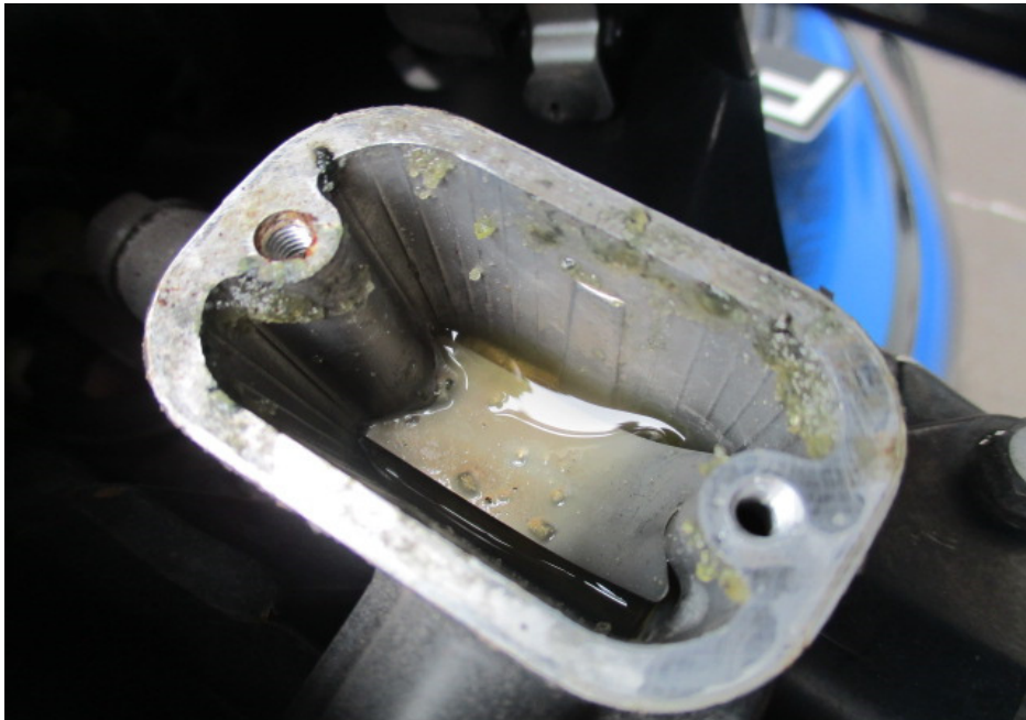
Photo 24 shows the brake fluid reservoir for the front brake of the Motorcycle. The brake fluid was observed to be without contamination however it was of insufficient level for operational purposes.
