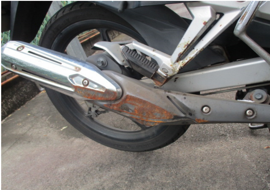
Photo 12 shows the exhaust muffler and exhaust muffler heat shield which were amongst the body parts of the Motorcycle that had sustained damages of grazing nature as a result of the accident.
