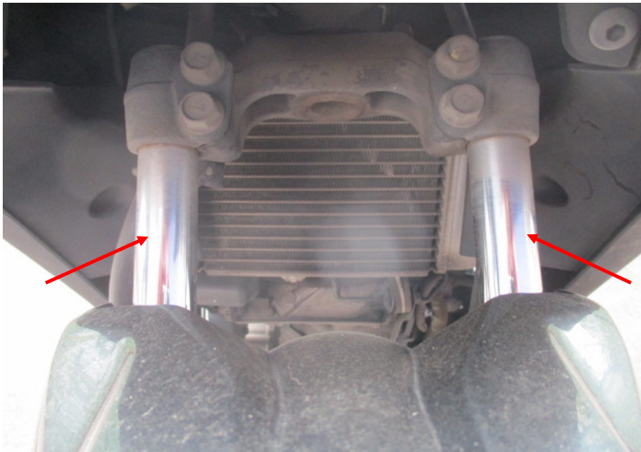
Photo 20 shows the front fork (arrowed) of the Motorcycle. The front fork and fork bracket of the Motorcycle were both found to be intact and undamaged. Turning the Motorcycle's handle bar towards the left and right did not produce any abnormal free play and/or resistance. The steering system of the Motorcycle was in serviceable condition at the time of our inspection.
