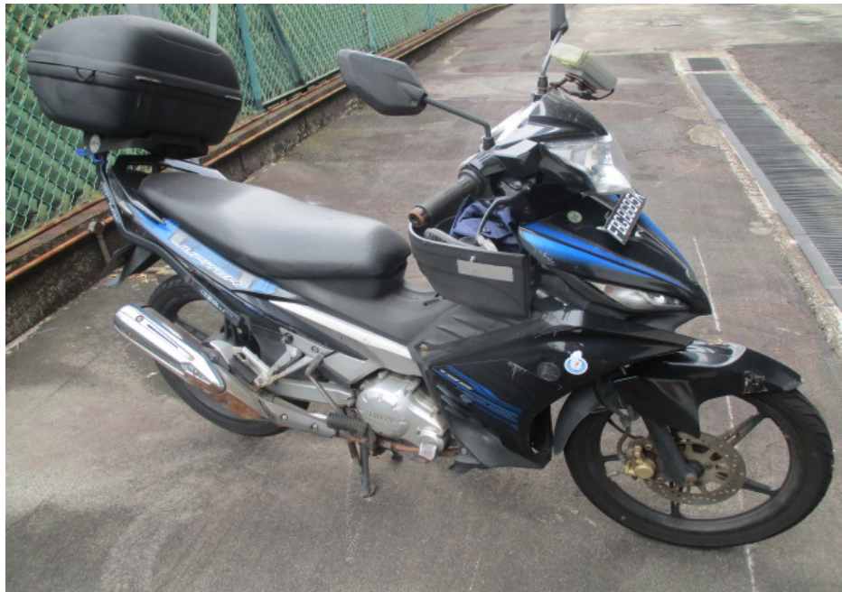
Photo 3 shows a general view of the right body of the Motorcycle at the time of our inspection. The Motorcycle was observed to have sustained damages all around. Amongst the body parts that were found to have been damaged include its headlight cowl, front cowl, front mudguard, side cowlings, front brake lever, right side mirror, right front footrest, rear brake pedal, right rear side cover and exhaust muffler, amongst others.
