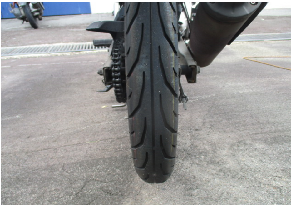
Photo 15 shows the condition of the Motorcycle's rear tyre. The rear tyre was observed to be in serviceable condition with remaining tread depth of approximately 3mm. The tyre was also observed to be sufficiently inflated for vehicular operation. We did not observe any tear, burst mark(s) and/or punctured hole(s) on the sidewalls as well as across the tread of the rear tyre.
