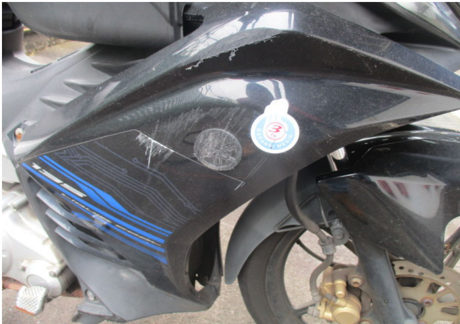
Photo 7 shows a closer view of the right cowling of the Motorcycle that had sustained damages as a result of the accident.
