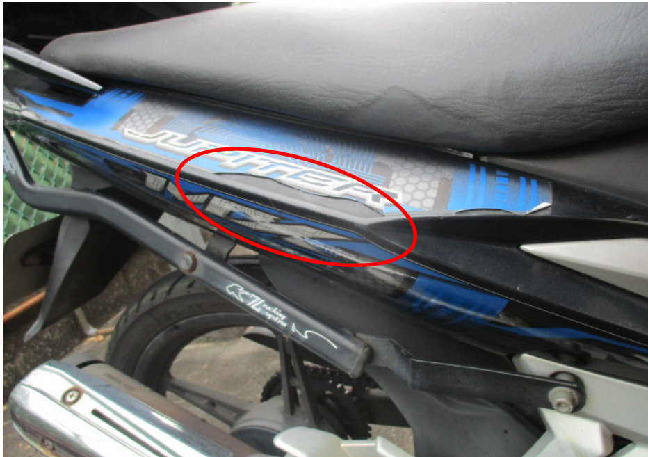
Photo 11 shows the right rear side cover of the Motorcycle which was observed to be missing as a result of the accident (circled).
