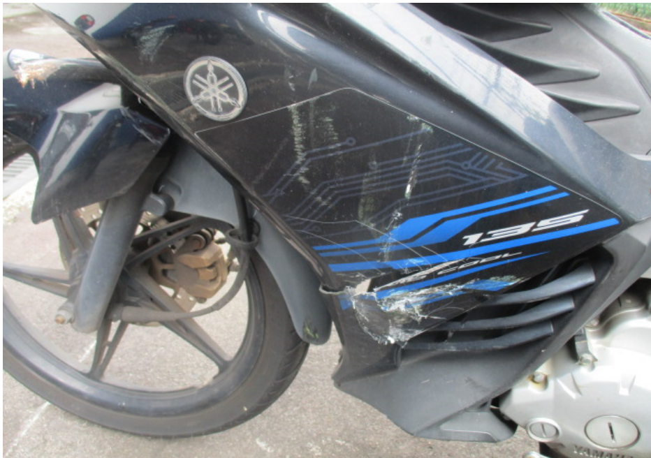
Photo 13 shows a closer view of the left cowling of the Motorcycle that had sustained damages as a result of the accident.
