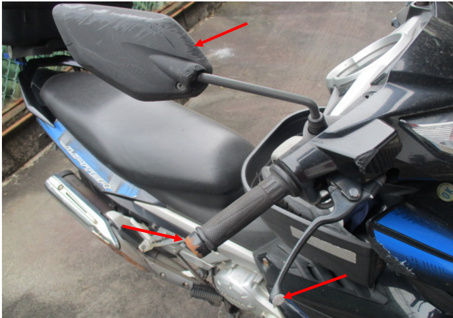
Photo 8 shows a closer view of the front brake lever, right handlebar end and right side mirror (circled) which were amongst the body parts of the Motorcycle that had sustained damage as a result of the accident.
