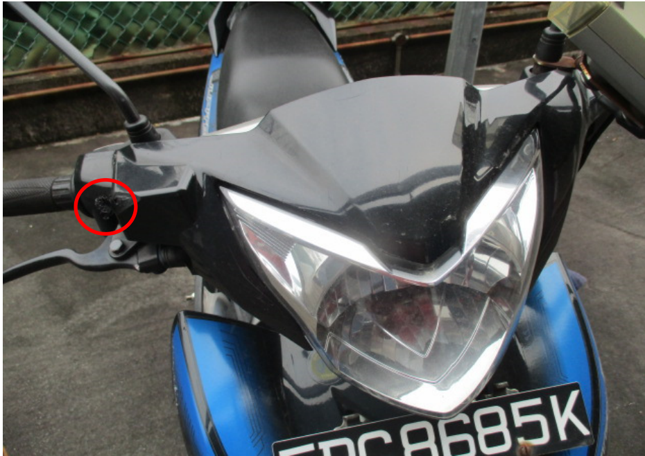
Photo 4 shows a closer view of the headlight cowl which was amongst the body parts at the front body of the Motorcycle that had sustained damage of grazing nature (circled) as a result of the accident.
