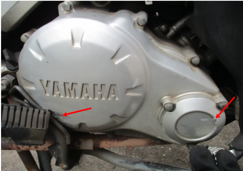
Photo 17 shows the right side of the engine of the Motorcycle at the time of our inspection. The various left engine components had sustained damage of grazing nature as a result of the accident (arrowed) however the engine components were still intact. There was also no fluid leak and/or fluid stain found around the right engine area of the Motorcycle.
