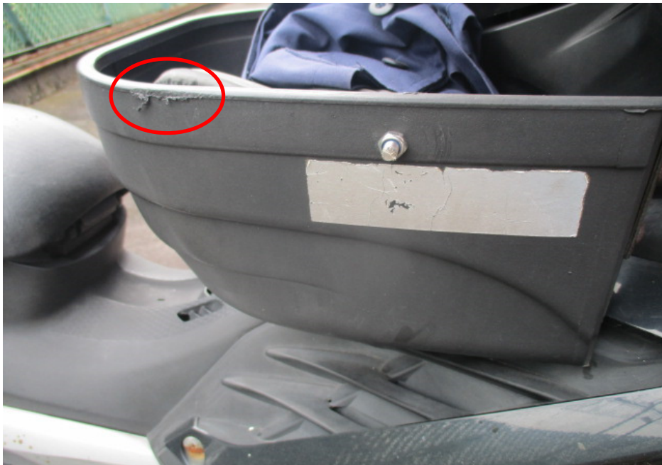
Photo 9 shows a closer view of the front box which was amongst the body parts of the Motorcycle that had sustained damage of grazing nature (circled) as a result of the accident.
