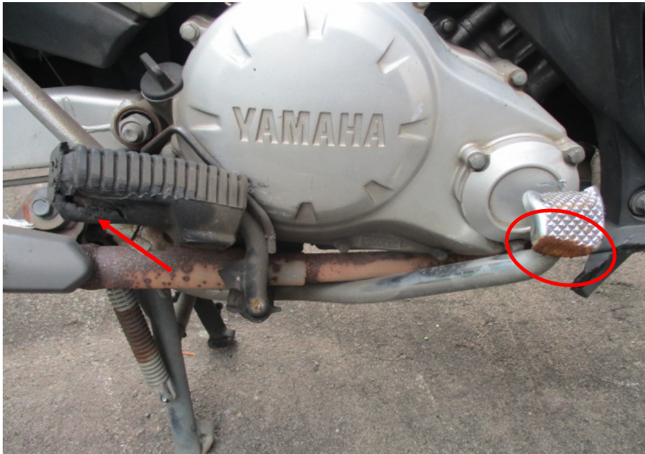
Photo 10 shows a closer view of the right front footrest (arrowed) and rear brake pedal (circled) which was amongst the body parts of the Motorcycle that had sustained damage as a result of the accident.
