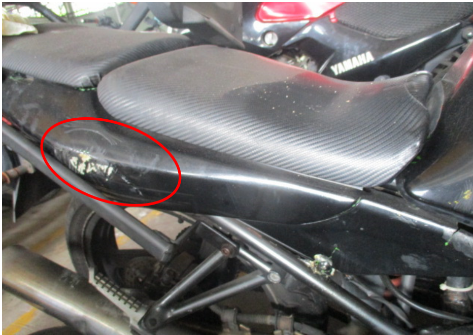
Photo 13 shows the right rear side cover (circled) which was amongst the body parts of the Motorcycle that had sustained damage as a result of the accident.
