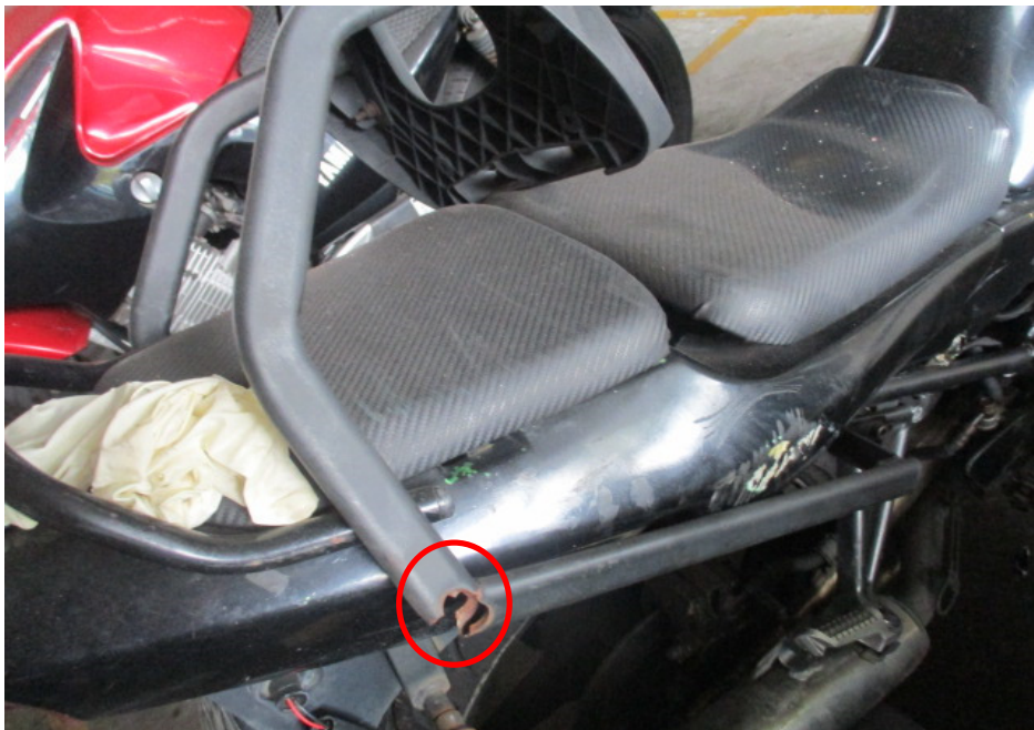
Photo 14 shows the top box rack (circled) which was amongst the body parts of the Motorcycle that had sustained damage as a result of the accident.
