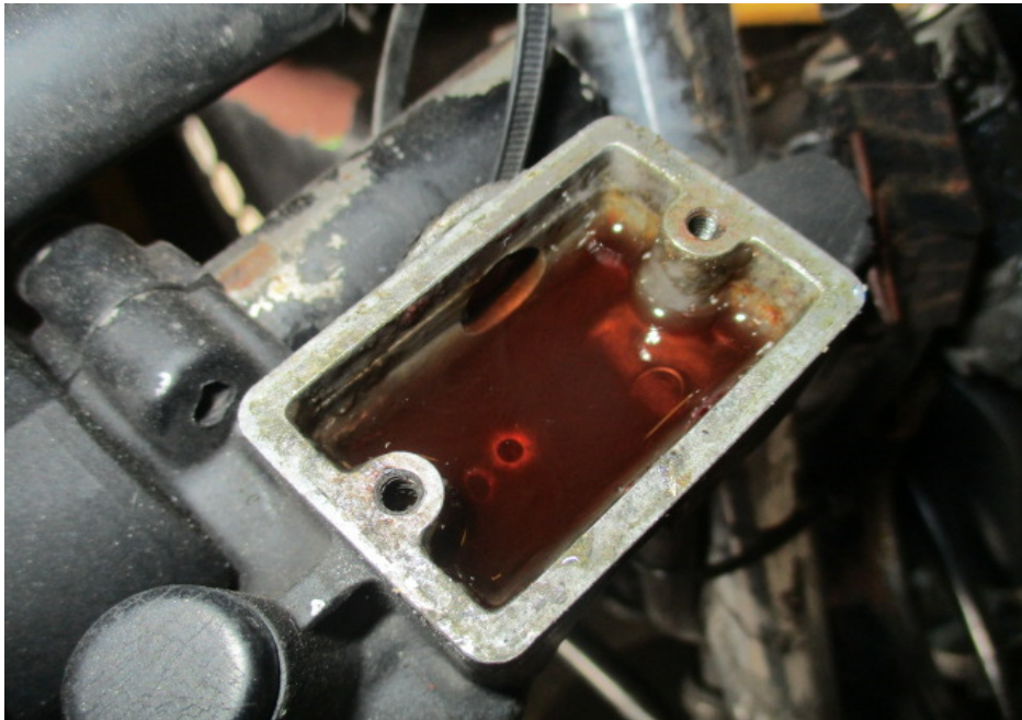
Photo 25 shows the brake fluid reservoir for the front brake of the Motorcycle. The brake fluid was observed to be of sufficient level and without contamination for operational purposes (arrowed).
