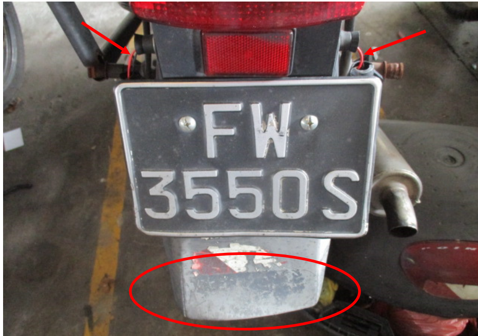
Photo 15 shows the dislodged rear signal lamps (arrowed) and deformed rear mudguard (circled) which was amongst the body parts at the rear of the Motorcycle that had sustained damage as a result of the accident.
