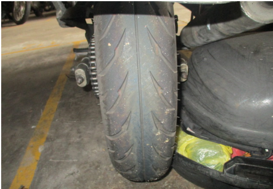
Photo 18 shows the condition of the Motorcycle's rear tyre. The rear tyre was observed to be in serviceable condition with remaining tread depth of approximately 3mm. The tyre was also observed to be sufficiently inflated for vehicular operation. We did not observe any tear, burst mark(s) and/or punctured hole(s) on the sidewalls as well as across the tread of the rear tyre.
