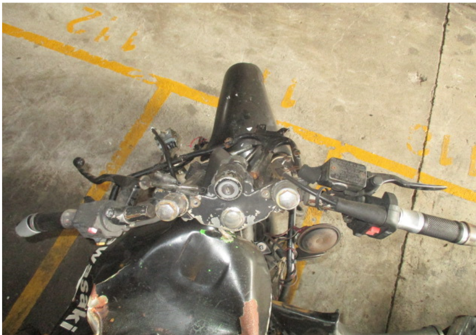
Photo 8 shows a closer view of the side mirrors, clutch lever, front brake lever, handlebars and handlebar ends of the Motorcycle. These parts were amongst the body parts of the Motorcycle which were damaged as a result of the accident.
