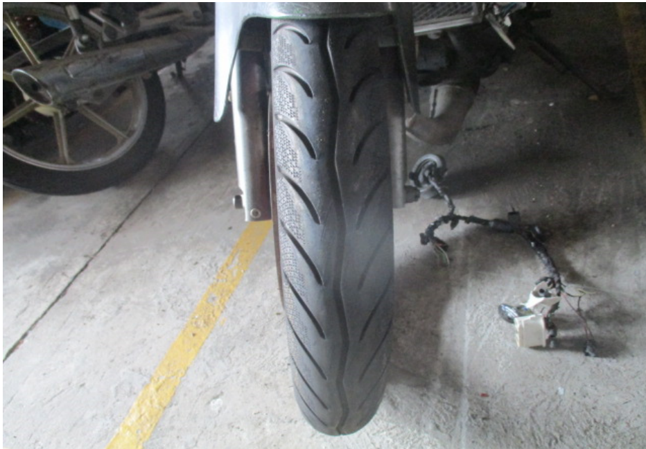
Photo 17 shows the front tyre of the Motorcycle at the time of our inspection. The front tyre was observed to be in serviceable condition with remaining tread depth of approximately 4mm. The tyre was also observed to be sufficiently inflated for vehicular operation. We did not observe any tear, burst mark(s) and/or punctured hole(s) on the sidewalls as well as across the tread of the front tyre.
