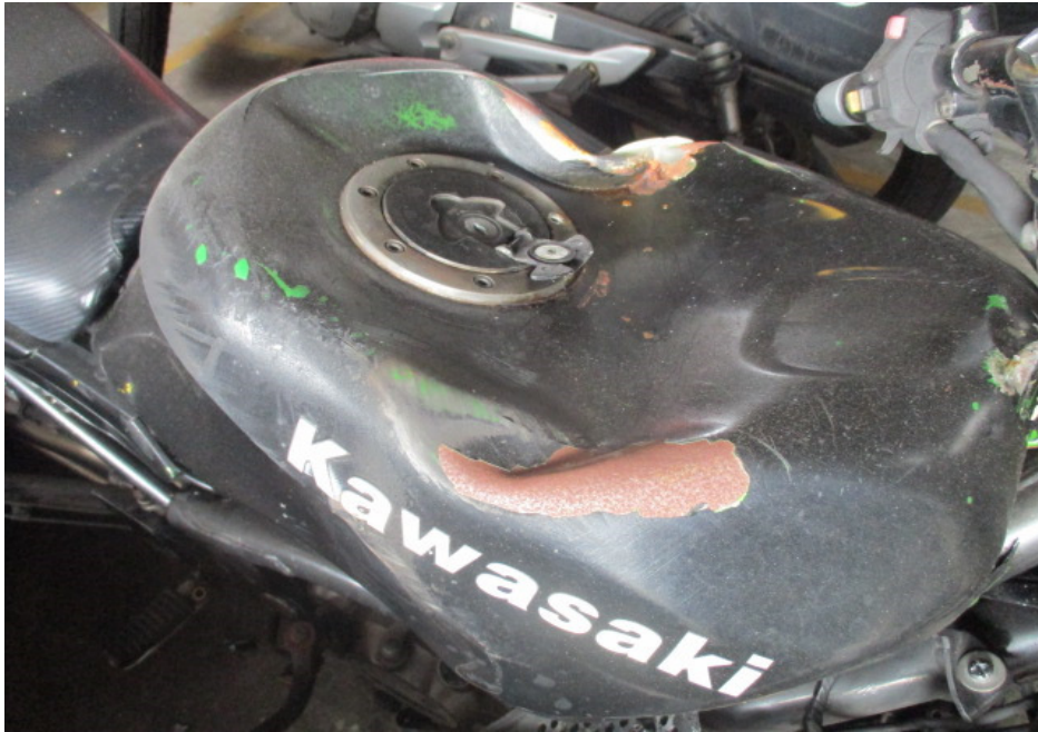
Photo 9 shows a closer view of the petrol tank, which was amongst the body parts of the Motorcycle that had sustained damage as a result of the accident.
