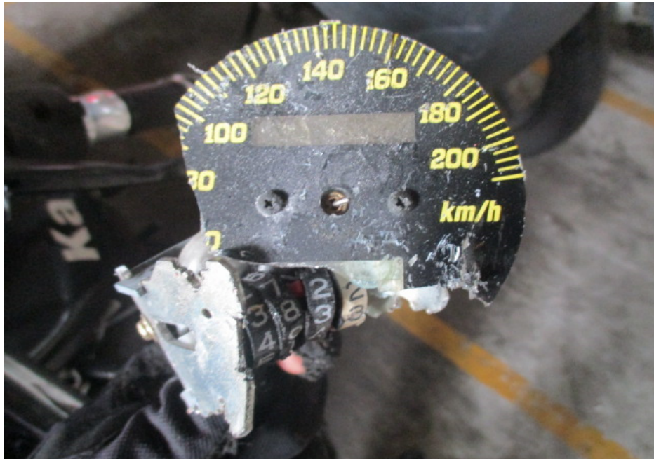
Photo 5 shows a closer view of the damaged speedometer gauge of the Motorcycle. The mileage of the Motorcycle at the time of our inspection was not recorded due to the damage sustained to the speedometer display screen as a result of the accident.
