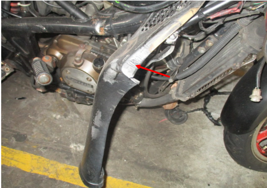
Photo 11 shows the right cowling of the Motorcycle which had sustained extensive damages (arrowed) as a result of the accident.
