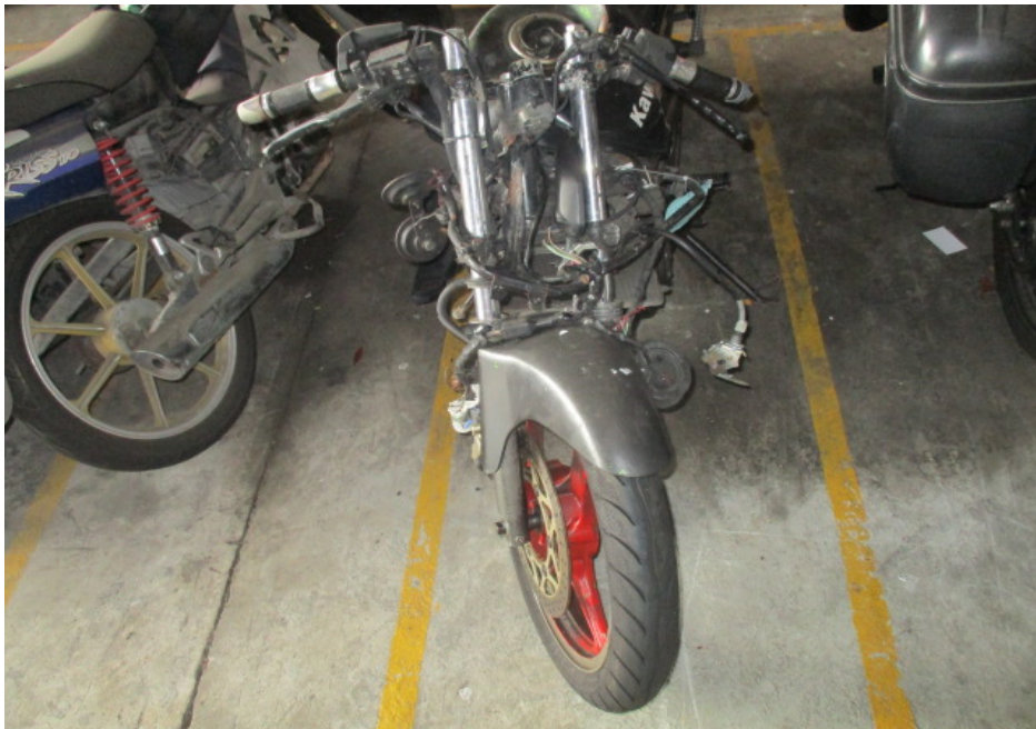
Photo 4 shows a general view of the front body of the Motorcycle at the time of our inspection. The Motorcycle was observed to have sustained damages all around. The body parts that were found to have been damaged include its speedometer gauge, headlight assembly, side cowlings, front mudguard, side mirrors, clutch lever, front brake lever, handlebars, petrol tank, rear brake pedal, exhaust muffler and rear side covers, amongst others.
