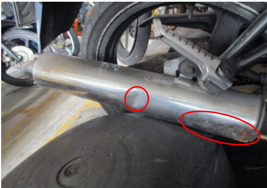
Photo 12 shows the exhaust muffler of the Motorcycle which was observed to be dented as a result of the accident (circled).
