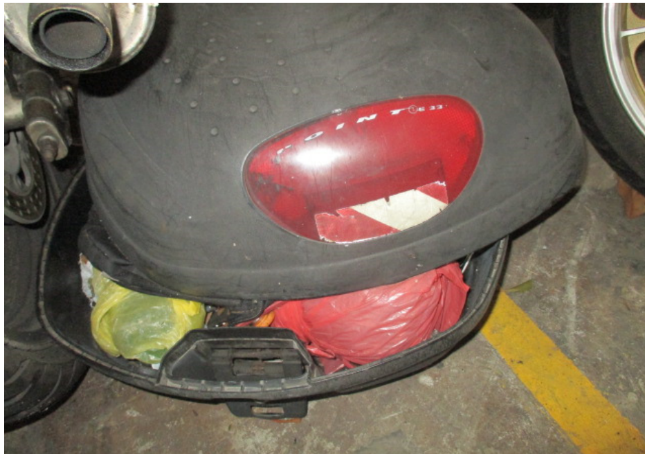
Photo 16 shows the broken top box which was amongst the body parts at the rear of the Motorcycle that had sustained damage as a result of the accident.
