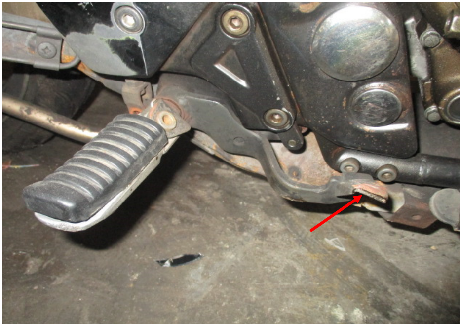
Photo 10 shows a closer view of the rear brake pedal (arrowed) which was amongst the body parts of the Motorcycle that had sustained damage as a result of the accident.
