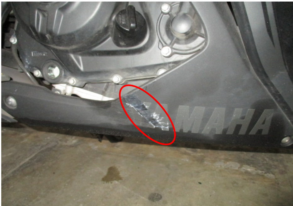
Photo 9 shows a closer view of the right bottom cowling (circled) which was amongst the body parts of the Motorcycle that had sustained damage as a result of the accident.
