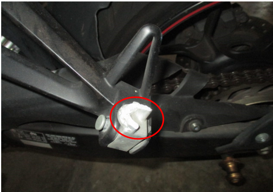
Photo 13 shows a closer view of the broken left pillion foot peg (circled) of the Motorcycle as a result of the accident.
