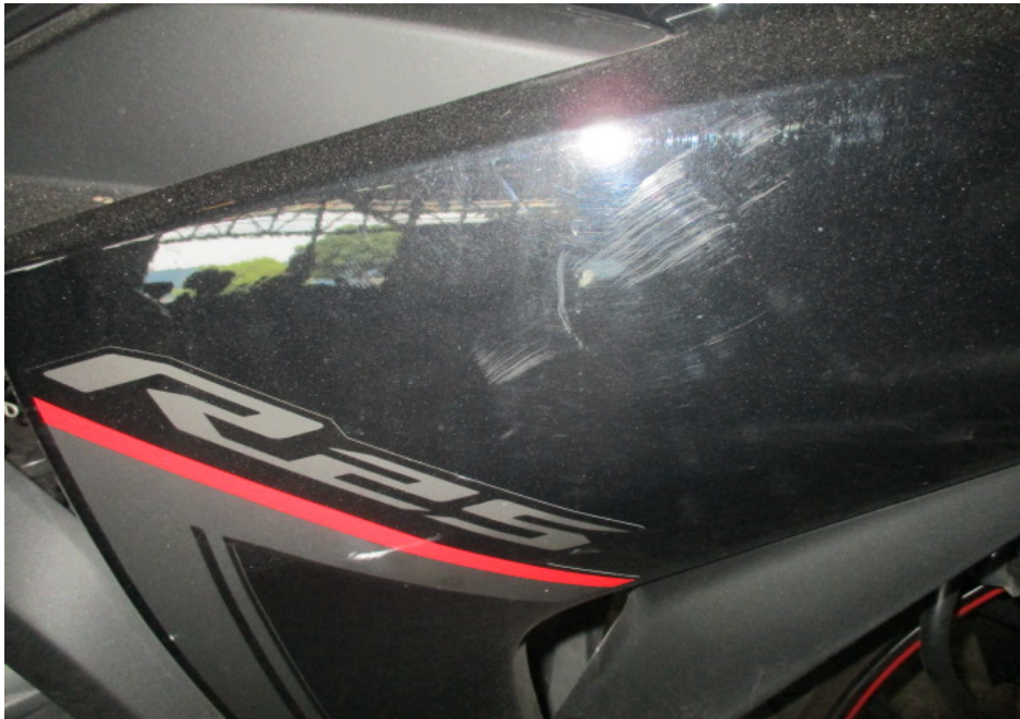
Photo 8 shows a closer view of the right cowling of the Motorcycle that had sustained damages of grazing nature as a result of the accident.
