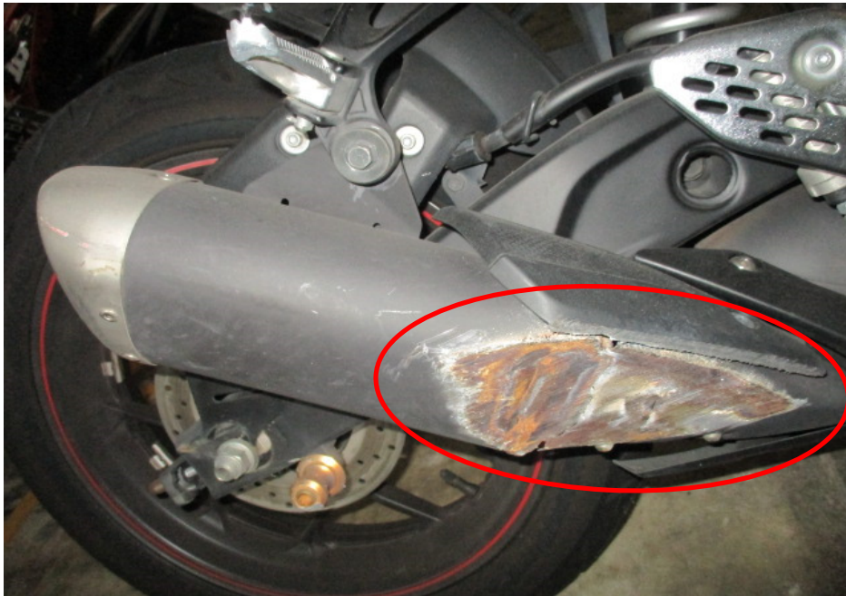
Photo 14 shows a closer view of the exhaust muffler and exhaust muffler heat shield (circled) of the Motorcycle that had sustained damages of grazing nature as a result of the accident.
