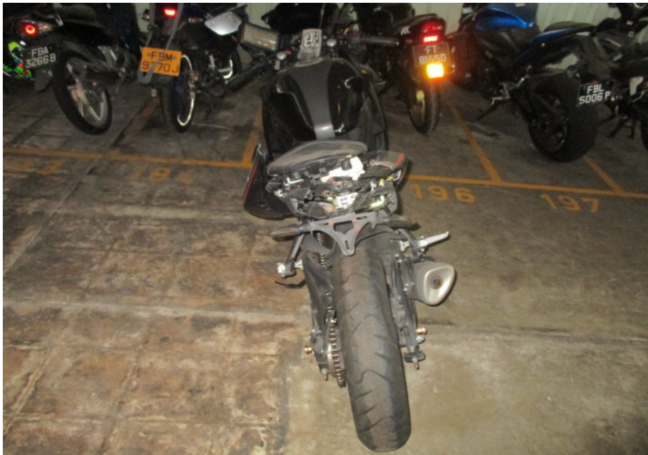
Photo 5 shows a general view of the rear portion of the Motorcycle at the time of our inspection. The Motorcycle was observed to have sustained damages all around. Amongst the body parts that were found to have been damaged include its head cowl, right cowl, rear brake pedal, right front footrest, left pillion foot peg, rear side covers, exhaust muffler and rear hugger, amongst others.
