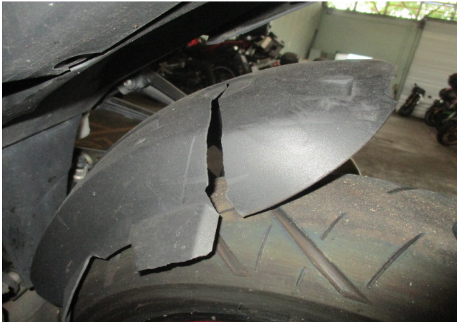
Photo 12 shows a closer view of the cracked rear hugger of the Motorcycle as a result of the accident.
