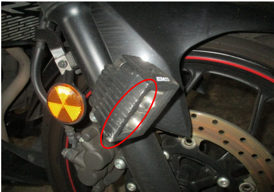
Photo 7 shows a closer view of the right fog lamp (circled) which was amongst the body parts at the front body of the Motorcycle that had sustained damage as a result of the accident.
