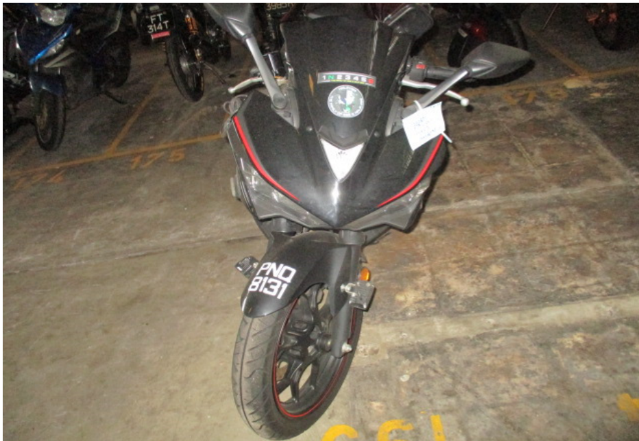
Photo 24 shows the front wheel of the Motorcycle turned towards its full right. Turning the Motorcycle's handle bar towards the left and right did not produce any abnormal free play and/or resistance. This would indicate that the steering system of the Motorcycle was in serviceable condition at the time of our inspection.
