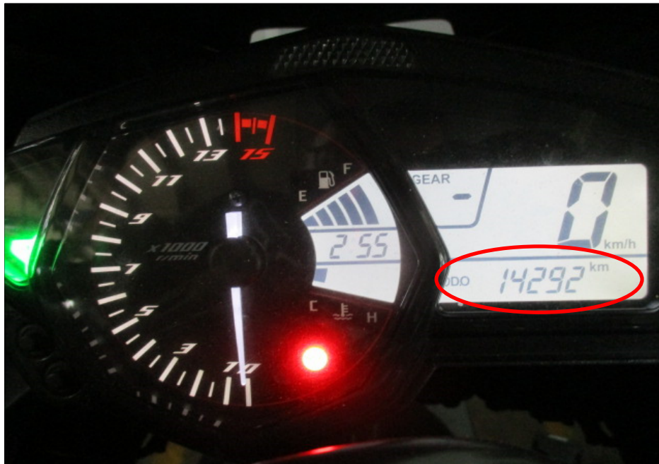
Photo 1 shows the speedometer gauge of the Motorcycle where the mileage recorded at the time of our inspection was 14, 292km (circled).
