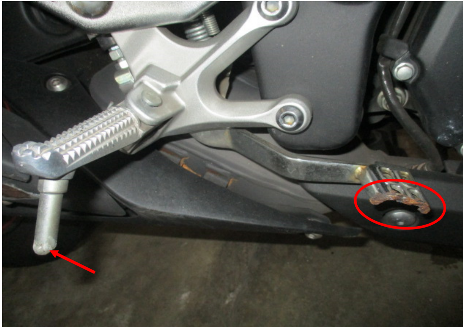
Photo 10 shows a closer view of the rear brake pedal (circled) and right front footrest (arrowed) which were amongst the body parts of the Motorcycle that had sustained damage as a result of the accident.
