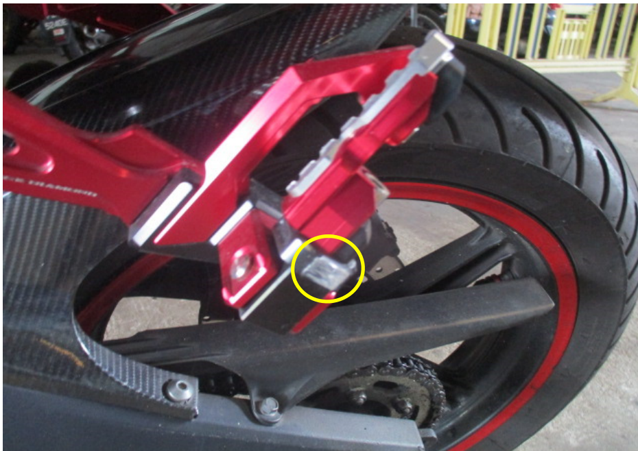
Photo 13 shows a closer view of the left pillion foot peg which was amongst the body parts of the Motorcycle that had sustained damages of grazing nature as a result of the accident (circled).
