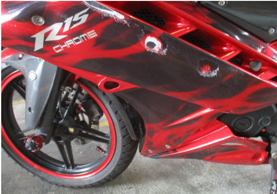
Photo 8 shows a closer view of the left cowling of the Motorcycle that had sustained damages of grazing nature as a result of the accident.
