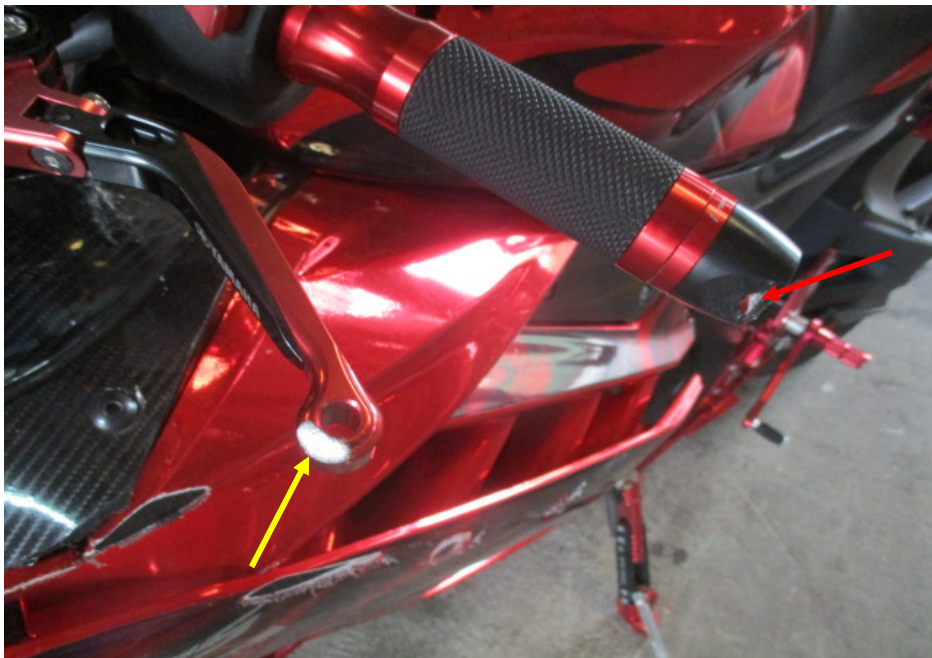
Photo 9 shows a closer view of the left handlebar end and clutch lever (arrowed) which were amongst the body parts of the Motorcycle that had sustained damage as a result of the accident.
