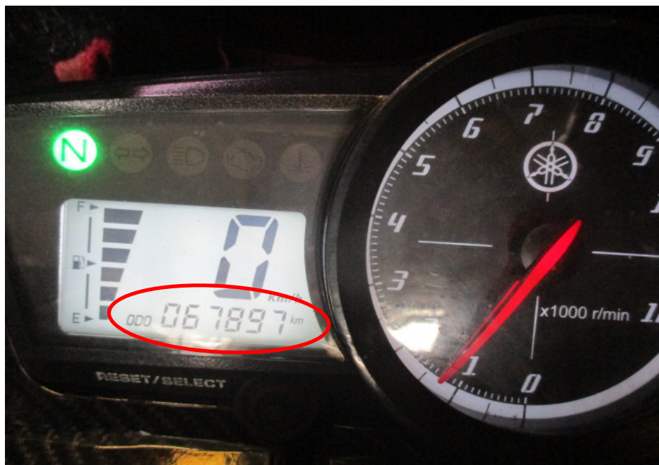
Photo 1 shows the speedometer gauge of the Motorcycle where the mileage recorded at the time of our inspection was 67, 897km (circled).
