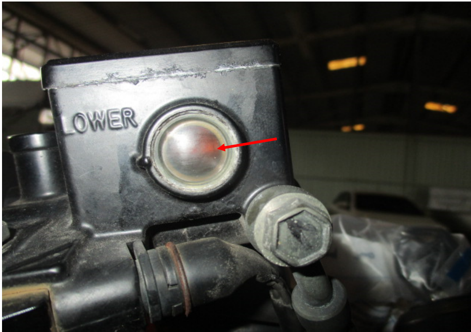
Photo 26 shows the brake fluid reservoir for the front brake of the Motorcycle. The brake fluid was observed to be of sufficient level and without contamination for operational purposes (arrowed).
