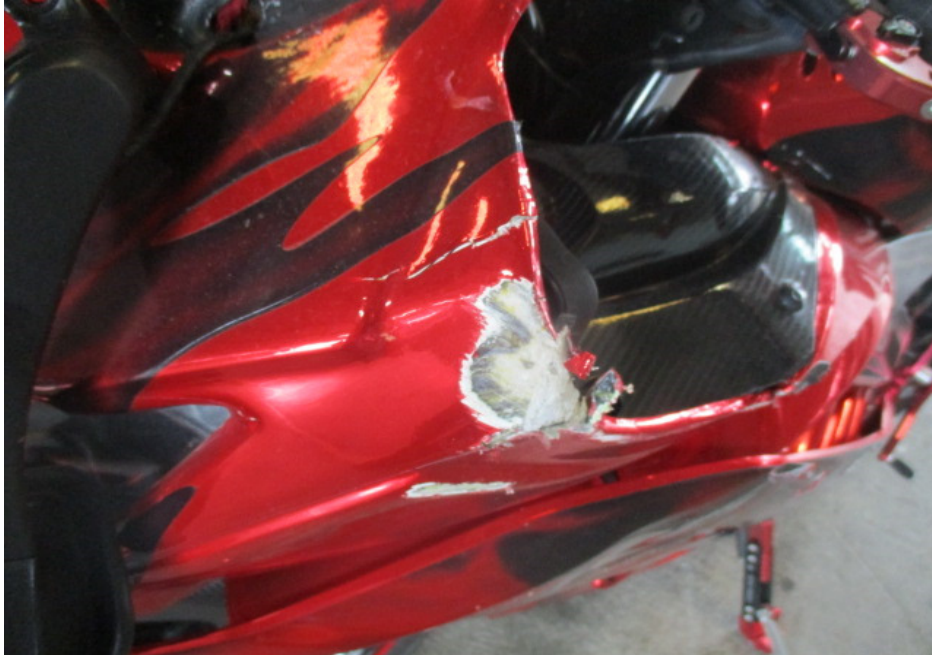
Photo 6 shows a close up view of the head cowl which was amongst the body parts of the Motorcycle that had sustained damage as a result of the accident.
