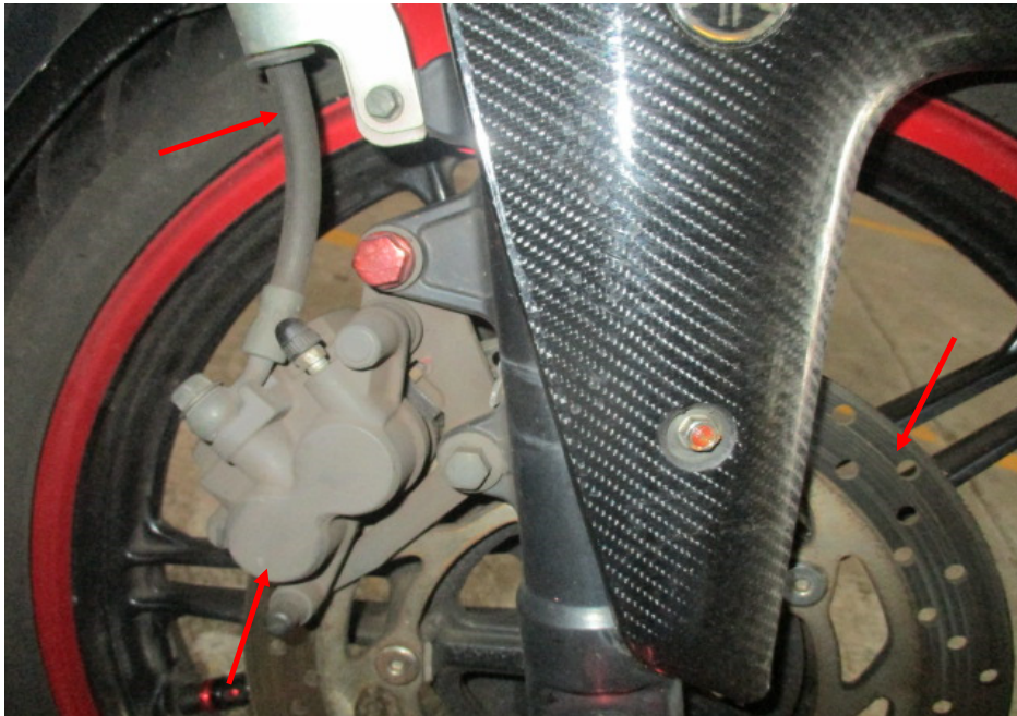
Photo 25 shows a close up view of the front brake caliper, front brake disc and front brake hose (arrowed) of the Motorcycle, which are all part of the components in the hydraulic front brake system of the Motorcycle. Our visual checks of these various components had revealed all to be intact with no visible damage. No leakage of brake fluid was also observed.
