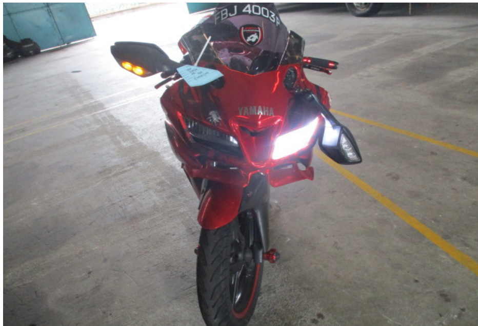
Photo 24 shows the front wheel of the Motorcycle turned towards its full right. Turning the Motorcycle's handle bar towards the left and right did not produce any abnormal free play and/or resistance. This would indicate that the steering system of the Motorcycle was in serviceable condition at the time of our inspection.
