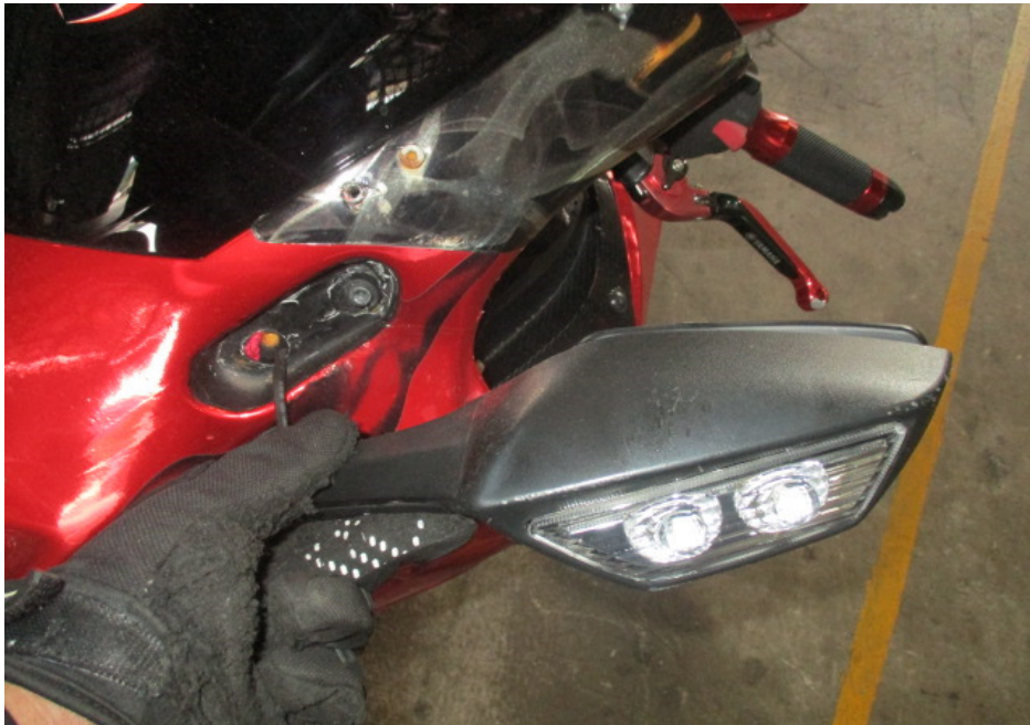
Photo 7 shows a closer view of the dislodged left side mirror which was amongst the body parts at the front body of the Motorcycle that had sustained damage as a result of the accident.
