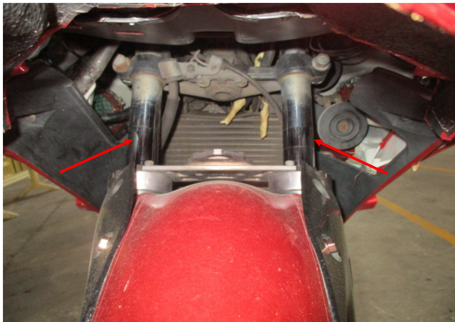
Photo 22 shows the front fork (arrowed) of the Motorcycle. The front fork and fork bracket of the Motorcycle were both found to be intact and undamaged. Turning the Motorcycle's handle bar towards the left and right did not produce any abnormal free play and/or resistance. The steering system of the Motorcycle was in serviceable condition at the time of our inspection.
