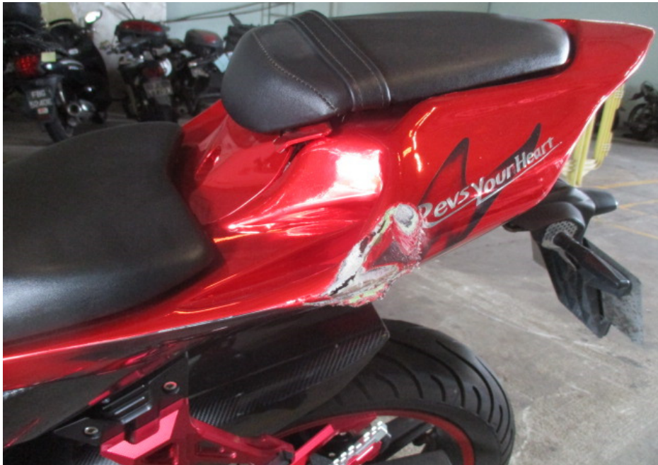
Photo 12 shows the cracked left rear side cover of the Motorcycle as a result of the accident.
