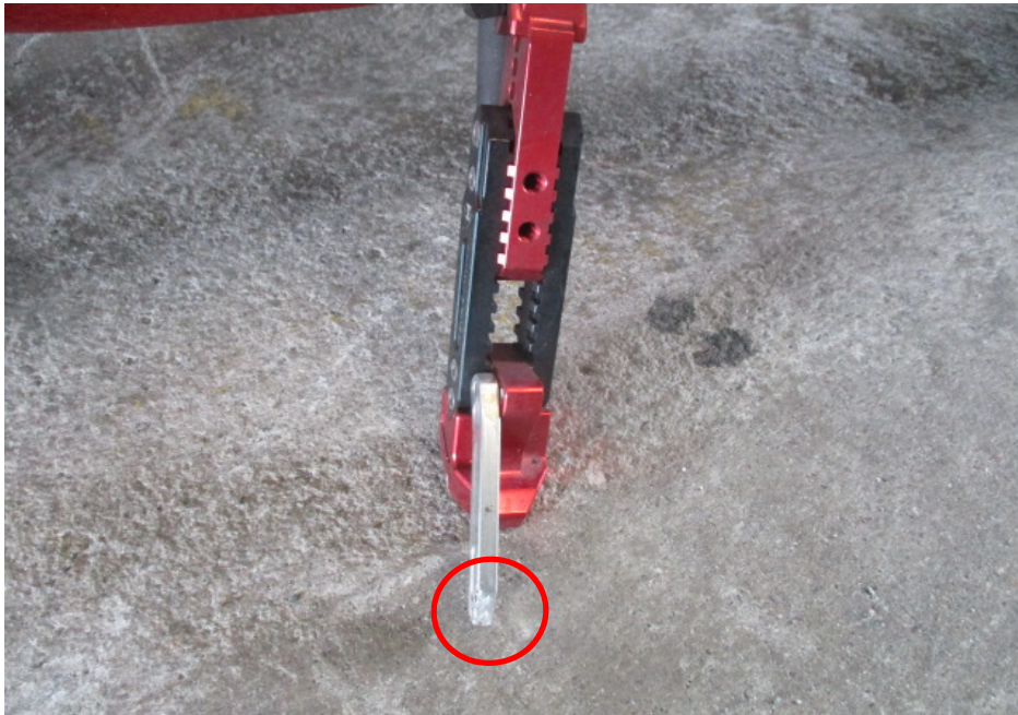
Photo 10 shows a closer view of the side stand of the Motorcycle that had sustained damages of grazing nature as a result of the accident (circled).
