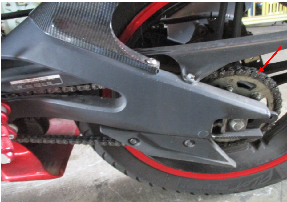
Photo 20 shows the general view of the gear train (arrowed) of the Motorcycle, which was observed to be intact with no misalignment. It was also adequately lubricated for operating purposes.
