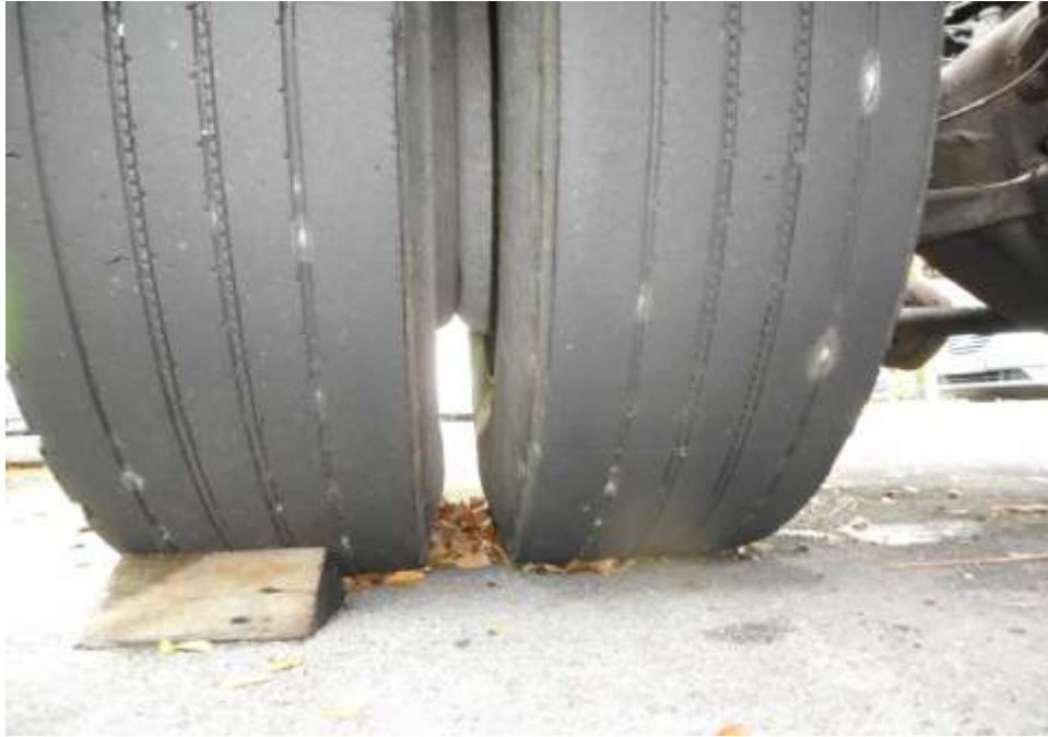
Photo 8 shows the condition of the rear right tyre of the Garbage Truck, which was observed to be in serviceable condition with remaining tread depth of approximately 3.5mm. The tyre, which was wrapped around standard steel wheel rim, was also observed to be sufficiently inflated for vehicular operation.
