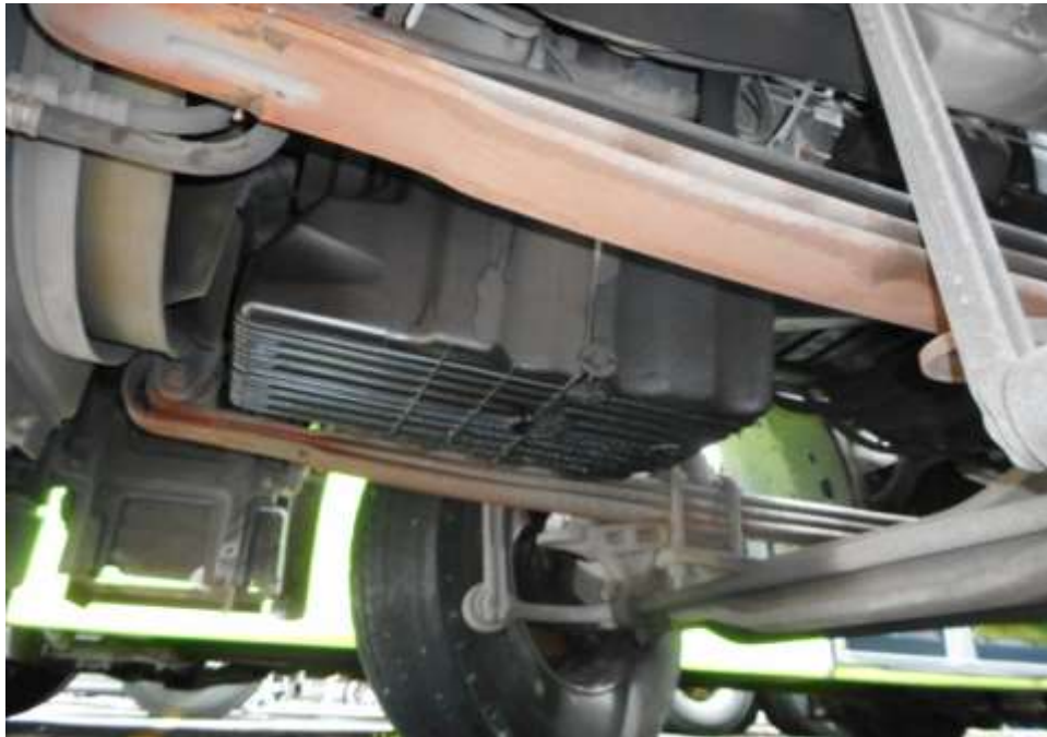
Photo 13 shows the undercarriage of the Garbage Truck, at the area where the engine housing located. I did find old fluid stain(s) on the underside oil sump of the Garbage Truck.
