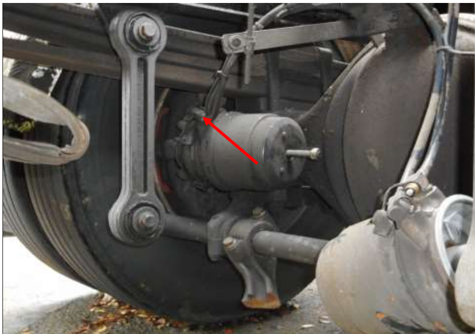
Photo 15 shows the brake pipe (arrowed) at the rear left wheel of the Garbage Truck. I did not observe any leakage of air at the time of my inspection of the Garbage Truck.
