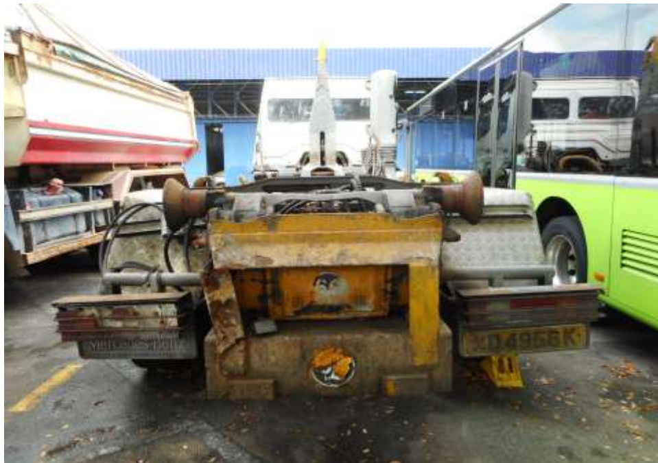
Photo 5 shows a general view of the Garbage Truck's rear body at the time of my inspection. Its rear left brake lamp and rear body panel was damaged as a result of the accident.
