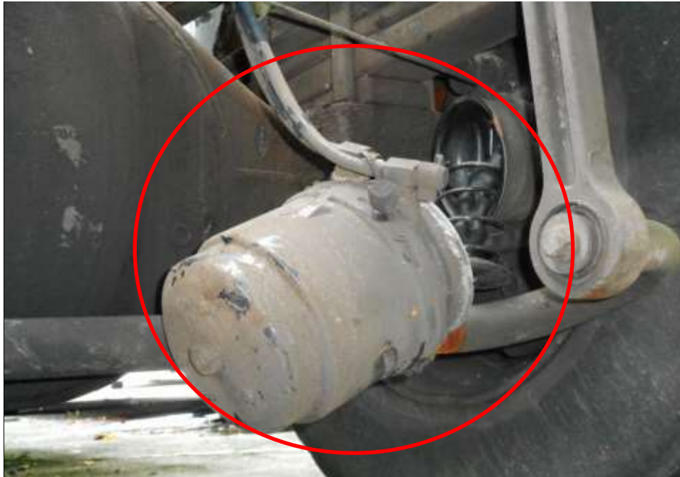
Photo 14 shows the brake cylinder of the (circled) the rear right wheel of the Garbage Truck. It was damaged was due to the impact caused by the result of the accident.
