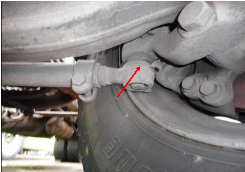
Photo 20 shows the various undercarriage components at the front left wheel of the Garbage Truck, in particular the steering tie rod end (arrowed). The various undercarriage components of the Garbage Truck were all found to be intact without any visible damage. There was also no sign of fluid stain(s) observed on the various undercarriage components.
