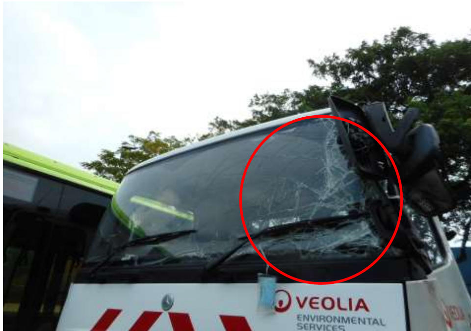
Photo 2 shows a close up view of the front body of the Garbage Truck at the time of my inspection. The Garbage Truck was observed to have sustained moderate damage at its front and left portion. Its front windscreen (circled) was damaged as a result of the accident
