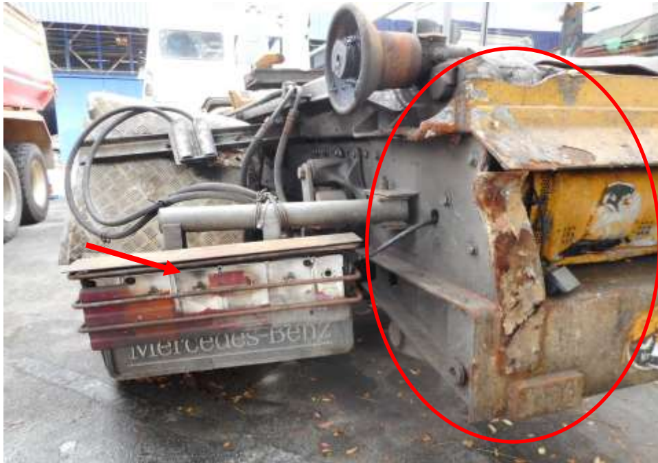
Photo 6 shows a close up view of the Garbage Truck's rear body at the time of my inspection. Its rear left brake lamp (arrowed) and rear body panel (circled) was damaged as a result of the accident.
