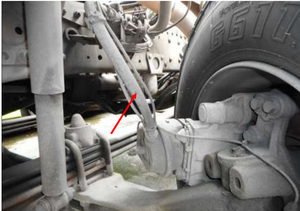
Photo 16 shows the brake pipe (arrowed) at the front left wheel of the Garbage Truck. I did not observe any leakage of air at the time of my inspection of the Garbage Truck.
