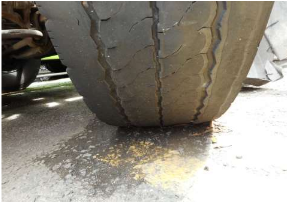
Photo 10 shows the condition of the front left tyres of the Garbage Truck, which were observed to be in serviceable condition with remaining tread depth of approximately 4.9mm. There was also no tear, cut or burst mark(s) on the outer and the inner sidewalls as well as across the tread of the 6 tyres that were fitted on the Garbage Truck.
