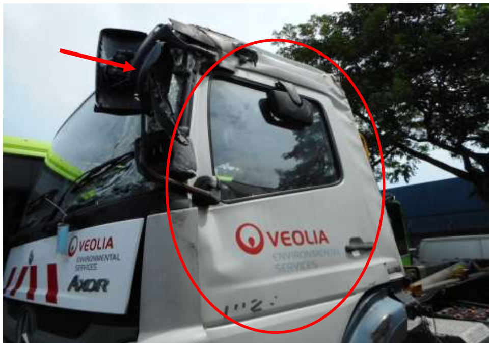
Photo 3 shows a close up view of the left body of the Garbage Truck at the time of my inspection. The Garbage Truck was observed to have sustained moderate damage at its front and left portion. Its left door (circled) and left rear-view mirror (arrowed) was damaged as a result of the accident
