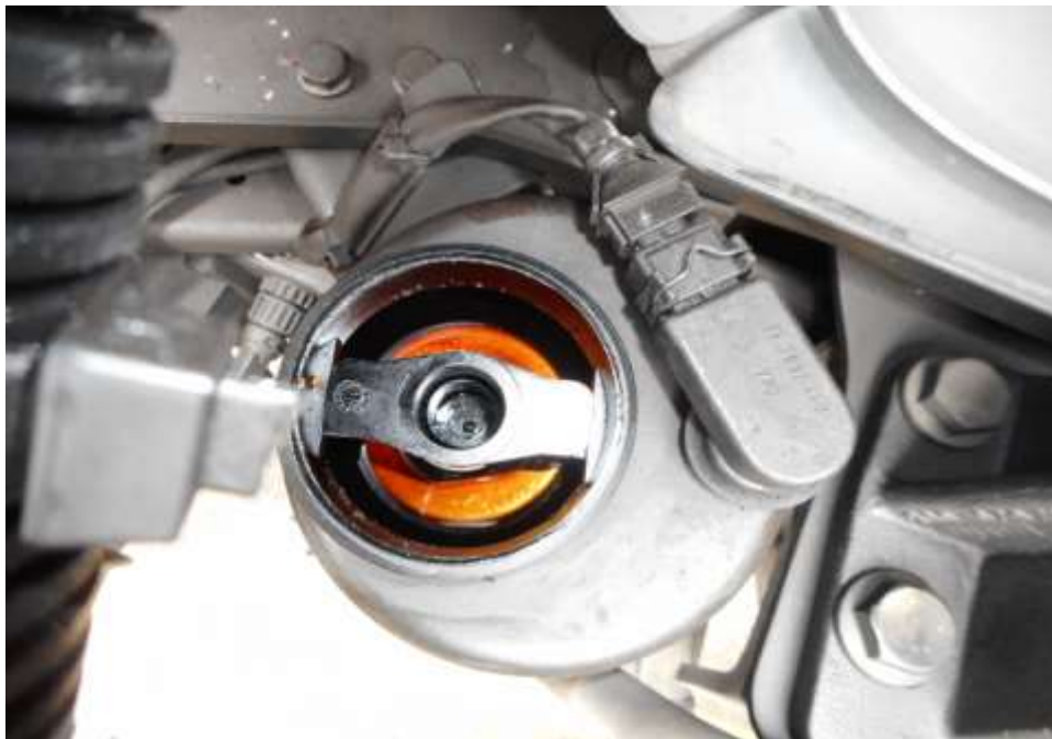
Photo 12 shows the power steering fluid reservoir of the Garbage Truck at the time of my inspection. The power steering fluid was observed to be of sufficient level and without any visible contamination.
