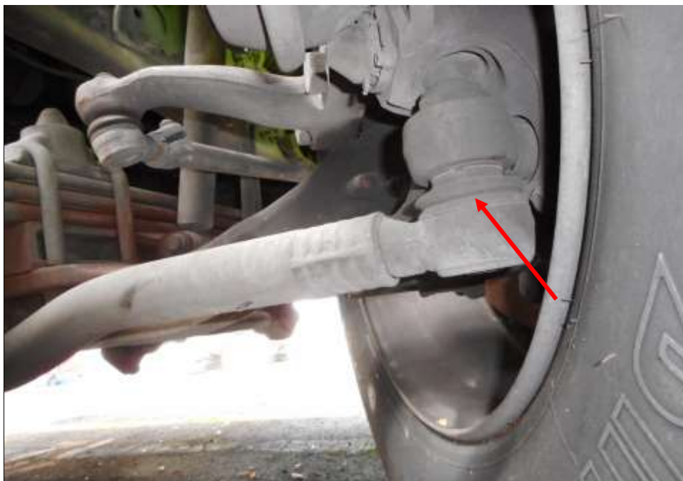
Photo 19 shows the various undercarriage components at the front right wheel of the Garbage Truck, in particular the steering tie rod end (arrowed). The various steering components were all found to be intact, suggesting that the steering system of the Garbage Truck was likely to be in serviceable condition at the material time of accident. There was also no sign of fluid stain(s) observed on the various undercarriage components.
