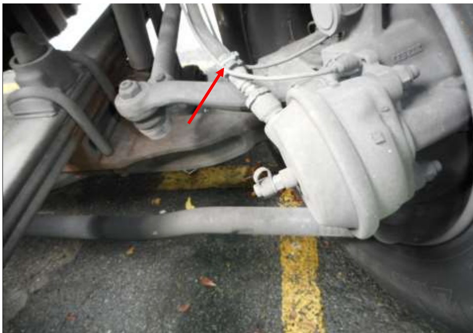
Photo 17 shows the brake pipe (arrowed) at the front right wheel of the Garbage Truck. I did not observe any leakage of brake fluid at the time of my inspection of the Garbage Truck.
