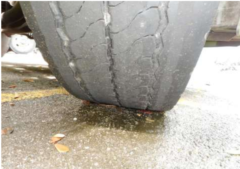
Photo 7 shows the condition of the front right tyre of the Garbage Truck, which was observed to be in serviceable condition with remaining tread depth of approximately 3.9 mm. The tyre, which was wrapped around standard steel wheel rim, was also observed to be sufficiently inflated for vehicular operation. There was no tear, cut or burst mark(s) on the outer and the inner sidewalls as well as across the tread of the 6 tyres that were fitted on the Garbage Truck.
