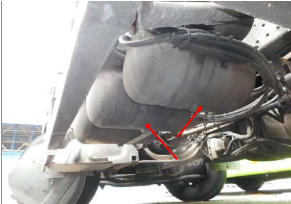
Photo 18 shows the air brake cylinders (arrowed) at the undercarriage of the Garbage Truck. I did not observe any leakage of air brake fluid at the time of my inspection of the Garbage Truck.
