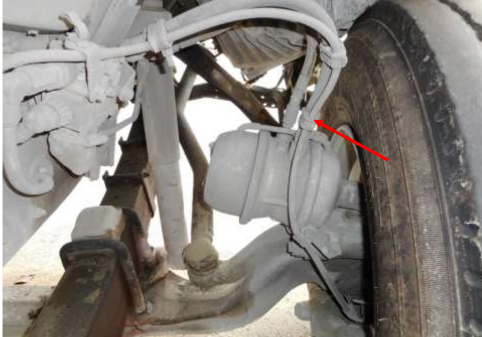
Photo 13 shows the brake pipe (arrowed) at the front right wheel of the Motor Lorry. I did not observe any leakage of brake fluid at the time of my inspection of the Motor Lorry. My static tests of the Motor Lorry's braking system, along with my visual examination of the various mechanical components in the braking system, had indicated that there was no internal leakage of pressure/vacuum. Hence the braking system of the Motor Lorry was likely to be in serviceable condition at the material time of accident.
