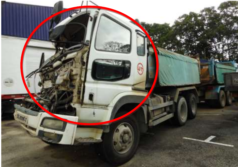
Photo 4 shows a close up view of the front left body of the Motor Lorry at the time of my inspection. Its whole front cabin, front left door (circled) were damaged as a result of the accident
