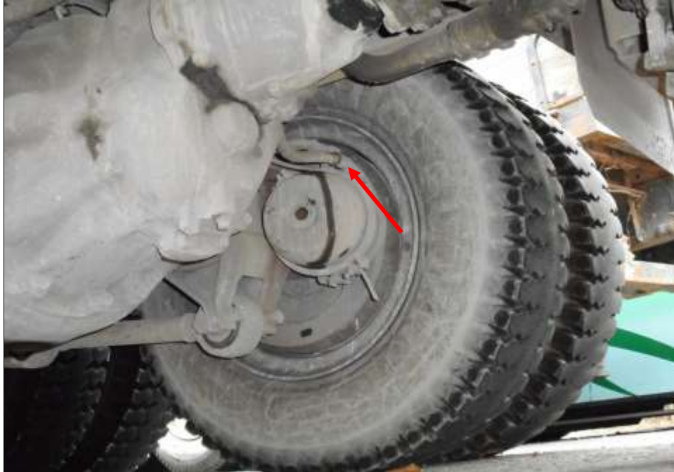
Photo 11 shows the brake pipe (arrowed) at the rear right wheel of the Motor Lorry. I did not observe any leakage of brake fluid at the time of my inspection of the Motor Lorry. My static tests of the Motor Lorry's braking system, along with my visual examination of the various mechanical components in the braking system, had indicated that there was no internal leakage of pressure/vacuum. Hence the braking system of the Motor Lorry was likely to be in serviceable condition at the material time of accident.
