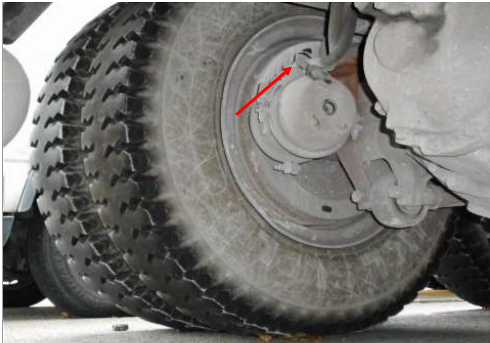
Photo 12 shows the brake pipe (arrowed) at the rear left wheel of the Motor Lorry. I did not observe any leakage of brake fluid at the time of my inspection of the Motor Lorry. My static tests of the Motor Lorry's braking system, along with my visual examination of the various mechanical components in the braking system, had indicated that there was no internal leakage of pressure/vacuum. Hence the braking system of the Motor Lorry was likely to be in serviceable condition at the material time of accident.
