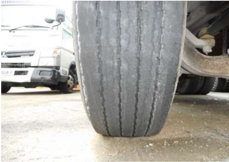
Photo 6 shows the condition of the front right tyre of the Motor Lorry, which was observed to be in serviceable condition with remaining tread depth of approximately 6.2 mm. The tyre, which was wrapped around standard steel wheel rim, was also observed to be sufficiently inflated for vehicular operation. There was no tear, cut or burst mark(s) on the outer and the inner sidewalls as well as across the tread of the 10 tyres that were fitted on the Motor Lorry.
