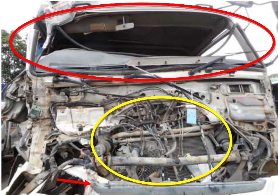
Photo 2 shows a close up view of the front body of the Motor Lorry at the time of my inspection. Its whole front cabin, front windscreen (red circle), front bumper, its ignition system and engine system (yellow circle) were damaged as a result of the accident
