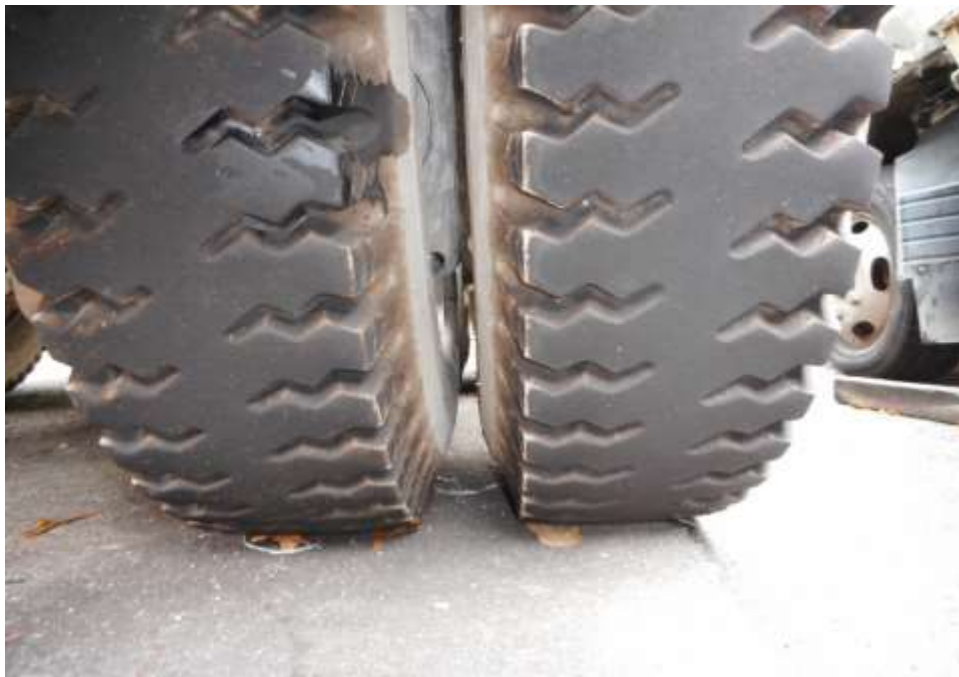
Photo 7 shows the condition of the rear right tyre of the Motor Lorry, which was observed to be in serviceable condition with remaining tread depth of approximately 11.4mm.
