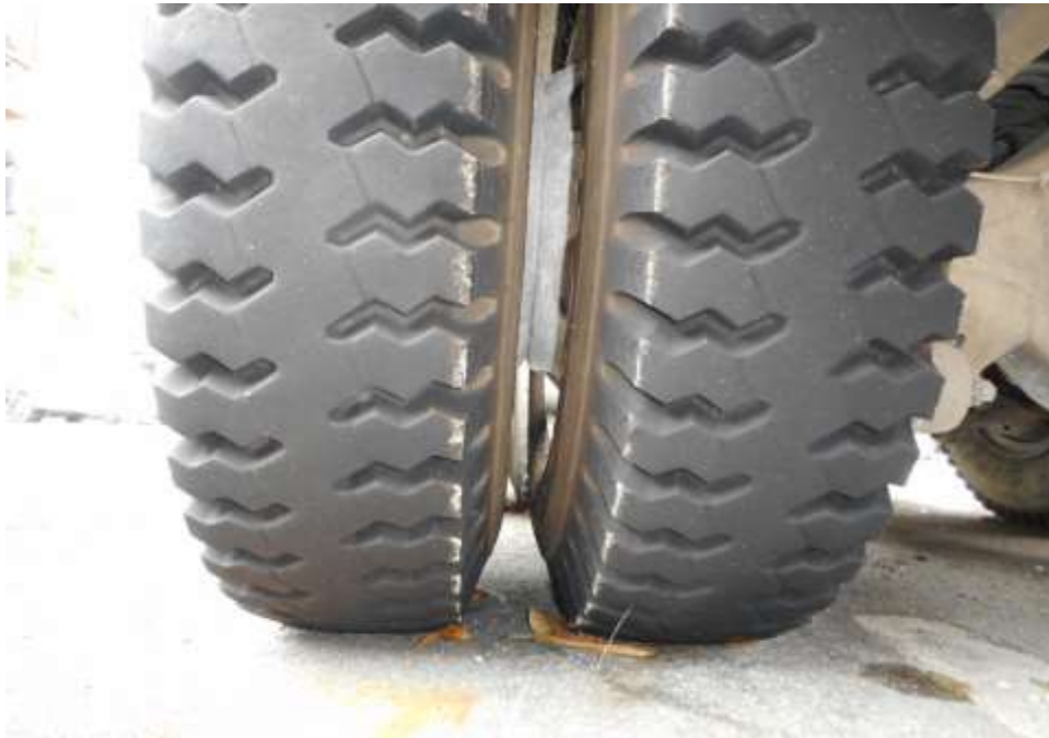
Photo 8 shows the condition of the rear left tyres of the Motor Lorry, which was observed to be in serviceable condition with remaining tread depth of approximately 11.8mm. The tyres, which were wrapped around standard steel wheel rim, were also observed to be sufficiently inflated for vehicular operation. There was also no damage found on all 10 steel wheel rims of the Motor Lorry.
