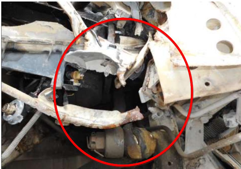
Photo 18 shows the steering box component (circled) at the undercarriage of the Motor Lorry was found to be damaged as a result of the accident.
