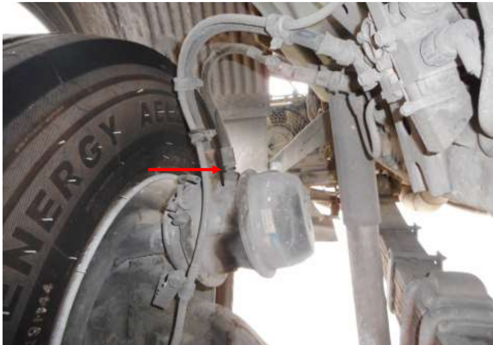
Photo 14 shows the brake pipe (arrowed) at the front left wheel of the Motor Lorry. I did not observe any leakage of brake fluid at the time of my inspection of the Motor Lorry. My static tests of the Motor Lorry's braking system, along with my visual examination of the various mechanical components in the braking system had indicated that there was no internal leakage of pressure/vacuum. Hence the braking system of the Motor Lorry was likely to be in serviceable condition at the material time of accident.
