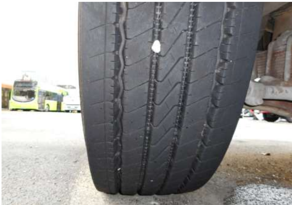
Photo 9 shows the condition of the front left tyres of the Motor Lorry, which were observed to be in serviceable condition with remaining tread depth of approximately 11.1mm.
