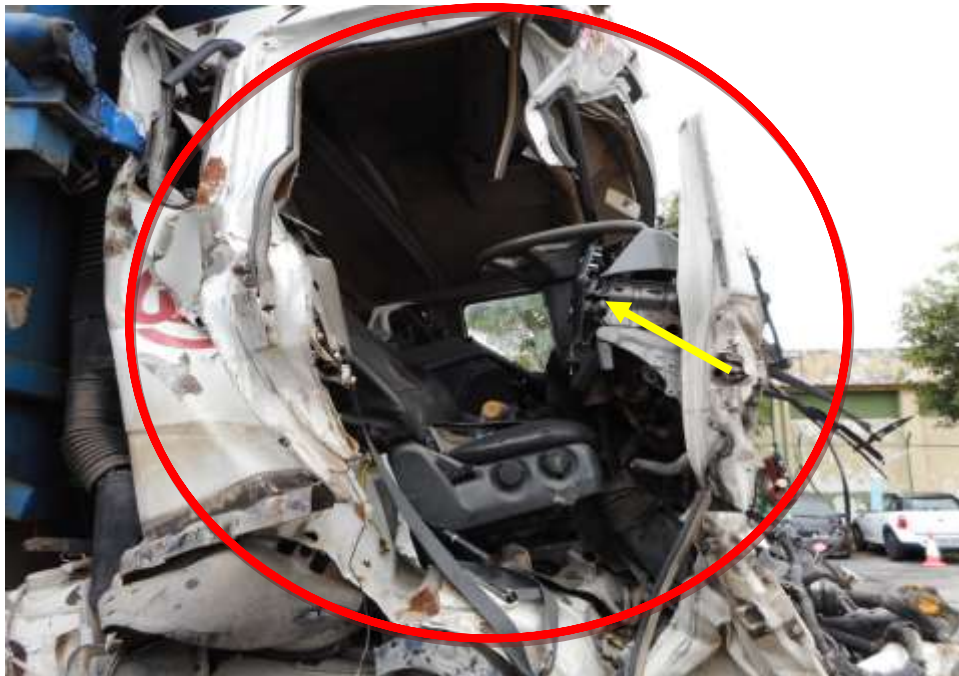
Photo 3 shows a close up view of the front right body of the Motor Lorry at the time of my inspection. Its whole front cabin, front right door (circled) and steering system (yellow arrow) were damaged as a result of the accident
