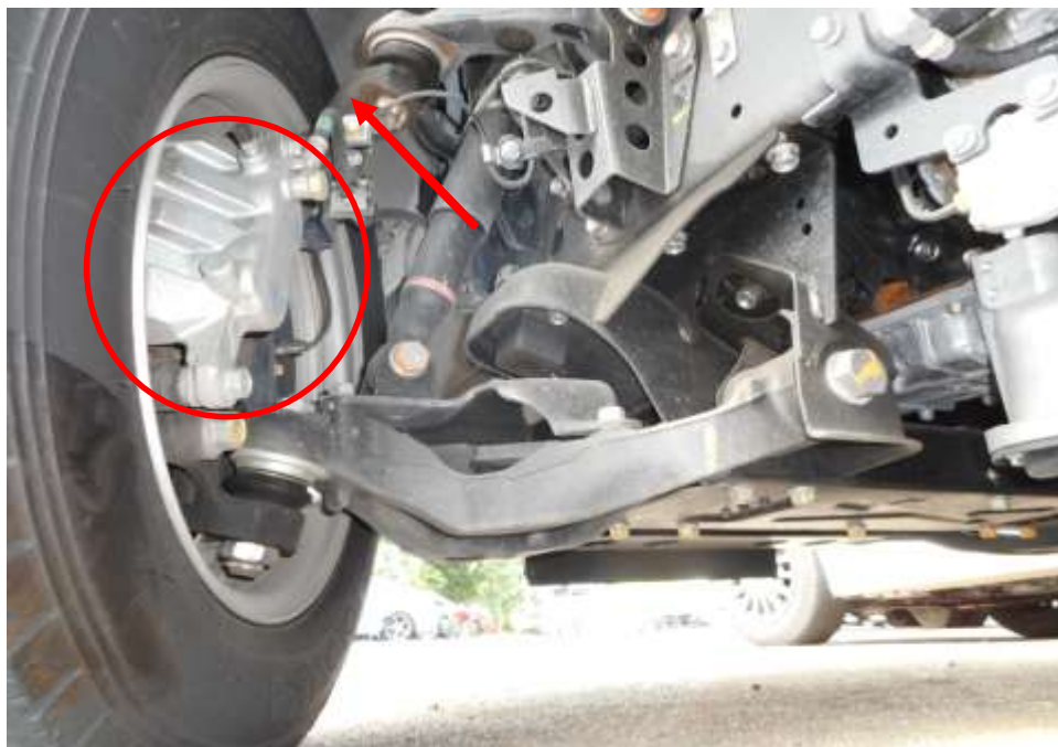
Photo 21 shows the brake hose/pipe (arrowed) at the front left wheel of the Motor Lorry. No leakage of brake fluid was observed. Visual examination of the various components of the braking system like the brake caliper (circled), brake booster, brake pedal etc had revealed all to be intact and without visible damage at the time of accident. There was also no sign of fluid stain(s) observed on the various undercarriage components.
