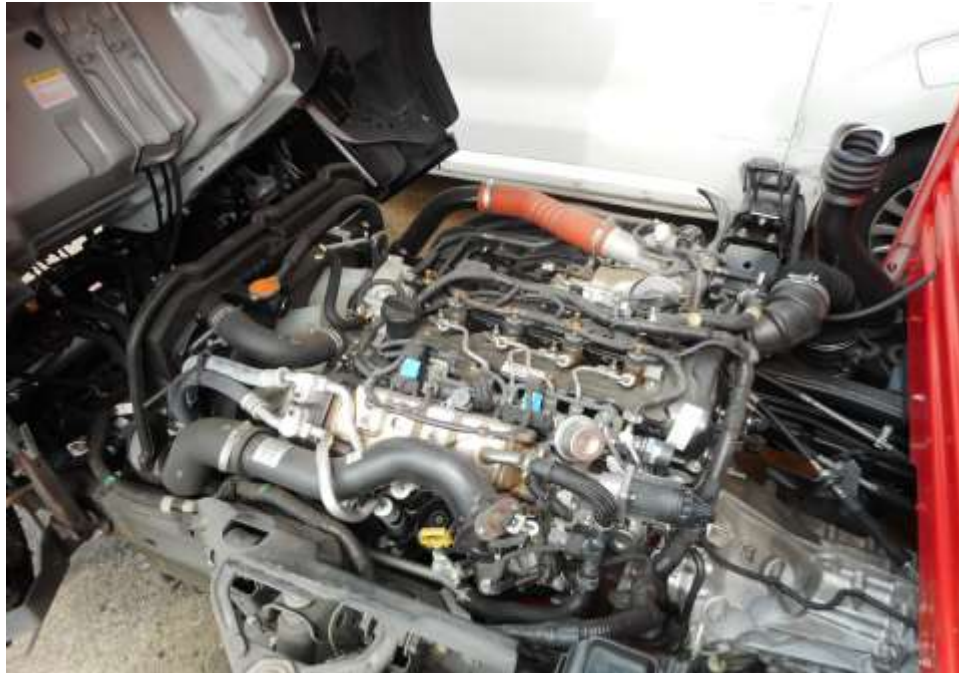
Photo 10 shows a general view of the Motor Lorry's engine compartment, which was accessed by lifting the front cabin of the Motor Lorry. The various parts and components inside the engine compartment were unaffected by the accident. There was also no sign(s) or indication(s) of fresh fluid leakage and/or fluid stain within the engine compartment (photograph shows the engine compartment as viewed from the left front side of the Motor Lorry).
