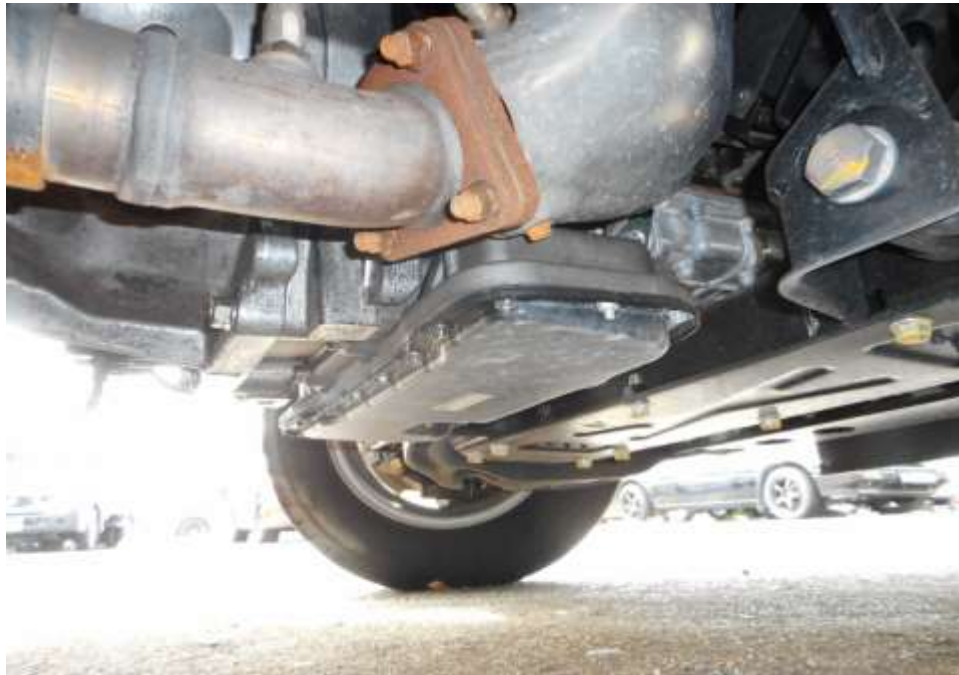
Photo 15 shows the undercarriage of the Motor Lorry, at the area where the engine housing and transmission housing are located. I did not find any sign(s) or indication(s) of fluid leak and/or fluid stain(s) on the underside of the Motor Lorry.
