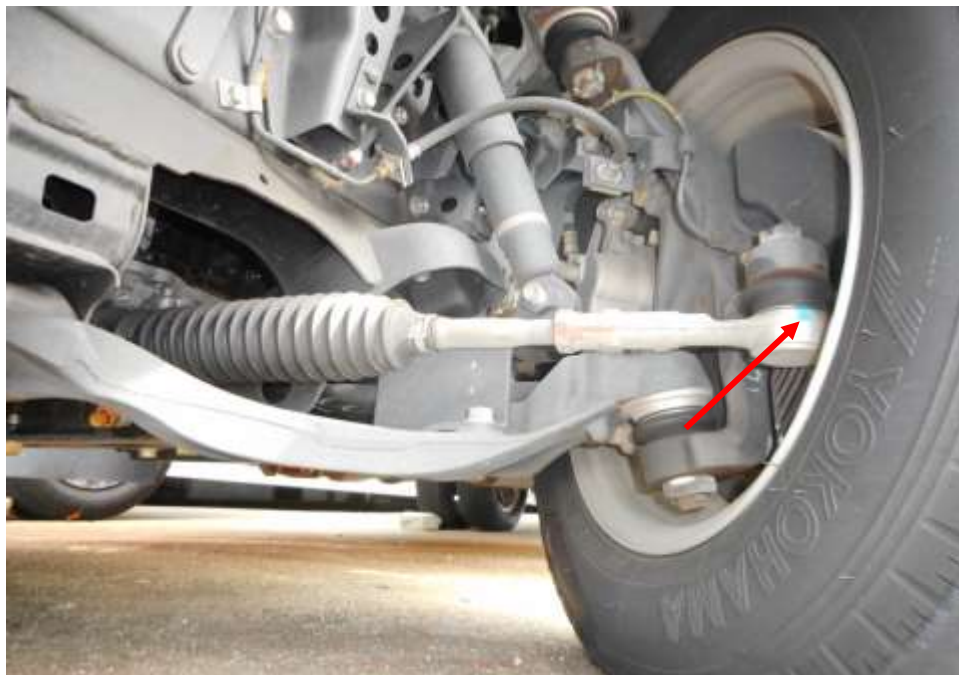
Photo 17 shows the various undercarriage components at the front left wheel of the Motor Lorry, in particular the steering tie rod end (arrowed). The various Undercarriage components of the Motor Lorry were all found to be intact without any visible damage. There was also no sign of fluid stain(s) observed on the various undercarriage components.
