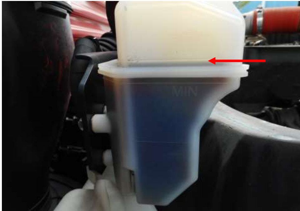
Photo 13 shows the power steering fluid reservoir of the Motor Lorry at the time of my inspection. The power steering fluid was observed to be of sufficient level (arrowed) and without any visible contamination.
