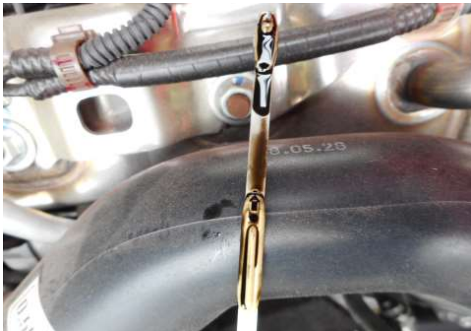
Photo 14 shows the engine dip stick of the Motor Lorry at the time of my inspection. The engine oil was observed to be of sufficient level and without any visible contamination.
