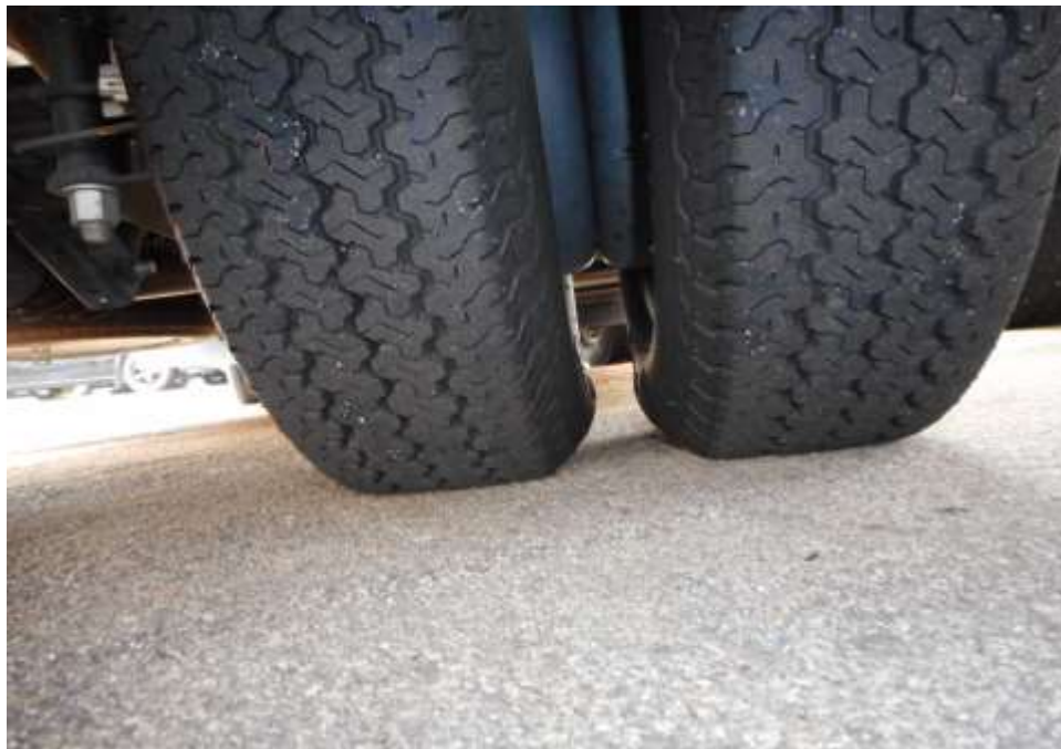
Photo 7 shows the condition of the rear right tyre of the Motor Lorry, which was observed to be in serviceable condition with remaining tread depth of approximately 6mm. The tyre, which was wrapped around standard steel wheel rim, was also observed to be sufficiently inflated for vehicular operation.
