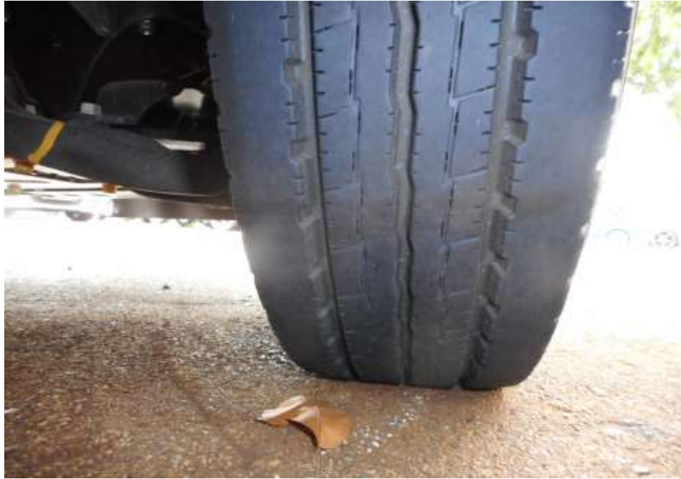
Photo 6 shows the condition of the front right tyre of the Motor Lorry, which was observed to be in serviceable condition with remaining tread depth of approximately 7.5mm. The tyre, which was wrapped around standard steel wheel rim, was also observed to be sufficiently inflated for vehicular operation. There was no tear, cut or burst mark(s) on the outer and the inner sidewalls as well as across the tread of the 6 tyres that were fitted on the Motor Lorry.
