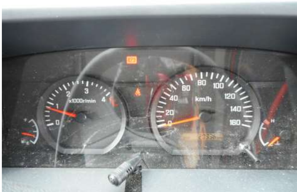
Photo 24 shows no warning lights illuminated on the instrument panel of the Motor Lorry after the engine was cranked. This would suggest that there was no abnormality to the electronic operating systems of the Motor Lorry, like the ABS and Traction Control (TC).
