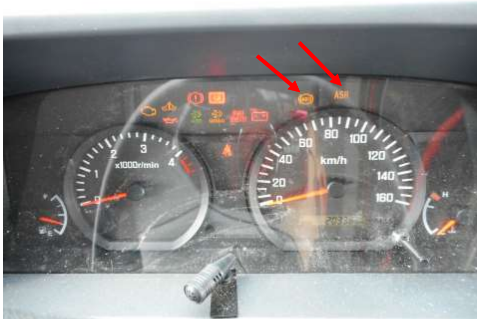
Photo 23 shows the warning light for Anti-Lock Brake System (ABS) and Traction Control (TC) (arrowed) appearing on the instrument panel of the Motor Lorry during the self-test of its various electronic operating systems when its engine was cranked.
