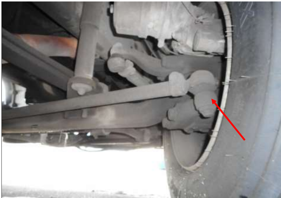
Photo 21 shows the various undercarriage components at the front right wheel of the Garbage truck, in particular the steering tie rod end (arrowed). The various steering components were all found to be intact, suggesting that the steering system of the Garbage truck was likely to be in serviceable condition at the material time of accident. There was also no sign of fluid stain(s) observed on the various undercarriage components.
