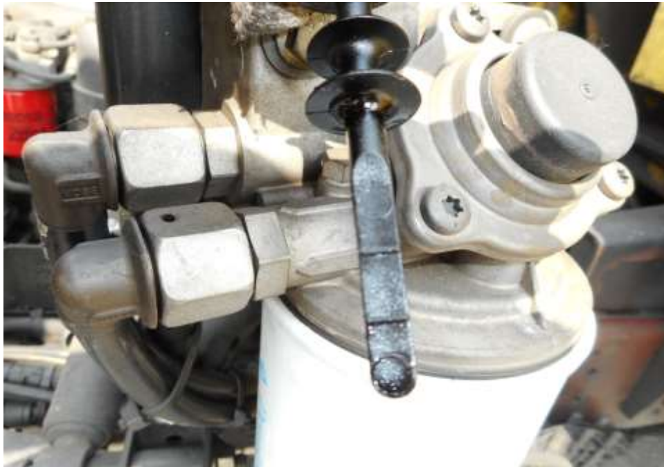
Photo 13 shows the power steering fluid dip stick of the Garbage truck at the time of my inspection. The power steering fluid was observed to be of low level and without any visible contamination.
