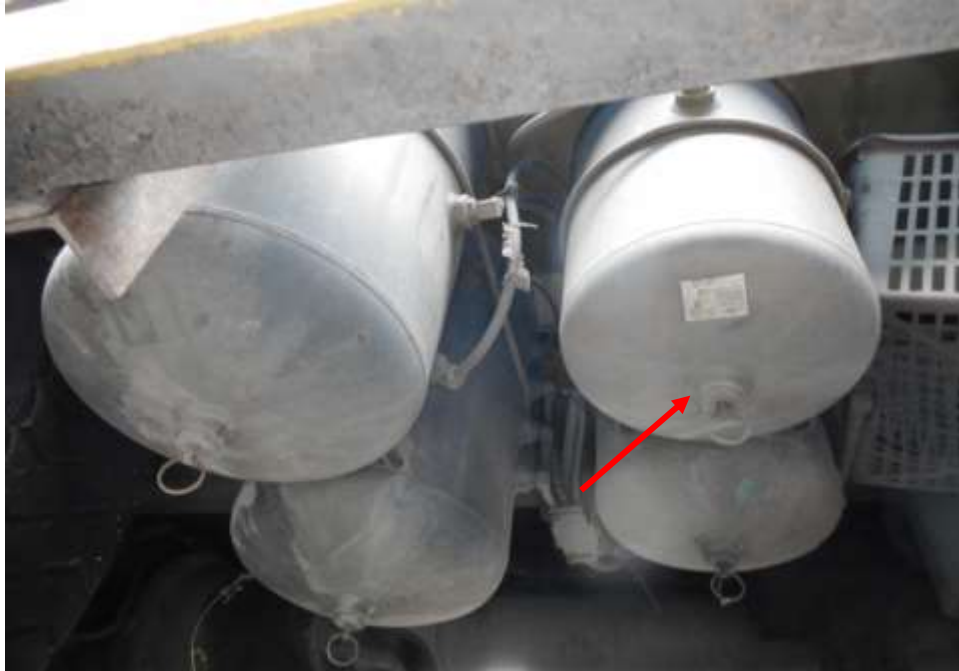
Photo 20 shows the air brake cylinder (arrowed) at the undercarriage of the Garbage truck. I did not observe any leakage of air brake fluid at the time of my inspection of the Garbage truck. My static tests of the Garbage truck's braking system, along with my visual examination of the various mechanical components in the braking system had indicated that there was no internal leakage of pressure/vacuum. Hence the braking system of the Garbage truck was likely to be in serviceable condition at the material time of accident.
