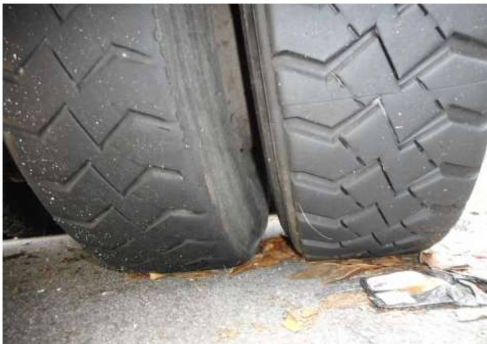
Photo 7 shows the condition of the rear right tyre of the Garbage truck, which was observed to be in serviceable condition with remaining tread depth of approximately 11mm. The tyre, which was wrapped around standard steel wheel rim, was also observed to be sufficiently inflated for vehicular operation.
