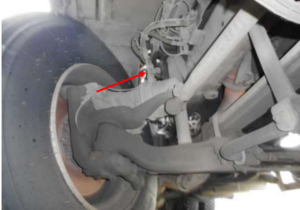
Photo 18 shows the brake pipe (arrowed) at the front right wheel of the Garbage truck. I did not observe any leakage of brake fluid at the time of my inspection of the Garbage truck. My static tests of the Garbage truck's braking system, along with my visual examination of the various mechanical components in the braking system, had indicated that there was no internal leakage of pressure/vacuum. Hence the braking system of the Garbage truck was likely to be in serviceable condition at the material time of accident.
