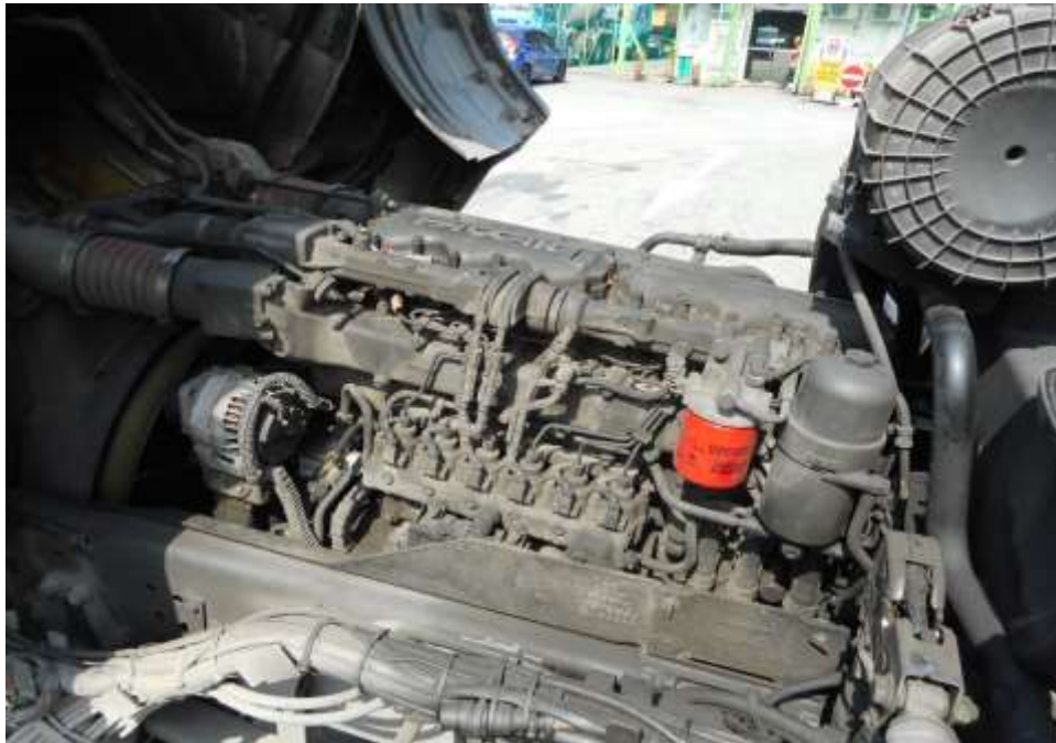
Photo 10 shows a general view of the Garbage truck's engine compartment, which was accessed by lifting the front cabin of the Garbage truck. The various parts and components inside the engine compartment were unaffected by the accident. There was also no sign(s) or indication(s) of fresh fluid leakage and/or fluid stain within the engine compartment
