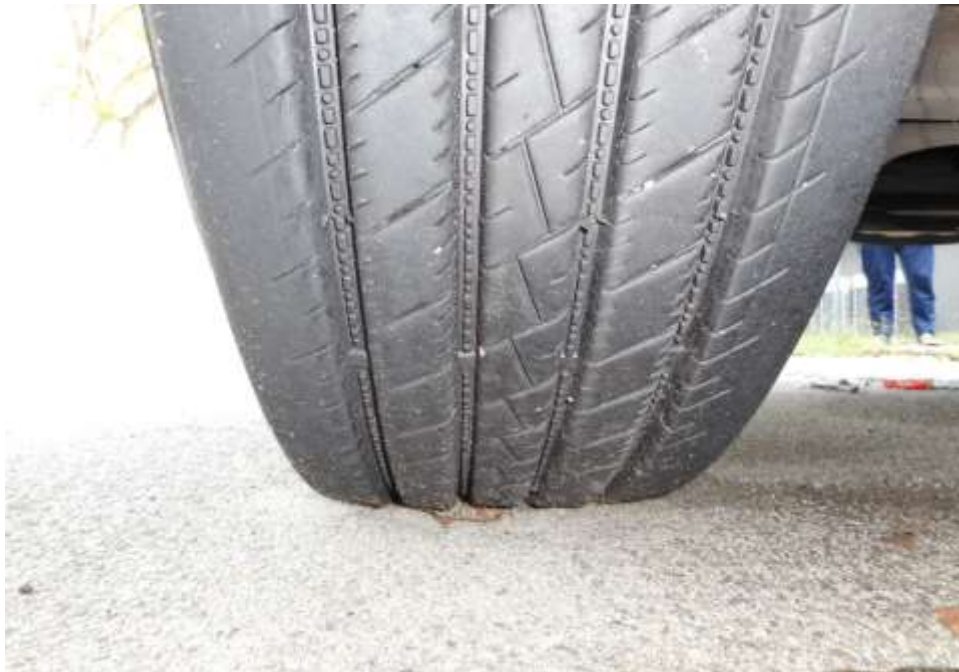
Photo 9 shows the condition of the front left tyres of the Garbage truck, which were observed to be in serviceable condition with remaining tread depth of approximately 10.3mm. There was also no tear, cut or burst mark(s) on the outer and the inner sidewalls as well as across the tread of the 10 tyres that were fitted on the Garbage truck.
