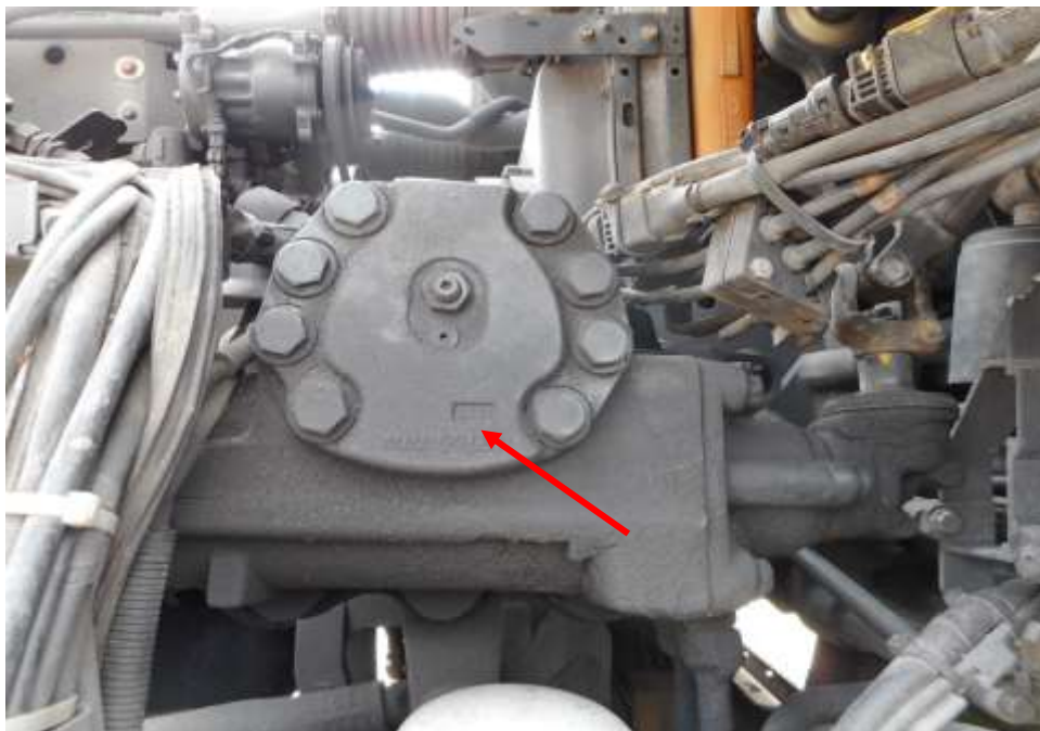
Photo 23 shows the steering box component (arrowed) at the undercarriage of the Garbage truck was found to be intact without any visible damage. There was also no sign of fluid stain(s) observed on the various undercarriage components.
