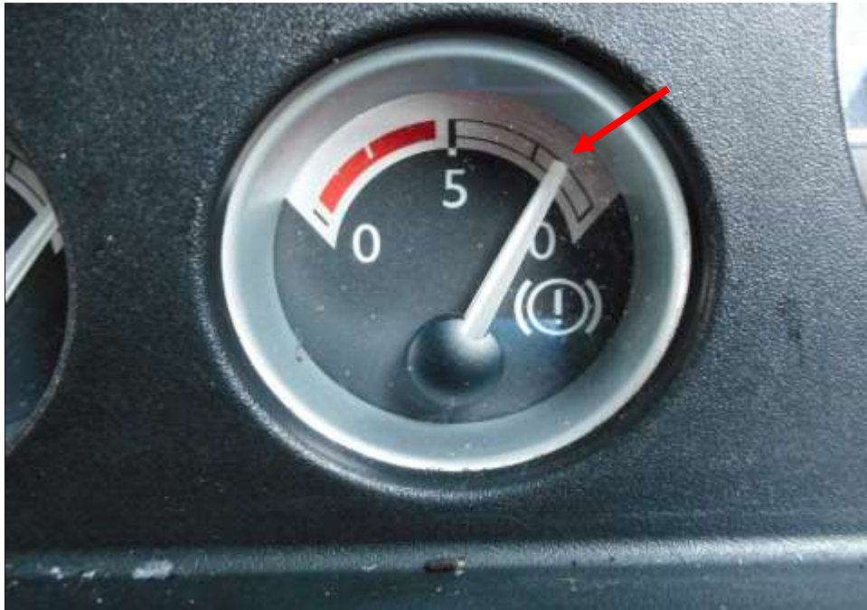
Photo 11 shows the air in the air brake cylinders of the Garbage truck at the time of my inspection. The air in the cylinder was observed to be of sufficient level & serviceable at the time of the accident.
