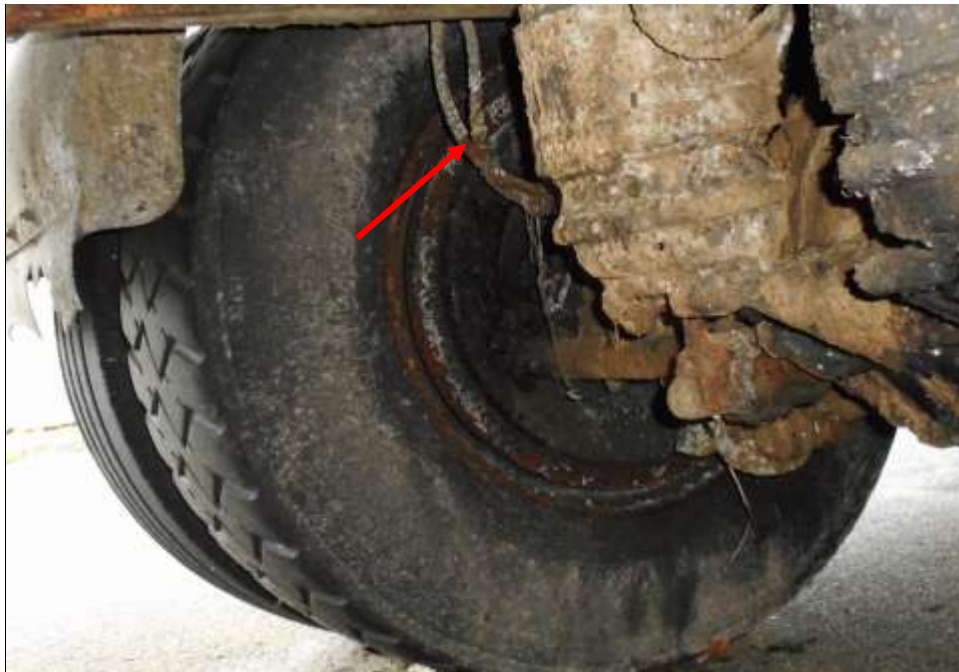
Photo 17 shows the brake pipe (arrowed) at the rear left wheel of the Garbage truck. I did not observe any leakage of brake fluid at the time of my inspection of the Garbage truck. My static tests of the Garbage truck's braking system, along with my visual examination of the various mechanical components in the braking system, had indicated that there was no internal leakage of pressure/vacuum. Hence the braking system of the Garbage truck was likely to be in serviceable condition at the material time of accident.
