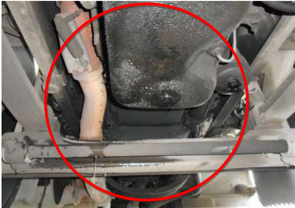
Photo 15 shows the undercarriage of the Garbage truck at the area where the engine housing located. Observed were fresh coolant fluid leakage and/or fluid stain(s) on the underside of the Garbage truck (circled)
