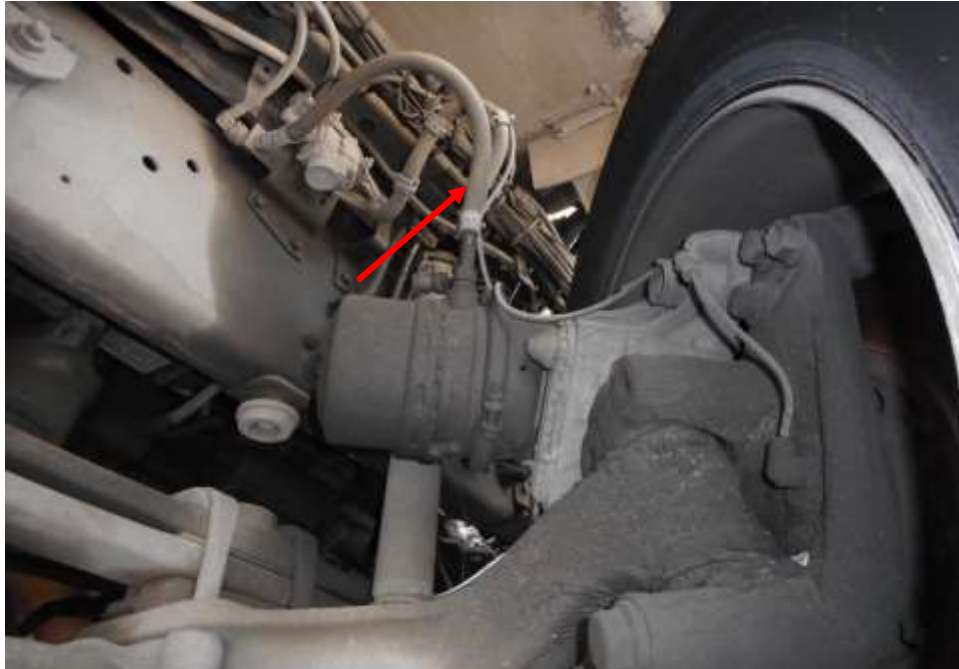
Photo 19 shows the brake pipe (arrowed) at the front left wheel of the Garbage truck. I did not observe any leakage of brake fluid at the time of my inspection of the Garbage truck. My static tests of the Garbage truck's braking system, along with my visual examination of the various mechanical components in the braking system had indicated that there was no internal leakage of pressure/vacuum. Hence the braking system of the Garbage truck was likely to be in serviceable condition at the material time of accident.
