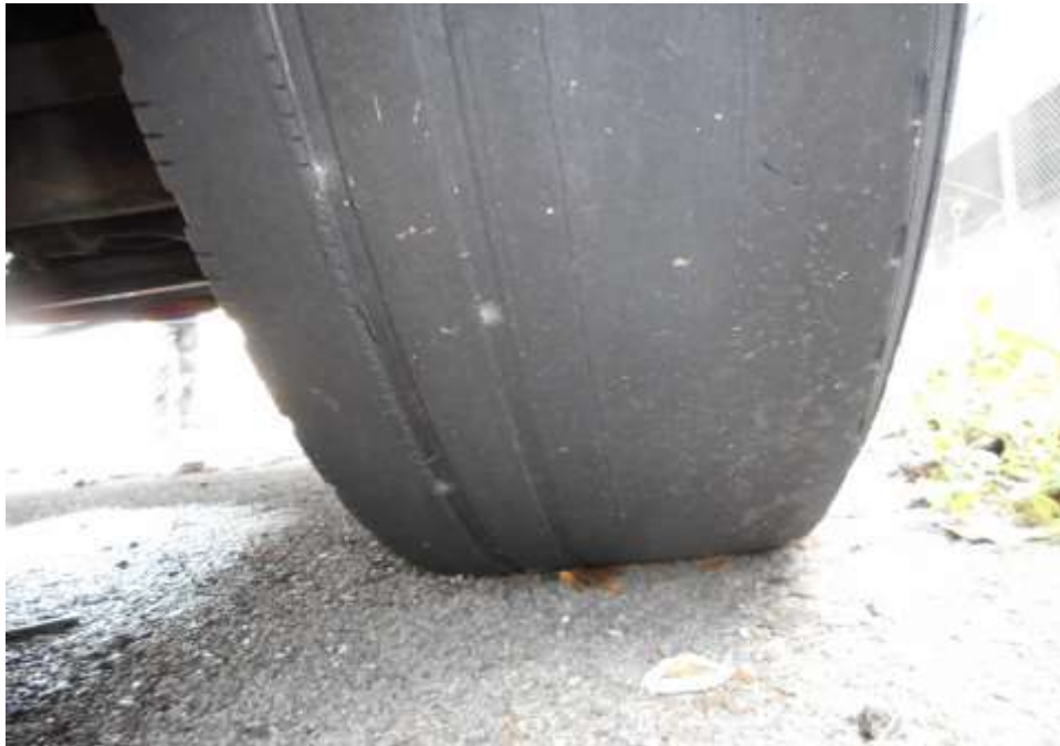
Photo 6 shows the condition of the front right tyre of the Garbage truck, which was observed to be in unserviceable condition with remaining tread depth of approximately 0 mm. The tyre, which was wrapped around standard steel wheel rim, was also observed to be sufficiently inflated for vehicular operation. There was no tear, cut or burst mark(s) on the outer and the inner sidewalls as well as across the tread of the 10 tyres that were fitted on the Garbage truck.
