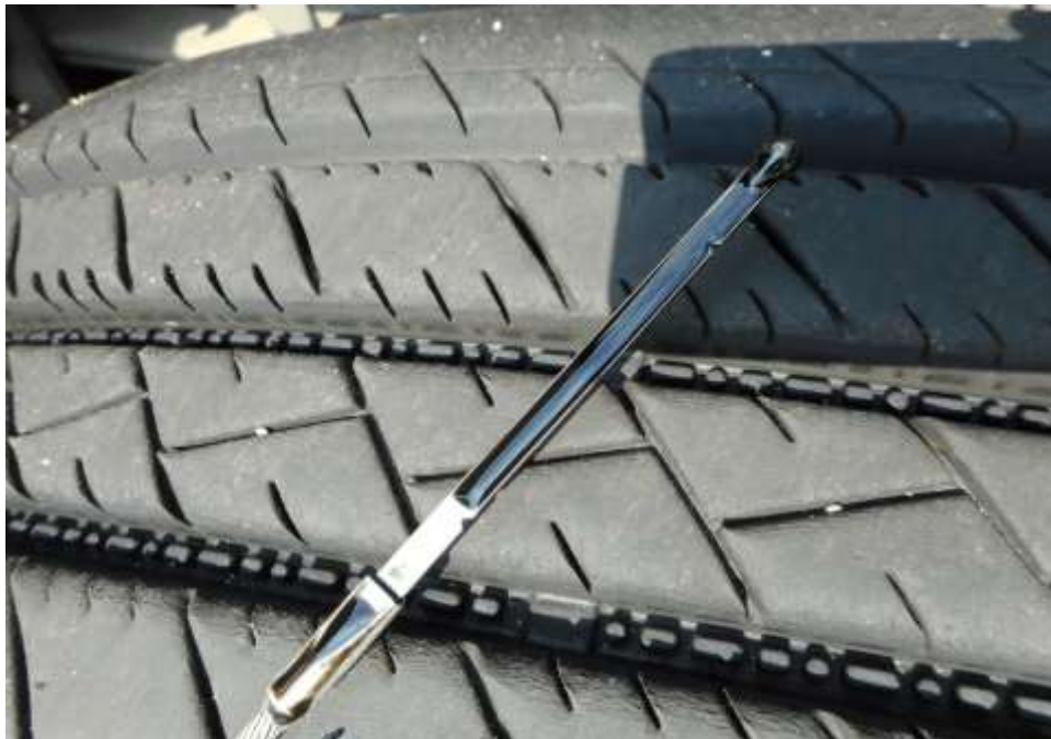
Photo 12 shows the engine oil dip stick of the Garbage truck at the time of my inspection. The engine oil was observed to be of sufficient level and without any visible contamination.
