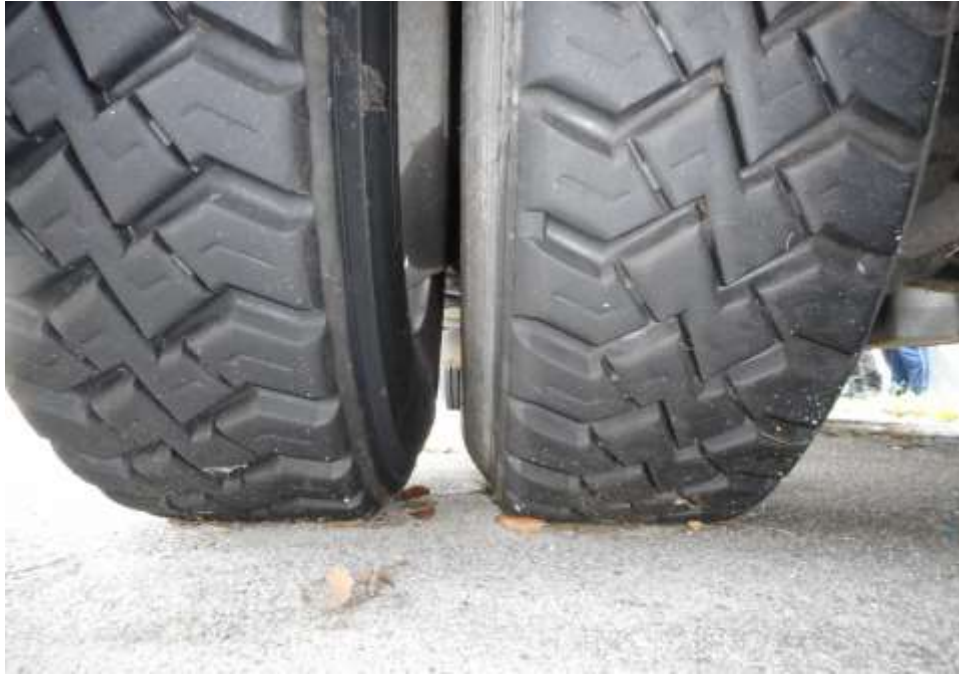
Photo 8 shows the condition of the rear left tyres of the Garbage truck, which was observed to be in serviceable condition with remaining tread depth of approximately 9.8mm. The tyres, which were wrapped around standard steel wheel rim, were also observed to be sufficiently inflated for vehicular operation. There was also no damage found on all 10 steel wheel rims of the Garbage truck.
