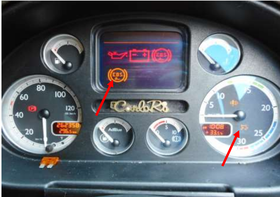
Photo 25 shows the warning light for Anti-Lock Brake System (ABS) and Traction Control System (TC) (arrowed) appearing on the instrument panel of the Garbage truck during the self-test of its various electronic operating systems when its engine was cranked.
