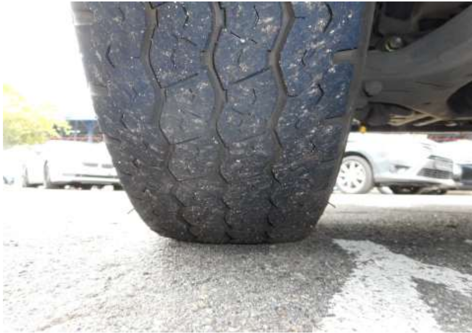
Photo 10 shows the condition of the rear right tyres of the Motor Van, which were observed to be in serviceable condition with remaining, tread depth of approximately 5.4mm. There was also no tear, cut or burst mark(s) on the outer and the inner sidewalls as well as across the tread of the 4 tyres that were fitted on the Motor Van.
