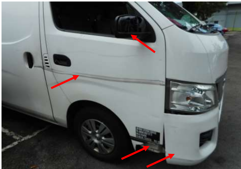
Photo 3 shows a close up view of the Motor Van's right portion at the time of my inspection. The Motor Van sustained moderate damage at its front right portion. Its front right door, right rear view mirror and front bumper (arrowed) were damage at the time of my inspection as a result of the accident.
