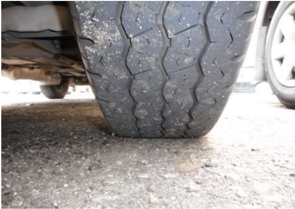
Photo 8 shows the condition of the rear right tyre of the Motor Van, which was observed to be in serviceable condition with remaining tread depth of approximately 4.7mm. The tyre, which was wrapped around standard steel wheel rim, was also observed to be sufficiently inflated for vehicular operation.
