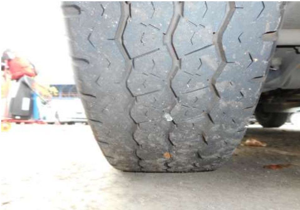
Photo 9 shows the condition of the rear left tyres of the Motor Van, which was observed to be in serviceable condition with remaining tread depth of approximately 4.6mm. The tyres, which were wrapped around standard steel wheel rim, were also observed to be sufficiently inflated for vehicular operation. There was also no damage found on all 4 steel wheel rims of the Motor Van.
