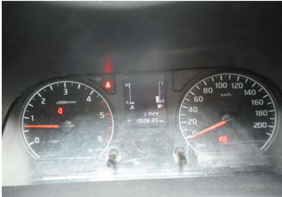
Photo 24 shows no warning lights illuminated on the instrument panel of the Motor Van after the engine was cranked. This would suggest that there was no abnormality to the various electronic operating systems of the Motor Van, like the ABS and SRS...Etc
