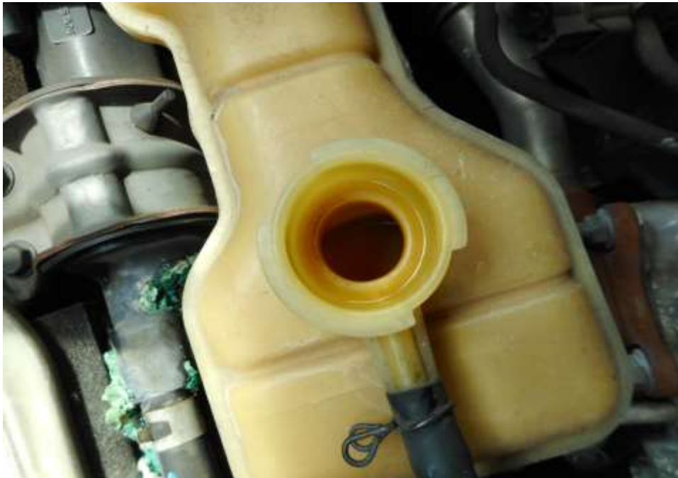
Photo 13 shows the engine coolant reservoir of the Motor Van at the time of my inspection. The engine coolant was observed to be of sufficient level and without any visible contamination.
