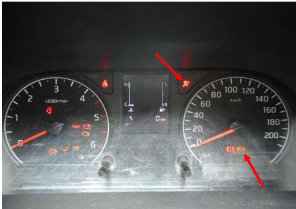
Photo 23 shows the warning light for Anti-Lock Brake System (ABS) and Supplemental Restraint System (SRS) appearing on the instrument panel of the Motor Van during the self-test of its various electronic operating systems when its engine was cranked.
