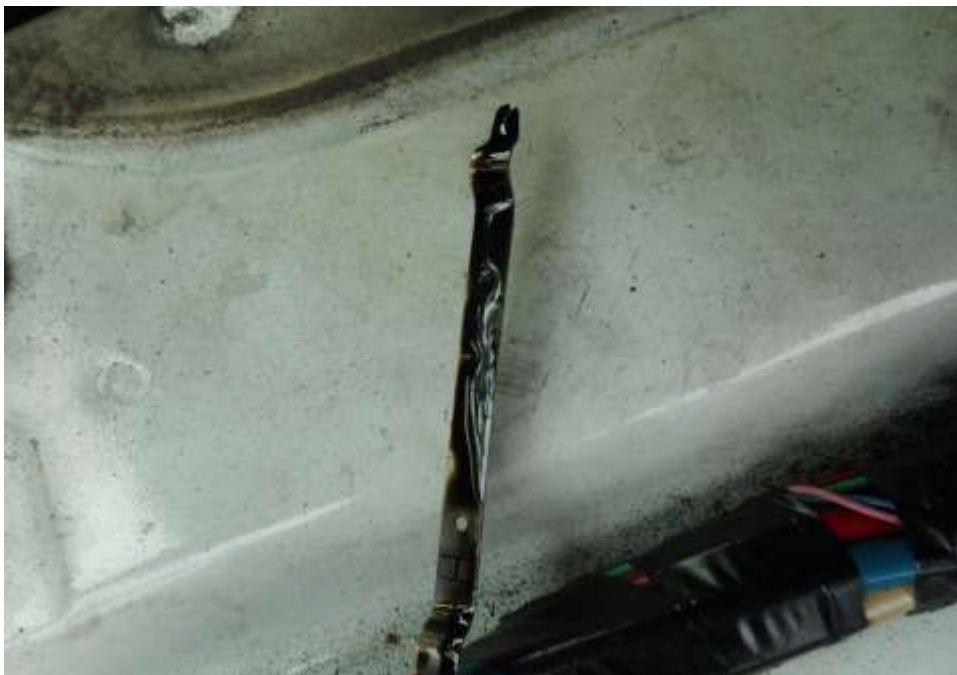
Photo 14 shows the engine dip stick of the Motor Van at the time of my inspection. The engine oil was observed to be of sufficient level and without any visible contamination.
