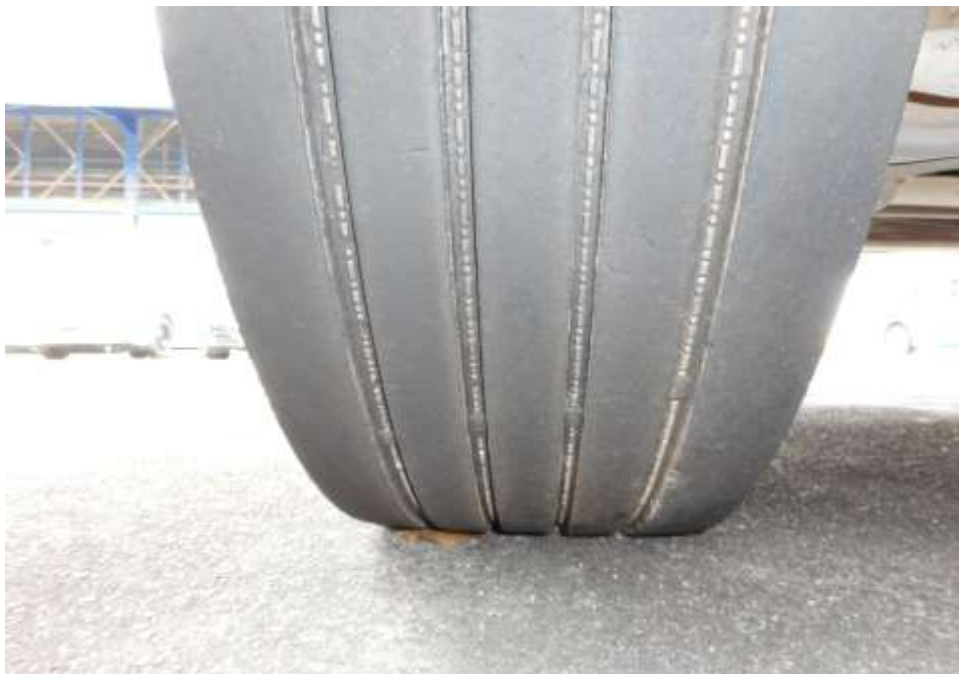
Photo 9 shows the condition of the front left tyres of the Tipper Lorry, which were observed to be in serviceable condition with remaining tread depth of approximately 8.3mm. There was also no tear, cut or burst mark(s) on the outer and the inner sidewalls as well as across the tread of the 10 tyres that were fitted on the Tipper Lorry.
