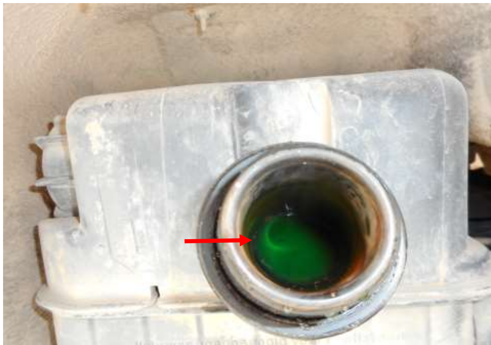
Photo 12 shows the engine coolant reservoir of the Tipper Lorry at the time of my inspection. The engine coolant was observed to be of sufficient level (arrowed) and without any visible contamination.
