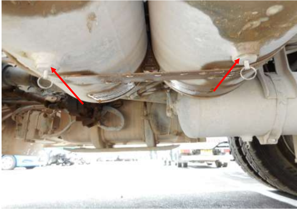
Photo 20 shows the air brake cylinders (arrowed) at the undercarriage of the Tipper Lorry. I did not observe any leakage of air brake fluid at the time of my inspection of the Tipper Lorry. My static tests of the Tipper Lorry's braking system, along with my visual examination of the various mechanical components in the braking system had indicated that there was no internal leakage of pressure/vacuum. Hence the braking system of the Tipper Lorry was likely to be in serviceable condition at the material time of accident.
