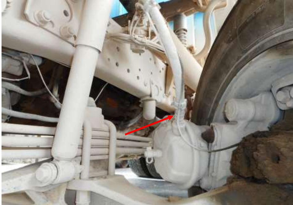
Photo 18 shows the brake pipe (arrowed) at the front left wheel of the Tipper Lorry. I did not observe any leakage of brake fluid at the time of my inspection of the Tipper Lorry. My static tests of the Tipper Lorry's braking system, along with my visual examination of the various mechanical components in the braking system, had indicated that there was no internal leakage of pressure/vacuum. Hence the braking system of the Tipper Lorry was likely to be in serviceable condition at the material time of accident.
