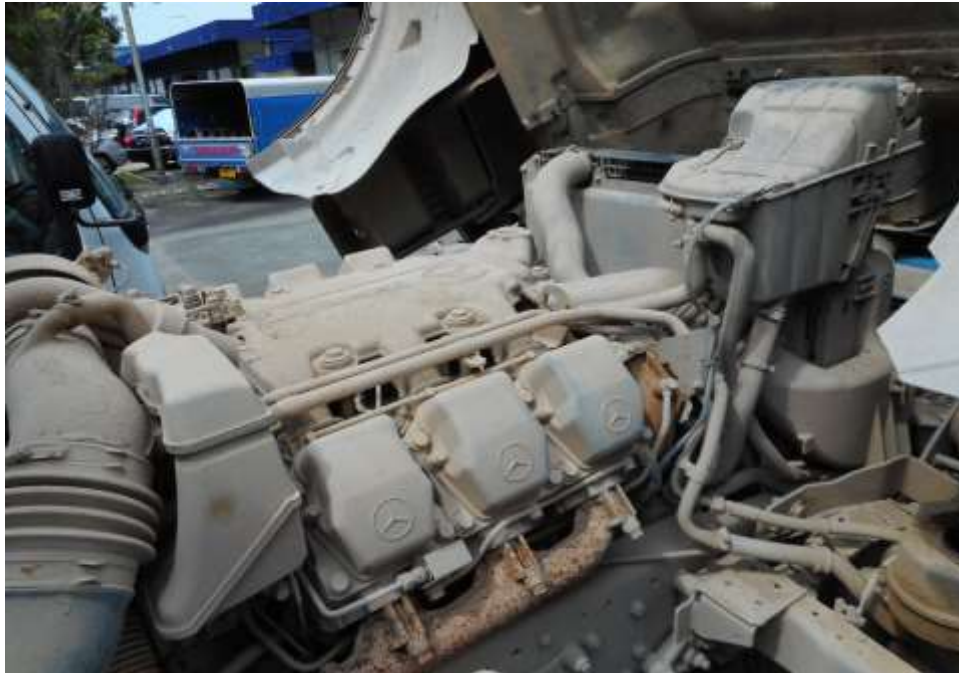
Photo 10 shows a general view of the Tipper Lorry's engine compartment, which was accessed by lifting the front cabin of the Tipper Lorry. The various parts and components inside the engine compartment were unaffected by the accident. There was also no sign(s) or indication(s) of fresh fluid leakage and/or fluid stain within the engine compartment
