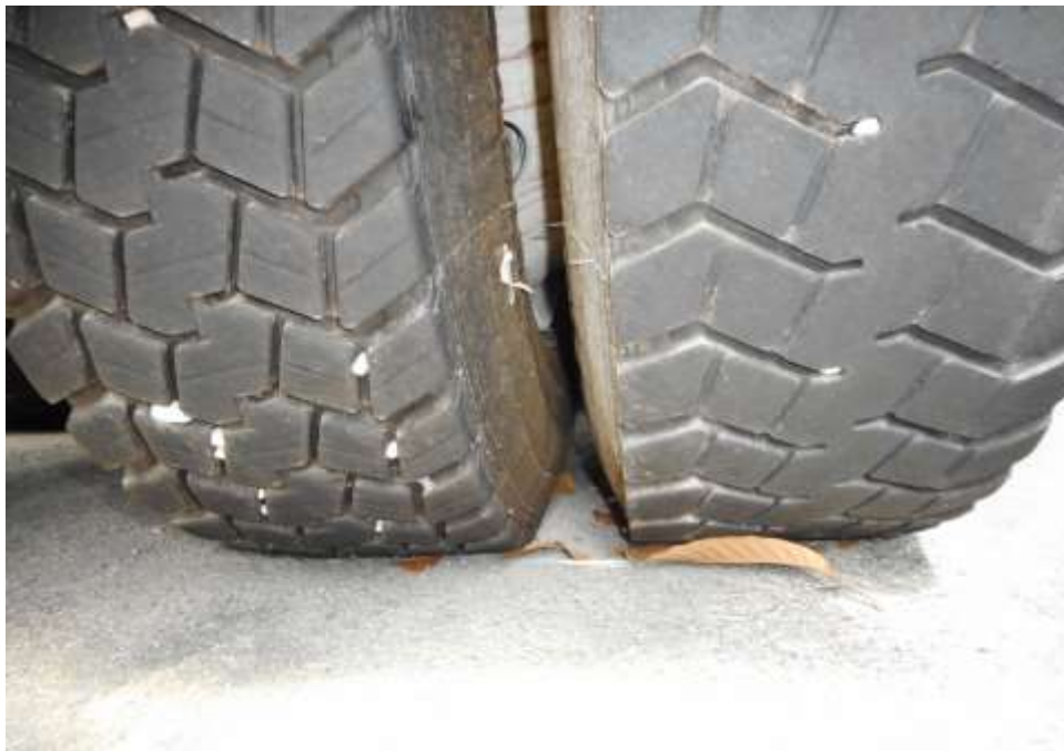
Photo 7 shows the condition of the rear right tyre of the Tipper Lorry, which was observed to be in serviceable condition with remaining tread depth of approximately 10.7mm. The tyre, which was wrapped around standard steel wheel rim, was also observed to be sufficiently inflated for vehicular operation.
