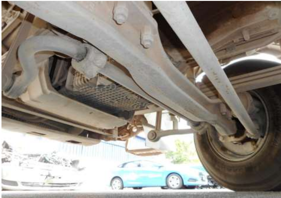
Photo 15 shows the undercarriage of the Tipper Lorry, at the area where the engine housing located. I did not find any sign(s) or indication(s) of fluid leak and/or fluid stain(s) on the underside of the Tipper Lorry.
