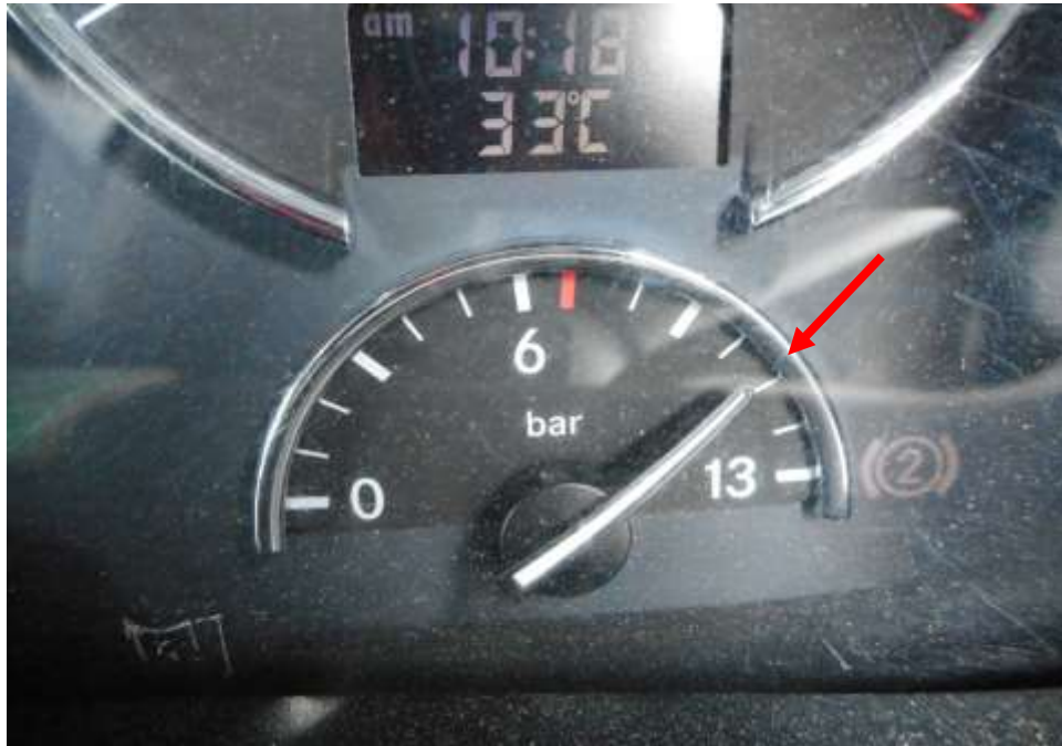
Photo 11 shows the air in the air brake cylinders of the Tipper Lorry at the time of my inspection. The air in the cylinder was observed to be of sufficient level & serviceable at the time of the accident.
