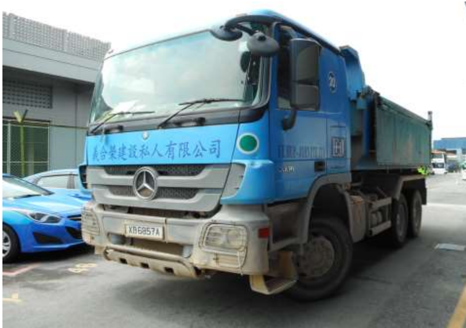
Photo 24 shows the front left wheel of the Tipper Lorry turned to its full right. During my steering system test, I did not experience any abnormal free play and/or resistance when I had turned the steering wheel towards full left and full right. This would suggest that the steering system of the Tipper Lorry was likely to be in serviceable condition at the material time of accident.
