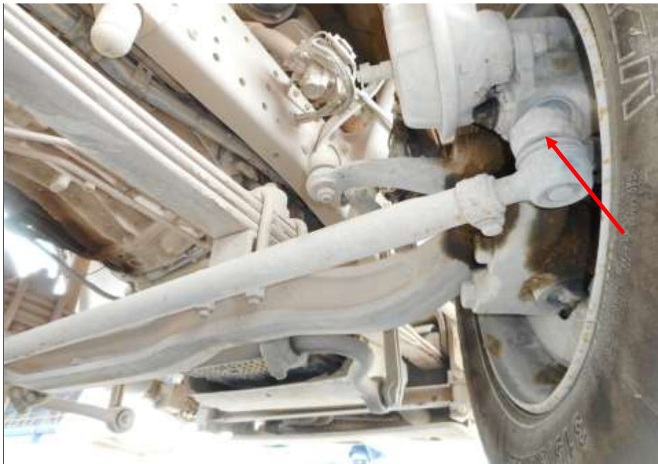
Photo 21 shows the various undercarriage components at the front right wheel of the Tipper Lorry, in particular the steering tie rod end (arrowed). The various steering components were all found to be intact, suggesting that the steering system of the Tipper Lorry was likely to be in serviceable condition at the material time of accident. There was also no sign of fluid stain(s) observed on the various undercarriage components.
