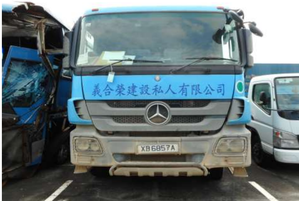
Photo 2 shows a general view of the front body of the Tipper Lorry at the time of my inspection. The Tipper Lorry was observed to not sustain any damage
