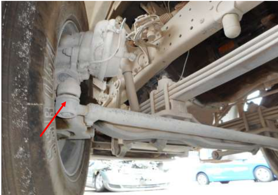
Photo 22 shows the various undercarriage components at the front left wheel of the Tipper Lorry, in particular the steering tie rod end (arrowed). The various undercarriage components of the Tipper Lorry were all found to be intact without any visible damage. There was also no sign of fluid stain(s) observed on the various undercarriage components.
