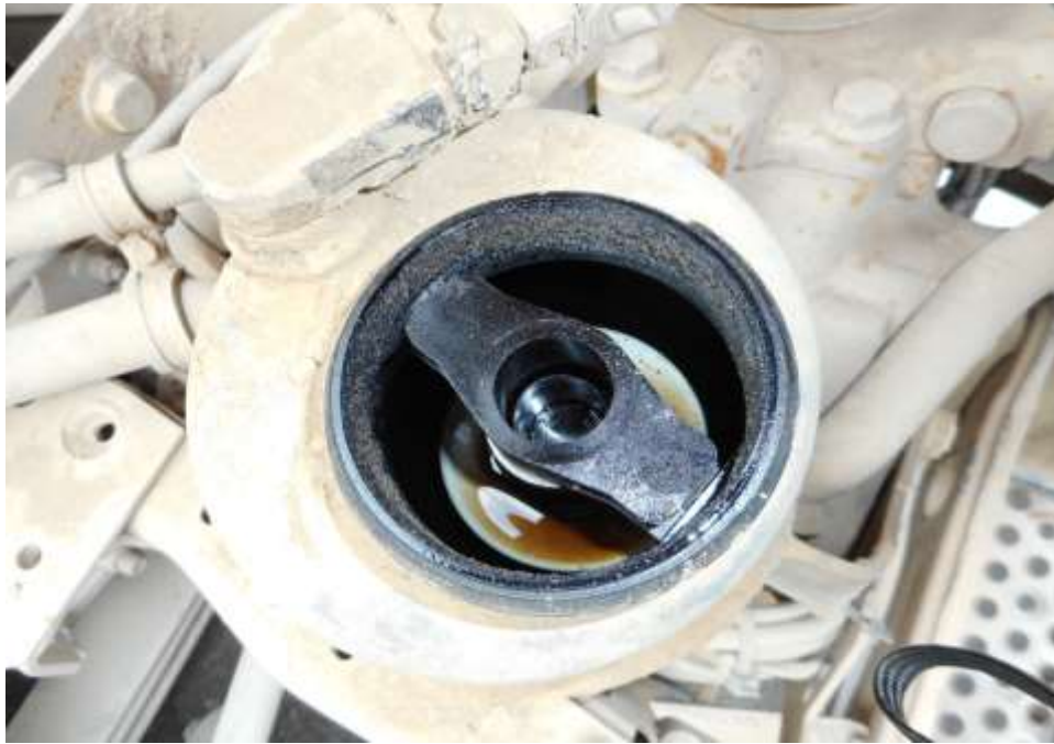
Photo 13 shows the power steering fluid reservoir of the Tipper Lorry at the time of my inspection. The power steering fluid was observed to be of sufficient level and without any visible contamination.
