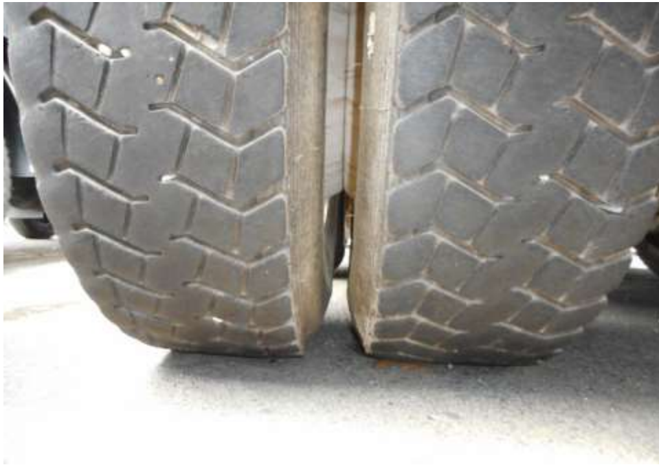
Photo 8 shows the condition of the rear left tyres of the Tipper Lorry, which was observed to be in serviceable condition with remaining tread depth of approximately 8.5mm. The tyres, which were wrapped around standard steel wheel rim, were also observed to be sufficiently inflated for vehicular operation. There was also no damage found on all 10 steel wheel rims of the Tipper Lorry.
