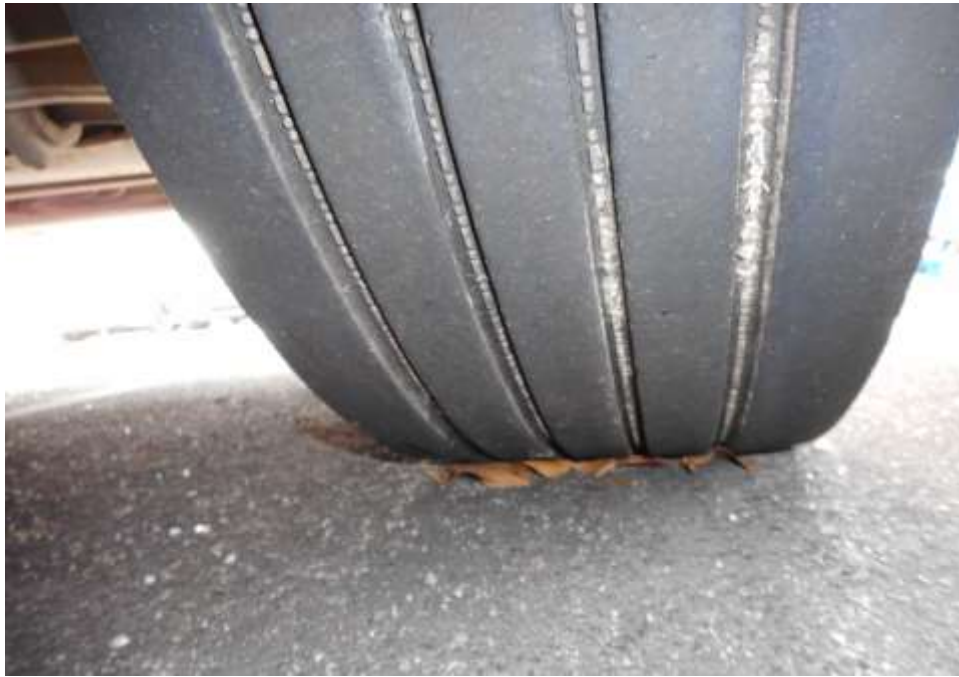
Photo 6 shows the condition of the front right tyre of the Tipper Lorry, which was observed to be in serviceable condition with remaining tread depth of approximately 7.7 mm. The tyre, which was wrapped around standard steel wheel rim, was also observed to be sufficiently inflated for vehicular operation. There was no tear, cut or burst mark(s) on the outer and the inner sidewalls as well as across the tread of the 10 tyres that were fitted on the Tipper Lorry.
