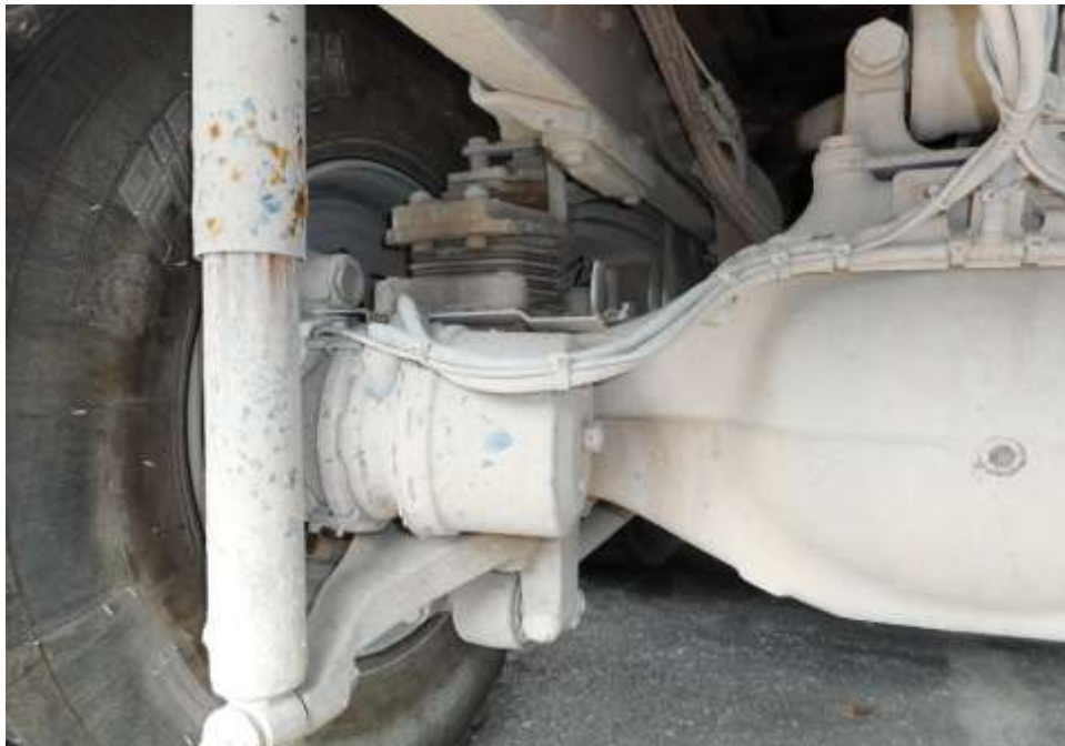
Photo 17 shows the brake pipe (arrowed) at the rear left wheel of the Tipper Lorry. I did not observe any leakage of brake fluid at the time of my inspection of the Tipper Lorry. My static tests of the Tipper Lorry's braking system, along with my visual examination of the various mechanical components in the braking system, had indicated that there was no internal leakage of pressure/vacuum. Hence the braking system of the Tipper Lorry was likely to be in serviceable condition at the material time of accident.
