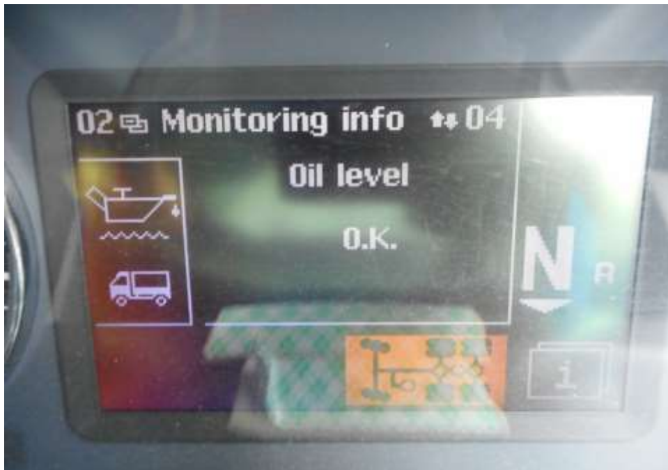
Photo 14 shows the engine oil level display of the Tipper Lorry at the time of my inspection. The engine oil was observed to be of sufficient level.
