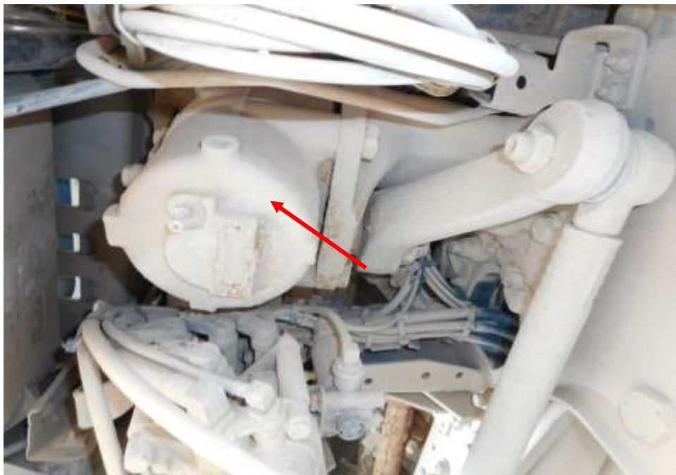
Photo 23 shows the steering box component (arrowed) at the undercarriage of the Tipper Lorry was found to be intact without any visible damage. There was also no sign of fluid stain(s) observed on the various undercarriage components.
