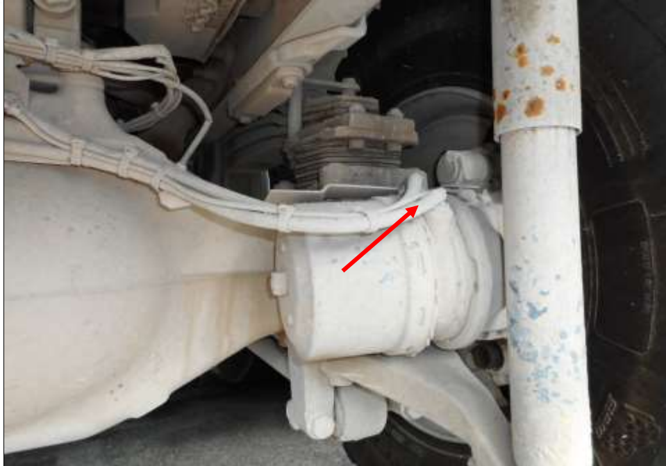
Photo 16 shows the brake pipe (arrowed) at the rear right wheel of the Tipper Lorry. I did not observe any leakage of brake fluid at the time of my inspection of the Tipper Lorry. My static tests of the Tipper Lorry's braking system, along with my visual examination of the various mechanical components in the braking system, had indicated that there was no internal leakage of pressure/vacuum. Hence the braking system of the Tipper Lorry was likely to be in serviceable condition at the material time of accident.
