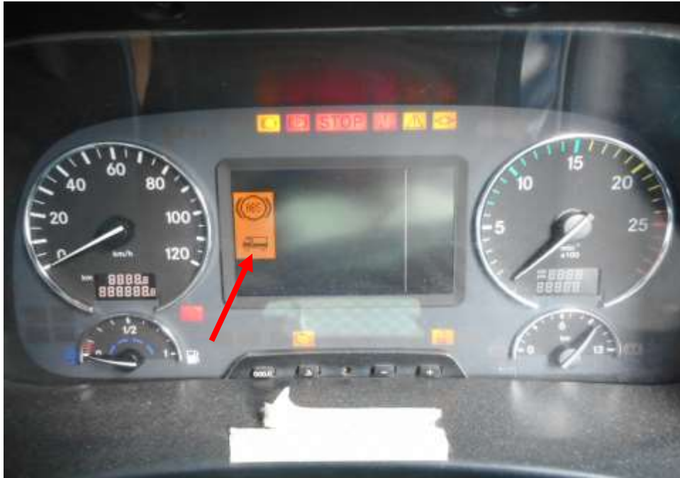
Photo 25 shows the warning light for Anti-Lock Brake System (ABS) (arrowed) appearing on the instrument panel of the Tipper Lorry during the self-test of its various electronic operating systems when its engine was cranked.
