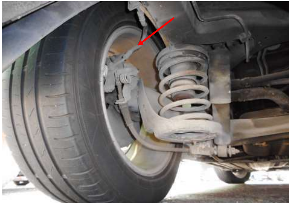
Photo 15 shows the brake hose/pipe (arrowed) at the rear left wheel of the Police Car. I did not observe any leakage of brake fluid at the time of my inspection of the Police Car. Static tests of the Police Car's braking system had indicated that there was no internal leakage of pressure/vacuum. The undercarriage components of the Police Car were also all found to be intact and without any visible damage.
