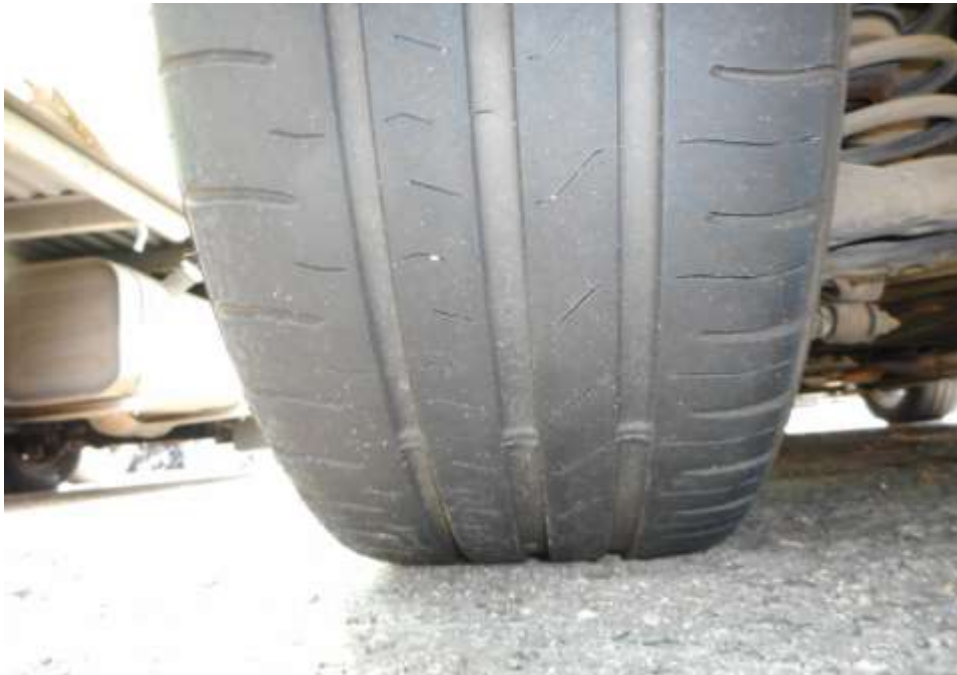
Photo 8 shows the condition of the rear left tyre of the Police Car, which was observed to be in serviceable condition with remaining tread depth of approximately 3.2mm. The tyre was also observed to be sufficiently inflated for vehicular operation with no tear, cut or burst mark(s).
