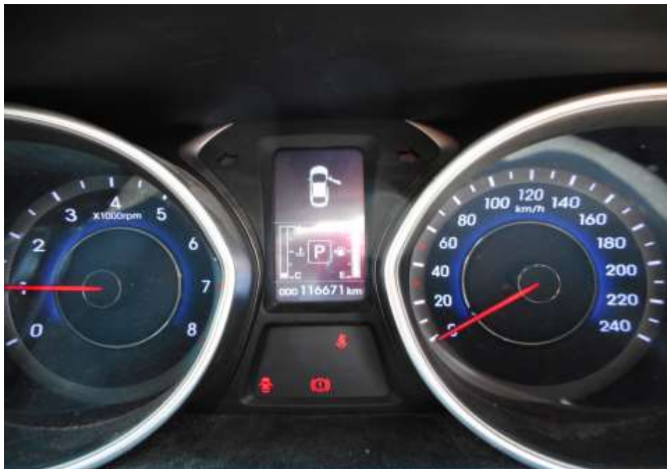
Photo 22 shows no warning lights illuminated on the instrument panel of the Police Car after the engine was cranked. This would suggest that there was no abnormality to the various electronic operating systems of the Police Car, like the ABS, EPS, SRS and TC etc.
