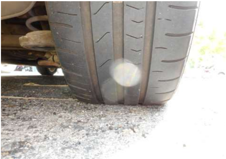
Photo 7 shows the condition of the rear right tyre of the Police Car, which was observed to be in serviceable condition with remaining tread depth of approximately 4.4mm. The tyre was also observed to be sufficiently inflated for vehicular operation with no tear, cut or burst mark(s).
