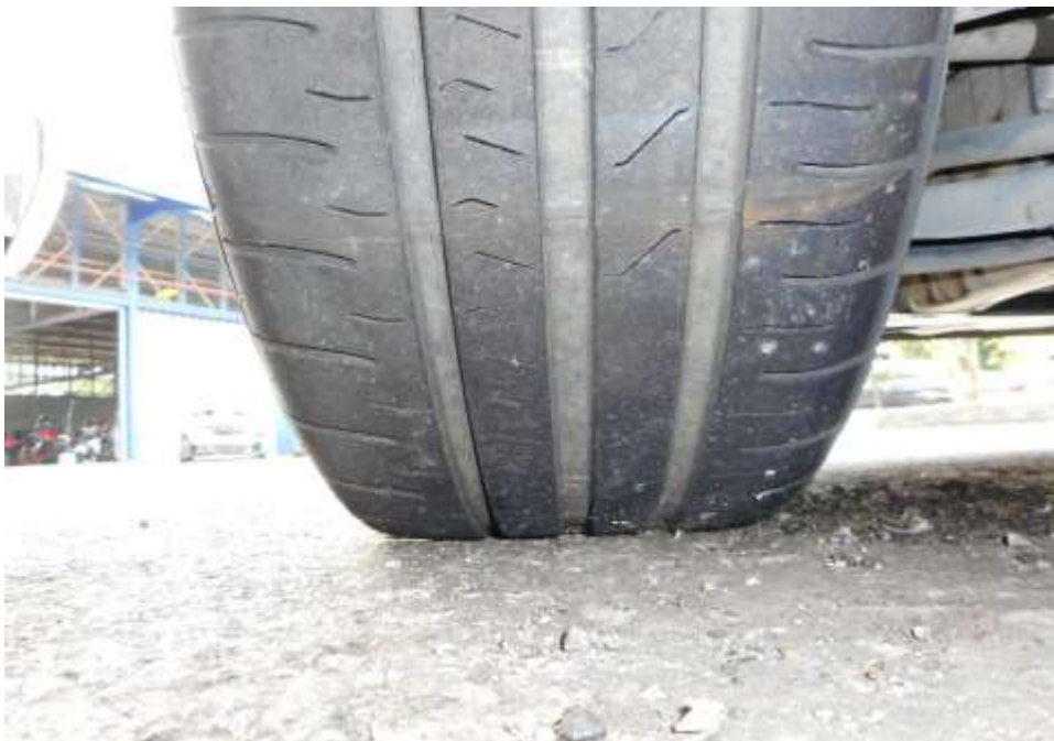
Photo 9 shows the condition of the front left tyre of the Police Car, which was observed to be in serviceable condition with remaining tread depth of approximately 4.3mm. The tyre was also observed to be sufficiently inflated for vehicular operation with no tear, cut or burst mark(s).
