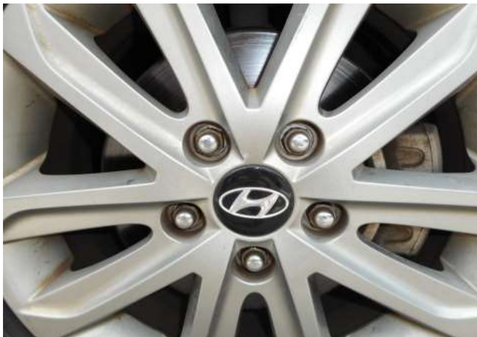
Photo 26 shows general view of the front right brake disc (arrowed) at the front right wheel of the Police Car after carrying out the operation tests. Visual examination of the brake disc shows no existing rust on the surface of the disc, as this is caused by the brake pads depressing against the brake discs when the brakes was applied to stop the vehicle. This is under the serviceable condition of the braking system
