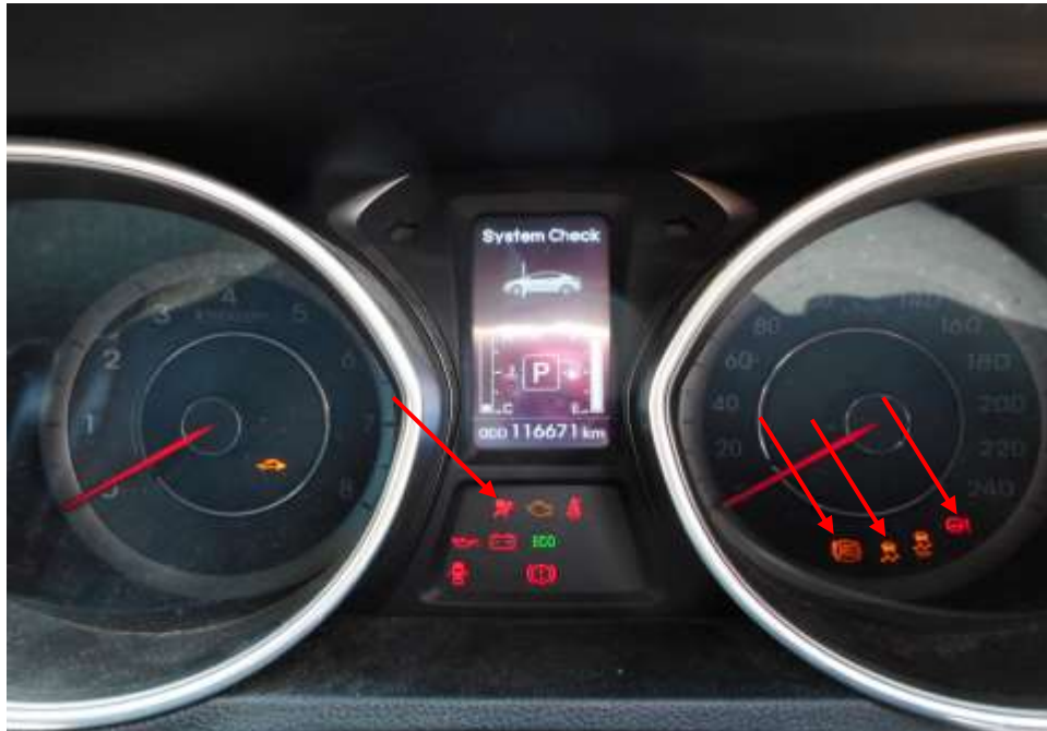
Photo 21 shows the warning light for Anti-Lock Brake System (ABS), Electric Power Steering System (EPS), Supplemental Restraint System (SRS) and Traction Control (TC) appearing on the instrument panel of the Police Car during the self-test of its various electronic operating systems when its engine was cranked.
