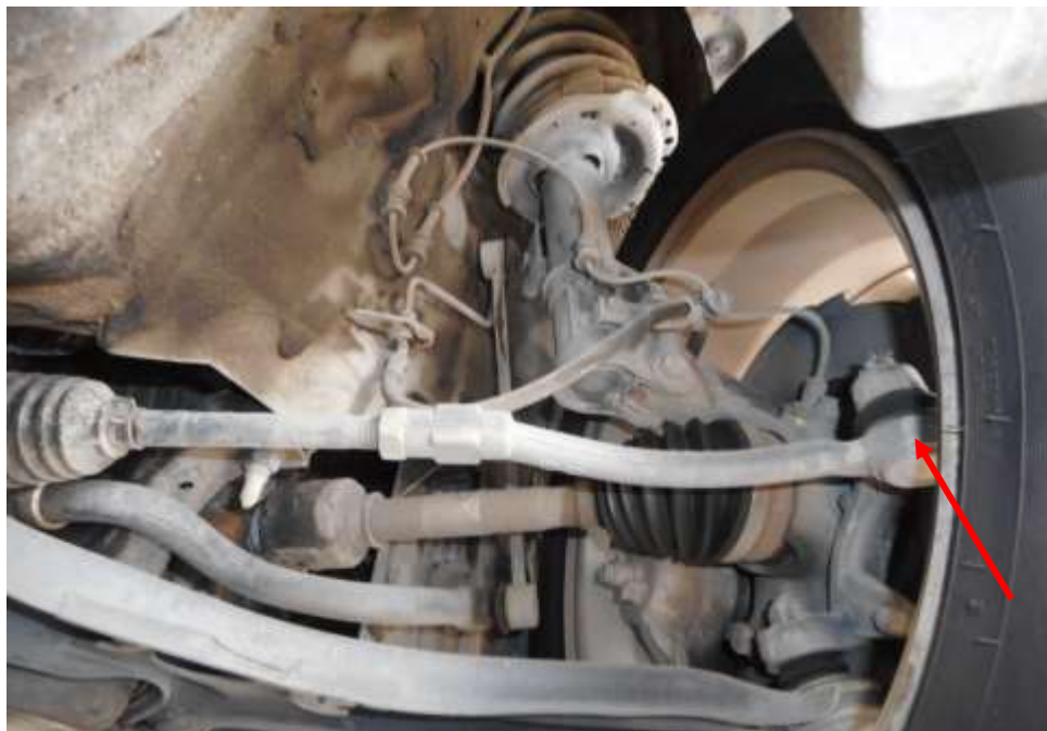
Photo 19 shows the various undercarriage components at the front right wheel of the Police Car, in particular the steering tie rod (arrowed). The various steering components were all found to be intact, suggesting that the steering system of the Police Car was likely to be in serviceable condition at the material time of accident. There was also no sign of fluid stain observed on the various undercarriage components at the front right wheel of the Police Car.
