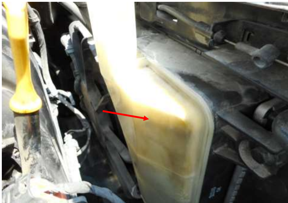
Photo 12 shows checks being carried out to the engine coolant of the Police Car at the time of my inspection. The engine coolant was observed to be of sufficient level (arrowed) and without any visible contamination.
