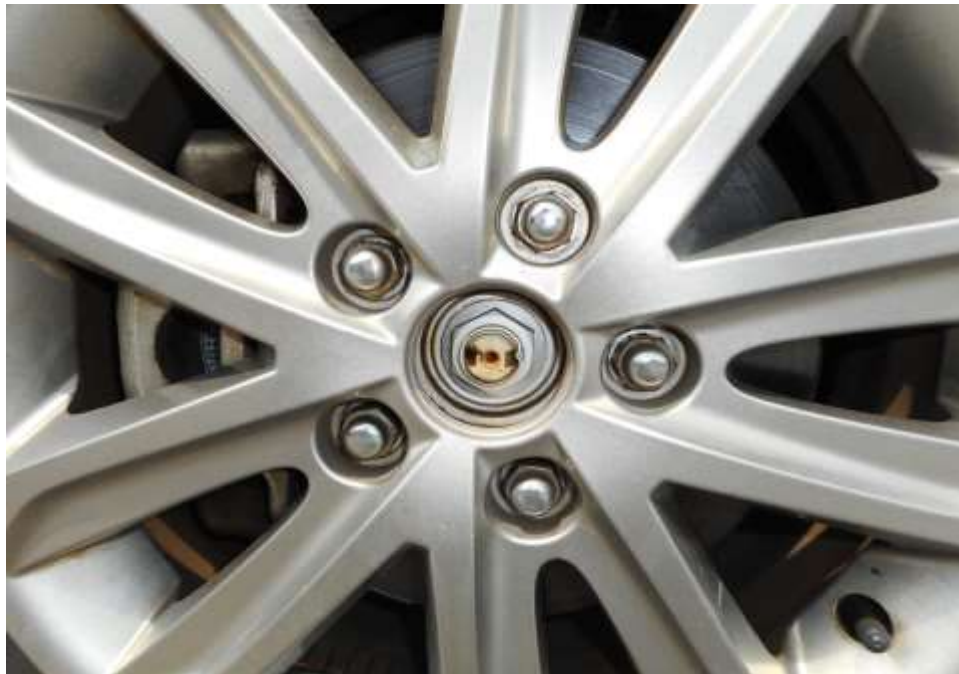
Photo 24 shows general view of the front left brake disc (arrowed) at the front left wheel of the Police Car after carrying out the operation tests. Visual examination of the brake disc shows no existing rust on the surface of the disc, as this is caused by the brake pads depressing against the brake discs when the brakes was applied to stop the vehicle. This is under the serviceable condition of the braking system
