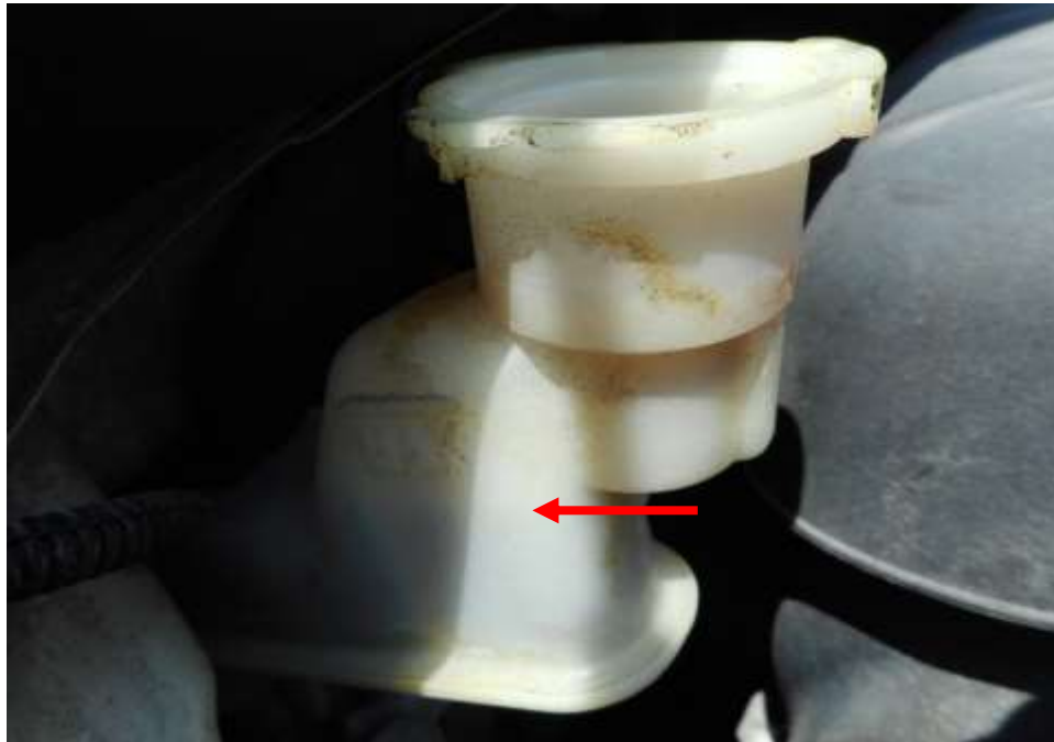
Photo 11 shows the brake fluid reservoir of the Police Car at the time of my inspection. The brake fluid was observed to be of sufficient level (arrowed) and without any visible contamination.
