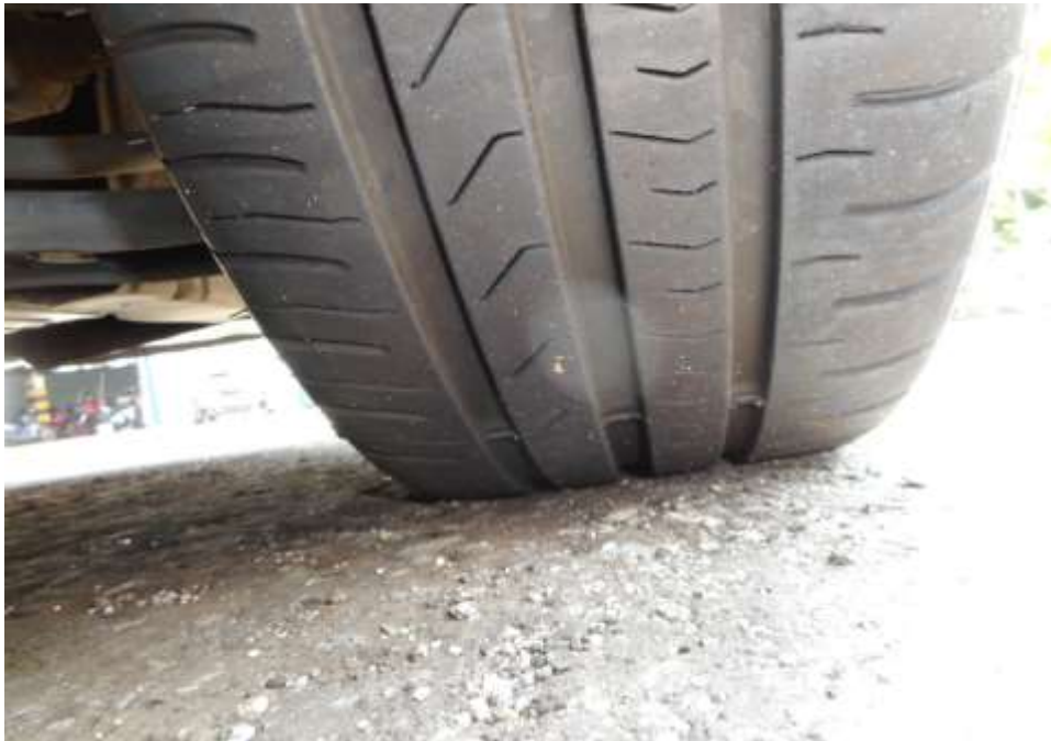
Photo 6 shows the condition of the front right tyre of the Police Car, which was observed to be in serviceable condition with remaining tread depth of approximately 5.9mm. The tyre was sufficiently inflated for vehicular operation with no tear, cut or burst mark(s) on the outer and the inner sidewalls as well as across the tread. The 4 tyres of the Police Car were wrapped around standard alloy wheel rims without any damage.
