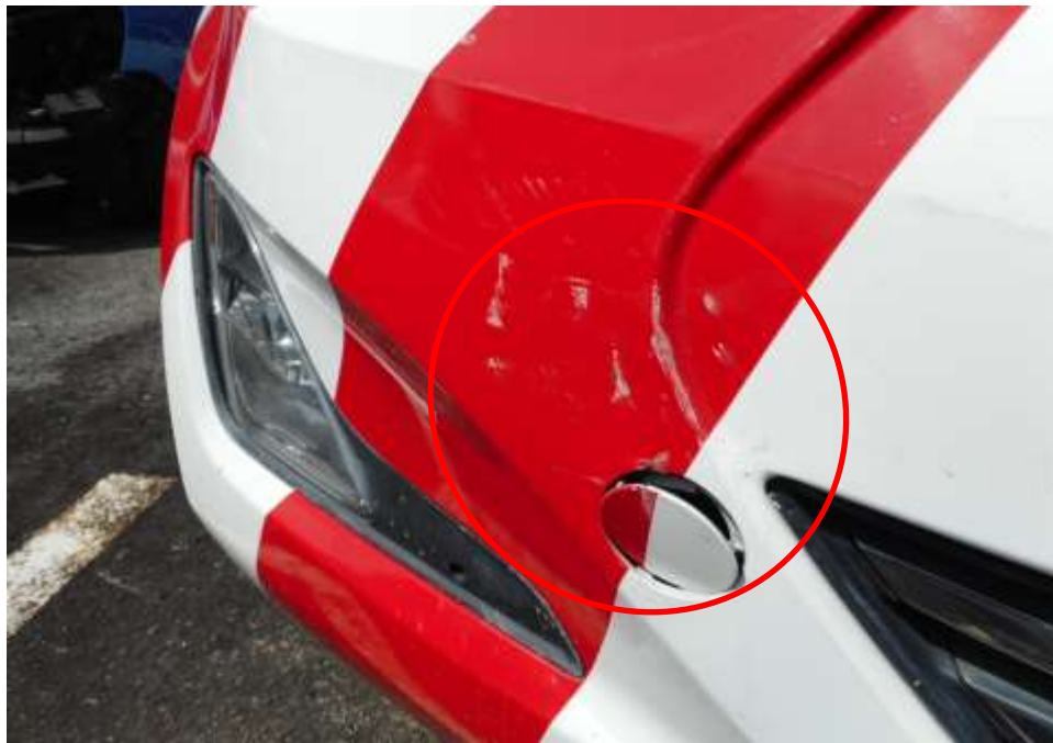
Photo 2 shows a close up view of the Police Car's at the time of my inspection. The front portion of the Police Car observed to have sustained minor damages at its frontal portion. Its front bumper (circled) was damage as a result of the accident at the time of my inspection.
