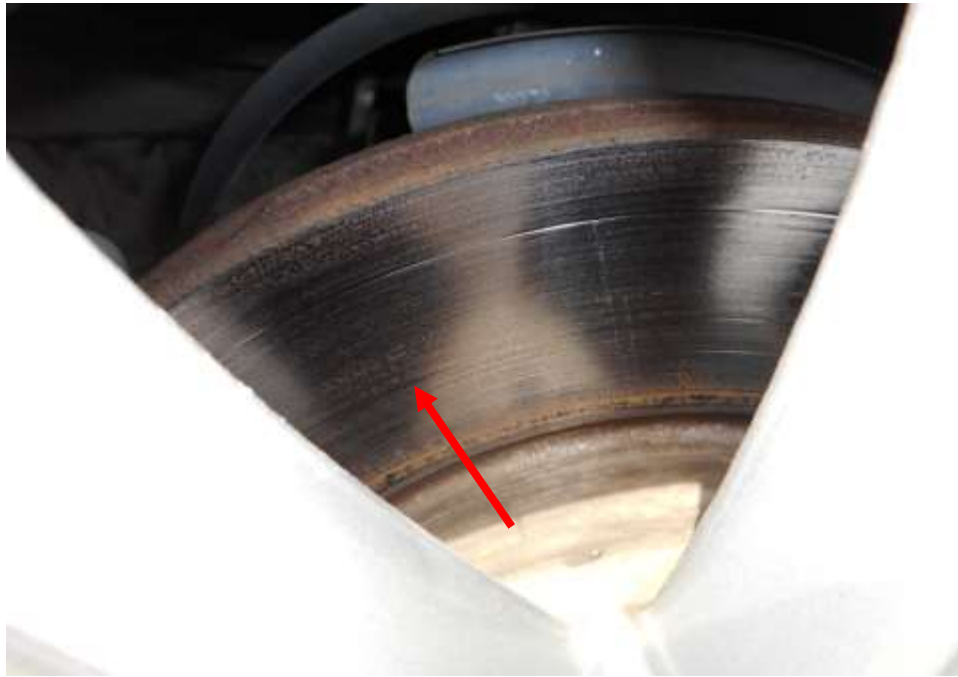
Photo 25 shows the close up view of the front left brake disc (arrowed) at the front left wheel of the Police Car after carrying out the operation tests. Visual examination of the brake disc shows no existing rust on the surface of the disc, as this is caused by the brake pads depressing against the brake discs when the brakes was applied to stop the vehicle. This is under the serviceable condition of the braking system
