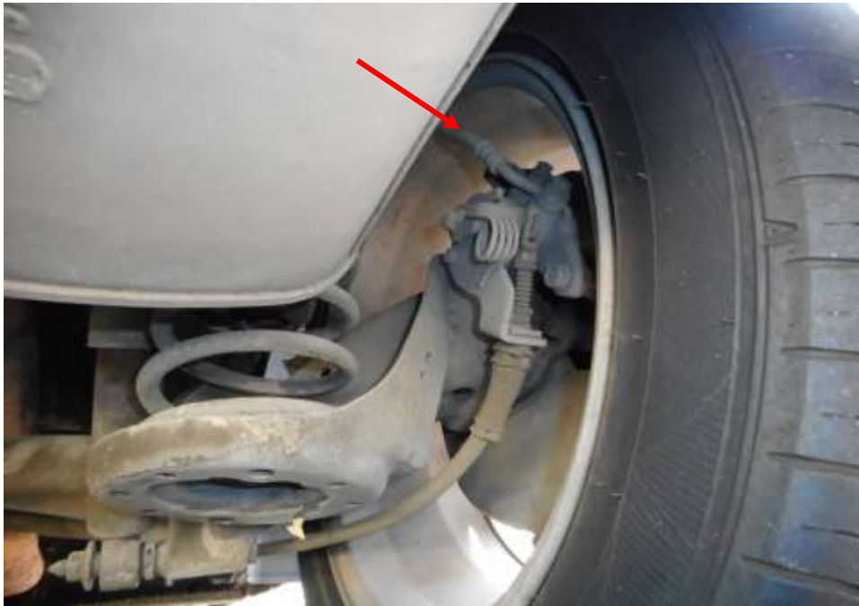
Photo 16 shows the brake hose/pipe (arrowed) at the rear right wheel of the Police Car. I did not observe any leakage of brake fluid at the time of my inspection of the Police Car. Static tests of the Police Car's braking system had indicated that there was no internal leakage of pressure/vacuum. The undercarriage components of the Police Car were also all found to be intact and without any visible damage.
