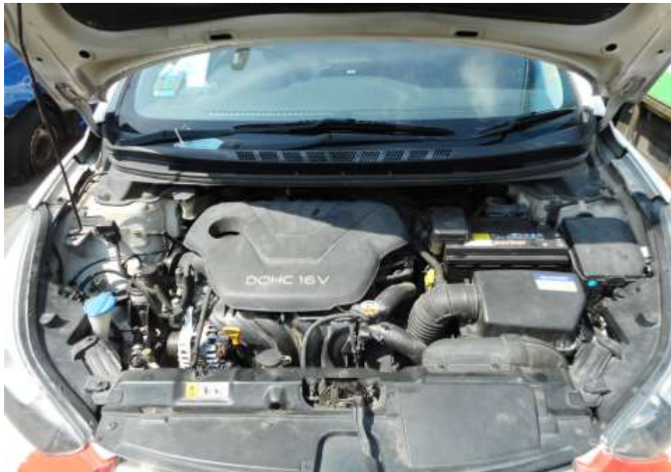
Photo 10 shows a general view of the Police Car's engine compartment. The various parts and components inside the engine compartment were unaffected by the accident. There was also no sign(s) or indication(s) of fluid leakage and/or fluid stain within the engine compartment.
