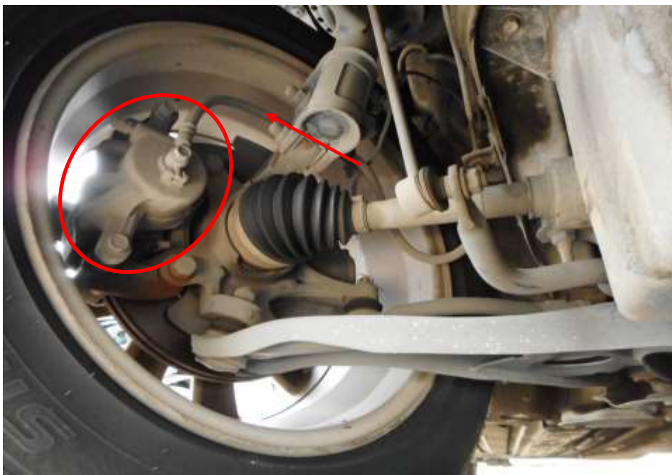
Photo 17 shows the brake hose/pipe (arrowed) at the front right wheel of the Police Car. No leakage of brake fluid was observed. Visual examination of the various components of the braking system like the brake caliper (circled), brake booster, brake pedal etc had revealed all to be intact and without visible damage.
