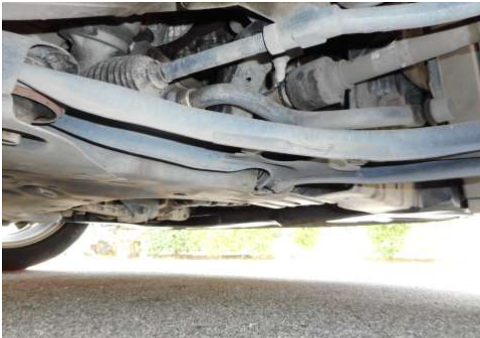
Photo 14 shows the undercarriage of the Police Car, at the area where the engine housing and transmission housing are located. I did not find any sign(s) or indication(s) of fluid leak and/or fluid stain(s) on the underside of the Police Car.
