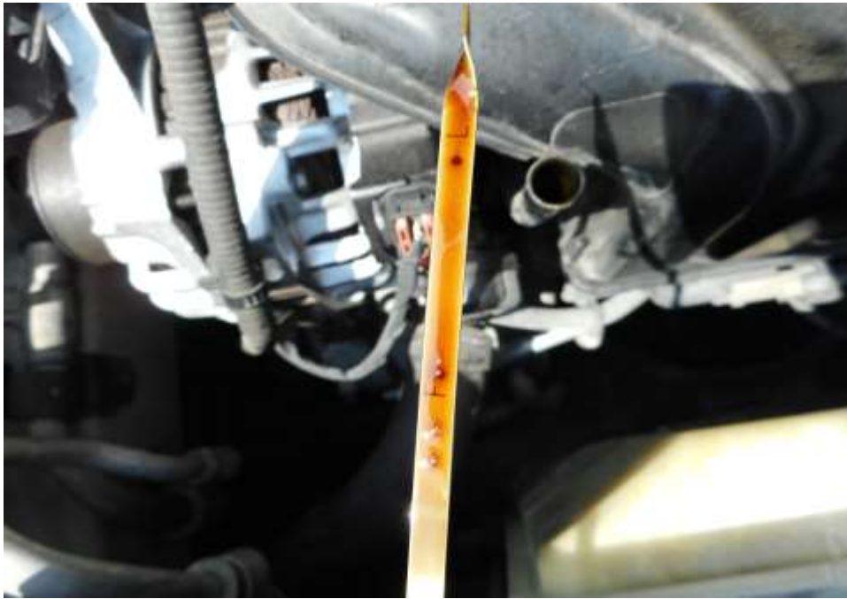
Photo 13 shows the engine oil dip stick of the Police Car at the time of my inspection. The engine oil was observed to be of sufficient level and without any visible contamination.
