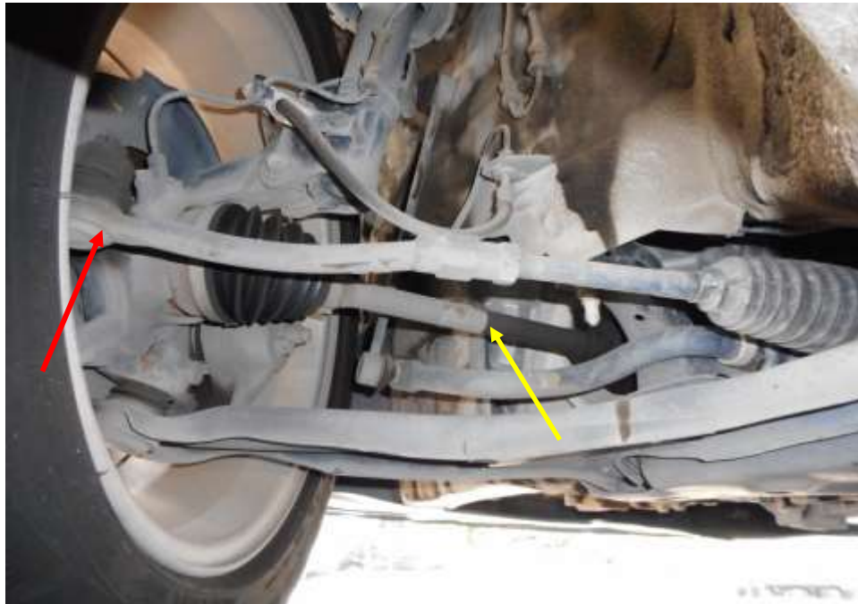
Photo 20 shows the various undercarriage components at the front left wheel of the Police Car, which had included the steering tie rod (red arrow) and front left drive shaft (yellow arrow). The various undercarriage components of the Police Car were all found to be intact without any visible damage.
