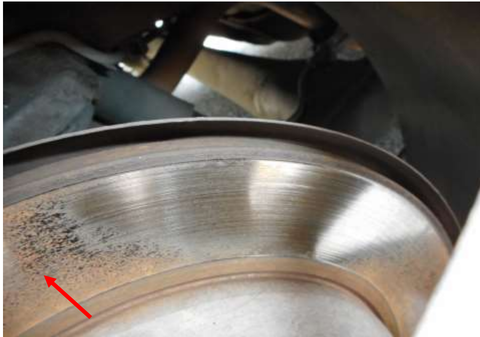
Photo 31 shows the close up view of the rear right brake disc (arrowed) at the rear right wheel of the Police Car after carrying out the operation tests. Visual examination of the brake disc shows the existing rust on the surface of the disc, this is caused by the brake pads not depressing against the brake discs when the brakes was applied to stop the vehicle. This affect has greatly decreased the braking efficiency of the braking system.
