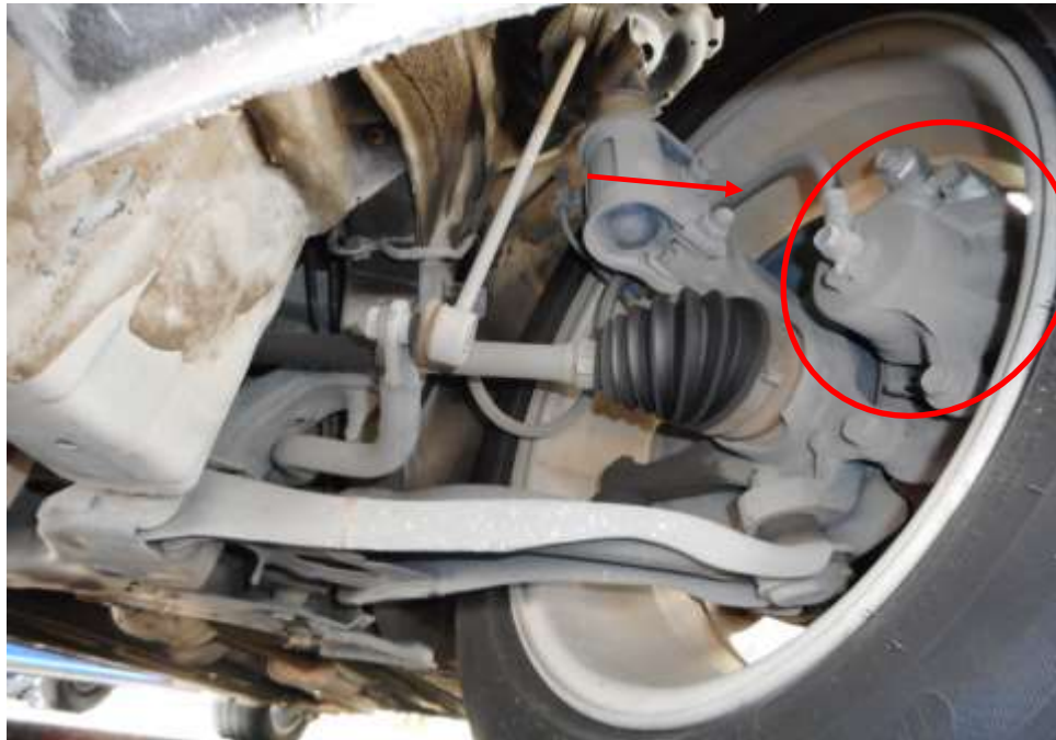
Photo 18 shows the brake hose/pipe (arrowed) at the front left wheel of the Police Car. No leakage of brake fluid was observed. Visual examination of the various components of the braking system like the brake caliper (circled), brake booster, brake pedal etc had revealed all to be intact and without visible damage.
