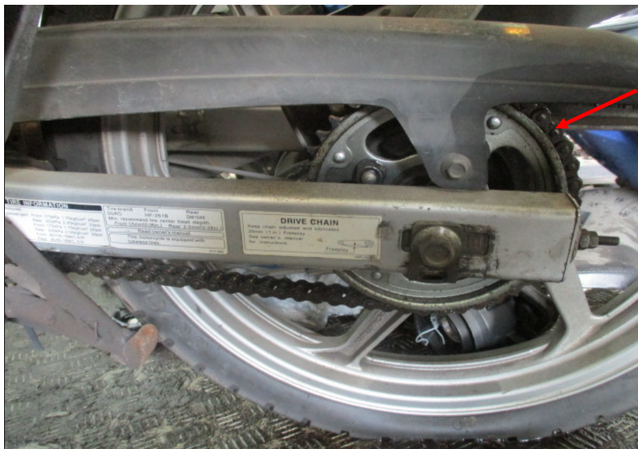
Photo 21 shows the gear chain (arrowed) of the Motorcycle, which was observed to be intact with no misalignment. It was also adequately lubricated for operating purposes. The gear chain rotates the rear wheel of the Motorcycle.
