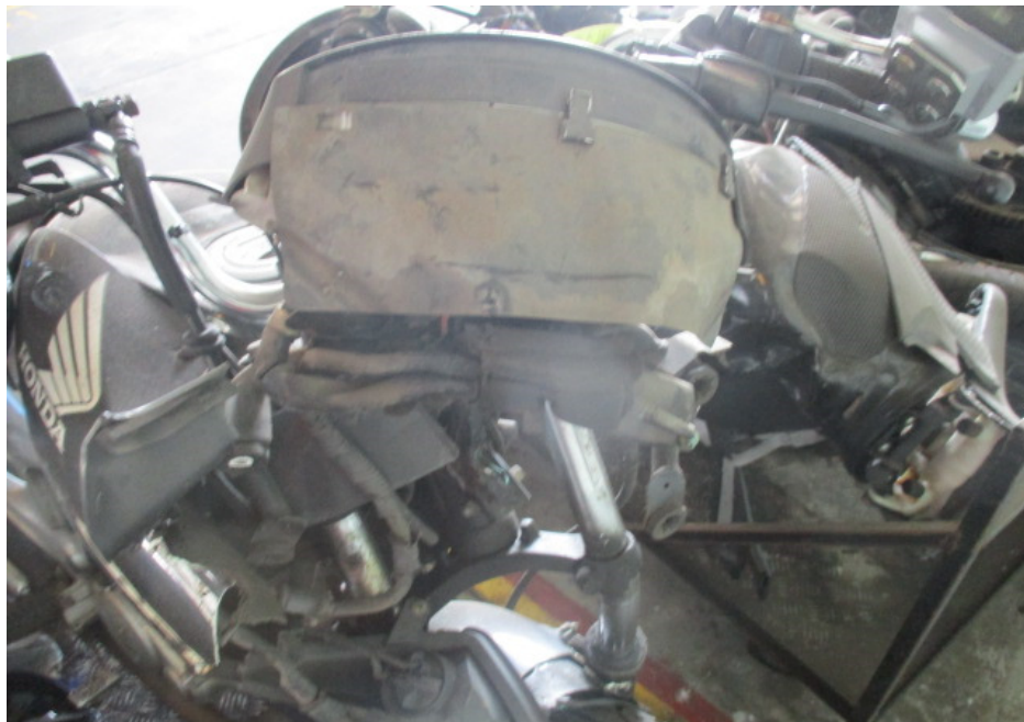
Photo 4 shows a general view of the front body of the Motorcycle at the time of our inspection. Body parts that were found to have been damaged include its headlamp assembly, fork assembly and speedometer gauge amongst others.
