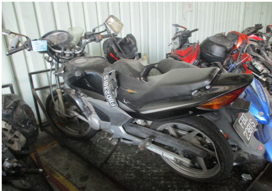
Photo 2 shows a general view of the left body of the Motorcycle at the time of our inspection. Body parts that were found to have been damaged include its headlamp assembly, front fork assembly, wheel rims, side mirrors, clutch lever, fuel tank, left side cover, gear shift pedal, seat and top box bracket, amongst others.
