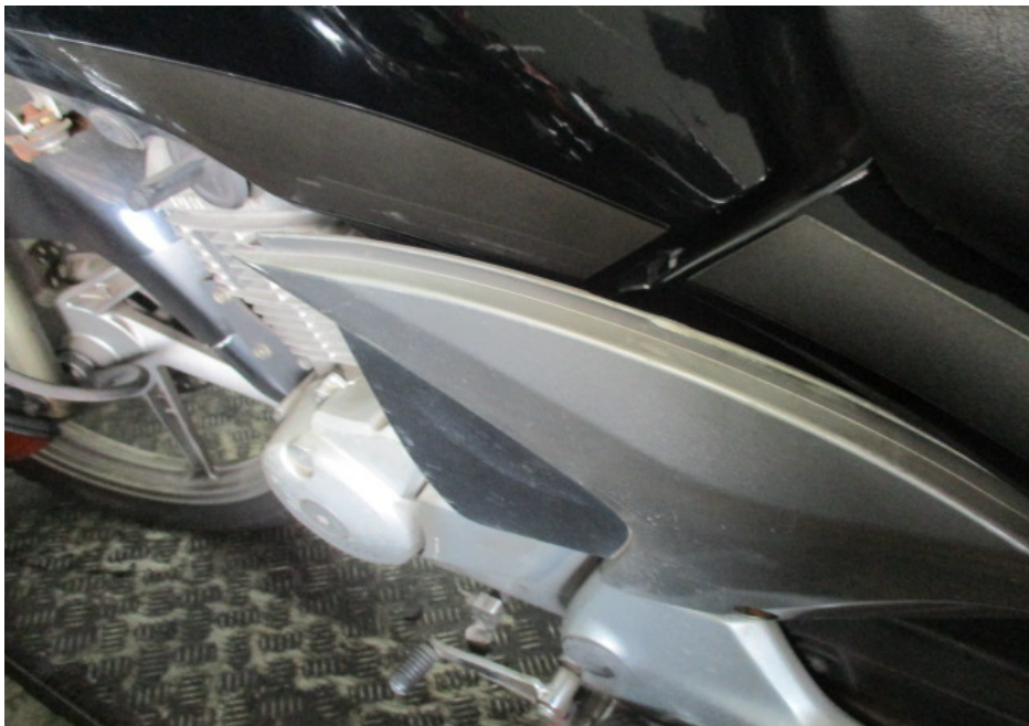
Photo 10 shows a closer view of the left side cover, which was amongst the body parts of the Motorcycle that had sustained damage as a result of the accident.
