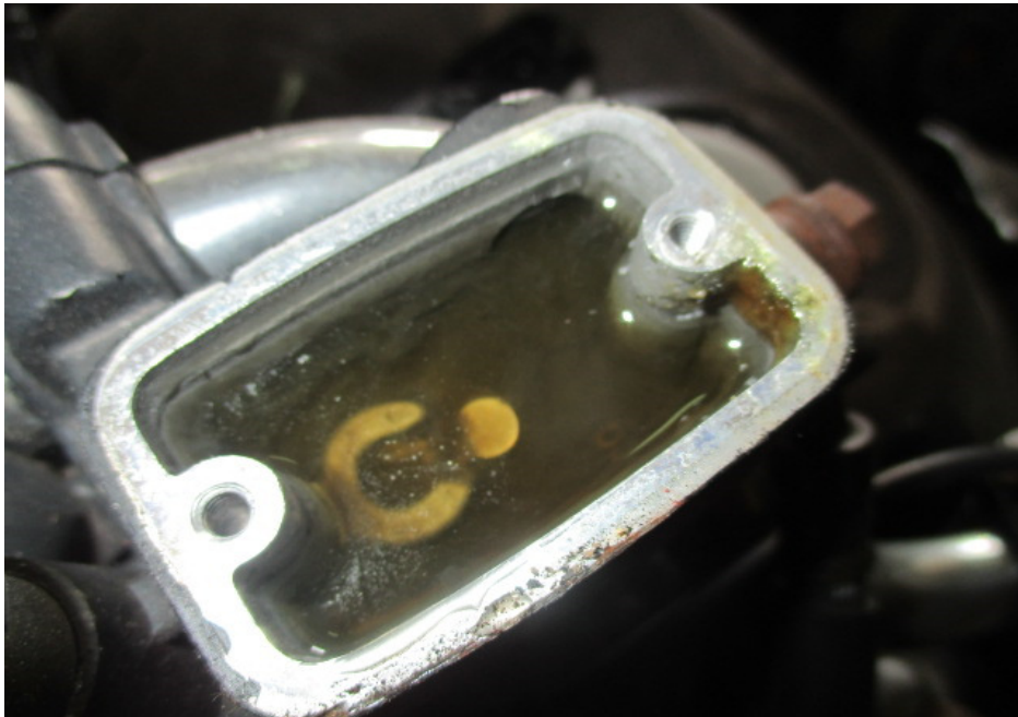
Photo 25 shows the brake fluid reservoir for the front brake of the Motorcycle. The brake fluid was observed to be without contamination and of sufficient level for operational purposes.
