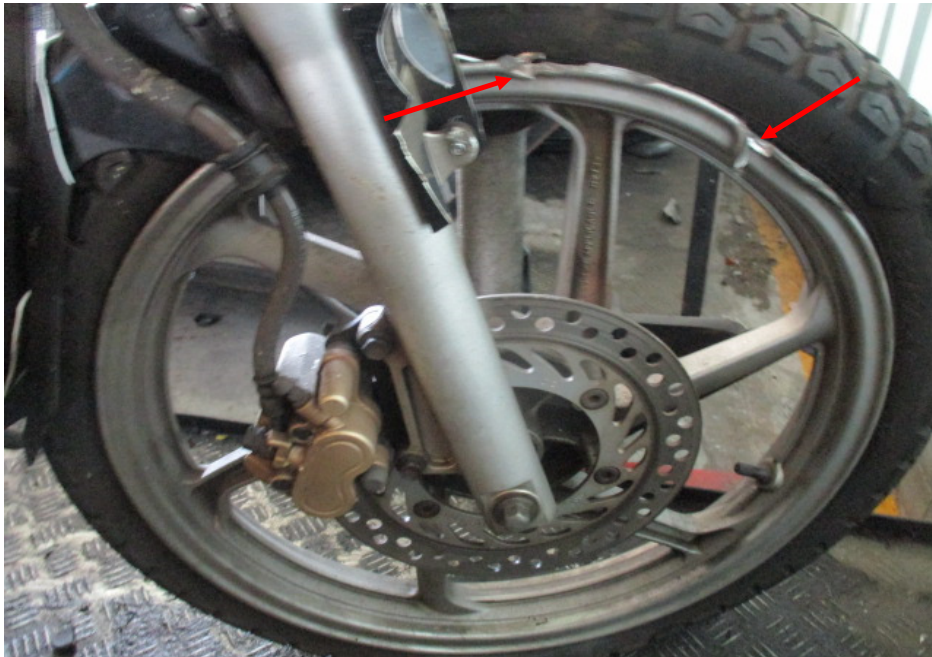
Photo 16 shows the bent front wheel rim of the Motorcycle at the time of our inspection (arrowed).
