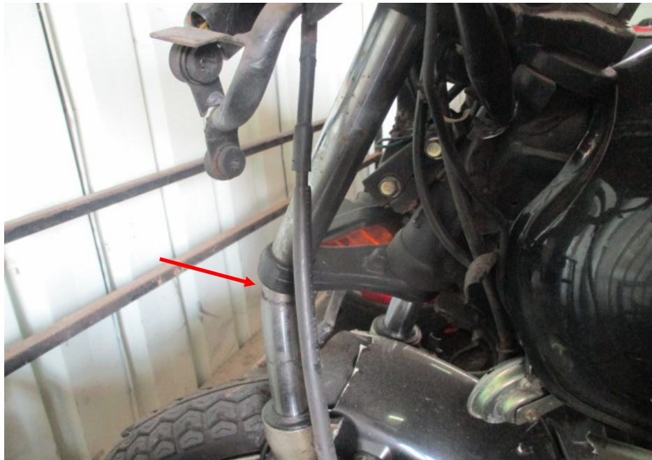
Photo 23 shows the front left fork of the Motorcycle. The front left fork (arrowed) was observed to be dislodged as a result of the accident. We were hence not able to conduct any tests on the steering system of the Motorcycle.
