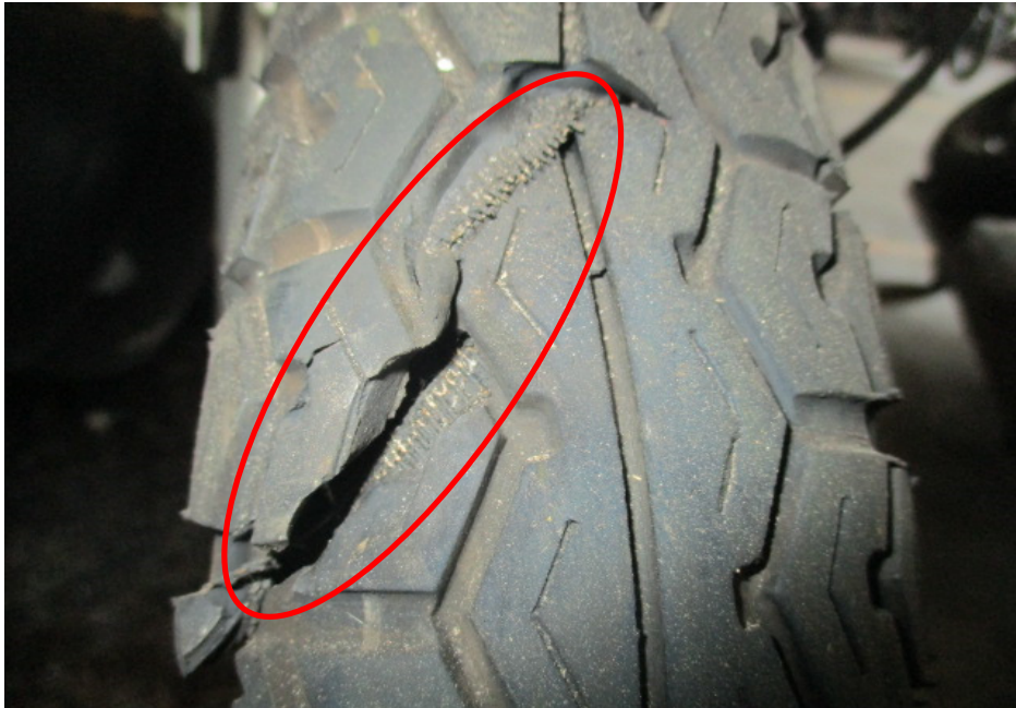
Photo 15 shows a close up view of the cut/tear on the front tyre of the Motorcycle (circled). The lines of the cut/tear were noted to be of a clean slicing type, suggesting that the cut/tear was by a sharp edge object. This would then indicate that the cut/tear of the Motorcycle's front tyre was a result of the accident and did not occur prior to the accident.
