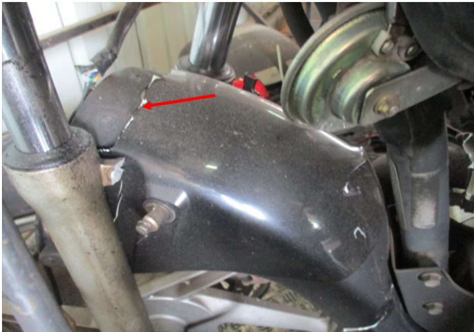
Photo 6 shows a closer view of the front mudguard (arrowed) which was amongst the body parts at the front body of the Motorcycle that had sustained damage as a result of the accident.
