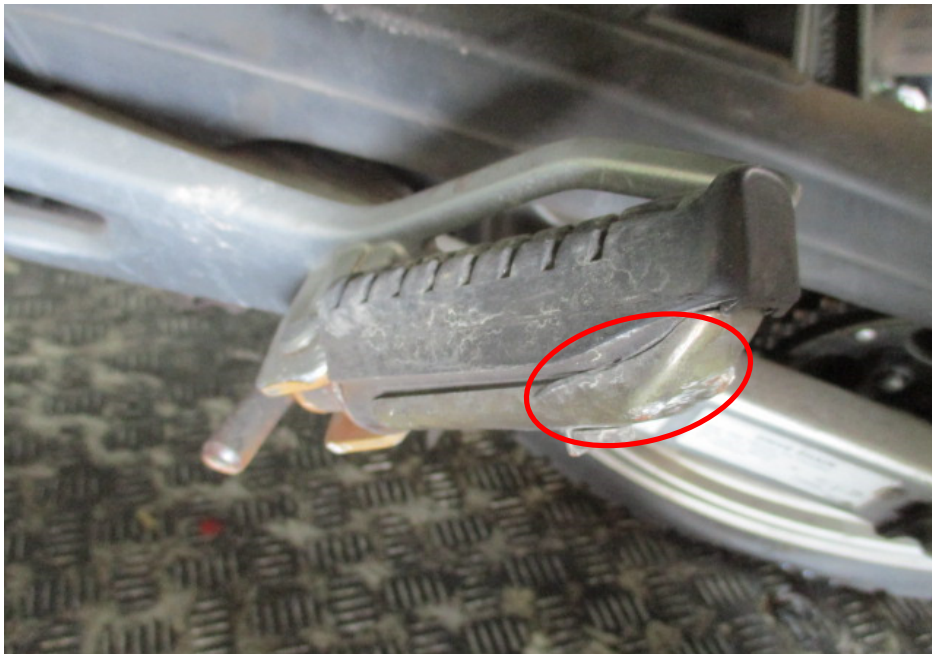
Photo 12 shows a closer view of the left pillion footrest which was amongst the body parts of the Motorcycle that had sustained damage as a result of the accident (circled).
