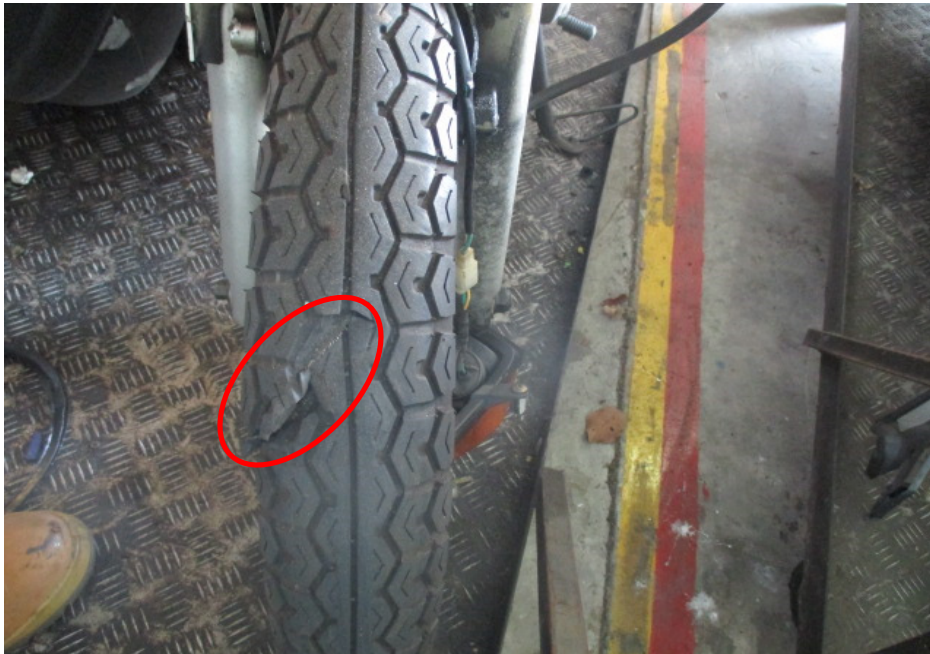
Photo 14 shows the front tyre of the Motorcycle at the time of our inspection. The pattern of the tread was clearly visible with remaining tread depth of approximately 3mm. We had observed a cut/tear on the tread area of this tyre (circled), which had penetrated into the core of the tyre resulting in the front tyre to be punctured.
