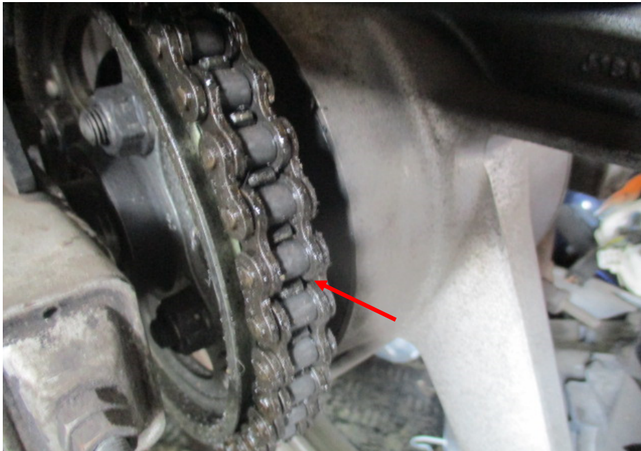
Photo 22 shows the closer view of the gear chain (arrowed) of the Motorcycle, which was observed to be intact with no misalignment. It was also adequately lubricated for operating purposes.
