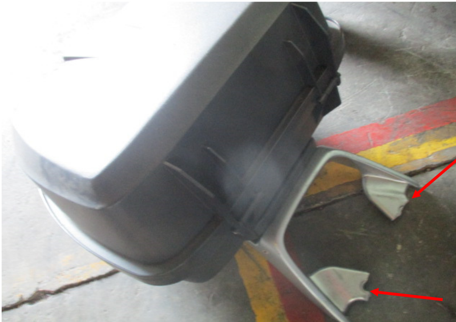
Photo 13 shows the top box bracket of the Motorcycle which had broken off as a result of the accident (arrowed).
