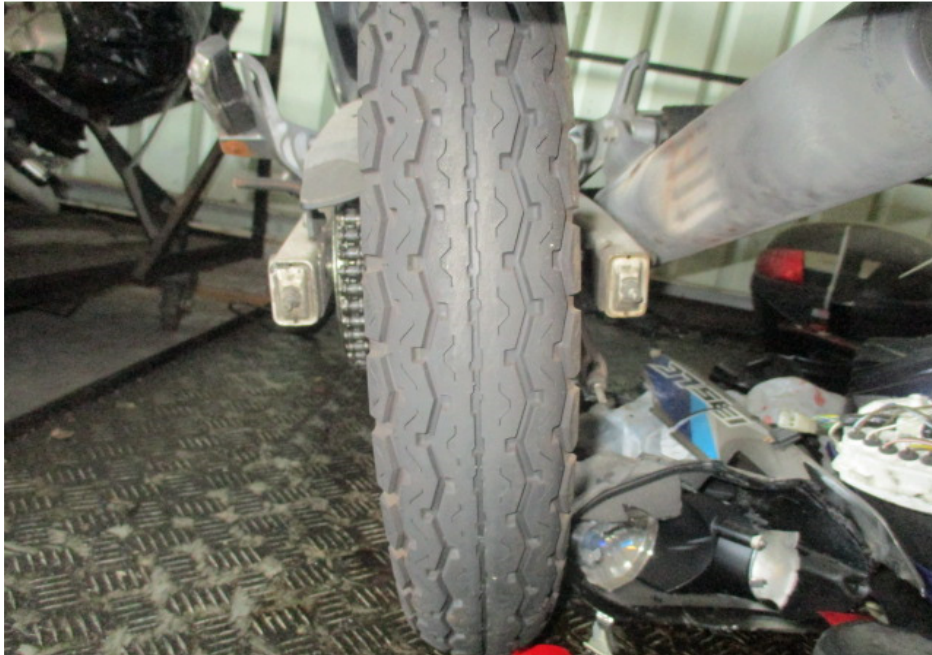
Photo 17 shows the condition of the Motorcycle's rear tyre. The pattern of the tread was clearly visible with remaining tread depth of approximately 5mm. We did not observe any tear, burst mark(s) and/or punctured hole(s) on the sidewalls as well as across the tread of the rear tyre. However we did observe that the rear tyre was deflated.
