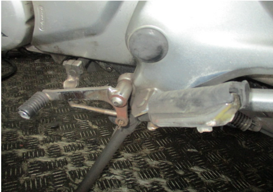
Photo 11 shows a closer view of the gear shift pedal and left front footrest which were amongst the body parts of the Motorcycle that had sustained damage as a result of the accident.
