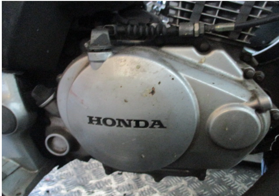
Photo 20 shows the right side of the engine of the Motorcycle at the time of our inspection. The various engine related parts and components were found to be intact with no visible damage. There was also no sign(s) or indication(s) of fluid leak observed around the right engine area of the Motorcycle.
