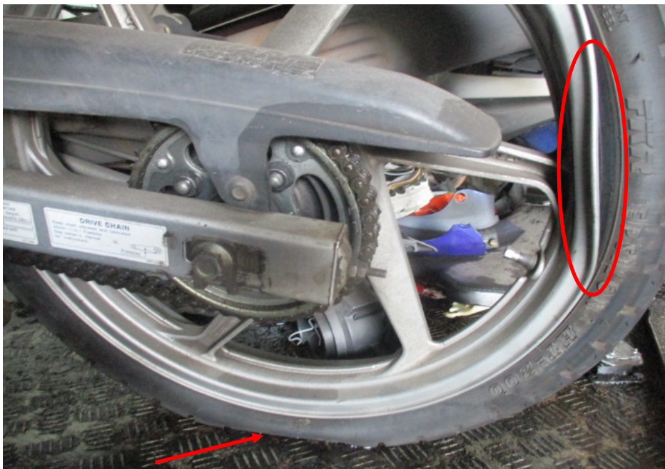
Photo 18 shows the deflated rear tyre (arrowed) and the bent rear wheel rim (circled) of the Motorcycle at the time of our inspection.
