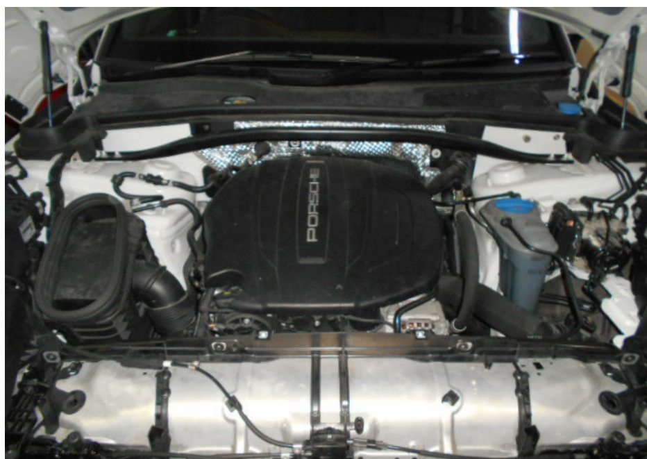
Photo 4 shows a general view of the engine compartment of the Motor Car at the time of my inspection. The various parts and components inside the engine compartment were all observed to be intact and properly fitted. There was also no sign(s) or indication(s) of fluid leak and/or fluid stain found inside the engine compartment. The engine oil, brake fluid and engine coolant were all found to be of sufficient level for operating purposes. Visually, there was also no contamination found to these fluids.
