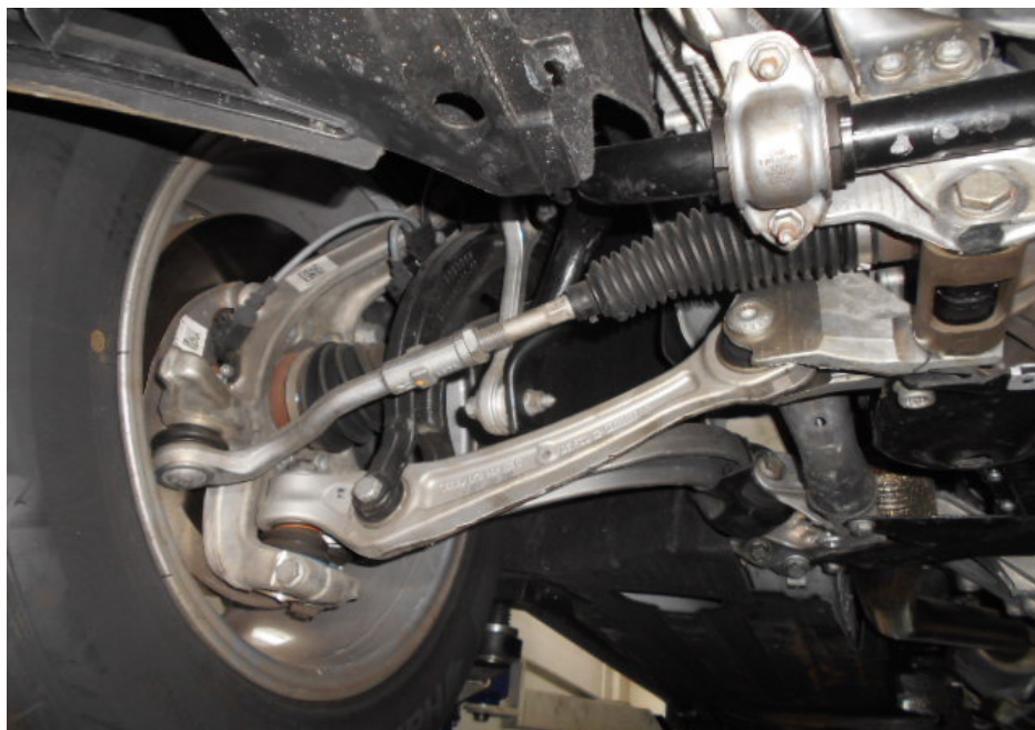
Photo 11 shows the various undercarriage components at the front right wheel of the Motor Car. The mechanical components, control arms and linkages were all found to be intact and secured in an appropriate manner. I also did not observe any fluid leak and/or fluid stain on the underside of the Motor Car.
