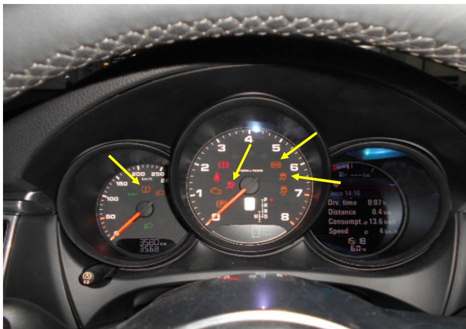
Photo 6 shows the warning lights for the various electronic safety features appearing on the instrument panel of the Motor Car during its self-test when the engine is cranked, in particular the ABS, SRS, TPM and TCS lights (arrowed).
