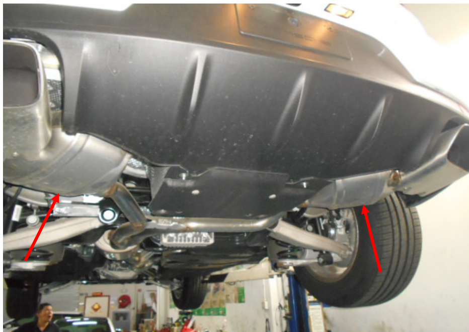
Photo 12 shows the Motor Car's rear exhaust mufflers (arrowed). My examination of the Motor Car's exhaust system revealed no sign(s) or indication(s) of any cut or weld marks along its exhaust pipes and on its rear mufflers.
