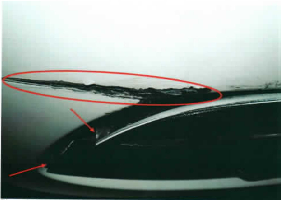
Photo 3 shows a close up view of the horizontal crack on the lower right portion of the front bumper of the VW (circled). The right fog light cover was also observed to be dislodged (arrowed).
