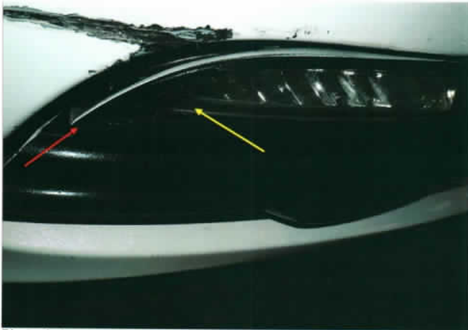
Photo 4 shows a close up view of the dislodged right fog light cover (red arrow) and right fog light (yellow arrow) of the VW.
