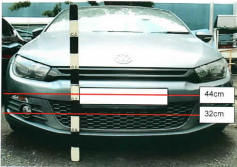
Photo 11 shows the height measurement being conducted on the front portion of the VW (using a similar make and model). The damages observed on the front bumper as well as right fog light cover of the VW were measured to be between the height ranges of 32cm to 44cm above ground level.
