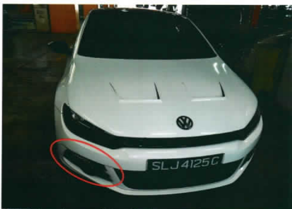
Photo 1 shows the general view of the front portion of the VW at the time of the Pre- Repair Survey conducted by LKK Auto Consultants Pte. Ltd. which was taken 2 days after the accident. The damages to the VW were observed to be confined to the front right portion, particularly to its front bumper (circled).
