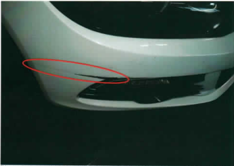
Photo 2 shows a closer view of the horizontal crack on the lower right portion of the front bumper of the VW (circled).
