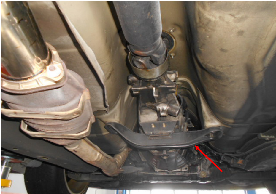
Photo 8 shows a general view of the transmission assembly that was fitted on the Motor Car, as viewed from the rear to front. The transmission assembly is supported by a bracket (arrowed) that is mounted on the underside of the floor board of the Motor Car, via bolts and nuts.
