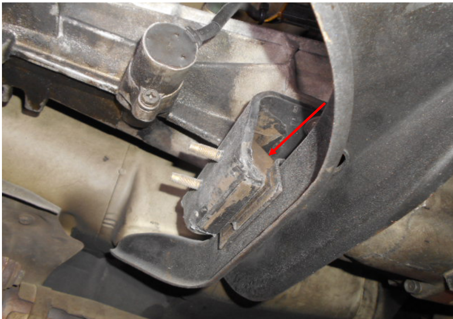
Photo 7 shows the rubber bushing (arrowed) that absorbs any vibrations arising from the rotation of the transmission gears, minimising any stress to the bracket.
