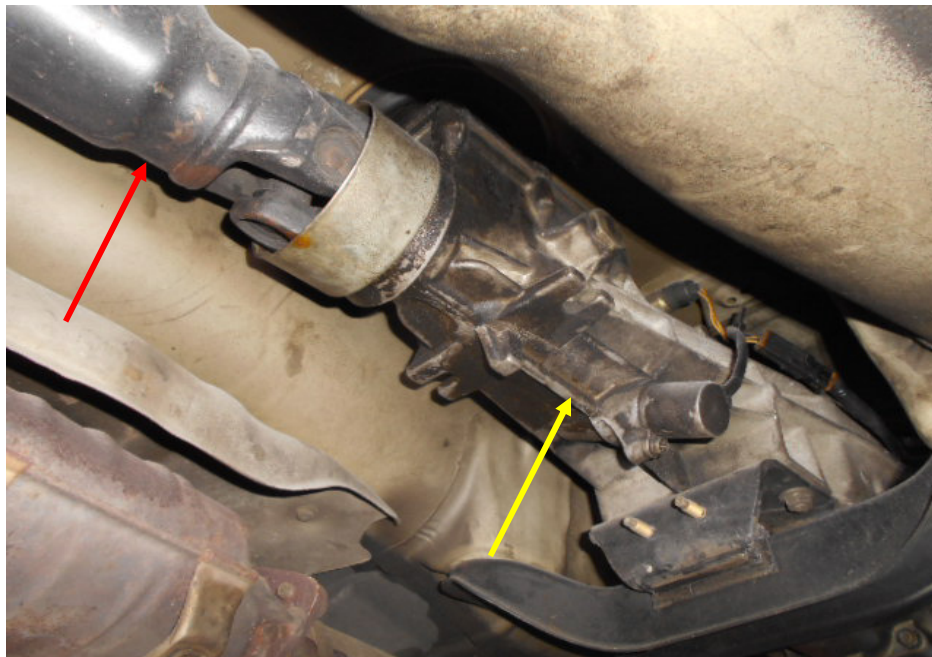
Photo 4 shows the rear (output) side of the transmission (yellow arrow), which connects to the propeller shaft (red arrow) that links to the rear axle of the Motor Car.
