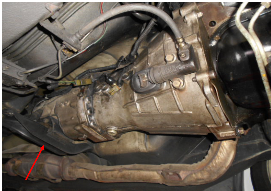
Photo 5 shows a general view of the bracket (arrowed) mounted to the underside of the floor board of the Motor Car, via bolts and nuts. The bracket supports the rear (output) side of the transmission.
