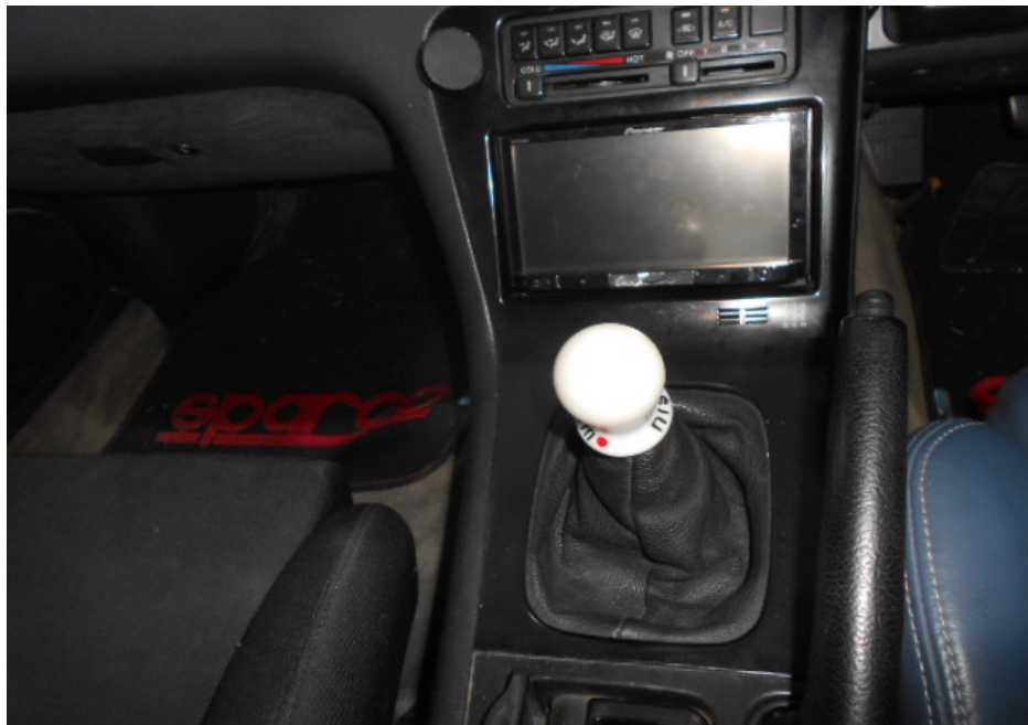
Photo 10 shows the manual gear shifter for manually selecting the transmission gear to be engaged.
