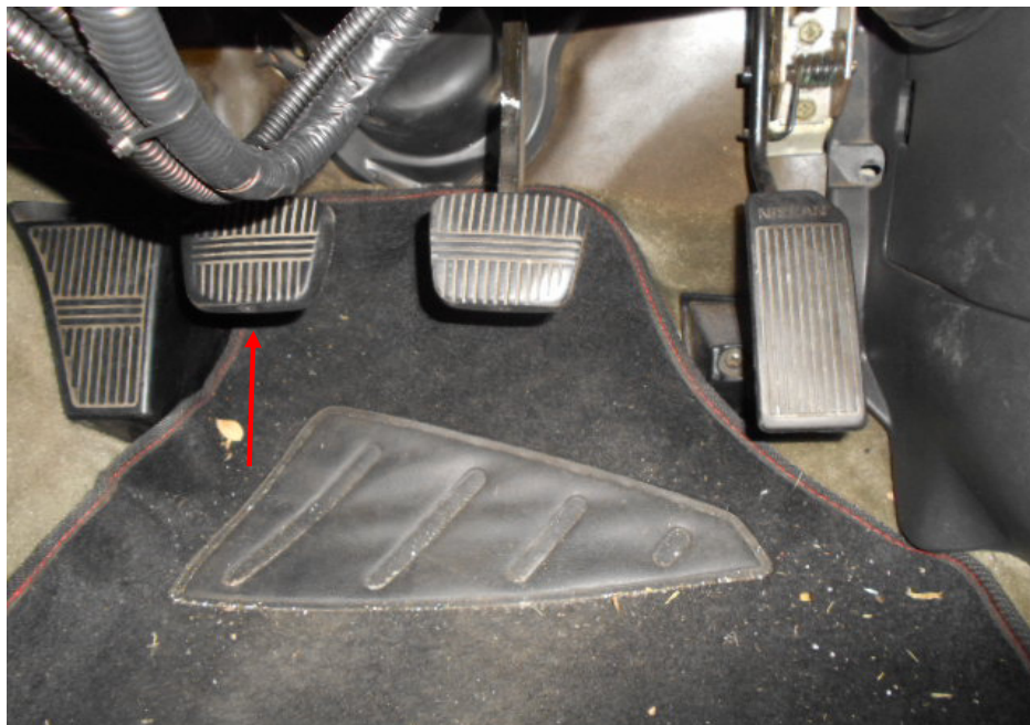
Photo 11 shows the clutch pedal (arrowed) for engaging and disengaging the transmission gears.
