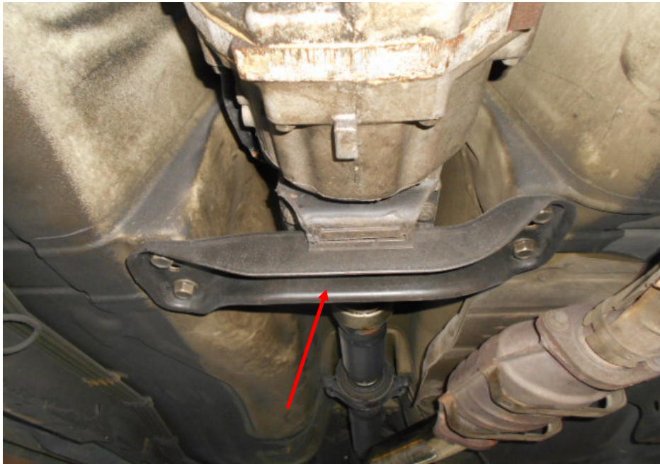
Photo 6 shows a closer view of the bracket (arrowed) mounted to the underside of the Motor Car's floor board, via bolts and nuts. The bracket supports the rear (output) side of the transmission. Rubber bushings absorb any vibrations arising from the rotation of the transmission gears, minimising any stress to the bracket.
