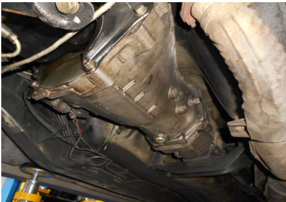
Photo 3 shows the front (input) side of the transmission, which is bolted to the crankshaft side of the Motor Car's engine block.
