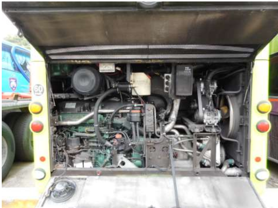
Photo 12 shows a general view of the Motor Bus's engine compartment, which was accessed by lifting the front cabin of the Motor Bus. The various parts and components inside the engine compartment were unaffected by the accident. There was also no sign(s) or indication(s) of fresh fluid leakage and/or fluid stain within the engine compartment
