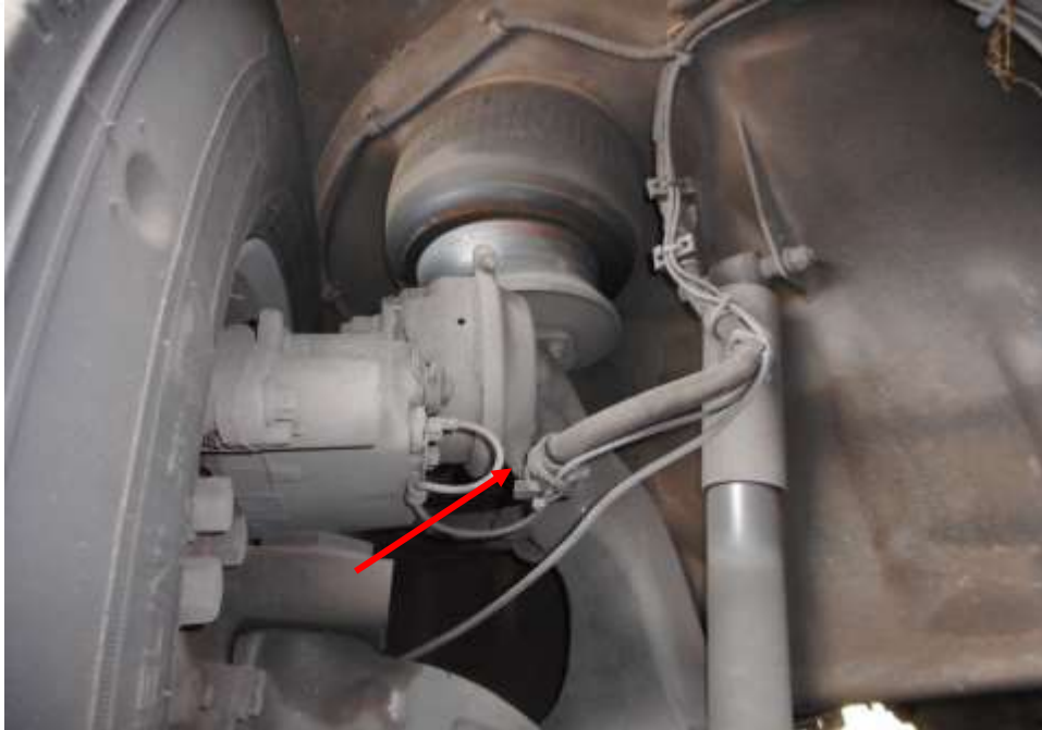
Photo 20 shows the brake pipe (arrowed) at the front left wheel of the Motor Bus. I did not observe any leakage of brake fluid at the time of my inspection of the Motor Bus. My static tests of the Motor Bus's braking system, along with my visual examination of the various mechanical components in the braking system had indicated that there was no internal leakage of pressure/vacuum. Hence the braking system of the Motor Bus was likely to be in serviceable condition at the material time of accident.
