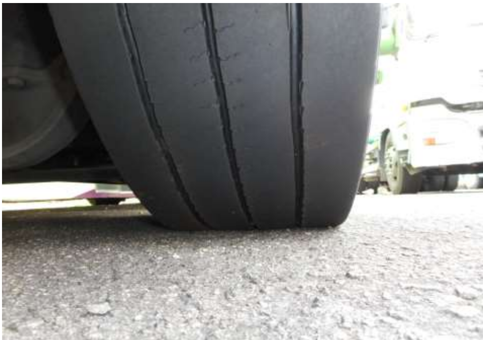
Photo 11 shows the condition of the front left tyres of the Motor Bus, which were observed to be in serviceable condition with remaining tread depth of approximately 7.3mm. There was also no tear, cut or burst mark(s) on the outer and the inner sidewalls as well as across the tread of the 10 tyres that were fitted on the Motor Bus.
