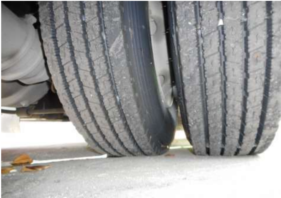
Photo 10 shows the condition of the rear left tyres of the Motor Bus, which was observed to be in serviceable condition with remaining tread depth of approximately 12.8mm. The tyres, which were wrapped around standard steel wheel rim, were also observed to be sufficiently inflated for vehicular operation. There was also no damage found on all 10 steel wheel rims of the Motor Bus.
