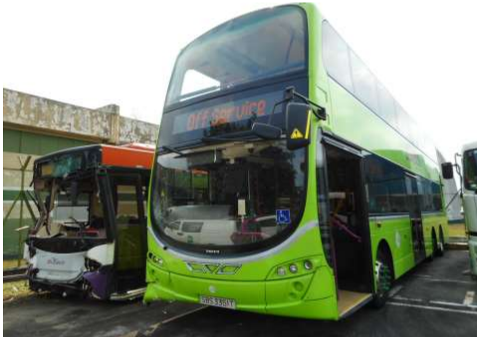
Photo 6 shows a general view of the left body of the Motor Bus at the time of my inspection. The Motor Bus was observed to be in good general condition and unaffected by the accident.
