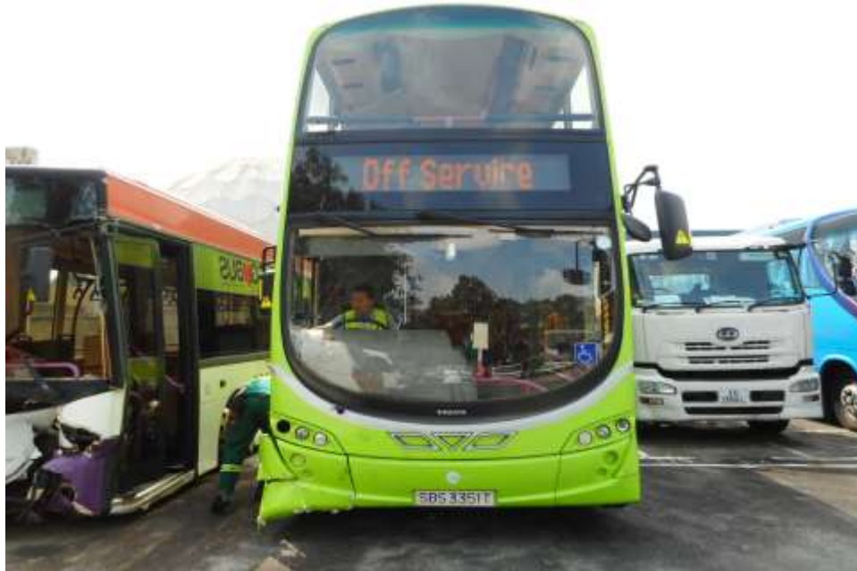
Photo 2 shows a general view of the front body of the Motor Bus at the time of my inspection. The Motor Bus sustained damages at its front portion. Its front windscreen, front body panel, front right bumper and front right headlight was damaged as a result of the accident at the time of my inspection.
