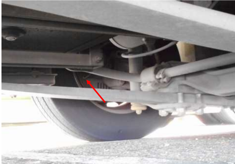
Photo 17 shows the brake pipe (arrowed) at the rear right wheel of the Motor Bus. I did not observe any leakage of brake fluid at the time of my inspection of the Motor Bus. My static tests of the Motor Bus's braking system, along with my visual examination of the various mechanical components in the braking system, had indicated that there was no internal leakage of pressure/vacuum. Hence the braking system of the Motor Bus was likely to be in serviceable condition at the material time of accident.
