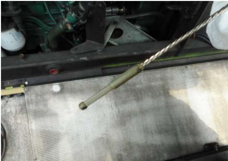
Photo 16 shows the engine oil dip stick system of the Motor Bus at the time of my inspection. The engine oil was observed to be of in the lower level but sufficient for operation and without any visible contamination.
