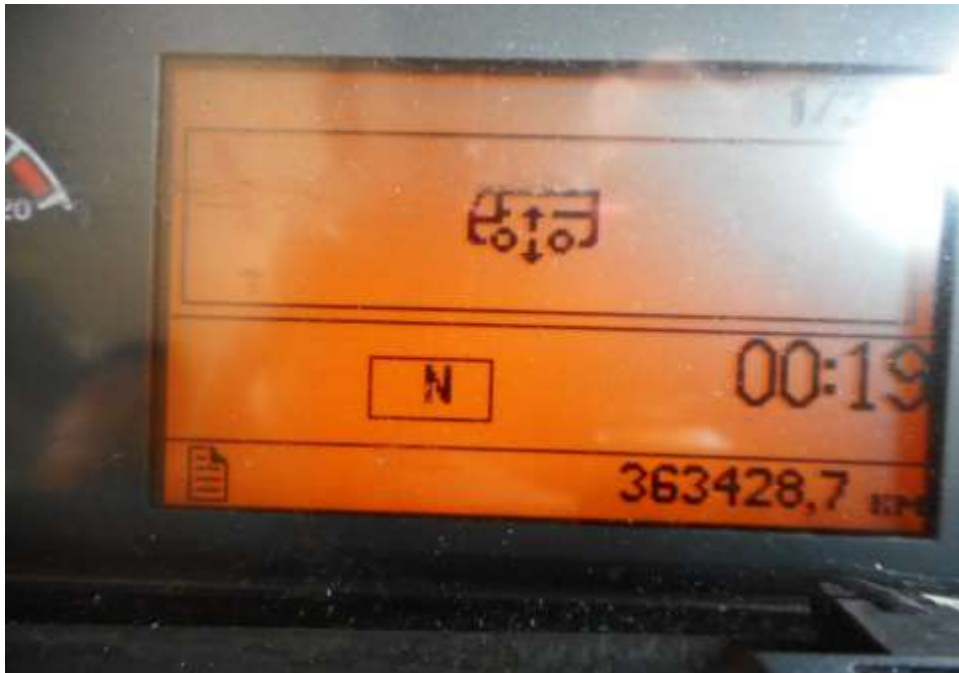
Photo 1 shows a general view of the instrument cluster of the Motor Bus at the time of my inspection. The mileage of the Motor Bus was 363,428km
