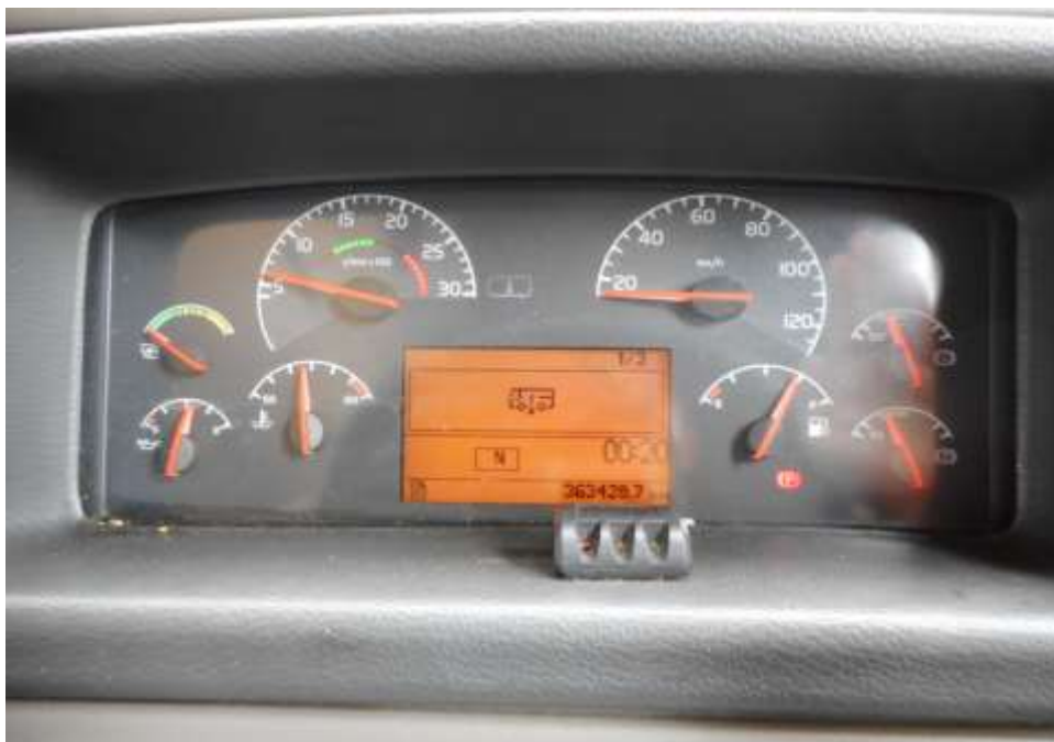
Photo 28 shows no warning lights illuminated on the instrument panel of the Motor Lorry after the engine was cranked. This would suggest that there was no abnormality to the various electronic operating systems of the Motor Lorry, like the ABS
