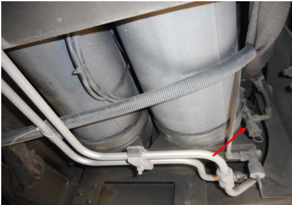
Photo 21 shows the air brake cylinder (arrowed) at the undercarriage of the Motor Bus. I did not observe any leakage of air brake fluid at the time of my inspection of the Motor Bus. My static tests of the Motor Bus's braking system, along with my visual examination of the various mechanical components in the braking system had indicated that there was no internal leakage of pressure/vacuum. Hence the braking system of the Motor Bus was likely to be in serviceable condition at the material time of accident.
