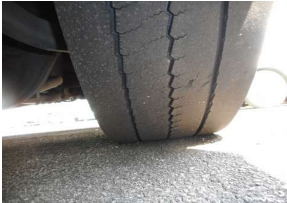
Photo 8 shows the condition of the front right tyre of the Motor Bus, which was observed to be in serviceable condition with remaining tread depth of approximately 6.9mm. The tyre, which was wrapped around standard steel wheel rim, was also observed to be sufficiently inflated for vehicular operation. There was no tear, cut or burst mark(s) on the outer and the inner sidewalls as well as across the tread of the 10 tyres that were fitted on the Motor Bus.
