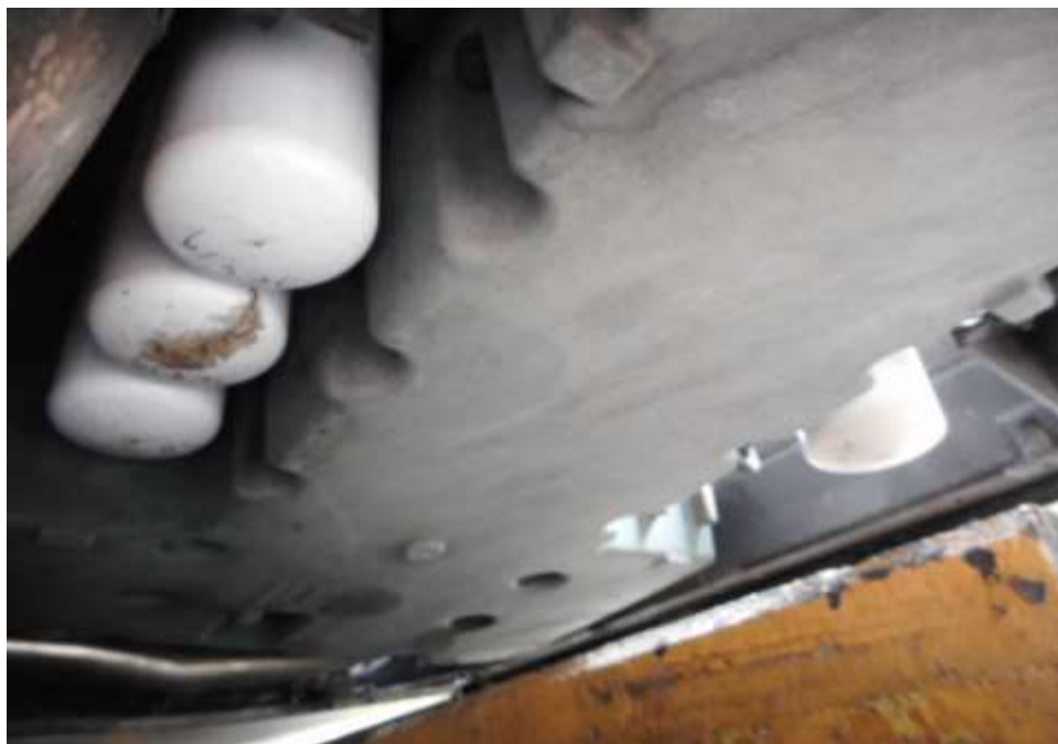
Photo 25 shows the undercarriage of the Motor Bus, at the area where the engine housing located. We observed minor fresh fluid stains on the surface of the engine oil sump. However the Motor Bus is still in serviceable condition.
