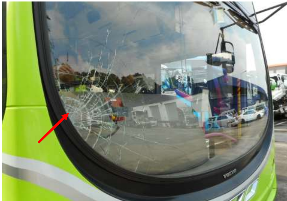
Photo 3 shows a close up view of the front body of the Motor Bus at the time of my inspection. Its front windscreen (arrowed) was damaged as a result of the accident at the time of my inspection.
