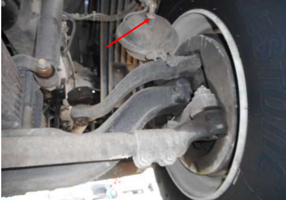
Photo 18 shows the brake pipe (arrowed) at the front left wheel of the Motor Lorry. I did not observe any leakage of brake fluid at the time of my inspection of the Motor Lorry. My static tests of the Motor Lorry's braking system, along with my visual examination of the various mechanical components in the braking system had indicated that there was no internal leakage of pressure/vacuum. Hence the braking system of the Motor Lorry was likely to be in serviceable condition at the material time of accident.
