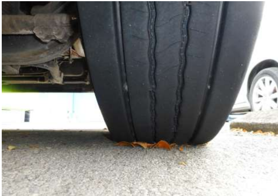
Photo 7 shows the condition of the front right tyre of the Motor Lorry, which was observed to be in serviceable condition with remaining tread depth of approximately 8.4mm. The tyre, which was wrapped around standard steel wheel rim, was also observed to be sufficiently inflated for vehicular operation. There was no tear, cut or burst mark(s) on the outer and the inner sidewalls as well as across the tread of the 10 tyres that were fitted on the Motor Lorry.
