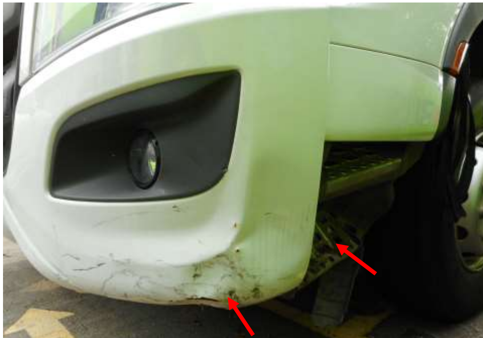
Photo 3 shows a close up view of the front body of the Motor Lorry at the time of my inspection. The Motor Lorry was observed to have sustained minor damages at its left portion at the time of my inspection. Its front bumper and left bed steps (arrowed) were damaged as a result of the accident.
