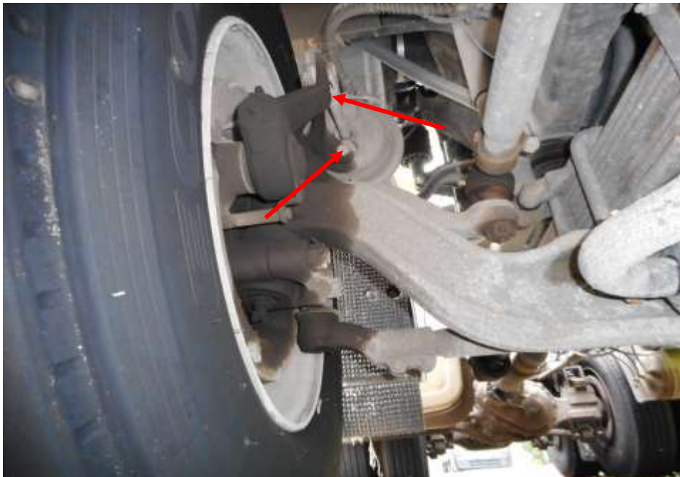
Photo 17 shows the brake pipe (arrowed) at the front right wheel of the Motor Lorry. I did not observe any leakage of brake fluid at the time of my inspection of the Motor Lorry. My static tests of the Motor Lorry's braking system, along with my visual examination of the various mechanical components in the braking system, had indicated that there was no internal leakage of pressure/vacuum. Hence the braking system of the Motor Lorry was likely to be in serviceable condition at the material time of accident.
