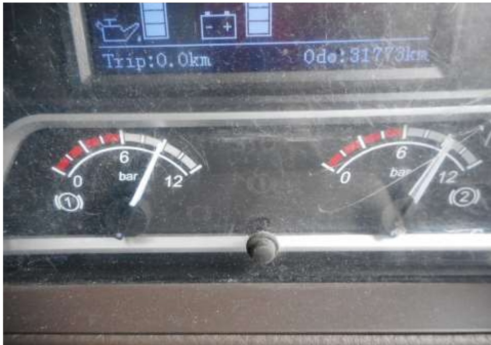
Photo 12 shows the air in the air brake cylinder of the Motor Lorry at the time of my inspection. The air in the cylinder was observed to be of sufficient level & serviceable at the time of the accident.
