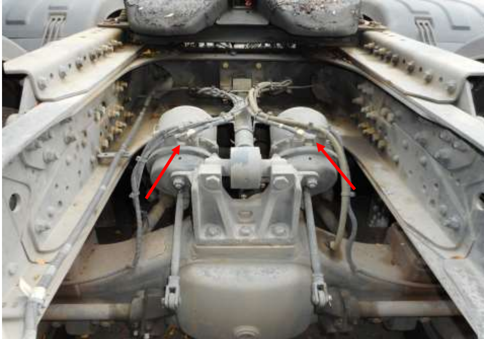
Photo 16 shows the brake pipe (arrowed) at the left and rear right wheel of the Motor Lorry. I did not observe any leakage of brake fluid at the time of my inspection of the Motor Lorry. My static tests of the Motor Lorry's braking system, along with my visual examination of the various mechanical components in the braking system, had indicated that there was no internal leakage of pressure/vacuum. Hence the braking system of the Motor Lorry was likely to be in serviceable condition at the material time of accident.
