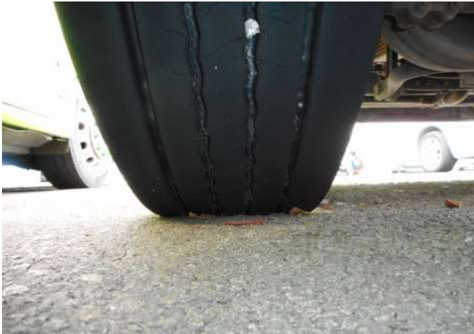
Photo 10 shows the condition of the front left tyres of the Motor Lorry, which were observed to be in serviceable condition with remaining tread depth of approximately 8.9mm. There was also no tear, cut or burst mark(s) on the outer and the inner sidewalls as well as across the tread of the 8 tyres that were fitted on the Motor Lorry.
