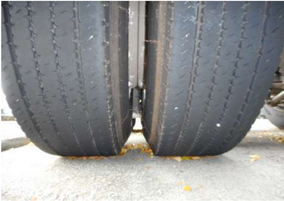
Photo 8 shows the condition of the rear right tyre of the Motor Lorry, which was observed to be in serviceable condition with remaining tread depth of approximately 7.7mm. The tyre, which was wrapped around standard steel wheel rim, was also observed to be sufficiently inflated for vehicular operation.
