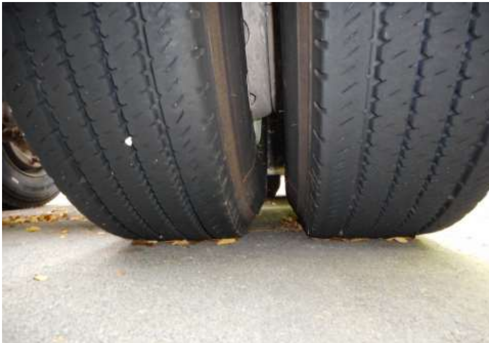
Photo 9 shows the condition of the rear left tyres of the Motor Lorry, which was observed to be in serviceable condition with remaining tread depth of approximately 9mm. The tyres, which were wrapped around standard steel wheel rim, were also observed to be sufficiently inflated for vehicular operation. There was also no damage found on all 8 steel wheel rims of the Motor Lorry.
