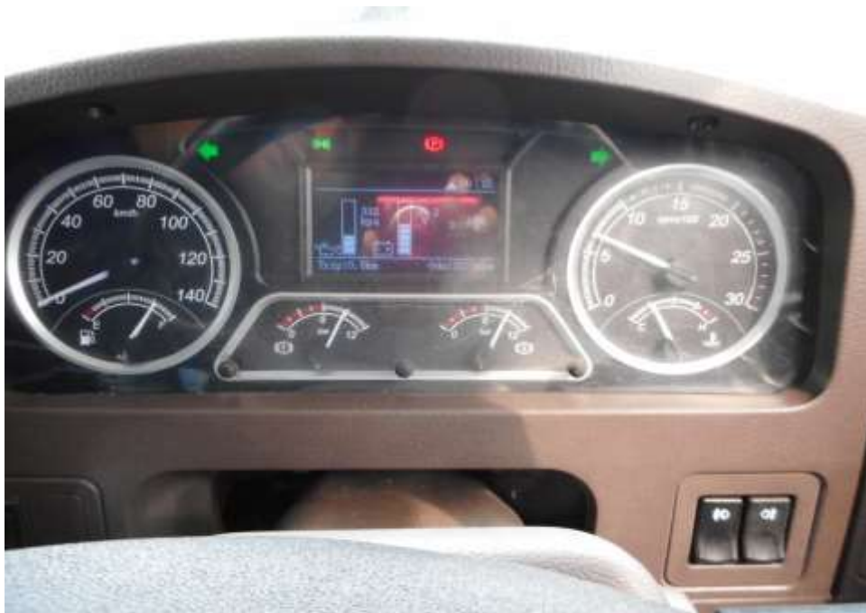
Photo 26 shows no warning lights illuminated on the instrument panel of the Motor Lorry after the engine was cranked. This would suggest that there was no abnormality to the various electronic operating systems of the Motor Lorry, like the ABS
