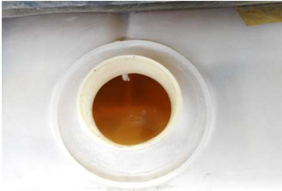
Photo 13 shows the engine coolant reservoir of the Motor Lorry at the time of my inspection. The engine coolant was observed to be of sufficient level and without any visible contamination.
