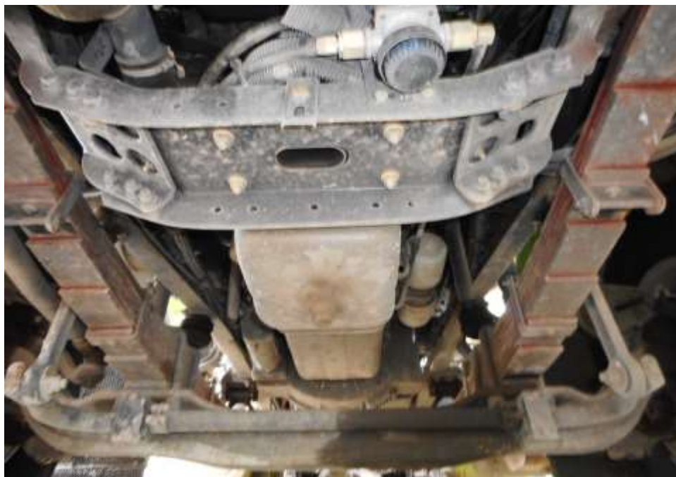
Photo 23 shows the undercarriage of the Motor Lorry, at the area where the engine housing located. I did not find any sign(s) or indication(s) of fluid leak and/or fluid stain(s) on the underside of the Motor Lorry.
