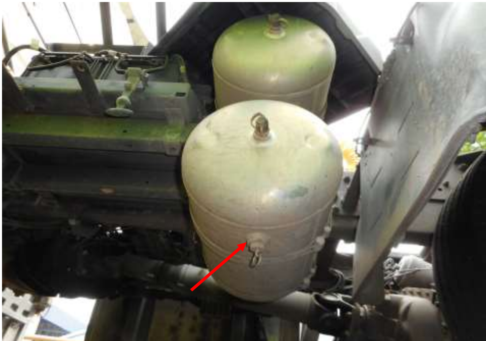
Photo 19 shows the air brake cylinder (arrowed) at the undercarriage of the Motor Lorry. I did not observe any leakage of air brake fluid at the time of my inspection of the Motor Lorry. My static tests of the Motor Lorry's braking system, along with my visual examination of the various mechanical components in the braking system had indicated that there was no internal leakage of pressure/vacuum. Hence the braking system of the Motor Lorry was likely to be in serviceable condition at the material time of accident.
