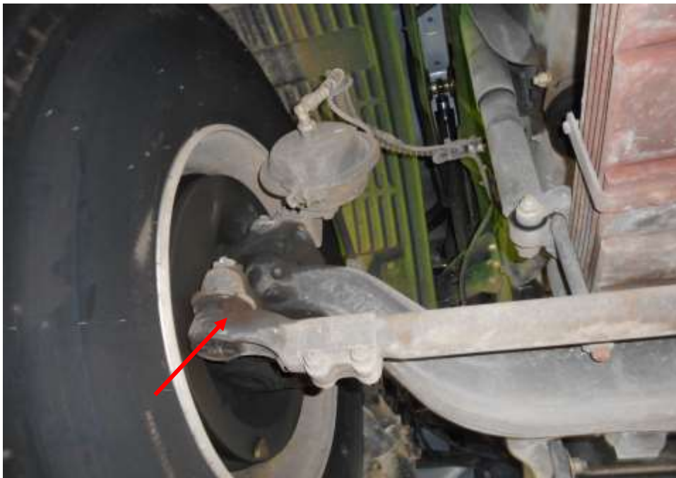
Photo 21 shows the various undercarriage components at the front left wheel of the Motor Lorry, in particular the steering tie rod end (arrowed). The various undercarriage components of the Motor Lorry were all found to be intact without any visible damage. There was also no sign of fluid stain(s) observed on the various undercarriage components.
