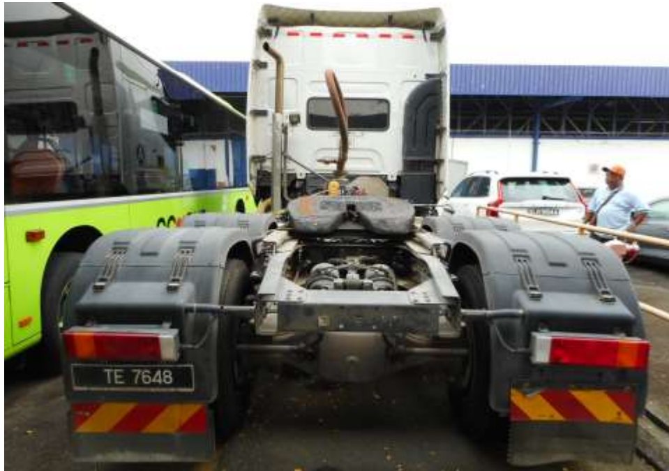
Photo 6 shows a general view of the Motor Lorry's rear body at the time of my inspection. The Motor Lorry was observed to be in good general condition and unaffected to by the accident.
