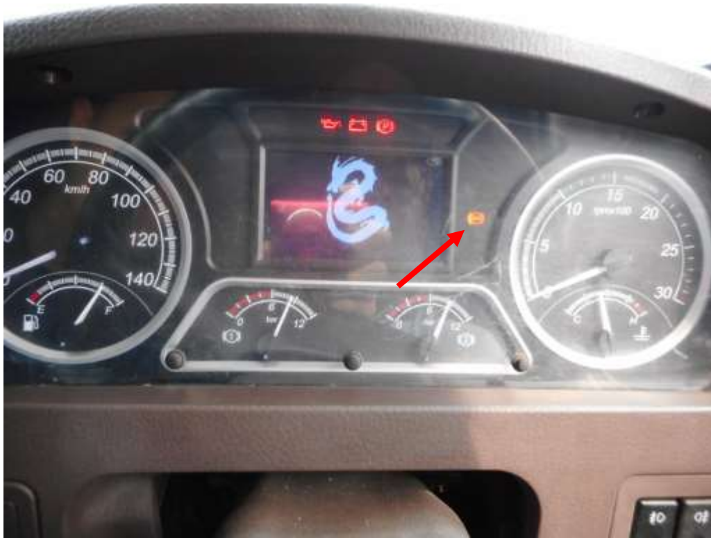
Photo 25 shows the warning light for Anti-Lock Brake System (ABS) appearing on the instrument panel of the Motor Lorry during the self-test of its various electronic operating systems when its engine was cranked.
