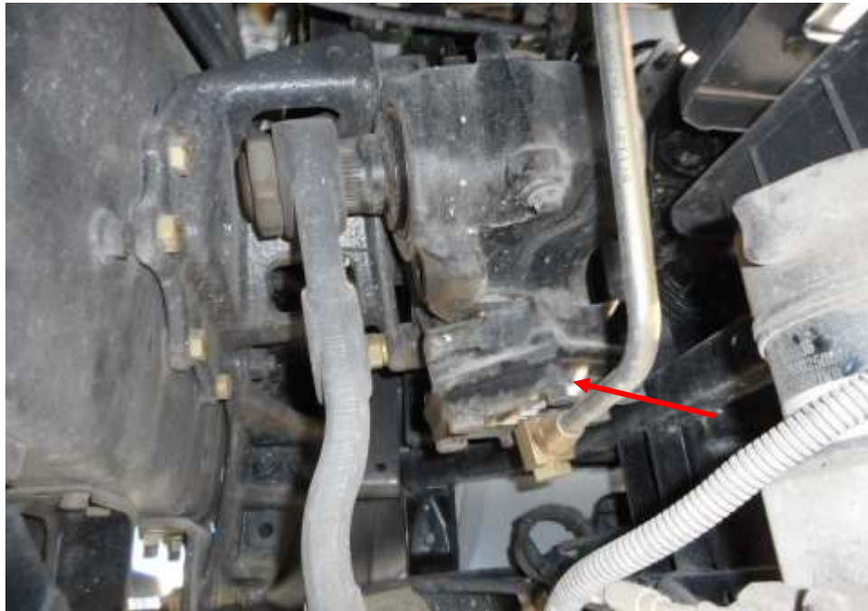
Photo 22 shows the steering box component (arrowed) at the undercarriage of the Motor Lorry was found to be intact without any visible damage. There was also no sign of fluid stain(s) observed on the various undercarriage components.
