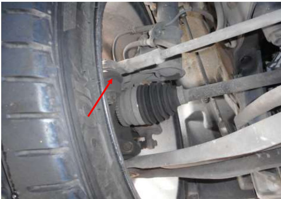
Photo 19 shows the various undercarriage components at the front left wheel of the Motor Car, which had included the steering tie rod (red arrow). The various undercarriage components of the Motor Car were all found to be intact without any visible damage.
