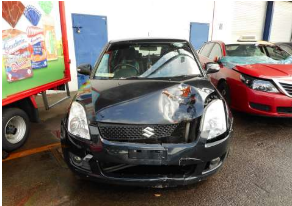
Photo 2 shows a general view of the Motor Car's front body at the time of my inspection. The Motor car was observed to have sustained moderate damage at its front portion. Its front windscreen, front bonnet, bonnet lock mechanism, front bumper, front number plate, front reinforcement and radiator was amongst the body parts that were damaged as a result of the accident.
