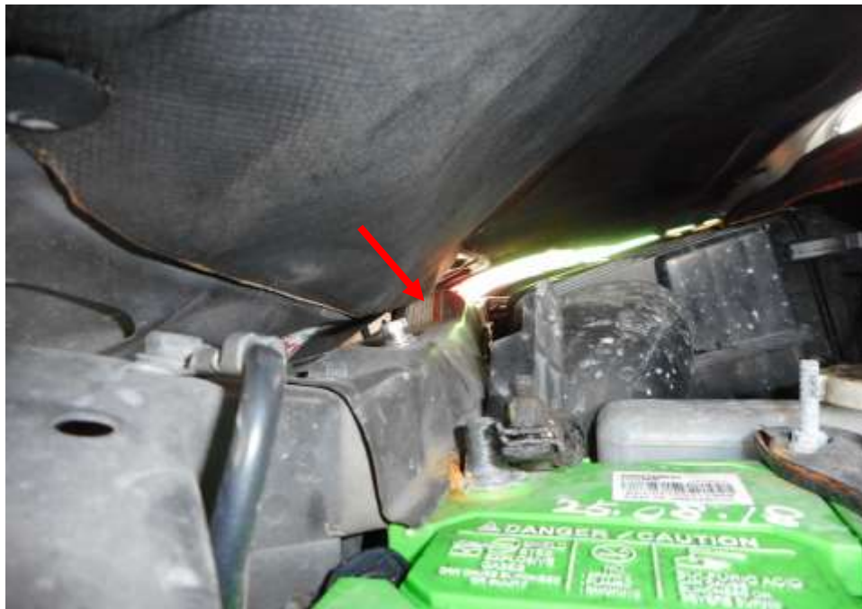
Photo 13 shows the damage to the locking mechanism (arrowed) Motor Car's front bonnet, rendering it unable to be unlocked and lifted up to carry out examination of the Motor Car's engine compartment as a result of the accident.
