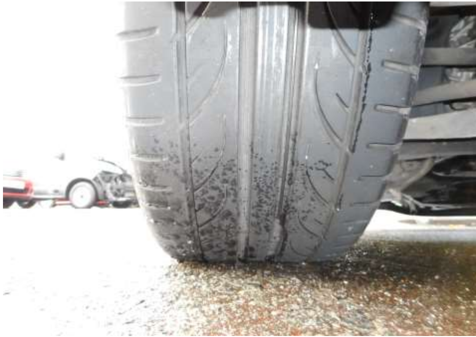
Photo 12 shows the condition of the front left tyre of the Motor Car, which was observed to be in serviceable condition with remaining tread depth of approximately 4.5mm. There was also no tear, cut or burst mark(s) on the outer and the inner sidewalls as well as across the tread of the Motor Car's 4 tyres.
