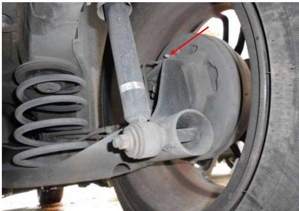
Photo 15 shows the brake hose/pipe (arrowed) at the rear right wheel of the Motor Car. No leakage of brake fluid was observed. Visual examination of the various components of the braking system like the drum brake, brake booster, brake pedal etc had revealed all to be intact and without visible damage.
