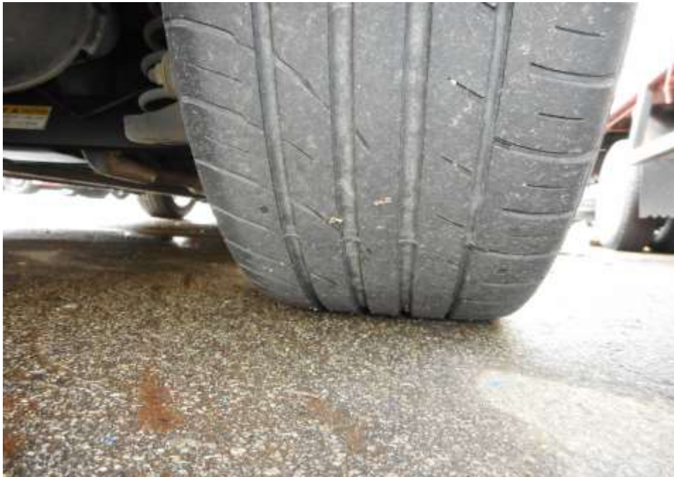
Photo 10 shows the condition of the rear right tyre of the Motor Car, which was observed to be in serviceable condition with remaining tread depth of approximately 5.2mm. The tyre was also observed to be sufficiently inflated for vehicular operation with no tear, cut or burst mark(s).
