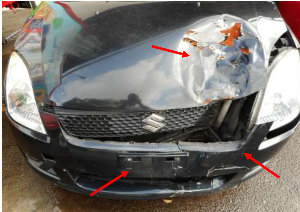
Photo 4 shows the close up view of the Motor Car's front body at the time of my inspection. The Motor car was observed to have sustained damage, its front bonnet, front bumper; front number plate (arrowed) was amongst the body parts that were damaged as a result of the accident.
