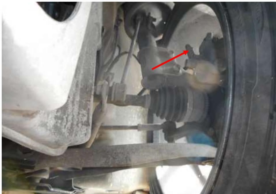
Photo 17 shows the brake hose/pipe (arrowed) at the front left wheel of the Motor Car. I did not observe any leakage of brake fluid at the time of my inspection of the Motor Car. Static tests of the Motor Car's braking system had indicated that there was no internal leakage of pressure/vacuum. The undercarriage components of the Motor Car were also all found to be intact and without any visible damage.
