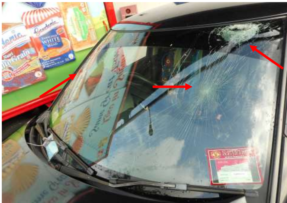
Photo 3 shows the close up view of the Motor Car's front body at the time of my inspection. The Motor car was observed to have sustained damage its front windscreen (arrowed) as a result of the accident.
