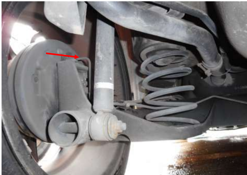
Photo 14 shows the brake hose/pipe (arrowed) at the rear left wheel of the Motor Car. I did not observe any leakage of brake fluid at the time of my inspection of the Motor Car. Static tests of the Motor Car's braking system had indicated that there was no internal leakage of pressure/vacuum. The undercarriage components of the Motor Car were also all found to be intact and without any visible damage.
