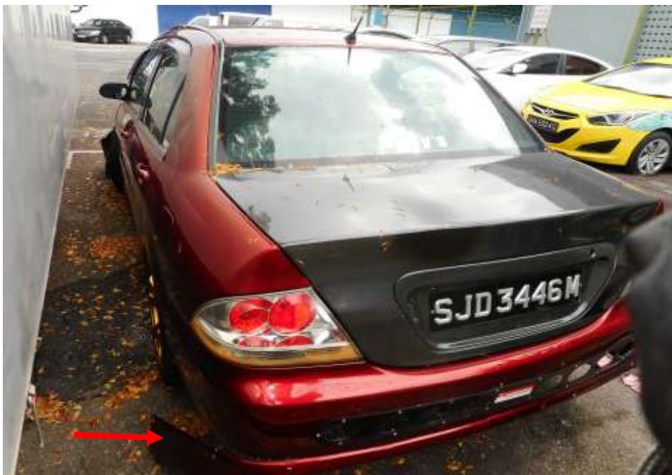
Photo 9 shows a general rear view of the Motor Car's left body panel at the time of my inspection. The rear bumper portion (arrowed) of the Motor Car was observed to have been damaged by the accident.
