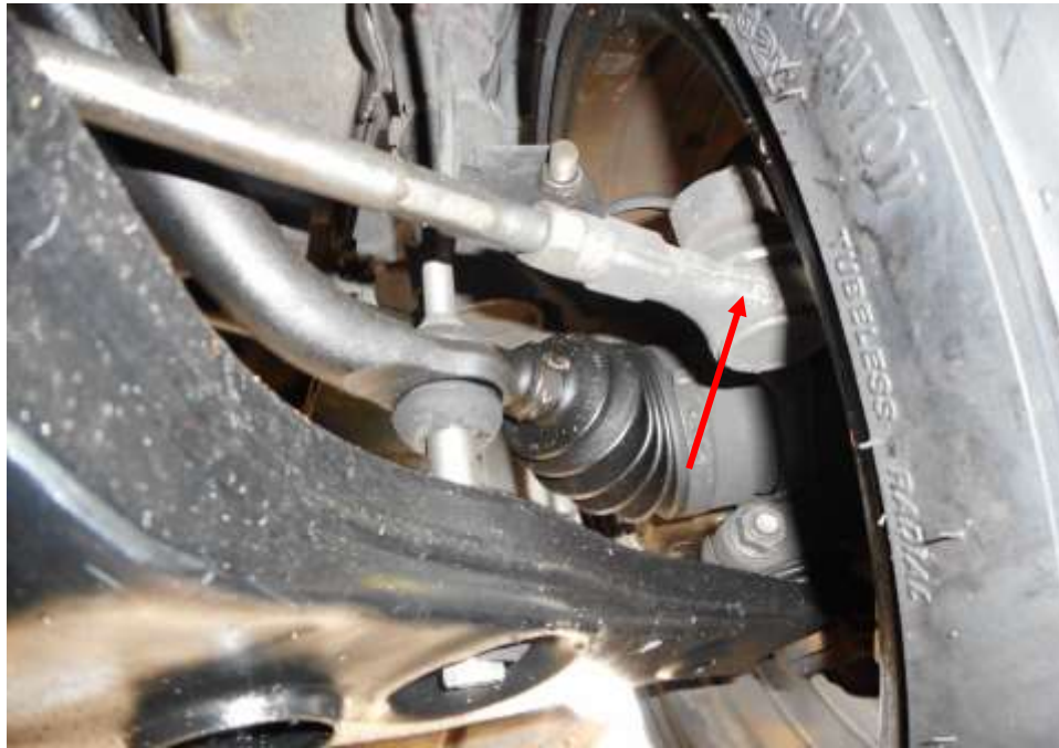
Photo 24 shows the various undercarriage components at the front right wheel of the Motor Car, which had included the steering tie rod (red arrow). The various undercarriage components of the Motor Car were all found to be intact without any visible damage.
