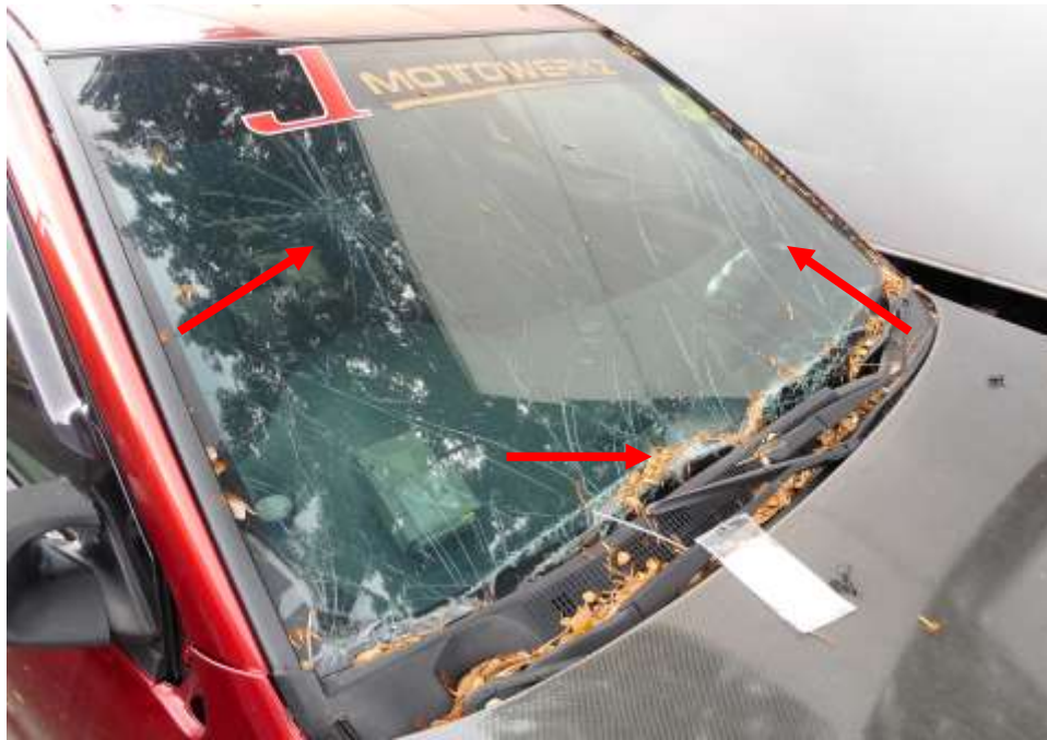
Photo 2 shows the close up view of the Motor Car's front body at the time of my inspection. The Motor car was observed to have sustained damage; its front windscreen (arrowed) as a result of the accident.
