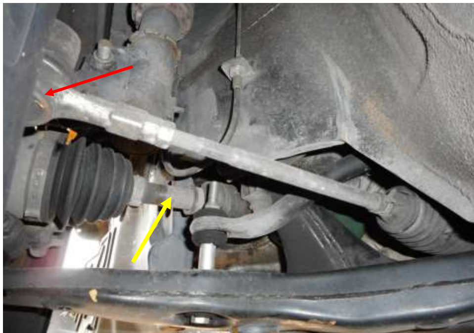
Photo 25 shows the various undercarriage components at the front left wheel of the Motor Car, in particular the steering tie rod (red arrow) and drive shaft (yellow arrow). The various steering components were all found to be intact, suggesting that the steering system of the Motor Car was likely to be in serviceable condition at the material time of accident. There was also no sign of fluid stain observed on the various undercarriage components at the front right wheel of the Motor Car.
