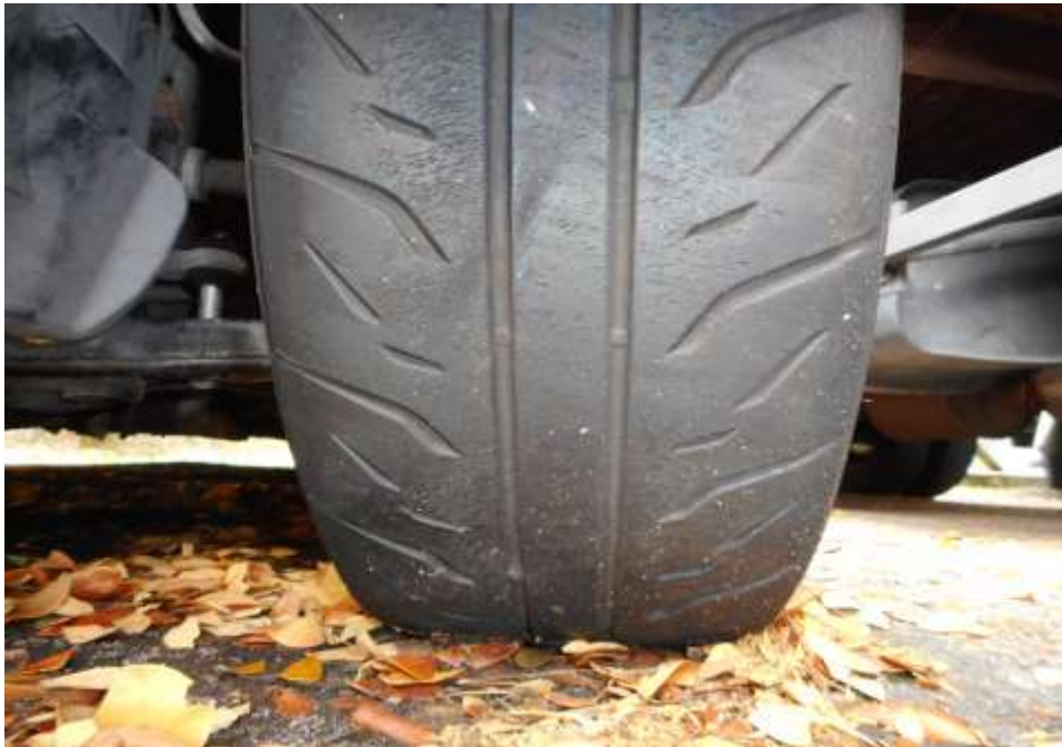
Photo 14 shows the condition of the front left tyre of the Motor Car, which was observed to be in serviceable condition with remaining tread depth of approximately 3.7mm. There was also no tear, cut or burst mark(s) on the outer and the inner sidewalls as well as across the tread of the Motor Car's 4 tyres.
