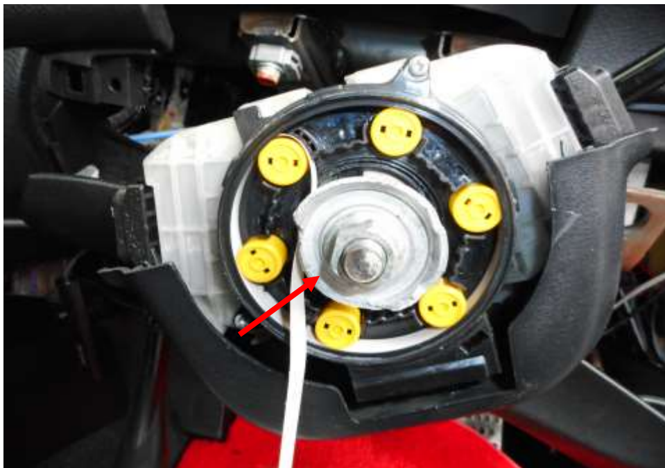
Photo 19 shows the close up view of the steering wheel of the Motor Car at time of my inspection of the Motor Car was observed to be damaged and missing (arrowed) as a result of the accident
