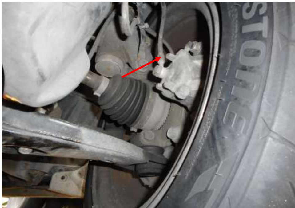
Photo 23 shows the brake hose/pipe (arrowed) at the front left wheel of the Motor Car. I did not observe any leakage of brake fluid at the time of my inspection of the Motor Car. Static tests of the Motor Car's braking system had indicated that there was no internal leakage of pressure/vacuum. The undercarriage components of the Motor Car were also all found to be intact and without any visible damage.
