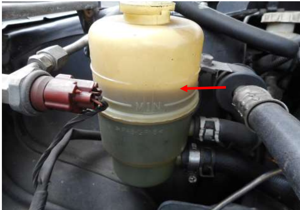
Photo 16 shows the brake fluid reservoir of the Motor Car at the time of my inspection. The brake fluid was observed to be of sufficient level (arrowed) and without any visible contamination.
