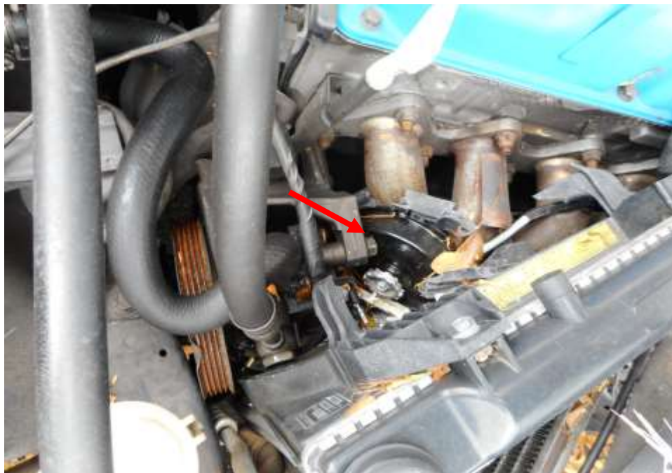
Photo 7 shows a close up view of the front portion of the Motor Car at the time of my inspection. The ignition system (arrowed) of the Motor Car was observed to have been damaged as a result of the induced impact as a result of the accident
