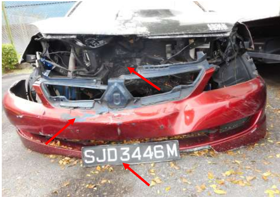
Photo 4 shows the general view of the Motor Car's front body at the time of my inspection. The Motor car was observed to have sustained damage, its front bumper; front number plate (arrowed) was amongst the body parts that were damaged as a result of the accident.
