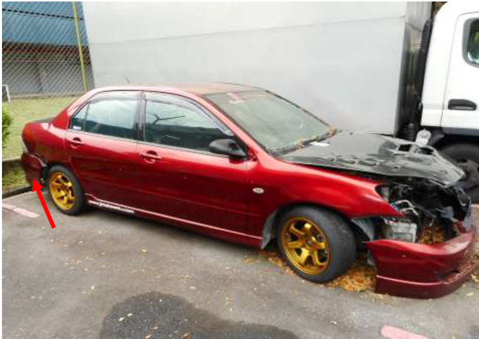
Photo 8 shows a general view of the Motor Car's right body panel at the time of my inspection. The rear bumper portion (arrowed) of the Motor Car was observed to have been damaged by the accident.
