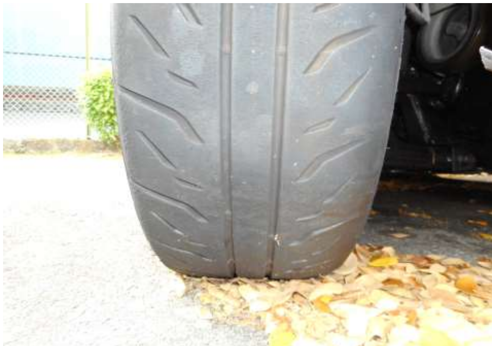
Photo 11 shows the condition of the front right tyre of the Motor Car, which was observed to be in serviceable condition with remaining tread depth of approximately 3.7mm. The tyre was sufficiently inflated for vehicular operation with no tear, cut or burst mark(s) on the outer and the inner sidewalls as well as across the tread. The 4 tyres of the Motor Car were wrapped around standard alloy wheel rims without any damage.
