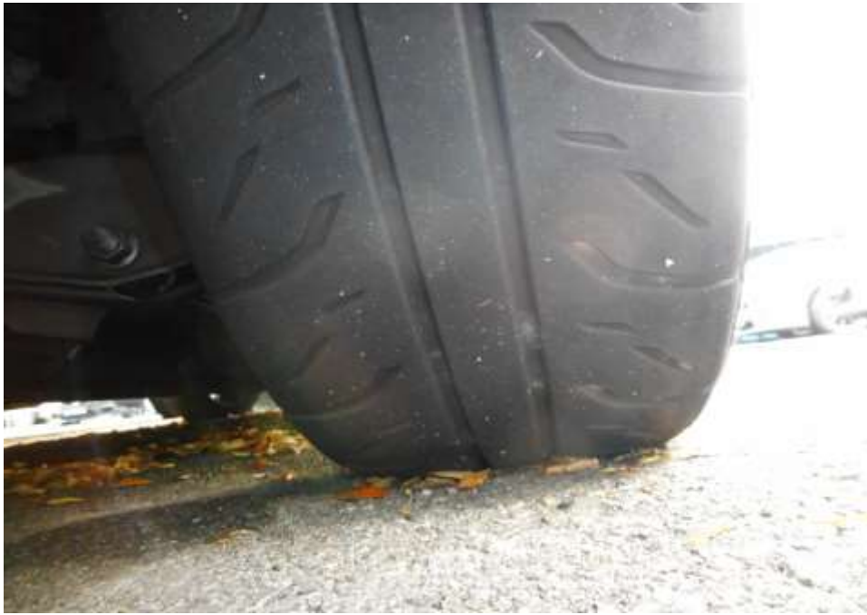
Photo 12 shows the condition of the rear right tyre of the Motor Car, which was observed to be in serviceable condition with remaining tread depth of approximately 4.5mm. The tyre was also observed to be sufficiently inflated for vehicular operation with no tear, cut or burst mark(s).
