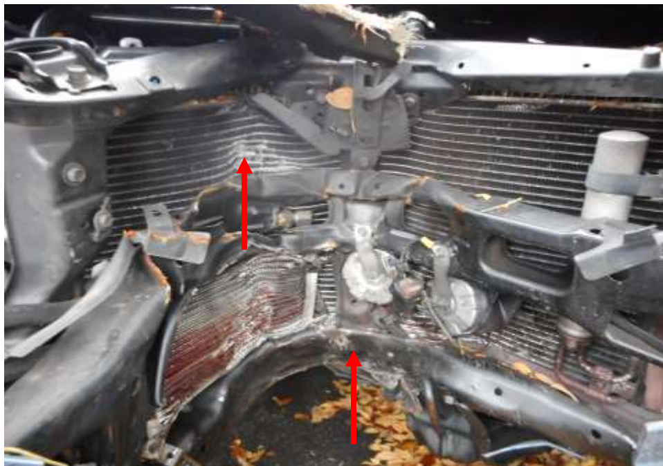
Photo 5 shows the close up view of the Motor Car's front body at the time of my inspection. The Motor car was observed to have sustained damage, its front radiator and front reinforcement (arrowed) was amongst the body parts that were damaged as a result of the accident.
