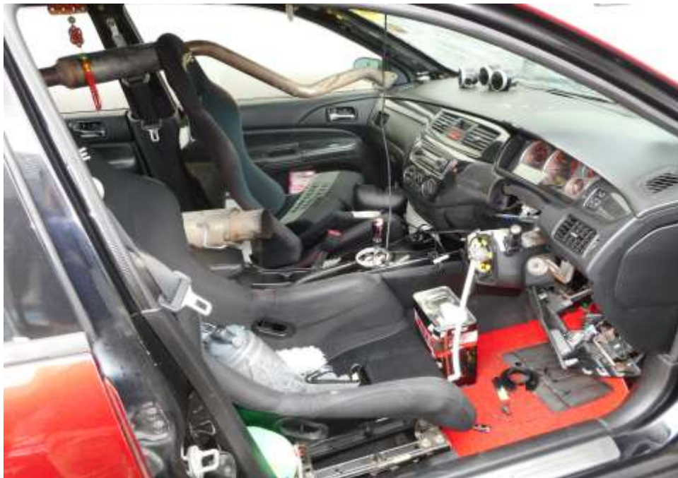
Photo 18 shows the interior cabin of the Motor Car. The steering wheel at time of my inspection of the Motor Car was observed to be damaged and missing as a result of the accident
