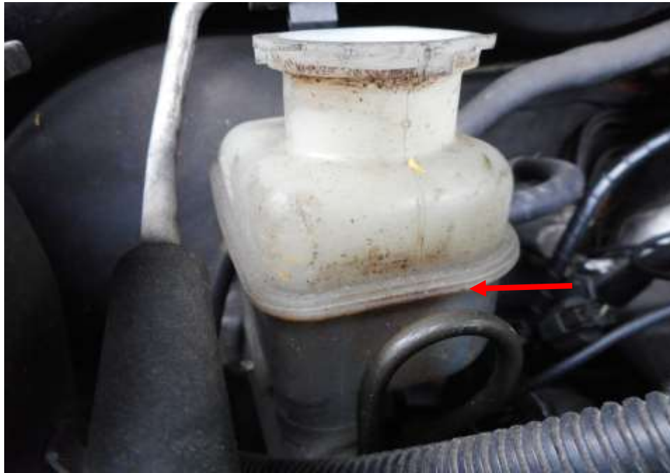
Photo 17 shows the power steering dip stick of the Motor Car at the time of my inspection. The power steering fluid was observed to be of sufficient level and with visible contamination.
