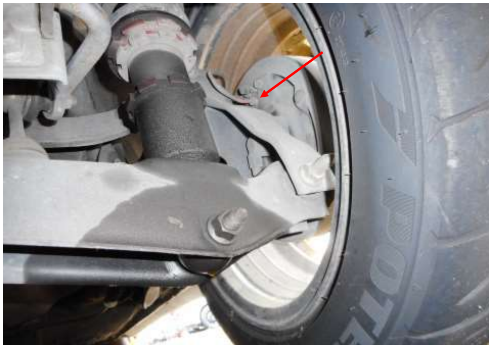
Photo 21 shows the brake hose/pipe (arrowed) at the rear right wheel of the Motor Car. No leakage of brake fluid was observed. Visual examination of the various components of the braking system like the drum brake, brake booster, brake pedal etc had revealed all to be intact and without visible damage.
