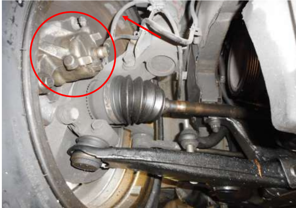
Photo 22 shows the brake hose/pipe (arrowed) at the front right wheel of the Motor Car. No leakage of brake fluid was observed. Visual examination of the various components of the braking system like the brake caliper (circled), brake booster, brake pedal etc had revealed all to be intact and without visible damage.
