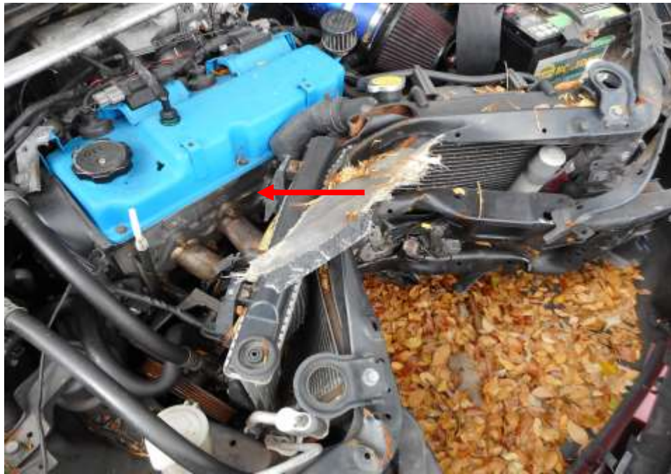
Photo 6 shows a close up view of the front portion of the Motor Car at the time of my inspection. The engine system (arrowed) of the Motor Car was observed to have been damaged by an induced impact as a result of the accident
