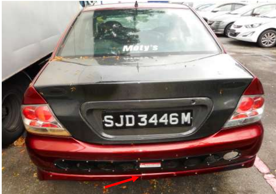
Photo 10 shows a general view of the Motor Car's rear body at the time of my inspection. The rear bumper portion of the Motor Car was observed to have been damaged by the accident.
