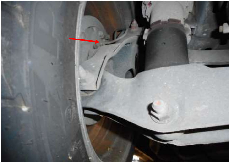
Photo 20 shows the brake hose/pipe (arrowed) at the rear left wheel of the Motor Car. I did not observe any leakage of brake fluid at the time of my inspection of the Motor Car. Static tests of the Motor Car's braking system had indicated that there was no internal leakage of pressure/vacuum. The undercarriage components of the Motor Car were also all found to be intact and without any visible damage.
