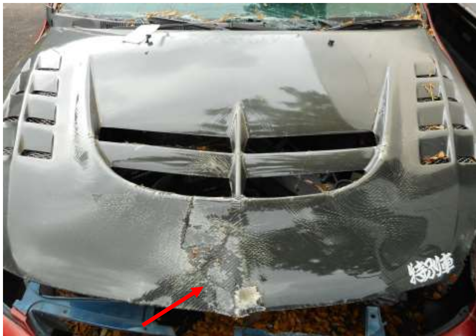
Photo 3 shows the close up view of the Motor Car's front body at the time of my inspection. The Motor car was observed to have sustained damage; its front bonnet (arrowed) was amongst the body parts that were damaged as a result of the accident.
