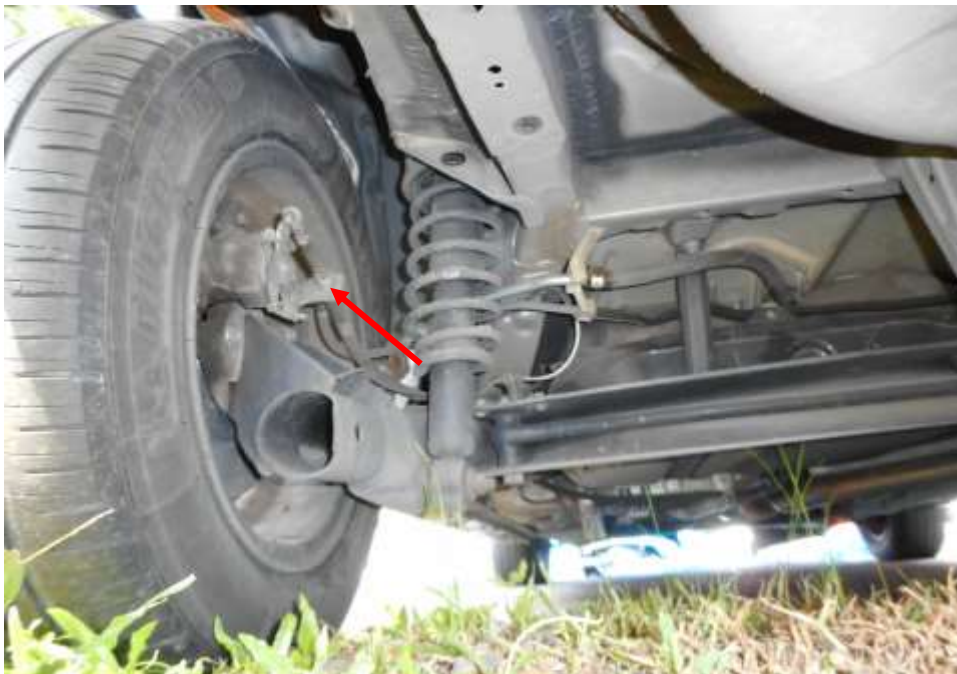
Photo 21 shows the various undercarriage components at the rear left wheel of the Motor Car, in particular the brake hose (arrowed). I did not observe any leakage of brake fluid at the 4 wheels of the Motor Car. My visual inspection of the various mechanical components of the Motor Car's braking system revealed all to be intact and without visible damage.
