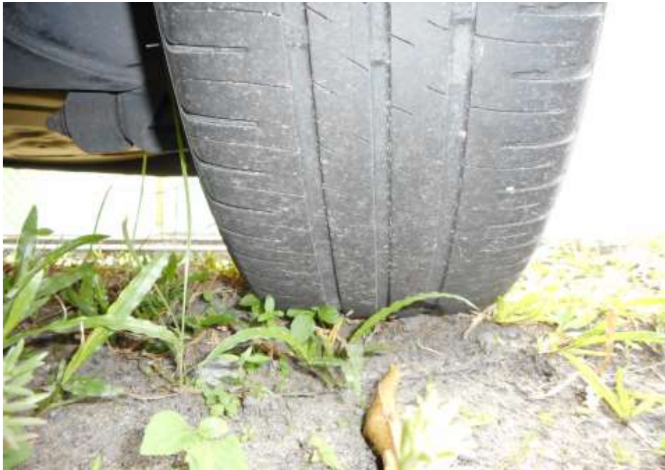
Photo 14 shows the condition of the rear left tyre of the Motor Car, which was observed to be in serviceable condition with remaining tread depth of approximately 3.3mm. There was no tear, cut or burst mark(s) on the outer and the inner sidewalls as well as across the tread of this tyre.
