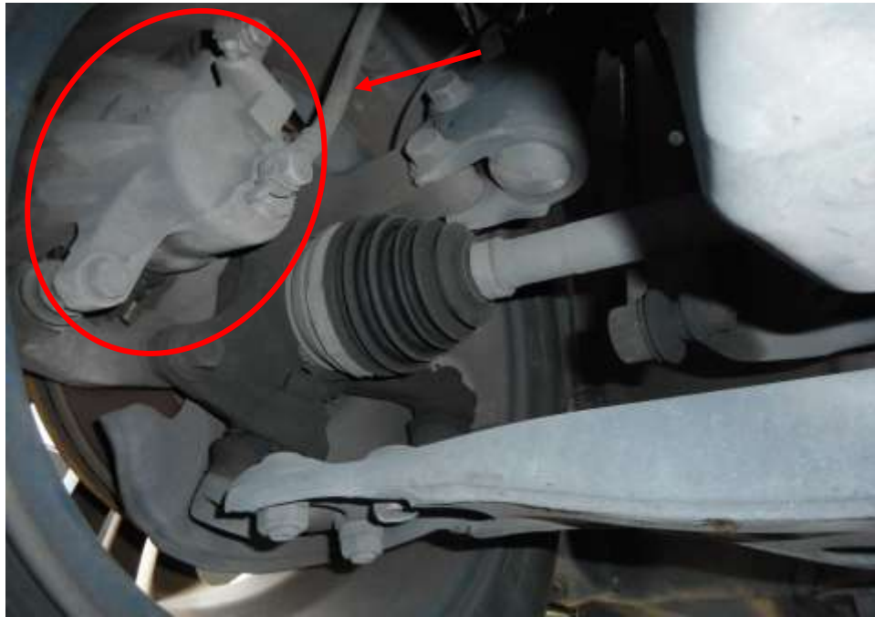
Photo 18 shows the brake hose (arrowed) at the front right wheel of the Motor Car. I did not observe any leakage of brake fluid at the 4 wheels of the Motor Car. My visual inspection of the various mechanical components of the Motor Car's braking system, including its brake caliper (circled), revealed all to be intact and without visible damage.
