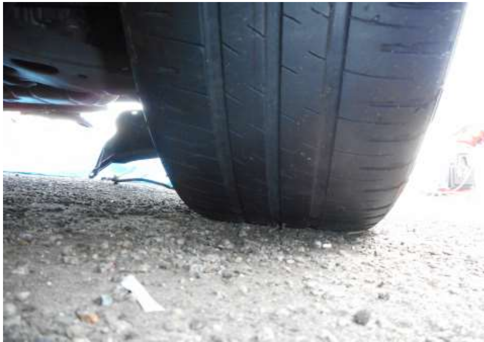
Photo 12 shows the condition of the front right tyre of the Motor Car, which was observed to be in serviceable condition with remaining tread depth of approximately 3mm. The tyre was sufficiently inflated for vehicular operation with no tear, cut or burst mark(s) on the outer and the inner sidewalls as well as across the tread. The 4 tyres of the Motor Car were wrapped around standard alloy wheel rims without any damage.
