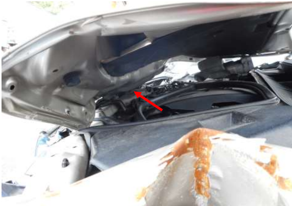
Photo 16 shows the damage to the locking mechanism (arrowed) Motor Car's front bonnet, rendering it unable to be unlocked and lifted up to carry out examination of the Motor Car's engine compartment as a result of the accident.
