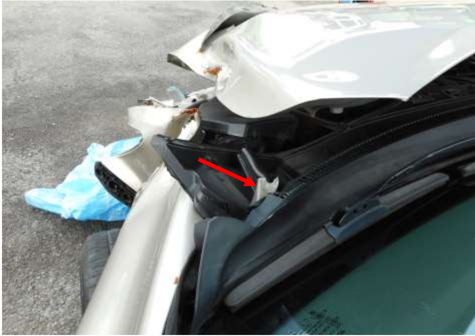
Photo 9 shows a close up view of the left bonnet hinge of the Motor Car at the time of my inspection. The left bonnet hinge of the Motor Car was observed to have been damaged as a result of the accident. (arrowed)
