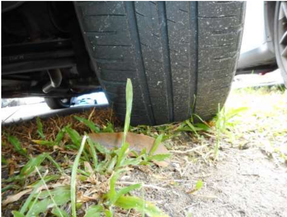
Photo 13 shows the condition of the rear right tyre of the Motor Car, which was observed to be in serviceable condition with remaining tread depth of approximately 3.3mm. There was no tear, cut or burst mark(s) on the outer and the inner sidewalls as well as across the tread of this tyre.
