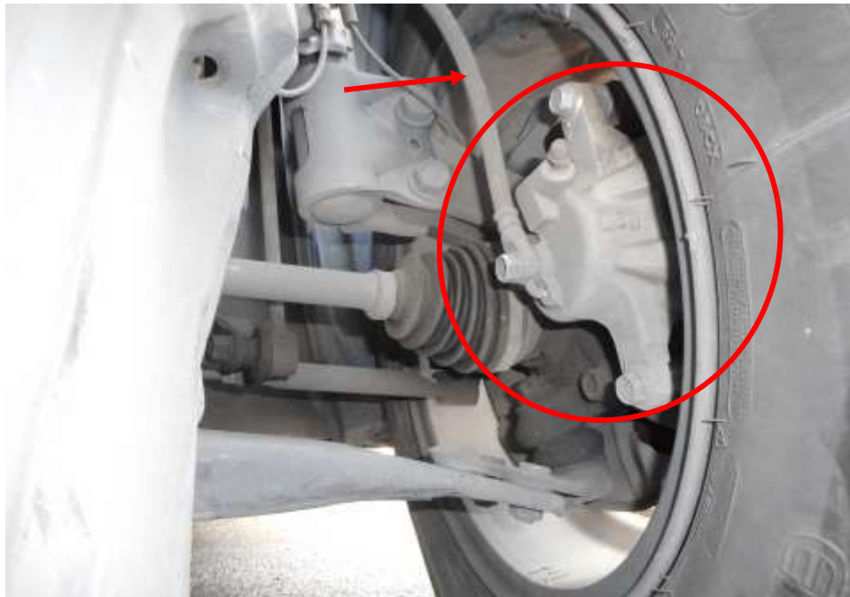
Photo 19 shows the brake hose (arrowed) at the front left wheel of the Motor Car. I did not observe any leakage of brake fluid at the 4 wheels of the Motor Car. My visual inspection of the various mechanical components of the Motor Car's braking system, including its brake caliper (circled), revealed all to be intact and without visible damage.
