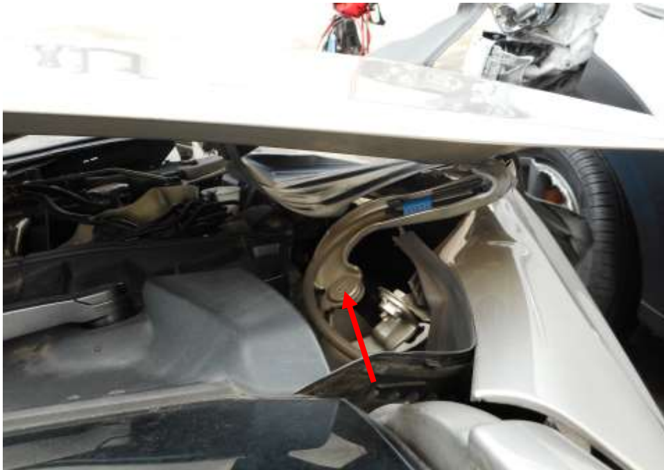
Photo 8 shows a close up view of the right bonnet hinge of the Motor Car at the time of my inspection. The right bonnet hinge of the Motor Car was observed to have been damaged as a result of the accident. (arrowed)
