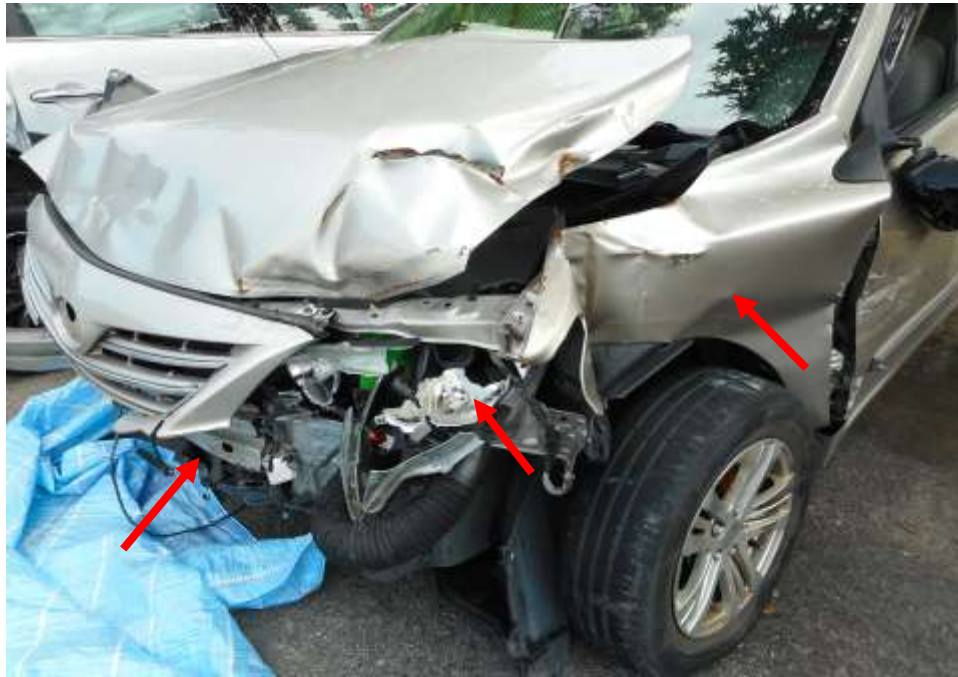
Photo 5 shows a close up view of the front portion of the Motor Car at the time of my inspection. The bonnet, front bumper, front number plate right fender and right head lamp (arrowed) of the Motor Car was observed to have been damaged as a result of the accident
