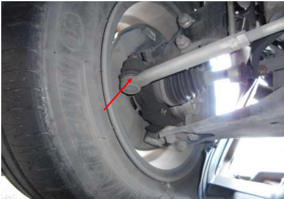
Photo 17 shows the undercarriage components at the front left wheel of the Motor Car. My checks on the underside of the Motor Car revealed damage to the various undercarriage components, the steering rack and pinion, tie rods, tie rod ends and ball joints (arrowed) revealed that these components were all generally in good condition.
