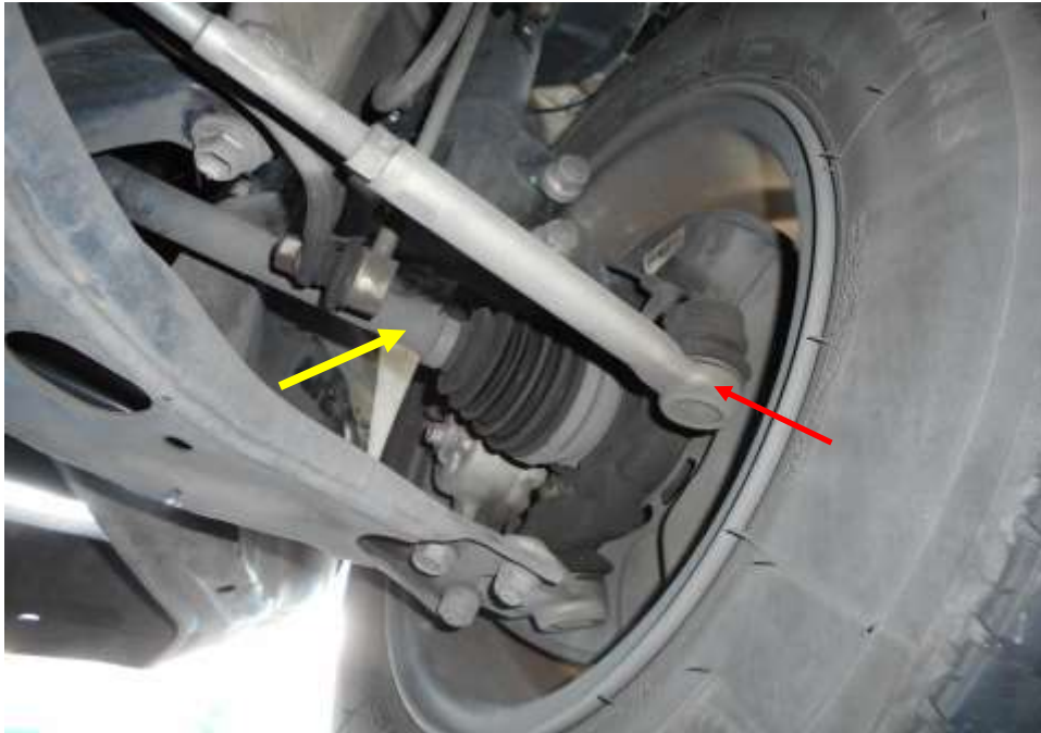
Photo 16 shows the various undercarriage components at the front right wheel of the Motor Car, which had included the steering tie rod (red arrow) and front left drive shaft (yellow arrow). The various undercarriage components of the Motor Car were all found to be intact without any visible damage.
