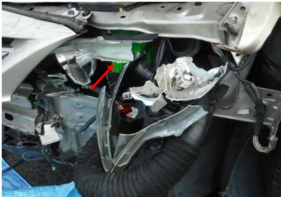
Photo 6 shows a close up view of the front portion of the Motor Car at the time of my inspection. The battery and ignition system (arrowed) of the Motor Car was observed to have been damaged as a result of the accident
