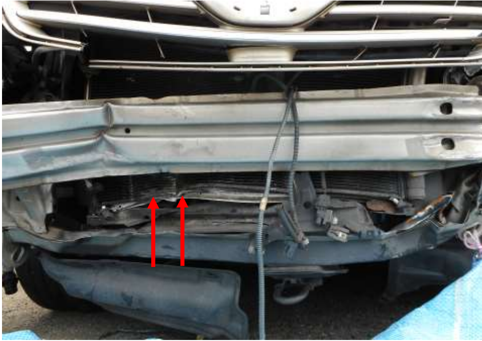
Photo 7 shows a close up view of the front portion of the Motor Car at the time of my inspection. The radiator of the Motor Car was observed to have been damaged by an induced impact (arrowed) as a result of the accident
