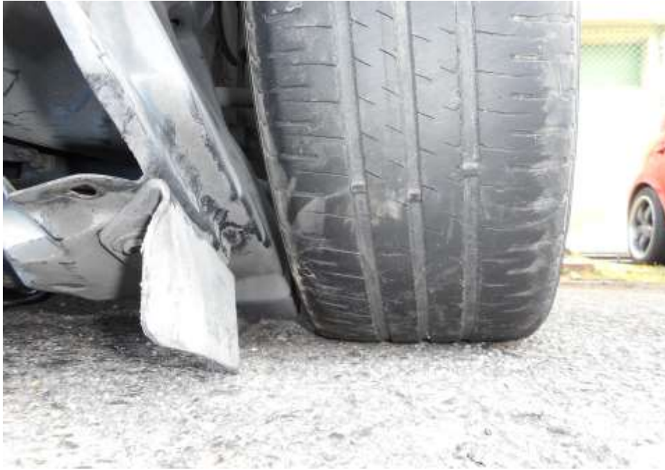
Photo 15 shows the condition of the front left tyre of the Motor Car, which was observed to be in serviceable condition with remaining tread depth of approximately 3mm. There was no tear, cut or burst mark(s) on the outer and the inner sidewalls as well as across the tread of this tyre, however observed to be deflated due to damage to the rims.
