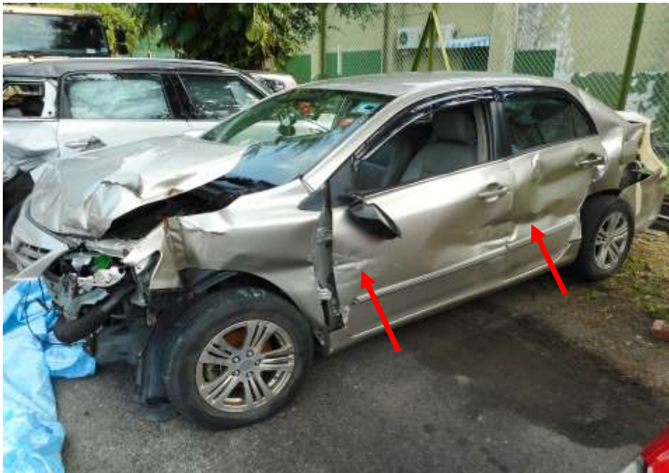
Photo 10 shows a general view of the front left portion of the Motor Car at the time of my inspection. The left door panels (arrowed) of the Motor Car were observed to have been damaged as a result of the accident.
