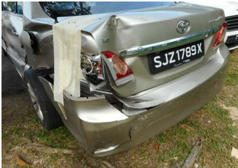
Photo 2 shows a close up view of the rear portion of the Motor Car at the time of my inspection. The rear portion of the Motor Car was observed to have been damaged by the accident. Its bonnet, left brake lamp, left body panel and bumper as a result of the accident.
