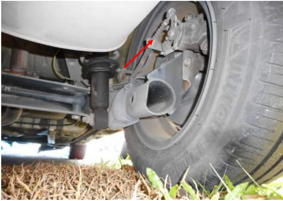
Photo 20 shows the various undercarriage components at the rear right wheel of the Motor Car, in particular the brake hose (arrowed). I did not observe any leakage of brake fluid at the 4 wheels of the Motor Car. My visual inspection of the various mechanical components of the Motor Car's braking system revealed all to be intact and without visible damage.
