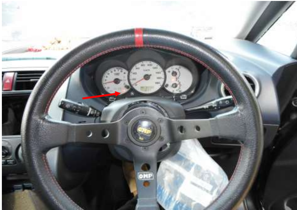
Photo 27 shows the aftermarket steering without its airbag component which triggered the warning lights of the Supplemental Restraint System (SRS) to remain illuminated on the instrument panel (arrowed) of the Motor Car after the engine was cranked.
