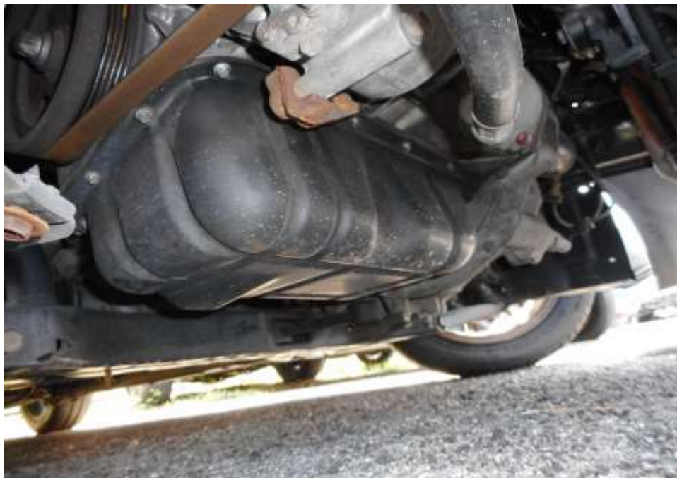
Photo 23 shows the undercarriage of the Motor Car, at the area where the engine housing and transmission housing are located. I did not find any sign(s) or indication(s) of fluid leak and/or fluid stain(s) on the underside of the Motor Car.
