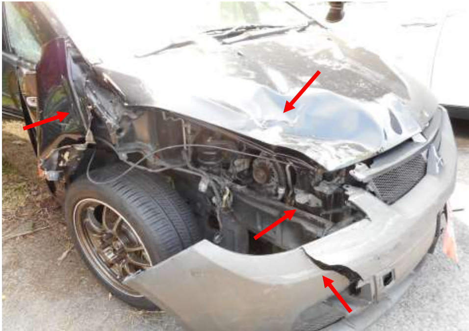
Photo 3 shows a close up view of the front right portion of the Motor Car at the time of my inspection. The Motor Car was also observed to have sustained extensive damage at its frontal portal, damaged parts had included its, front bonnet, front bumper, right fender, front right headlamp (arrowed) were amongst the body parts that were observed to have been damaged as a result of the accident.
