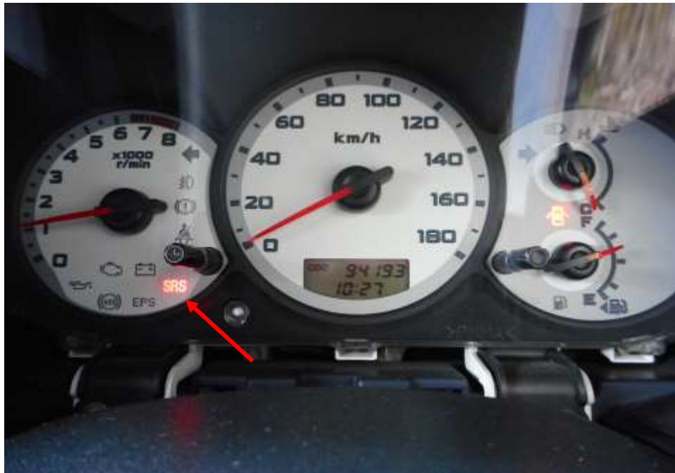
Photo 26 shows only the Supplemental Restraint System (SRS) lights remained illuminated on the instrument panel of the Motor Car after the engine was cranked. However the ABS and EPS light disappear and this would suggest that there was no abnormality to this various electronic operating systems of the Motor Car.
