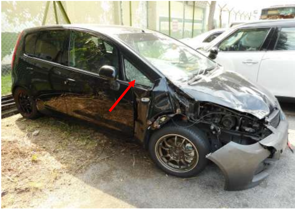
Photo 5 shows a general view of the front right portion of the Motor Car at the time of my inspection. The right side windscreen (arrowed) of the Motor Car was observed to have been damaged as a result of the accident.
