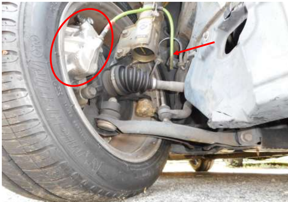
Photo 19 shows the brake hose (arrowed) at the front right wheel of the Motor Car. I did not observe any leakage of brake fluid at the 4 wheels of the Motor Car. My visual inspection of the various mechanical components of the Motor Car's braking system, including its brake caliper (circled), revealed all to be intact and without visible damage.
