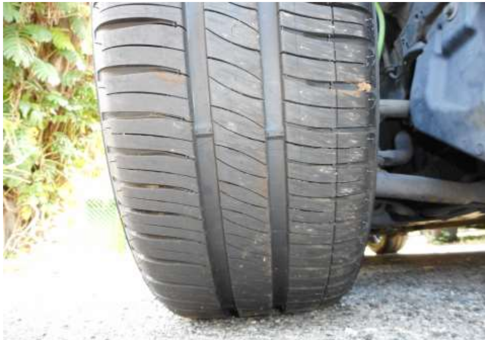
Photo 9 shows the condition of the front right tyre of the Motor Car, which was observed to be in serviceable condition with remaining tread depth of approximately 7.4mm. There was no tear, cut or burst mark(s) on the outer and the inner sidewalls as well as across the tread of this tyre.
