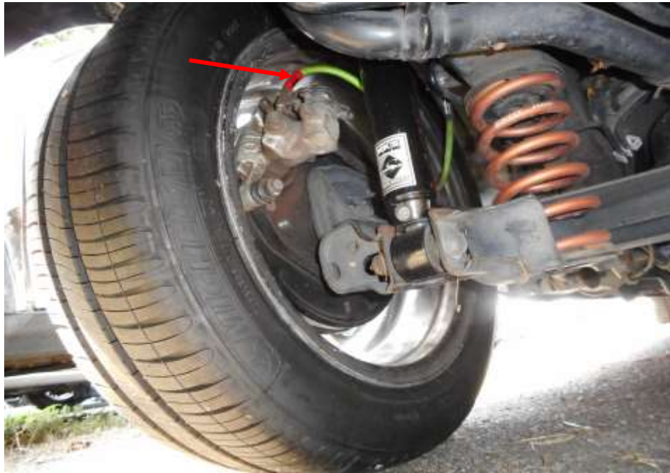
Photo 22 shows the brake hose/pipe (arrowed) at the rear left wheel of the Motor Car. I did not observe any leakage of brake fluid at the time of my inspection of the Motor Car. Static tests of the Motor Car's braking system had indicated that there was no internal leakage of pressure/vacuum. The undercarriage components of the Motor Car were also all found to be intact and without any visible damage.
