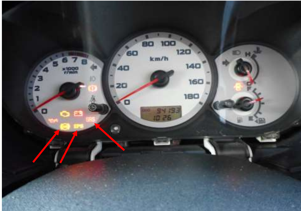
Photo 25 shows the warning light for Anti-Lock Brake System (ABS), Electronic Power Steering (EPS) and Supplemental Restraint System (SRS) appearing on the instrument panel of the Motor Car during the self-test of its various electronic operating systems when its engine was cranked.
