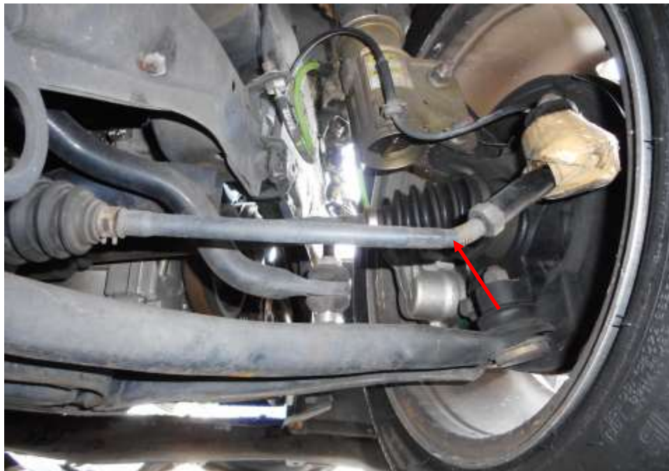
Photo 17 shows the undercarriage components at the front right wheel of the Motor Car. My checks on the underside of the Motor Car revealed damage to the steering tie rod (arrowed) as a result of the accident.
