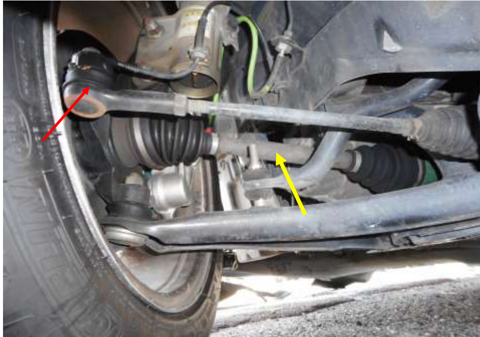
Photo 18 shows the various undercarriage components at the front left wheel of the Motor Car, which had included the steering tie rod (red arrow) and front left drive shaft (yellow arrow). The various undercarriage components of the Motor Car were all found to be intact without any visible damage.
