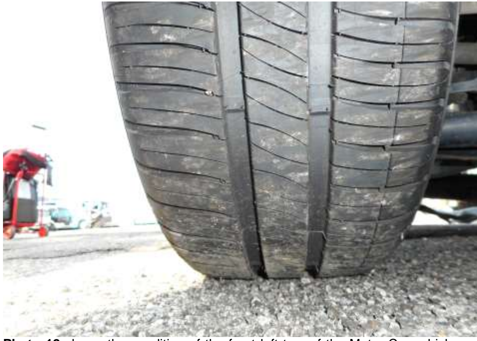
Photo 12 shows the condition of the front left tyre of the Motor Car, which was observed to be in serviceable condition with remaining tread depth of approximately 7.3mm. There was no tear, cut or burst mark(s) on the outer and the inner sidewalls as well as across the tread of this tyre.
