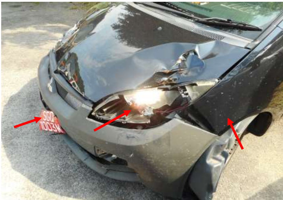
Photo 4 shows a close up view of the front left portion of the Motor Car at the time of my inspection. The Motor Car was also observed to have sustained extensive damage at its frontal portal, damaged parts had included its, front bumper, left fender, front left headlamp and front number plate (arrowed) were amongst the body parts that were observed to have been damaged as a result of the accident.
