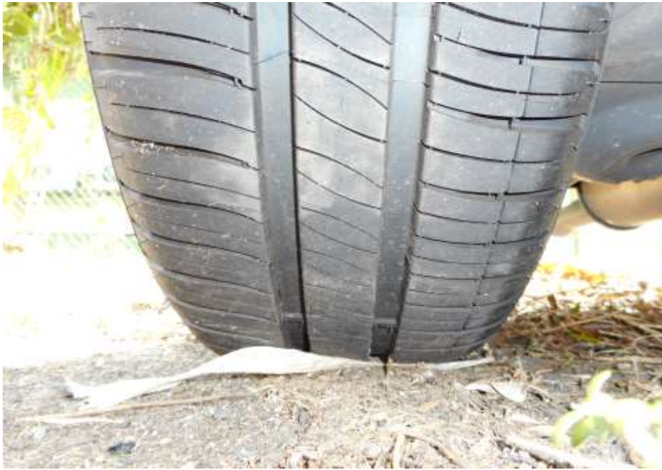
Photo 10 shows the condition of the rear right tyre of the Motor Car, which was observed to be in serviceable condition with remaining tread depth of approximately 7.2mm. There was no tear, cut or burst mark(s) on the outer and the inner sidewalls as well as across the tread of this tyre.
