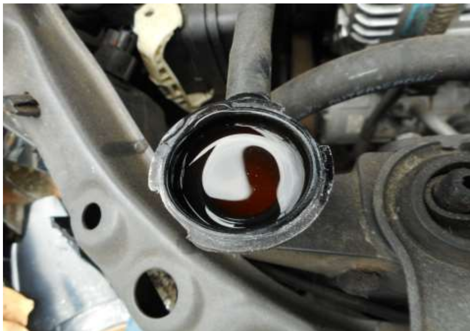
Photo 14 shows the engine coolant reservoir of the Motor Car at the time of my inspection. The engine coolant was observed to be of sufficient level and without any visible contamination.
