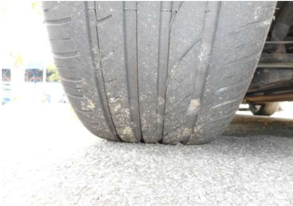
Photo 10 shows the condition of the rear left tyres of the Motor Car, which was observed to be in serviceable condition with remaining tread depth of approximately 4.2mm. The tyres, which were wrapped around standard alloy wheel rim, were also observed to be sufficiently inflated for vehicular operation. There was also no damage found on all 4 alloy wheel rims of the Motor Car.
