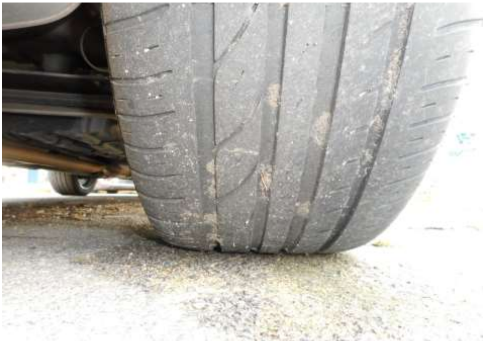
Photo 9 shows the condition of the rear right tyre of the Motor Car, which was observed to be in serviceable condition with remaining tread depth of approximately 4.6mm. The tyre, which was wrapped around standard alloy wheel rim, was also observed to be sufficiently inflated for vehicular operation.
