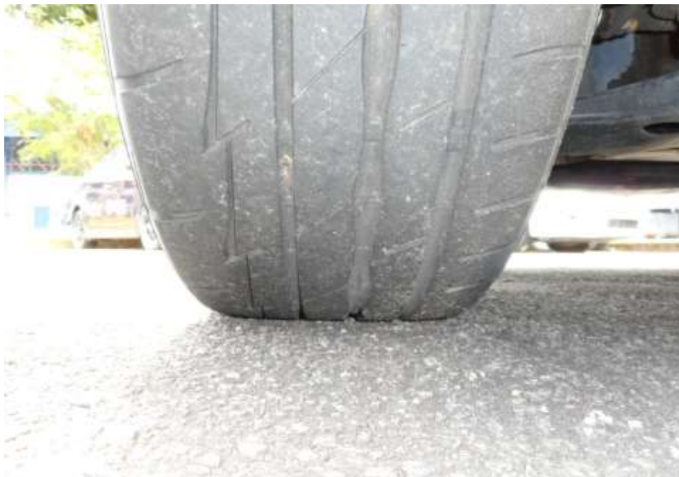
Photo 11 shows the condition of the rear right tyres of the Motor Car, which were observed to be in serviceable condition with remaining, tread depth of approximately 4.4mm. There was also no tear, cut or burst mark(s) on the outer and the inner sidewalls as well as across the tread of the 4 tyres that were fitted on the Motor Car.
