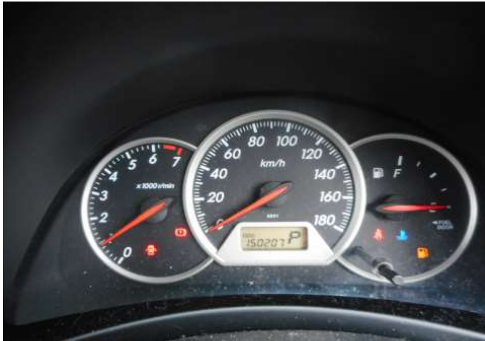
Photo 25 shows no warning lights illuminated on the instrument panel of the Motor Car after the engine was cranked. This would suggest that there was no abnormality to the various electronic operating systems of the Motor Car, like the ABS, SRS and EPS.
