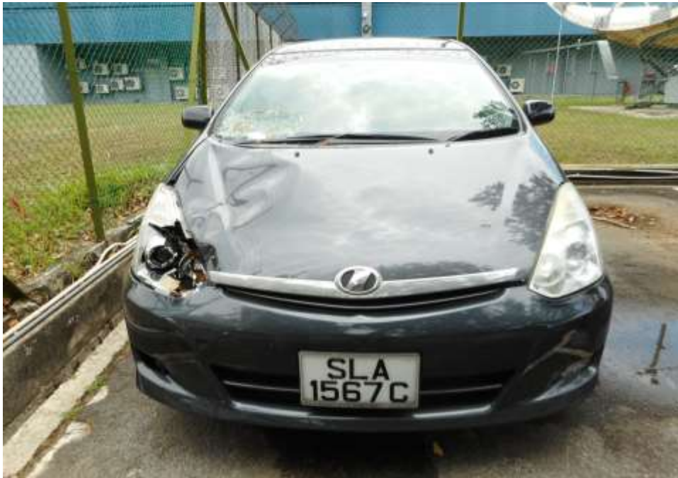
Photo 2 shows a general view of the Motor Car's frontal portion at the time of my inspection. It appeared to have sustained moderate damage at its frontal portion. Its front windscreen, front bonnet, front bumper and front right headlamp were damage at the time of my inspection.
