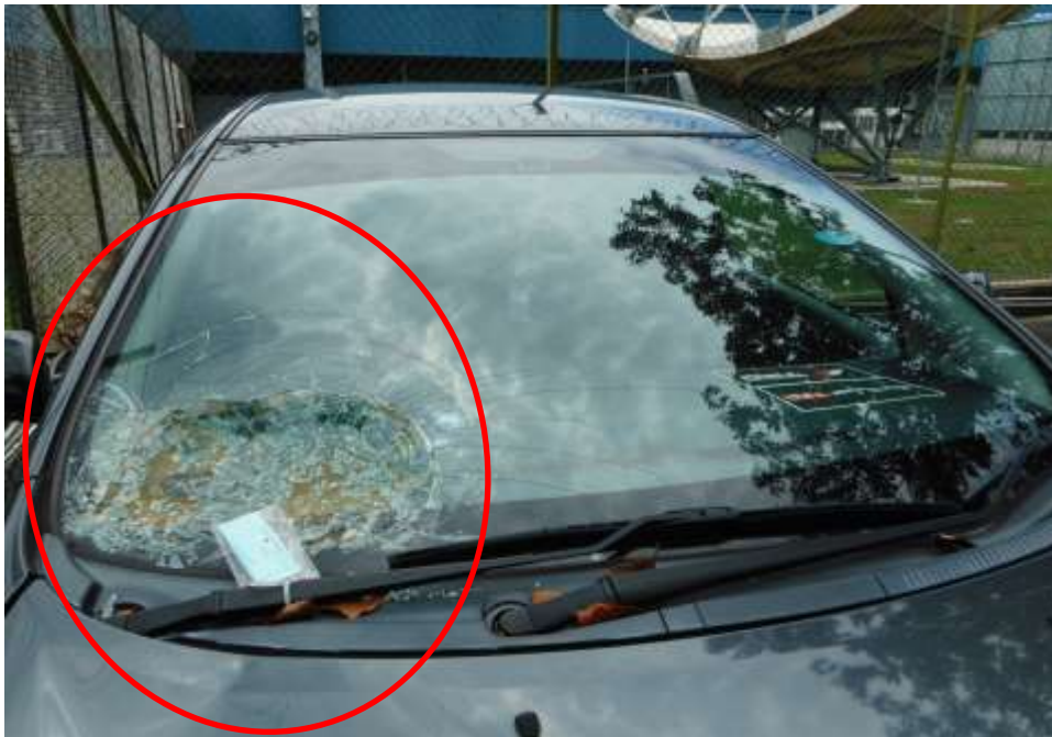
Photo 3 shows a close up view of the Motor Car's frontal portion at the time of my inspection. Its front windscreen (circled) was damage at the time of my inspection.
