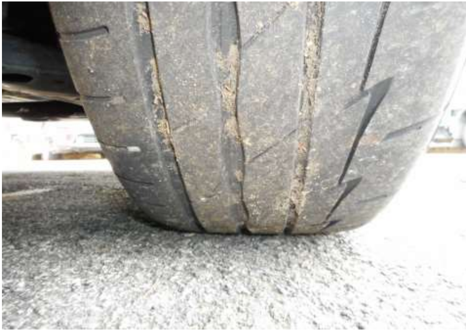
Photo 8 shows the condition of the front right tyre of the Motor Car, which was observed to be in serviceable condition with remaining tread depth of approximately 4.5mm. The tyre, which was wrapped around standard alloy wheel rim, was also observed to be sufficiently inflated for vehicular operation. There was no tear, cut or burst mark(s) on the outer and the inner sidewalls as well as across the tread of the 4 tyres that were fitted on the Motor Car.
