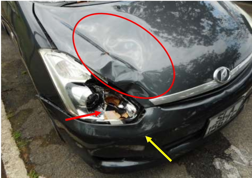
Photo 4 shows a close up view of the Motor Car's frontal portion at the time of my inspection. Its front bonnet (circled), front bumper (yellow arrow) and front right headlamp (red arrow) were damage at the time of my inspection.
