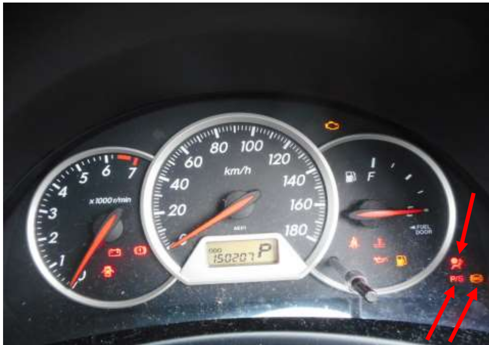
Photo 24 shows the warning light for Anti-Lock Brake System (ABS) and Supplemental Restraint System (SRS) and Electric Power Steering System (EPS) appearing on the instrument panel of the Motor Car during the self-test of its various electronic operating systems when its engine was cranked.
