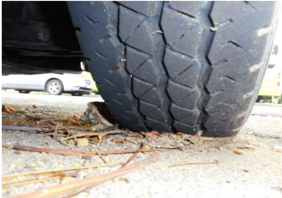
Photo 6 shows the condition of the front right tyre of the Motor Pick-Up, which was observed to be in serviceable condition with remaining tread depth of approximately 6.1mm. The tyre was sufficiently inflated for vehicular operation with no tear, cut or burst mark(s) on the outer and the inner sidewalls as well as across the tread. The 4 tyres of the Motor Pick-Up were wrapped around standard steel wheel rims without any damage.
