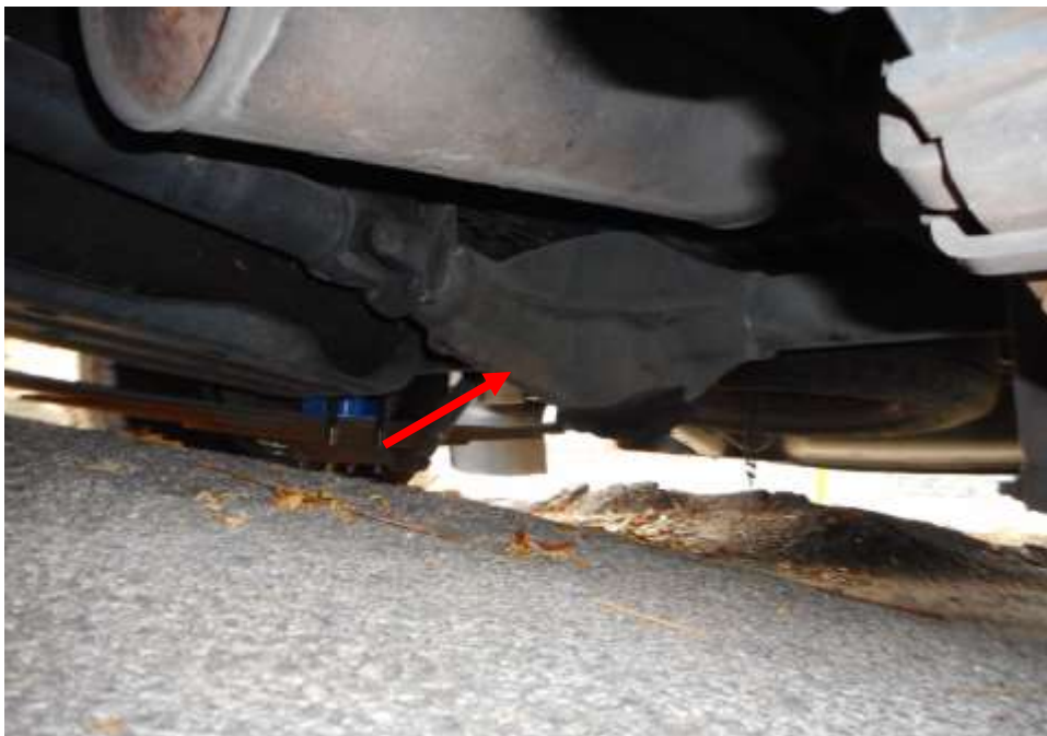
Photo 23 shows the various undercarriage components of the Motor Pick-Up, which had included the drive shaft (red arrow). The various undercarriage components of the Motor Pick-Up were all found to be intact without any visible damage.
