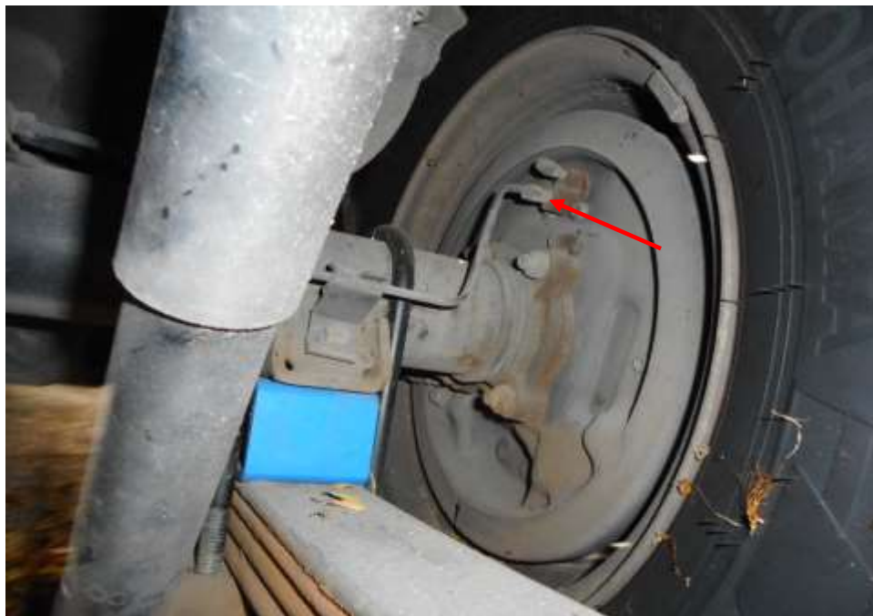
Photo 17 shows the brake hose/pipe (arrowed) at the rear right wheel of the Motor Pick-Up. No leakage of brake fluid was observed. Visual examination of the various components of the braking system like the drum brake, brake booster, brake pedal etc had revealed all to be intact and without visible damage.
