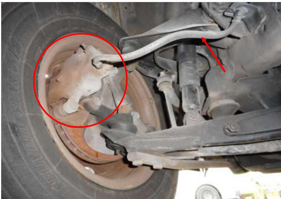
Photo 19 shows the brake hose/pipe (arrowed) at the front left wheel of the Motor Pick-Up. No leakage of brake fluid was observed. Visual examination of the various components of the braking system like the brake caliper (circled), brake booster, brake pedal etc had revealed all to be intact and without visible damage.
