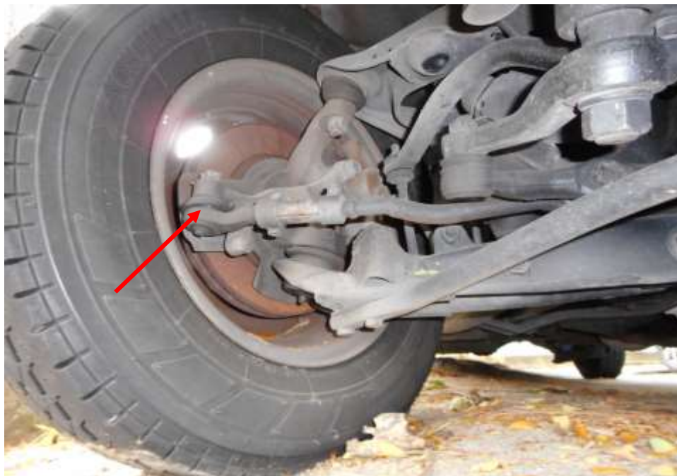
Photo 21 shows the various undercarriage components at the front right wheel of the Motor Pick-Up, in particular the steering tie rod (red arrow). The various steering components were all found to be intact, suggesting that the steering system of the Motor Pick-Up was likely to be in serviceable condition at the material time of accident. There was also no sign of fluid stain observed on the various undercarriage components at the front right wheel of the Motor Pick-Up.
