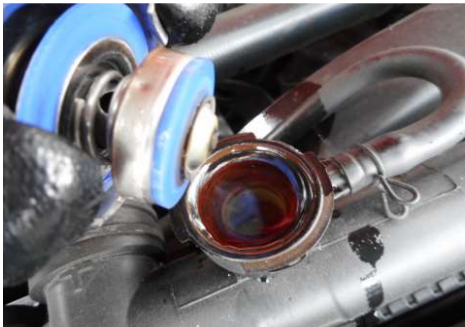
Photo 12 shows checks being carried out to the engine coolant of the Motor Pick-Up at the time of my inspection. The engine coolant was observed to be of sufficient level and without any visible contamination.
