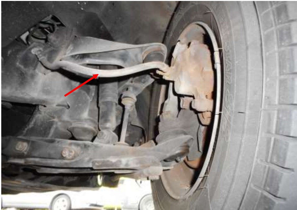
Photo 18 shows the brake hose/pipe (arrowed) at the front right wheel of the Motor Pick-Up. I did not observe any leakage of brake fluid at the time of my inspection of the Motor Pick-Up. Static tests of the Motor Pick-Up's braking system had indicated that there was no internal leakage of pressure/vacuum. The undercarriage components of the Motor Pick-Up were also all found to be intact and without any visible damage.
