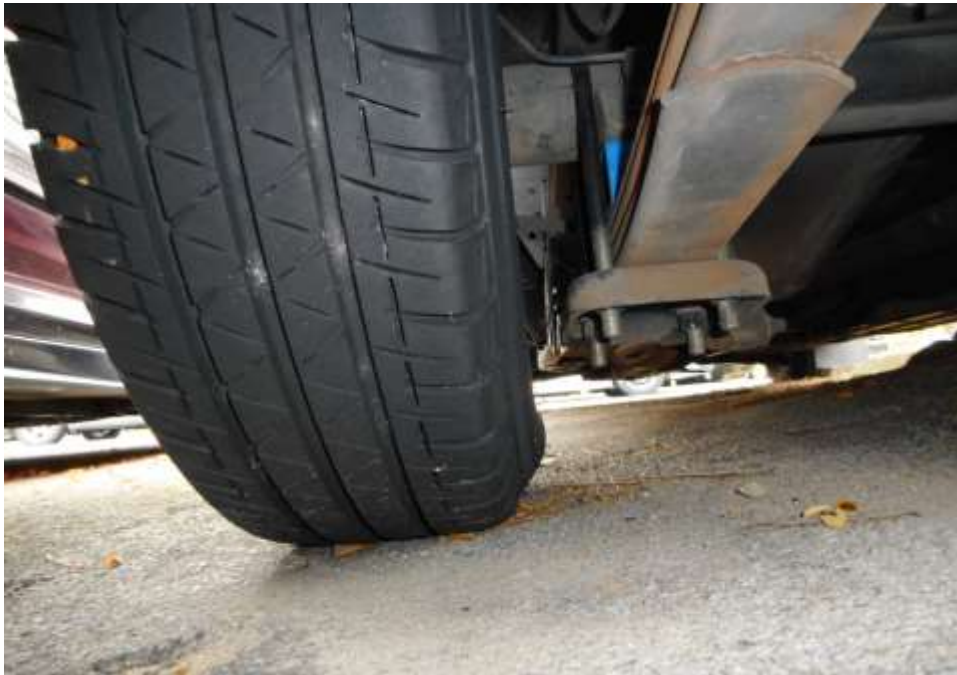
Photo 8 shows the condition of the rear left tyre of the Motor Pick-Up, which was observed to be in serviceable condition with remaining tread depth of approximately 7.3mm. The tyre, which was wrapped around steel wheel rim, was also observed to be sufficiently inflated for vehicular operation. The 4 tyres of the Motor Pick-Up were wrapped around standard steel wheel rims.
