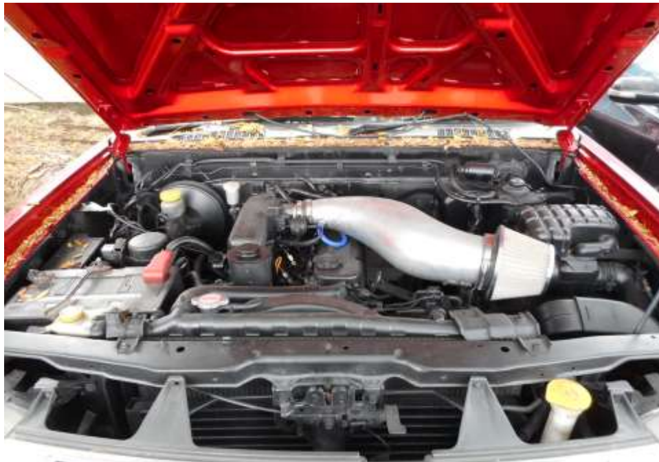
Photo 10 shows a general view of the Motor Pick-Up's engine compartment. The various parts and components inside the engine compartment were unaffected by the accident. There was also no sign(s) or indication(s) of fluid leakage and/or fluid stain within the engine compartment.
