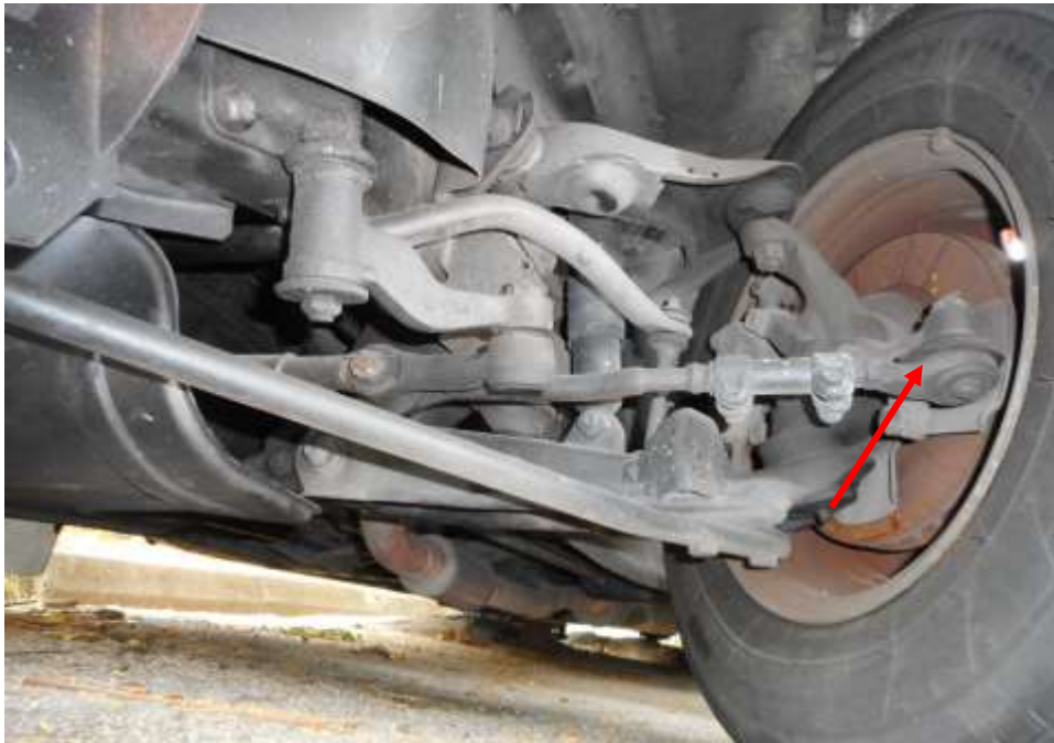
Photo 22 shows the various undercarriage components at the front left wheel of the Motor Pick-Up, which had included the steering tie rod (red arrow). The various undercarriage components of the Motor Pick-Up were all found to be intact without any visible damage.
