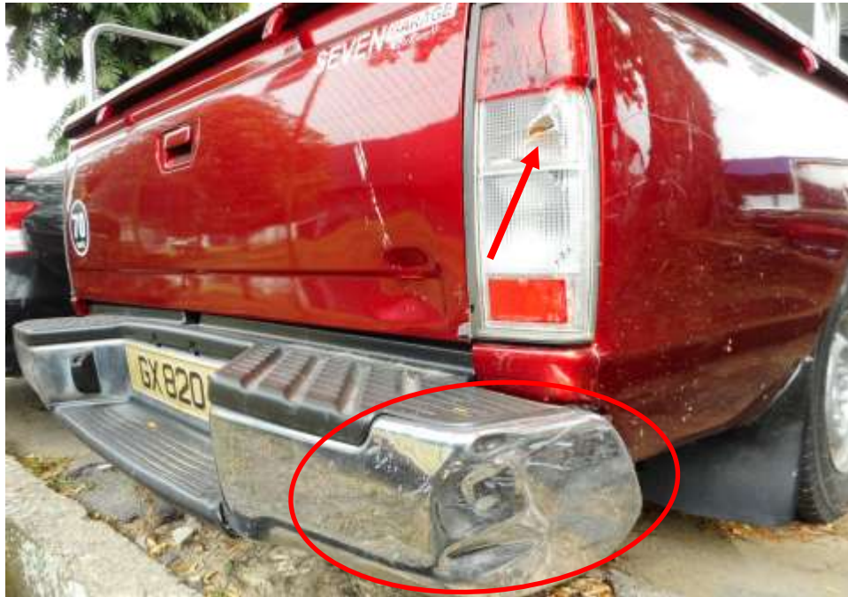
Photo 2 shows the close up view of the Motor Pick-Up's rear body at the time of my inspection. The Motor Pick-Up was observed to have sustained damage at its rear bumper (circled) and rear left brake lamp (arrowed) as a result of the accident.
