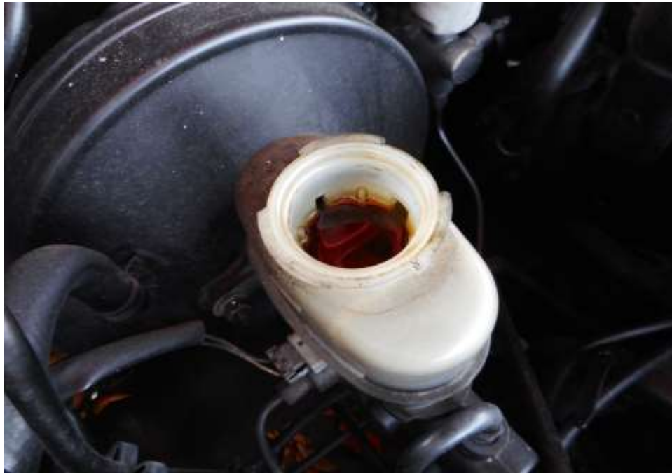
Photo 11 shows the brake fluid reservoir of the Motor Pick-Up at the time of my inspection. The brake fluid was observed to be of sufficient level and without any visible contamination.
