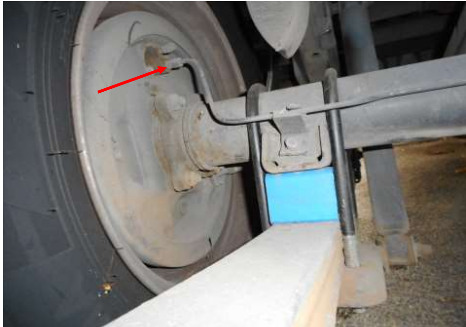
Photo 16 shows the brake hose/pipe (arrowed) at the rear left wheel of the Motor Pick-Up. I did not observe any leakage of brake fluid at the time of my inspection of the Motor Pick-Up. Static tests of the Motor Pick-Up's braking system had indicated that there was no internal leakage of pressure/vacuum. The undercarriage components of the Motor Pick-Up were also all found to be intact and without any visible damage.
