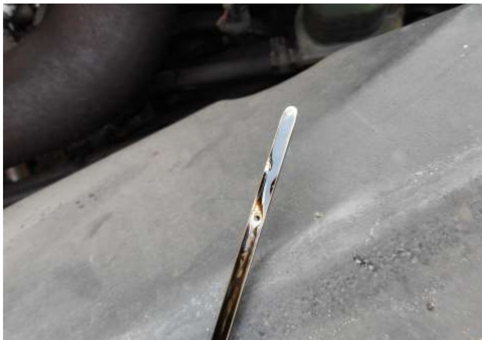
Photo 14 shows the engine oil dip stick of the Motor Pick-Up at the time of my inspection. The engine oil was observed to be of sufficient level and without any visible contamination.
