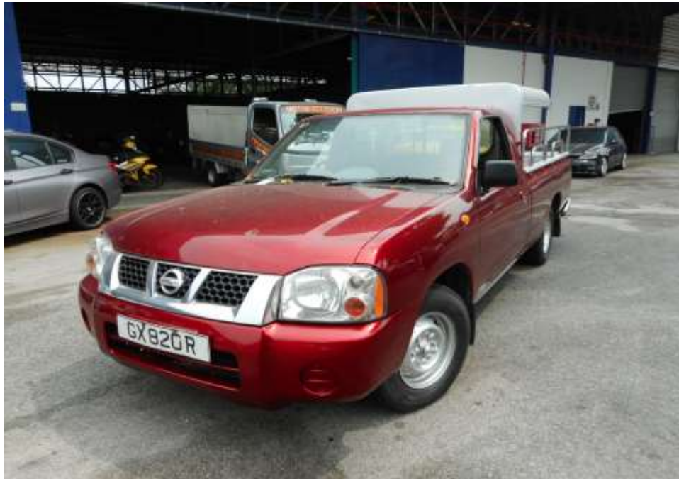
Photo 20 shows the front left wheel of the Motor Pick-Up turned to its full right. During my steering system test, I did not experience any abnormal free play and/or resistance when I had turned the steering wheel towards the left and right. This would suggest that the steering system of the Motor Pick-Up was likely to be in serviceable condition at the material time of accident.
